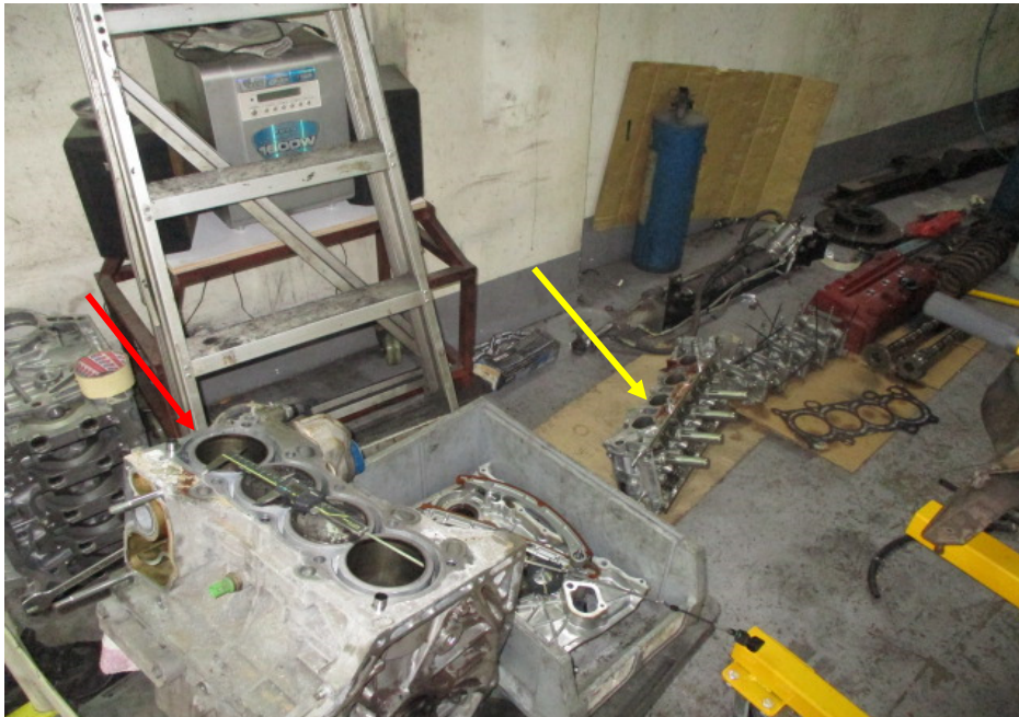
Photo 5 shows the top block (red arrow) of the Honda engine separated from its bottom block (yellow arrow). This was to enable me to carry out measurements of its cylinders, in particular the bore and stroke measurements of each cylinder, which typically can be used to determine the engine displacement or more commonly referred to as engine cc.
