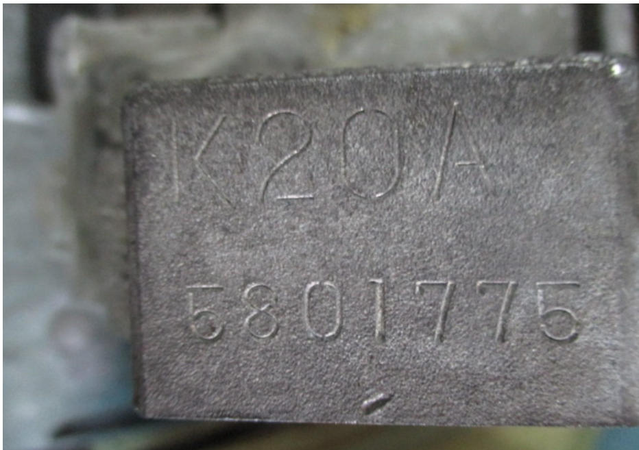
Photo 4 shows the engine number engraved on the housing of the Honda engine that I had inspected. The engine number was K20A5801775.
