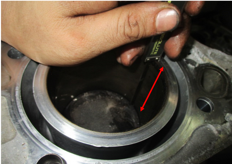
Photo 21 shows measurement being carried out to the stroke (arrowed) of cylinder 4 of the Honda engine. The bore and stroke measurements of the Honda engine were carried out using a digital Vernier Caliper that was calibrated prior to the start of measurements.
