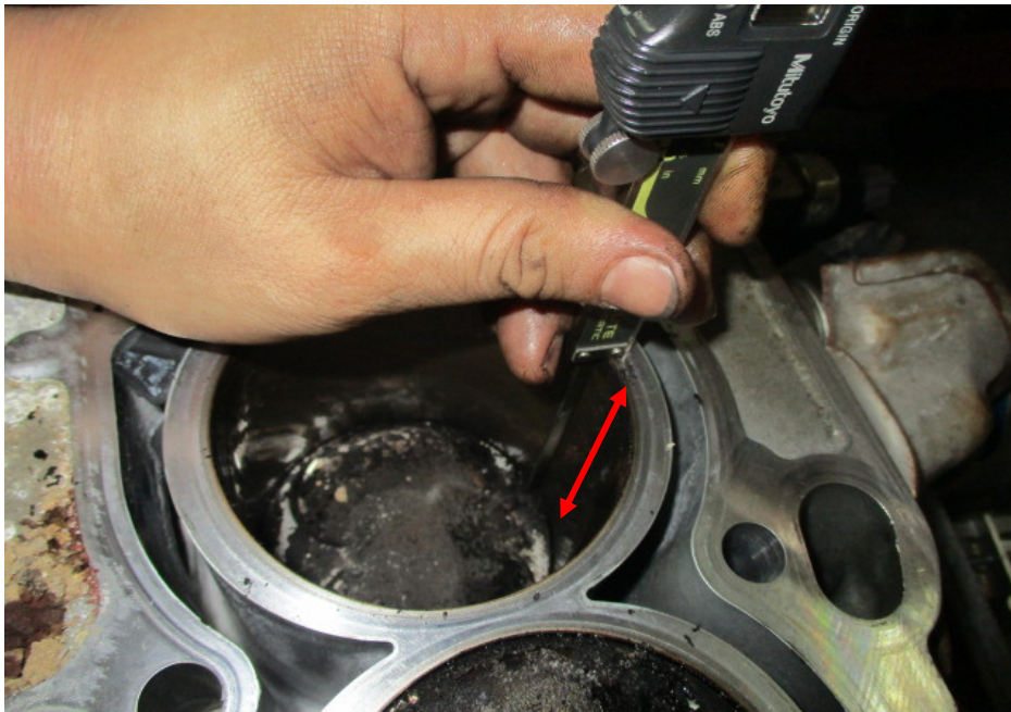
Photo 10 shows measurement being carried out to the stroke (arrowed) of cylinder 1 of the Honda engine. The bore and stroke measurements of the Honda engine were carried out using a digital Vernier Caliper that was calibrated before the start of the measurements,
