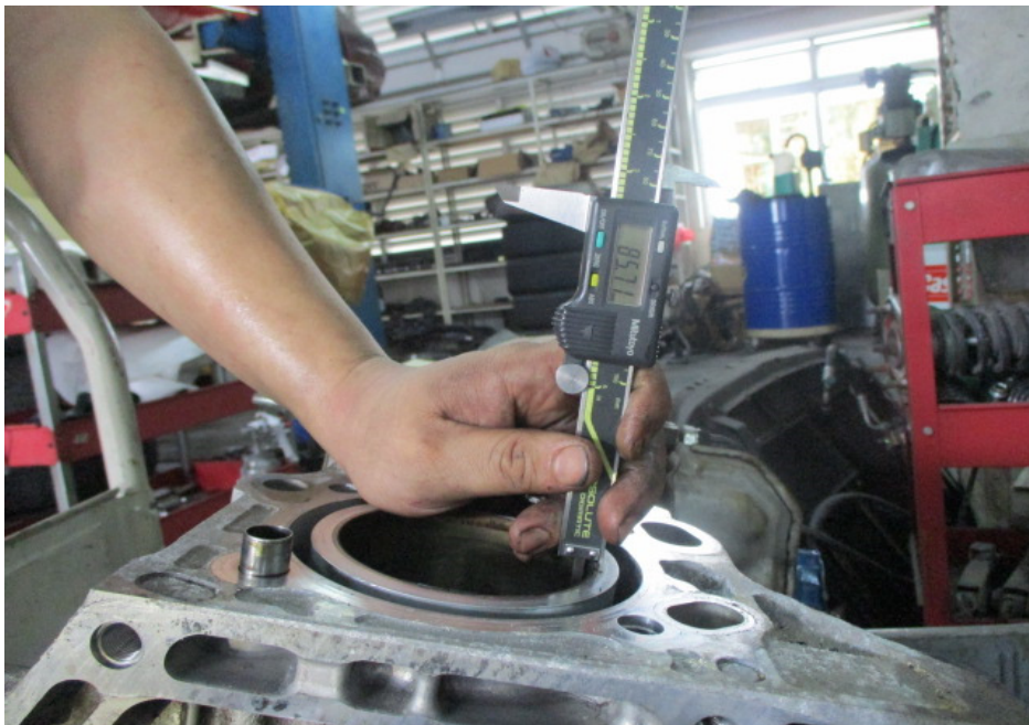
Photo 22 shows the stroke measurement of cylinder 4, which was recorded to be 85.71mm.
