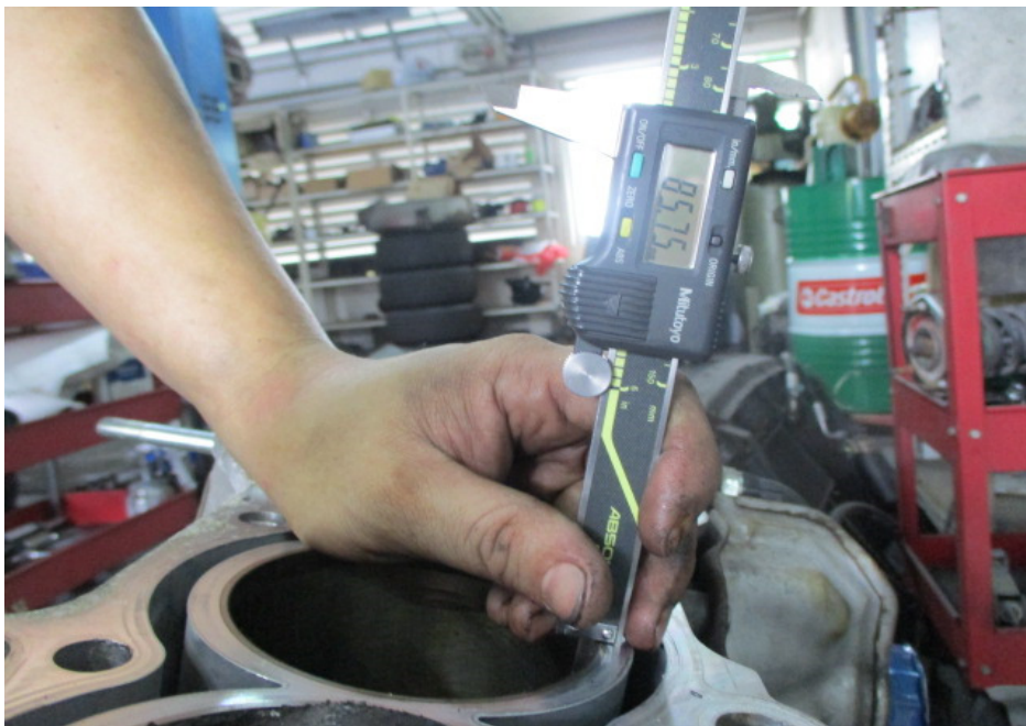
Photo 18 shows the stroke measurement of cylinder 3, which was recorded to be 85.75mm.
