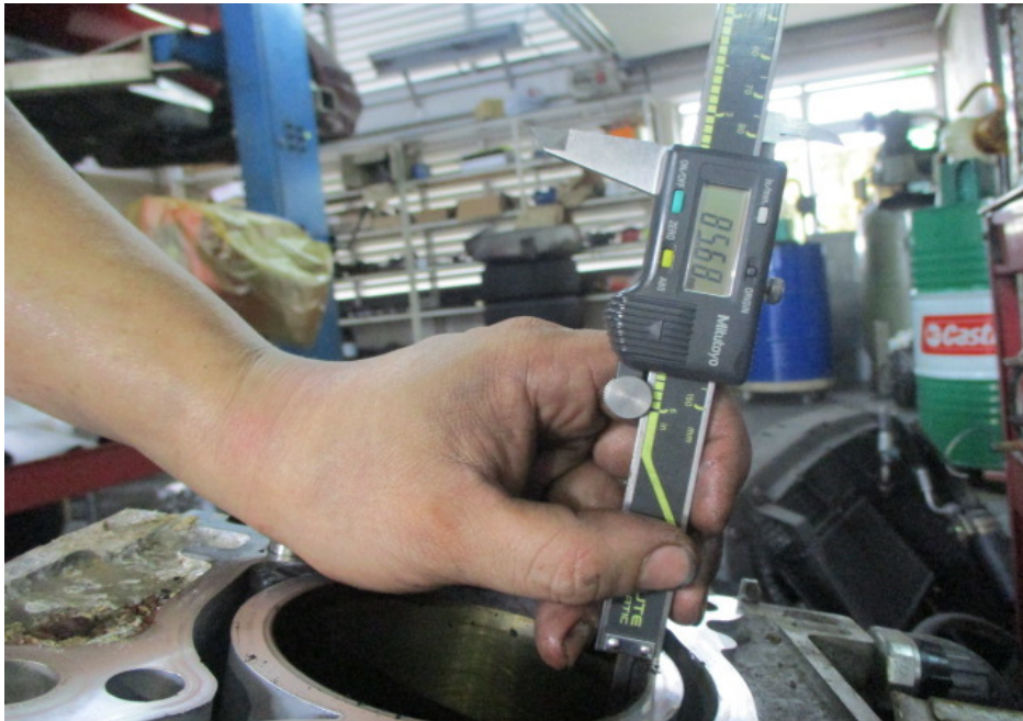
Photo 11 shows the stroke measurement of cylinder 1, which was recorded to be 85.68mm.
