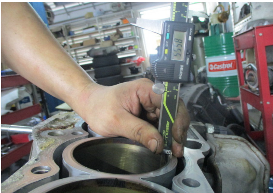
Photo 14 shows the stroke measurement of cylinder 2, which was recorded to be 85.55mm.
