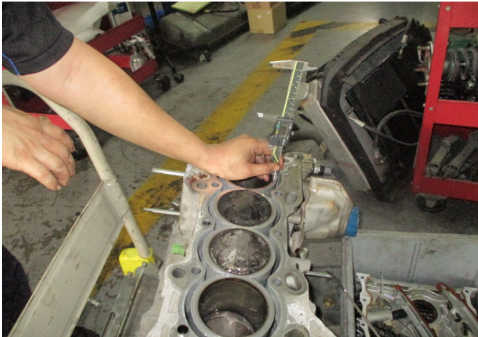
Photo 9 shows measurement being carried out to the stroke of cylinder 1 of the Honda engine. The bore and stroke measurements of the Honda engine were carried out using a digital Vernier Caliper.
