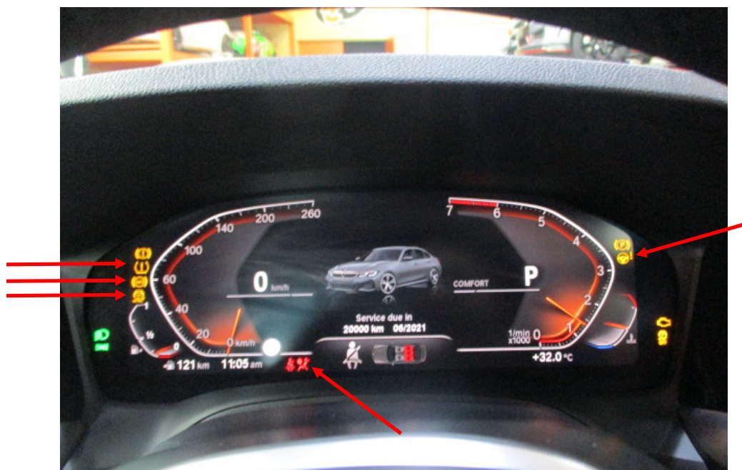
Photo 10 shows the warning lights for the various electronic safety features appearing on the instrument panel of the Motor Car during its self-test when the engine is cranked, in particular the ABS, SRS, IAS, TPM and DSC lights (arrowed).
