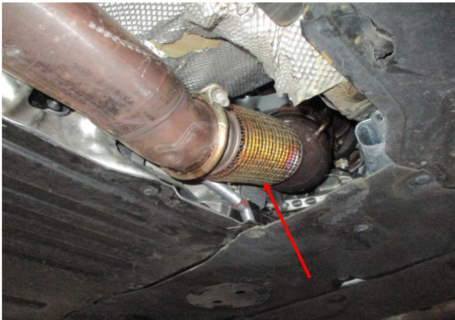
Photo 16 shows the Motor Car's catalytic converter (arrowed). My examination of the Motor Car's exhaust system revealed no sign(s) or indication(s) of any cut or weld marks along its exhaust pipes and on its rear muffler.
