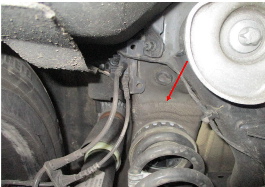
Photo 18 shows the chassis/structural body at the underside rear left of the Motor Car. The original factory sealant (arrowed) at the joints along the chassis/structural body was also untouched, indicating no work was done on the chassis/structural body of the Motor Car and that the chassis/structural body was originally fitted.
