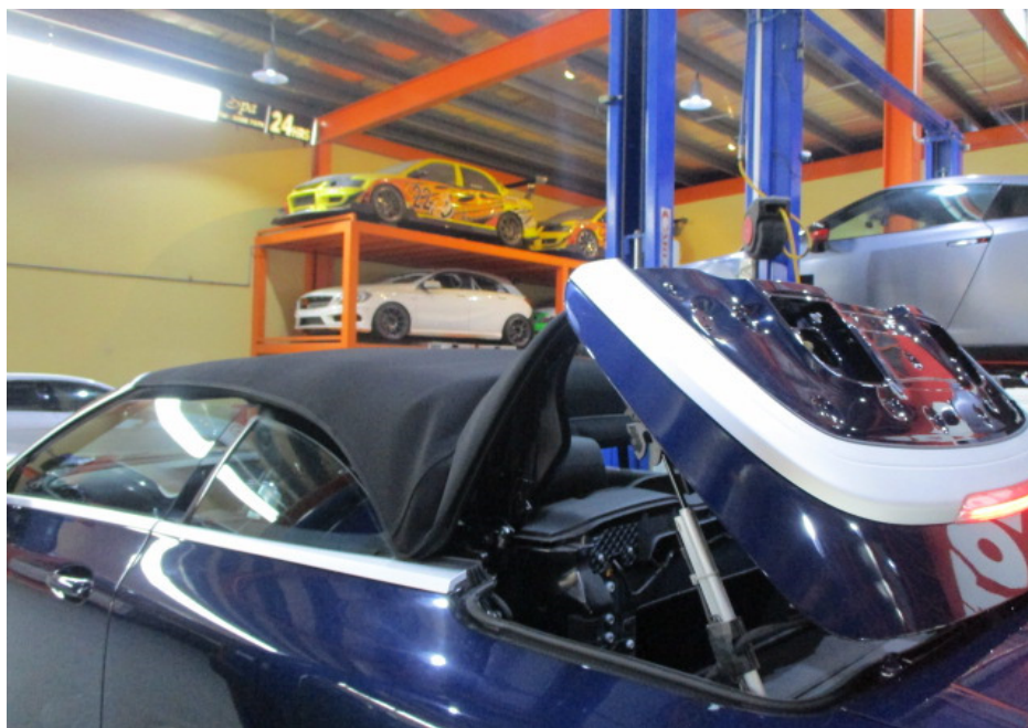
Photo 12 shows the Motor Car's soft top (convertible) being tested. It was observed that as a safety feature, the soft top could only open and close when the Motor Car was in a stationary position. When opened, the soft top is completely folded into the rear boot compartment with no parts protruding out of the Motor Car's body. The soft top was also found adequately secured to the "A" pillar after closing.
