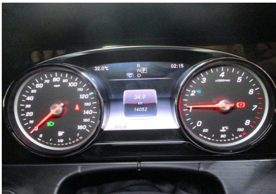
Photo 11 shows the respective warning lights no longer illuminated, indicating that there is no fault detected to the ABS, SRS, EPS, TPM and TCS systems of the Motor Car during the self-test. These electronic systems were hence in working condition at the time of my inspection.
