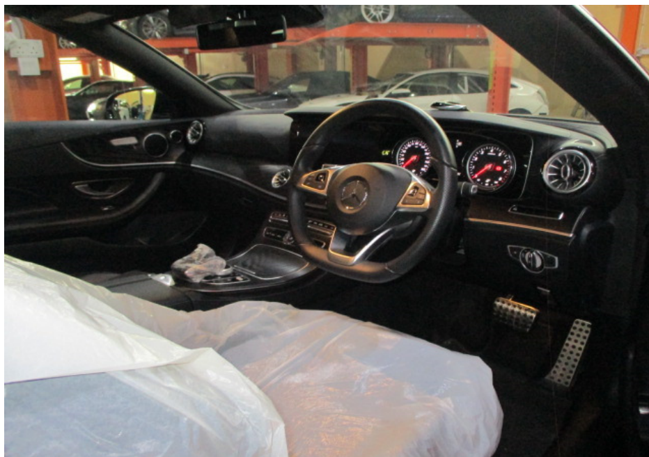
Photo 9 shows the interior compartment of the Motor Car. All the seats of the Motor Car were secured via seat rails to the floorboard and were also all fitted with a retractable seat belt reel and pre-tensioner. The seat belts were tested and able to be fastened into the respective pre-tensions that were fitted on the side of each individual seat.
