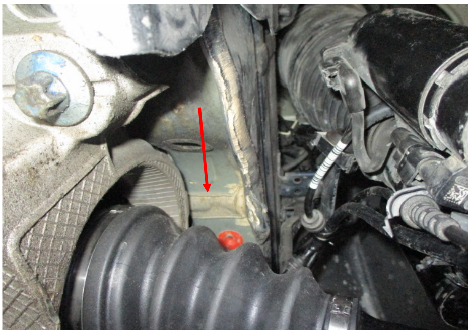
Photo 20 shows the chassis/structural body at the underside front right of the Motor Car. The original factory sealant (arrowed) at the joints along the chassis/structural body was also untouched, indicating no work was done on the chassis/structural body of the Motor Car and that the chassis/structural body was originally fitted.
