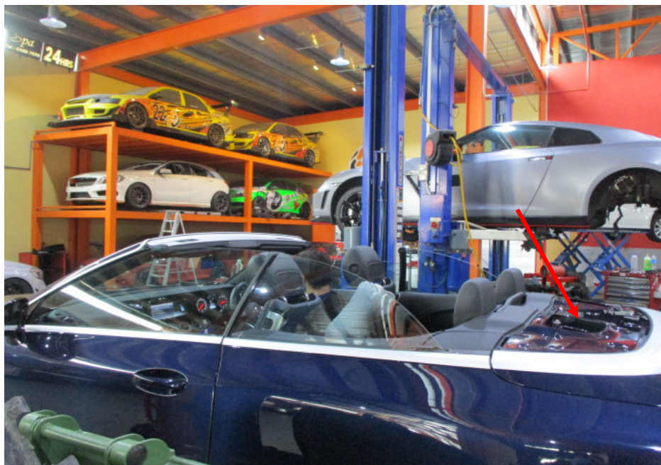
Photo 13 shows the Motor Car's soft top (convertible) completely opened during my testing. It was observed that as a safety feature, the soft top could only open and close when the Motor Car was in a stationary position. When opened, the soft top is completely folded into the rear boot compartment (arrowed) with no parts protruding out of the Motor Car's body. The soft top was also found adequately secured to the "A" pillar after closing.
