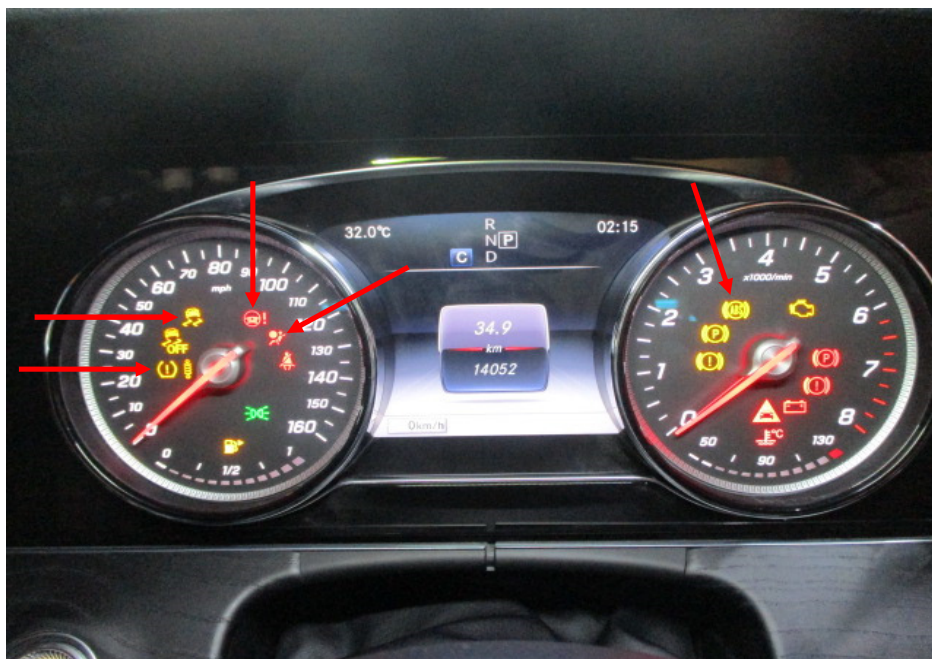
Photo 10 shows the warning lights for the various electronic safety features appearing on the instrument panel of the Motor Car during its self-test when the engine is cranked, in particular the ABS, SRS, EPS, TPM and TCS lights (arrowed).
