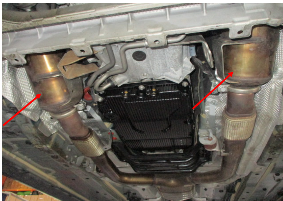
Photo 18 shows the Motor Car's catalytic converters (arrowed). My examination of the Motor Car's exhaust system revealed no sign(s) or indication(s) of any cut or weld marks along its exhaust pipes and on its rear mufflers.
