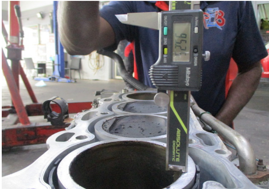
Photo 9 shows the stroke measurement of cylinder 1, which was recorded to be 95.25mm.
