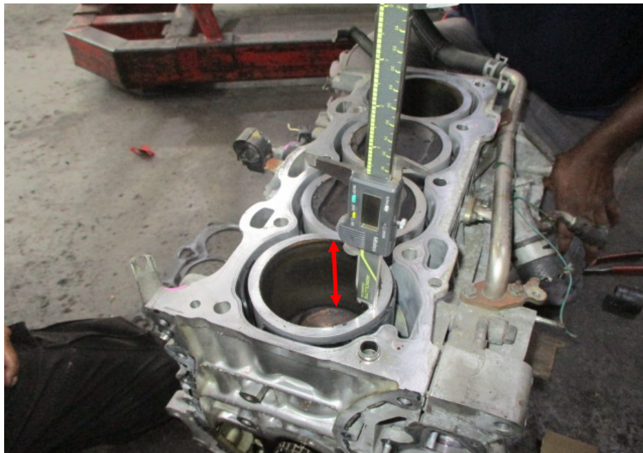
Photo 8 shows measurement being carried out to the stroke (arrowed) of cylinder 1 of the Toyota engine. The bore and stroke measurements of the Toyota engine were carried out using a digital Vernier Caliper that was calibrated before the start of the measurements.
