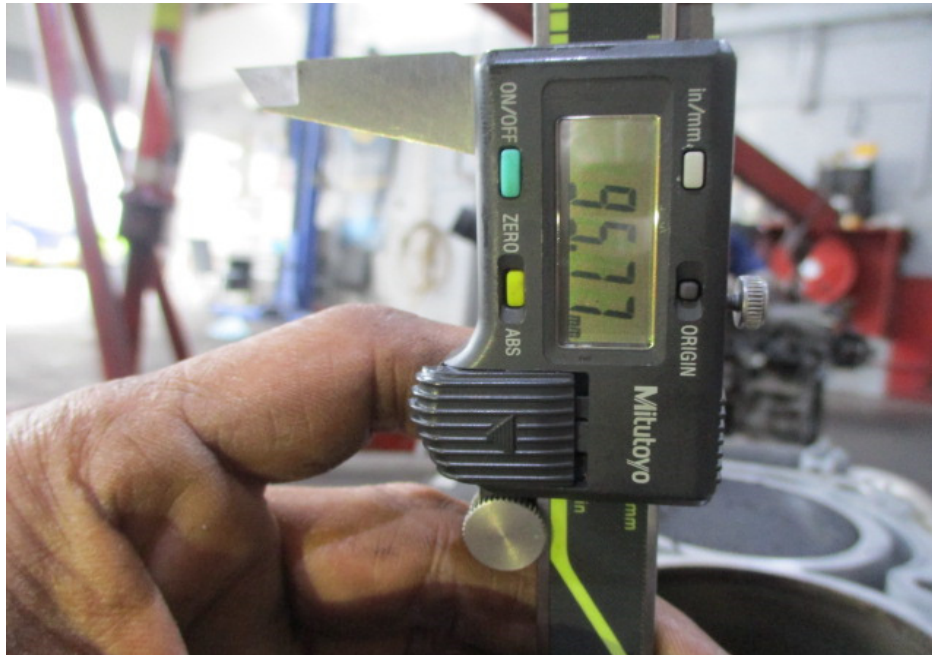
Photo 13 shows the stroke measurement of cylinder 2, which was recorded to be 95.77mm.
