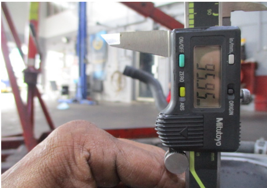
Photo 16 shows the stroke measurement of cylinder 3, which was recorded to be 95.95mm.
