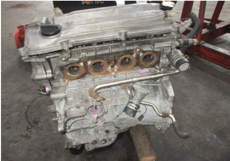
Photo 3 shows a general view of the Toyota engine that I had inspected. My visual examination of the engine housing revealed the housing to be of serviceable/satisfactory condition. There was no crack and/or hole observed on the engine housing.
