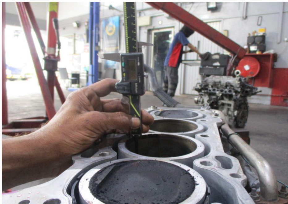
Photo 12 shows measurement of the stroke for cylinder 2 of the Toyota engine that I had inspected. The bore and stroke measurements of the Toyota engine were carried out using a digital Vernier Caliper that was calibrated before the start of the measurements.
