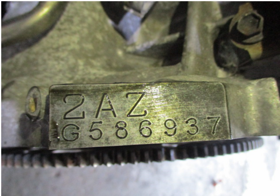
Photo 4 shows the engine number engraved on the housing of the Toyota engine that I had inspected. The engine number was 2AZG586937.
