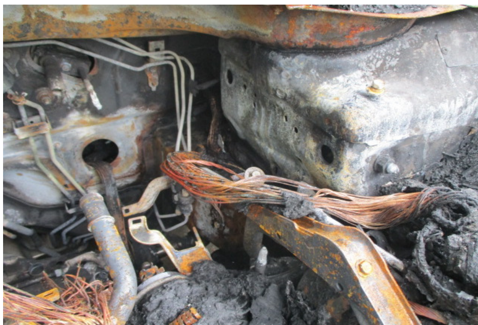
Photo 11 shows a closer view of the wirings at the rear left area of the engine compartment that was burnt to its bare copper state, and in bright reddish colour.
