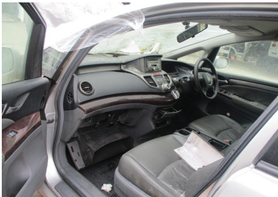
Photo 4 shows the interior compartment of the Insured Vehicle, which was slightly affected at the front area by the fire incident. The front windscreen, instrument panel and front area of the dashboard were amongst the parts within the interior compartment that were affected.
