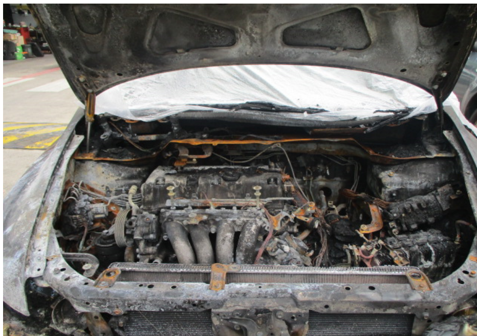
Photo 3 shows the engine compartment of the Insured Vehicle at the time of my inspection. Almost all the parts inside the engine compartment were observed to have been burnt and/or melted. The parts include the air intake manifold, exhaust manifold, engine top cover, battery, wirings, fuse box, various hoses and pipes amongst others.
