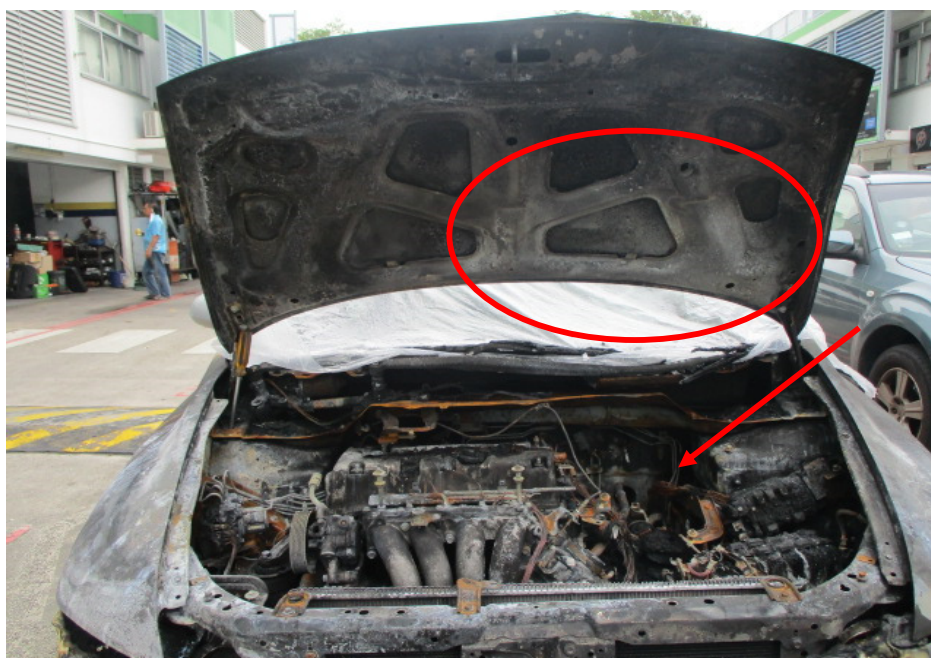
Photo 8 shows the high heat intensity burn marks (circled) that were found on the rear left area of the Insured Vehicle's front bonnet. Such whitish burn marks are a result of exposure to prolonged heat intensity. Following the characteristic of heat rising upwards, the fire to the Insured Vehicle can then be determined to have originated around the rear left area (arrowed) of the Insured Vehicle's engine compartment.
