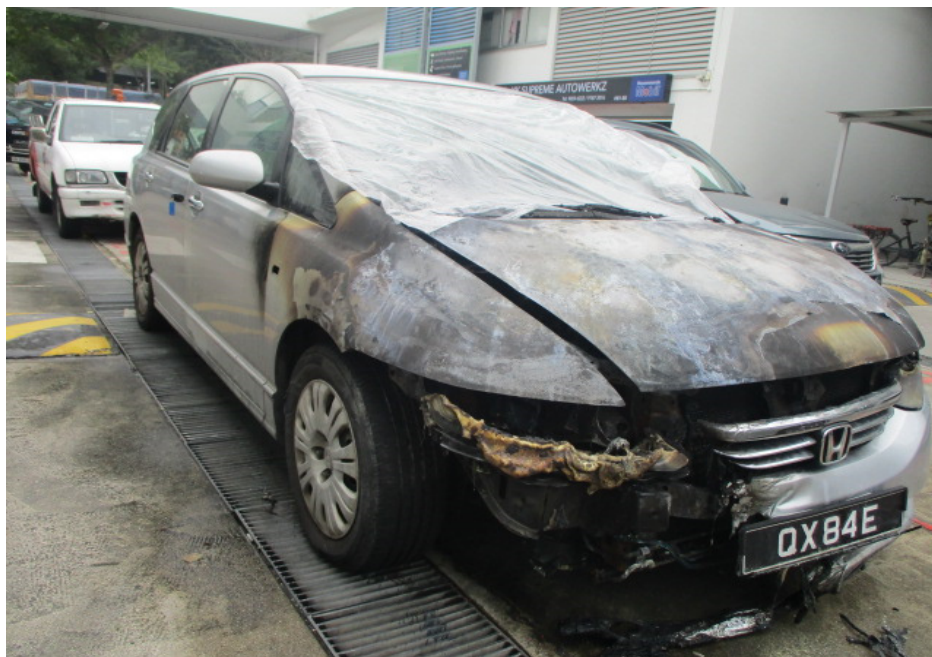
Photo 1 shows a general view of the front right body of the Insured Vehicle at the time of my inspection. The fire damage to the Insured Vehicle was confined to its frontal portion. Its front bumper, front bonnet, front right headlamp, front grille, front right door and front right fender were amongst the exterior body parts that were found to have been affected as a result of the fire.
