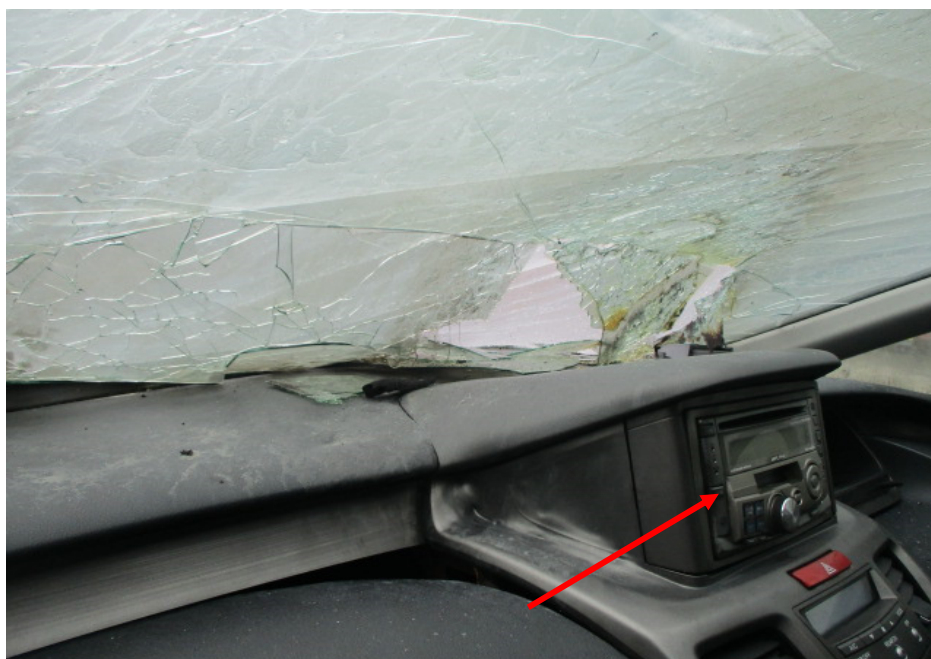
Photo 12 shows the in-car entertainment unit (arrowed) of the Insured Vehicle. Due to the fire, affecting the front dashboard of the Insured Vehicle, the in-car entertainment unit was also affected.
