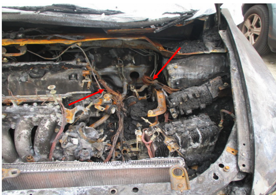
Photo 9 shows the wirings around the rear left area of the Insured Vehicle's engine compartment, which was where the fire to the Insured Vehicle had originated. I had observed several stretches of original wire harnesses (arrowed) around this area to be burnt to its bare copper state, and in bright reddish colour. This indicates internal heating of copper wires, which is a sign of an electrical short circuit.
