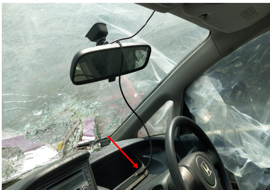
Photo 13 shows an additional wire dangling around the rear-view mirror of the Insured Vehicle, likely for a video camera device. However, there was no video camera device connected to this wire at the time of my inspection. The connecting socket of the wire (arrowed) was seen not connected to any device.
