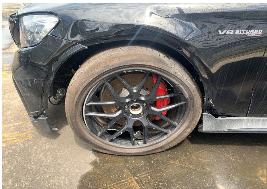
Photo 2 shows a closer view of the damaged front left portion of the Motor Car prior to any repairs being carried out (photograph provided to me). The front bumper, front left fender and left side rocker panel garnish were observed to be damaged. The front left wheel was observed to be shifted backwards, an indication that the front left undercarriage parts of the Motor Car were damaged.
