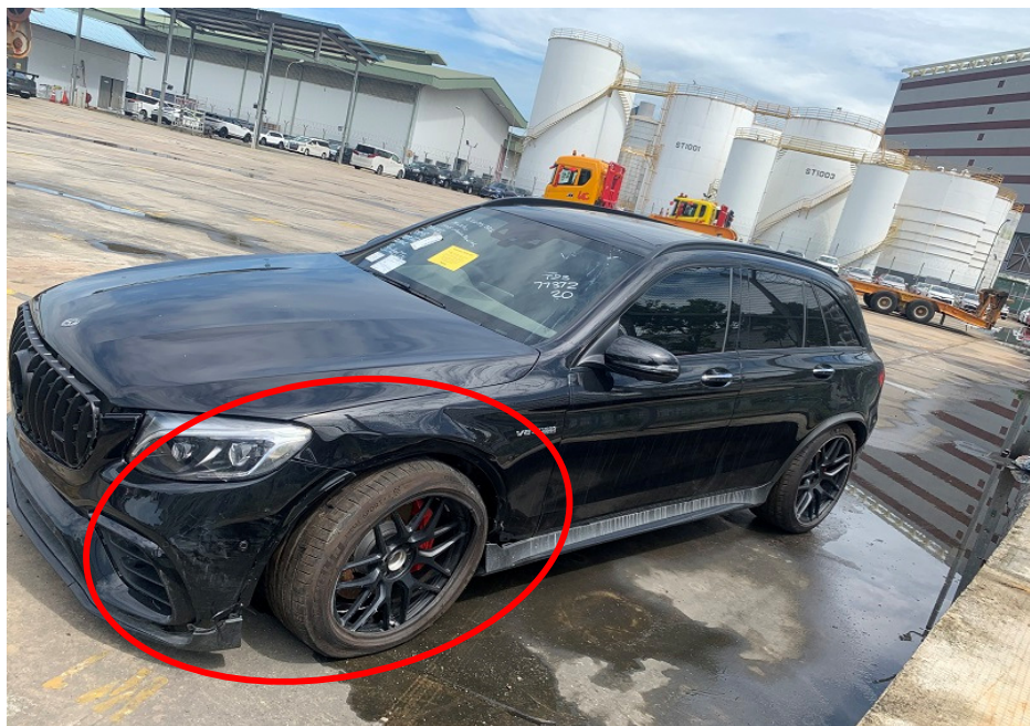
Photo 1 shows the front left body of the Motor Car prior to any repairs being carried out (photograph provided to me). The Motor Car was observed to have sustained damages at its front left portion (circled). The body parts observed to be damaged include the front bumper, front left fender, front left headlamp and front left wheel rim amongst others.
