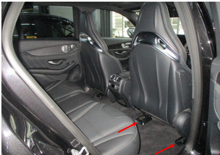
Photo 11 shows the seats of the Motor Car, which were secured via seat rails (arrowed) to the floorboard. All the seats of the Motor Car were fitted with a retractable seat belt reel and pre-tensioner. The seat belts were tested and able to be fastened into the respective pre-tension that were fitted on the side of each individual seat.
