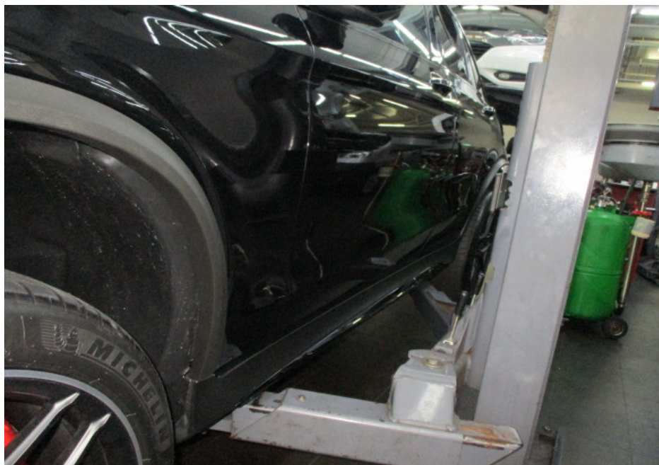
Photo 7 shows a closer view of the front left fender garnish and left side rocker panel garnish of the Motor Car. The body parts at the front left portion of the Motor Car were visually examined and it was observed that the repair/restoration works carried out to the damaged area of the Motor Car (refer photograph 1 & 2 above) were reasonably adequate and in order.
