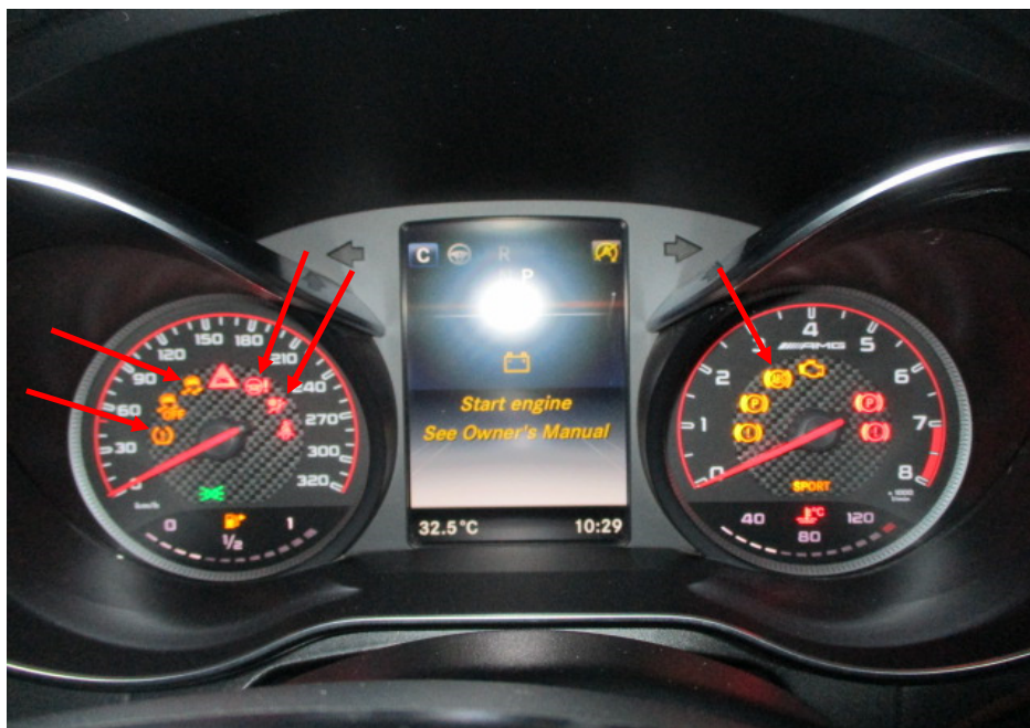
Photo 12 shows the warning lights for the various electronic safety features appearing on the instrument panel of the Motor Car during its self-test when the engine is cranked, in particular the ABS, SRS, EPS, TPM and ESP lights (arrowed).
