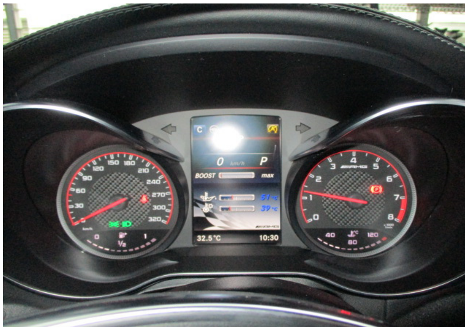
Photo 13 shows the respective warning lights no longer illuminated after the engine was started, indicating that there was no fault detected to the ABS, SRS, EPS, TPM and ESP systems of the Motor Car during the self-test. These electronic systems were hence in working condition at the time of my inspection.
