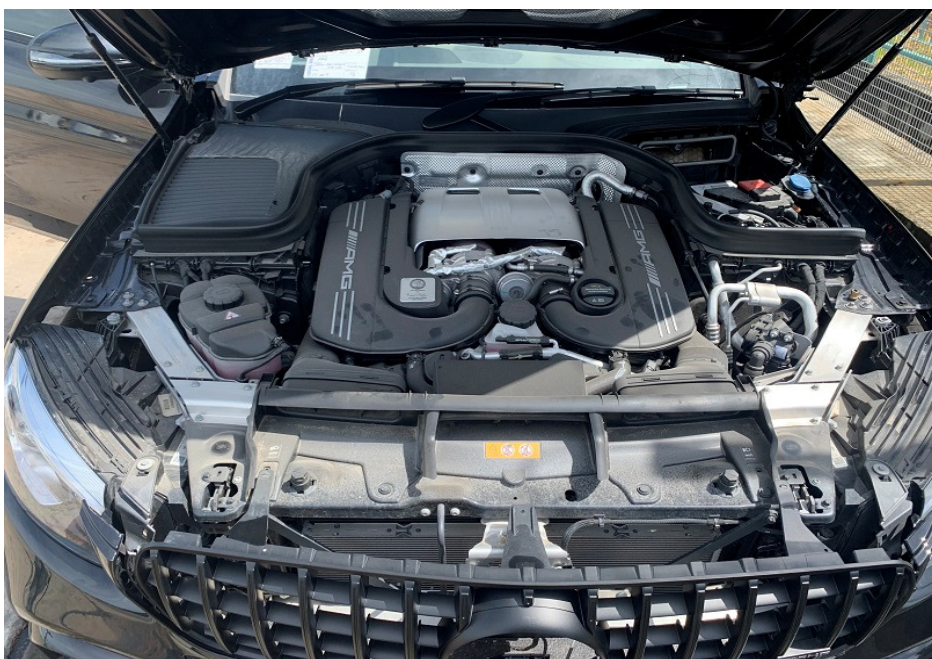
Photo 4 shows the engine compartment of the Motor Car prior to any repairs being carried out (photograph provided to me). Parts and components within the engine compartment were observed to be intact and unaffected.
