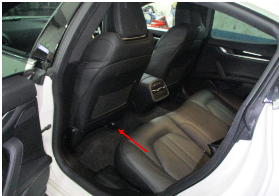
Photo 13 shows the seats of the Motor Car, which were secured via seat rails (arrowed) to the floorboard. All the seats of the Motor Car were fitted with a retractable seat belt reel and pre-tensioner. The seat belts were tested and able to be fastened into the respective pre-tension that were fitted on the side of each individual seat.
