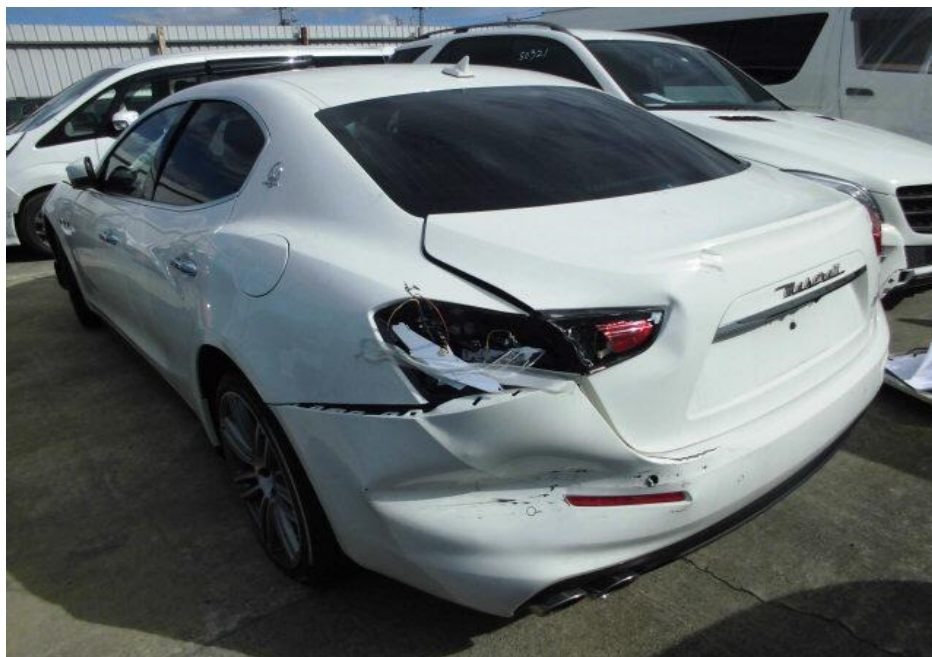
Photo 3 shows the rear left body of the Motor Car prior to any repairs being carried out (photograph provided to me). Apart for the front left portion, the Motor Car had also sustained damage to its rear left portion. Body parts damage include the rear bumper, rear left fender, rear left taillamp, rear bootlid and rear left bootlid lamp amongst others.
