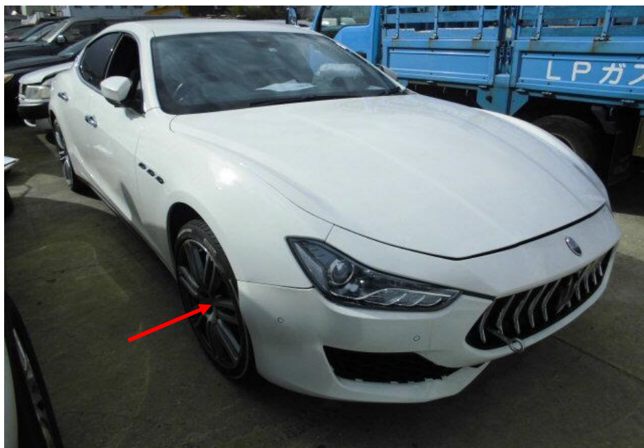
Photo 2 shows the front right body of the Motor Car prior to any repairs being carried out (photograph provided to me). The front right wheel (arrowed) and front left wheel were both oriented inwards of the Motor Car (refer to photograph 1 above). This would indicate damage to the front undercarriage parts of the Motor Car, likely to be the front left undercarriage parts since the front left wheel rim was damaged.
