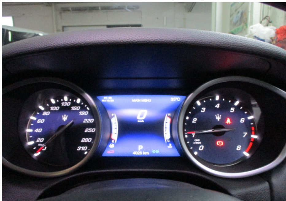
Photo 15 shows the respective warning lights no longer illuminated after the engine was started, indicating that there was no fault detected to the ABS, SRS, TPM and TCS systems of the Motor Car during the self-test. These electronic systems were hence in working condition at the time of my inspection.
