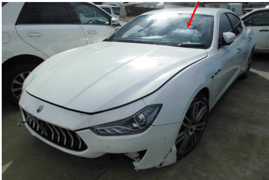
Photo 1 shows the front left body of the Motor Car prior to any repairs being carried out (photograph provided to me). The Motor Car was observed to have sustained damages at its front left portion. The body parts observed to be damaged include the front bumper, front bumper left lower grille and front left wheel rim. The front left passenger airbag was also observed to be deployed (arrowed).
