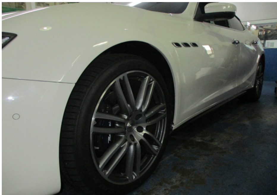
Photo 7 shows a closer view of the front left wheel rim of the Motor Car. The body parts at the front left portion of the Motor Car were visually examined and it was observed that the repair/restoration works carried out to the damaged area of the Motor Car (refer photograph 1 above) were reasonably adequate and in order.
