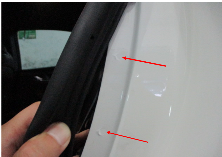
Photo 23 shows the rear left "C" pillar of the Motor Car. I did not find any weld marks other than original spot weld marks (arrowed) on the rear left "C" pillar of the Motor Car. In general, I had found the non-detachable body panels of the Motor Car to be originally fitted at the time of my inspection.
