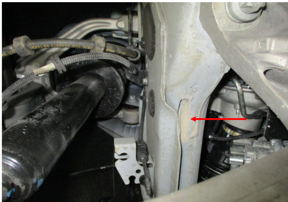
Photo 22 shows the chassis/structural body at the underside front left of the Motor Car. The original factory sealant (arrowed) at the joints along the chassis/structural body was also untouched, indicating no work was done on the chassis/structural body of the Motor Car and that the chassis/structural body was originally fitted.
