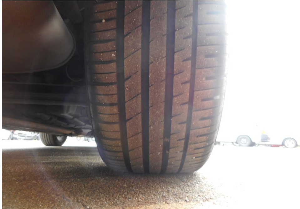
Photo 7 shows the condition of the rear right tyre of the Motor Car, which was observed to be in serviceable condition with remaining tread depth of approximately 4.5mm. The tyre, which was wrapped around standard alloy wheel rim, was also observed to be sufficiently inflated for vehicular operation.
