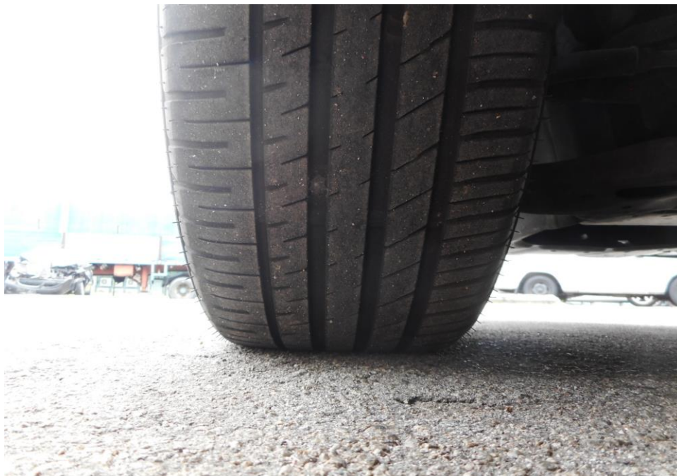
Photo 9 shows the condition of the rear right tyres of the Motor Car, which were observed to be in serviceable condition with remaining, tread depth of approximately 3.9mm. There was also no tear, cut or burst mark(s) on the outer and the inner sidewalls as well as across the tread of the 4 tyres that were fitted on the Motor Car.
