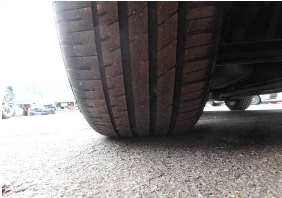
Photo 8 shows the condition of the rear left tyres of the Motor Car, which was observed to be in serviceable condition with remaining tread depth of approximately 3.9mm. The tyres, which were wrapped around standard alloy wheel rim, were also observed to be sufficiently inflated for vehicular operation. There was also no damage found on all 4 alloy wheel rims of the Motor Car.
