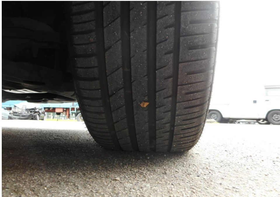
Photo 6 shows the condition of the front right tyre of the Motor Car, which was observed to be in serviceable condition with remaining tread depth of approximately 4.3mm. The tyre, which was wrapped around standard alloy wheel rim, was also observed to be sufficiently inflated for vehicular operation. There was no tear, cut or burst mark(s) on the outer and the inner sidewalls as well as across the tread of the 4 tyres that were fitted on the Motor Car.
