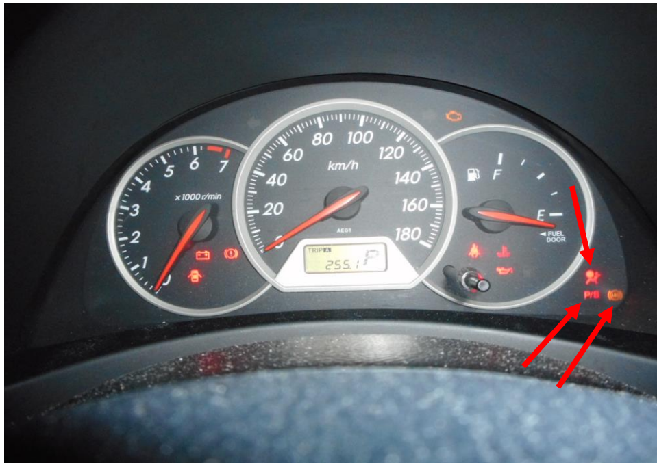
Photo 22 shows the warning light for Anti-Lock Brake System (ABS), Supplemental Restraint System (SRS) and Electric Power Steering System (EPS) appearing on the instrument panel of the Motor Car during the self-test of its various electronic operating systems when its engine was cranked.
