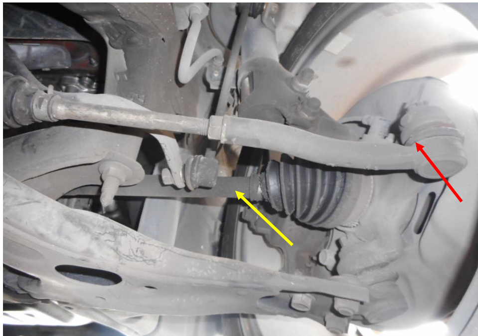
Photo 15 shows the various undercarriage components at the front right wheel of the Motor Car, in particular the steering tie rod end (red arrowed) and drive shaft (yellow arrow). The various steering components were all found to be intact, suggesting that the steering system of the Motor Car was likely to be in serviceable condition at the material time of accident. There was also no sign of fluid stain(s) observed on the various undercarriage components.
