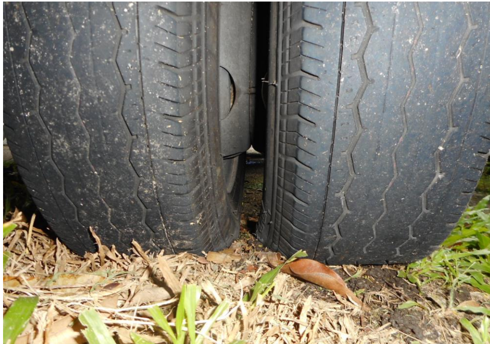
Photo 10 shows the condition of the rear right tyres of the Motor Lorry, which observed to be in serviceable condition with remaining tread depth of approximately 2mm. The tyres, which were wrapped around standard steel wheel rim, were also observed to be sufficiently inflated for vehicular operation.
