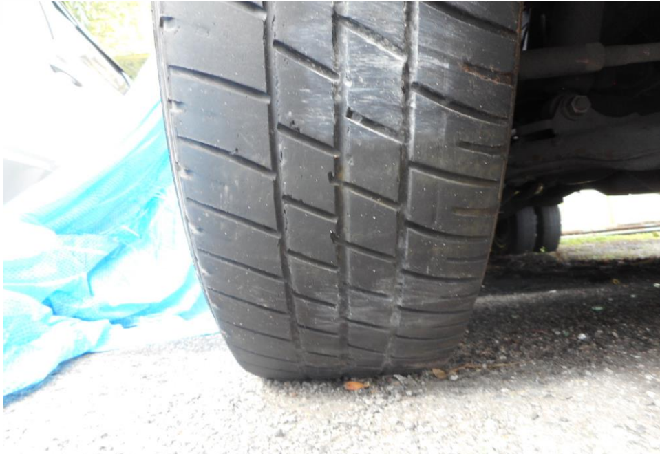
Photo 9 shows the condition of the front right tyre of the Motor Lorry, which was observed to be in serviceable condition with remaining tread depth of approximately 2.3mm. The tyre, which was wrapped around standard steel wheel rim, was also observed to be sufficiently inflated for vehicular operation.
