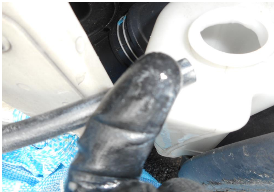
Photo 15 shows the engine coolant reservoir of the Motor Lorry at the time of our inspection. The coolant fluid was observed to be of sufficient level and without any visible contamination.
