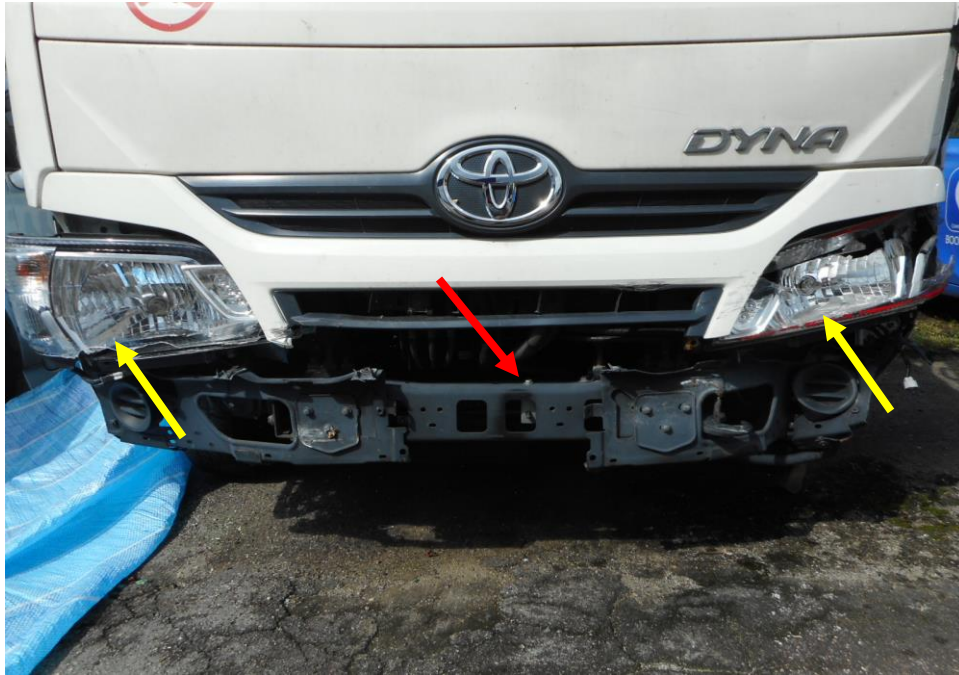
Photo 3 shows the close up view of the front portion of the Motor Lorry at the time of our inspection. The Motor Lorry was observed to have sustained damages to front bumper (red arrow) and its front left and right headlamps (yellow arrow) due to the accident's impact.
