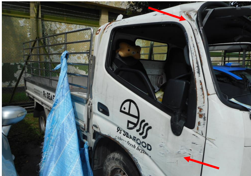
Photo 4 shows the close up view of the right door of the Motor Lorry at the time of our inspection. The Motor Lorry right door (arrowed) was observed to have sustained damages due to the accident.
