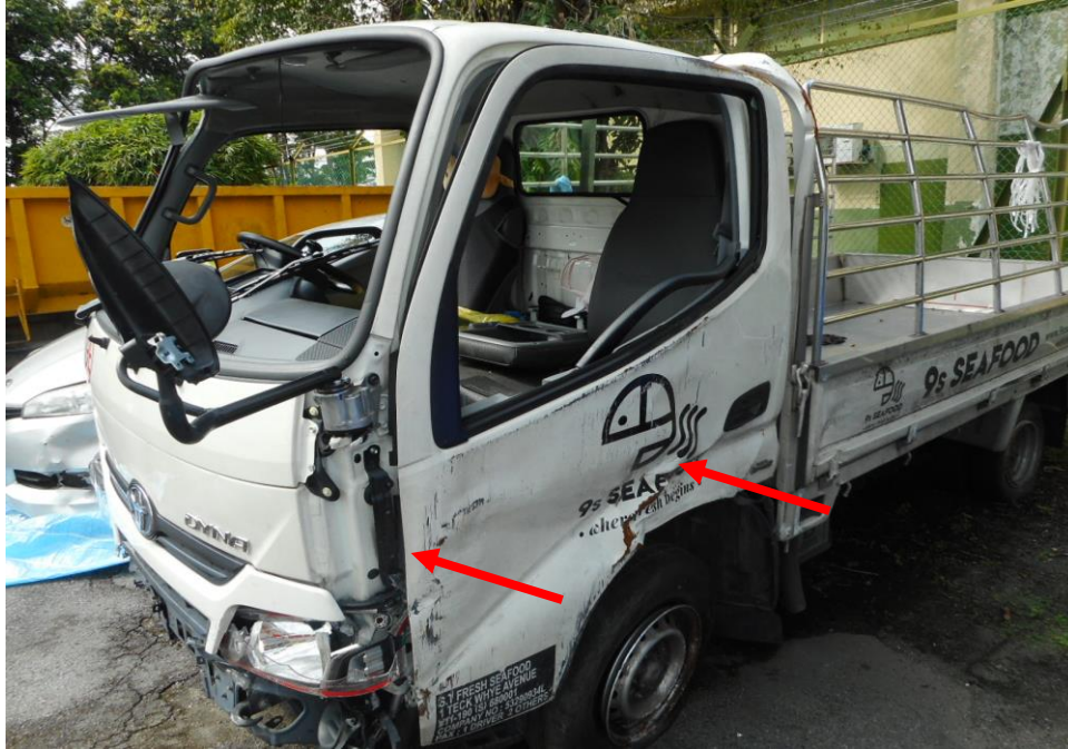
Photo 5 shows the close up view of the left door of the Motor Lorry at the time of our inspection. The Motor Lorry was observed to have sustained damages to its left door (arrowed) as result of the accident.
