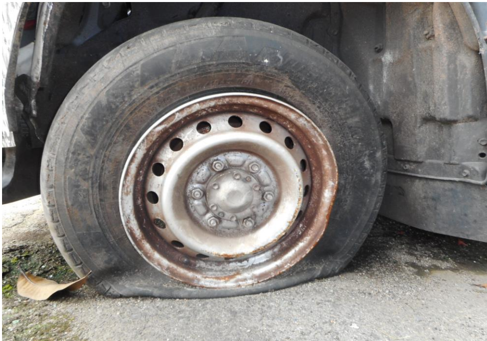
Photo 12 shows the condition of the front right tyre of the Motor Lorry, the tyre were observed to have slipped off the rim and deflated as a result of the accident, tread depth of approximately 2.1mm.
