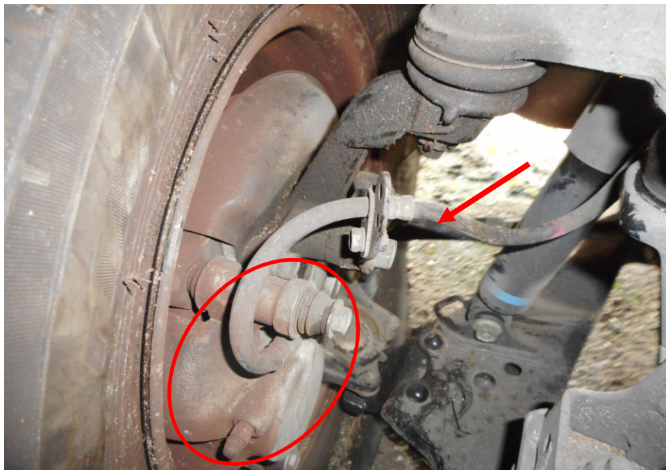
Photo 20 shows the various undercarriage components at the front left wheel of the Motor Lorry, in particular the brake hose (arrowed) and callipers (circled). The various undercarriage components of the Motor Lorry were all found to be intact without any visible damage. There was also no sign of fluid stain(s) observed on the various undercarriage components.
