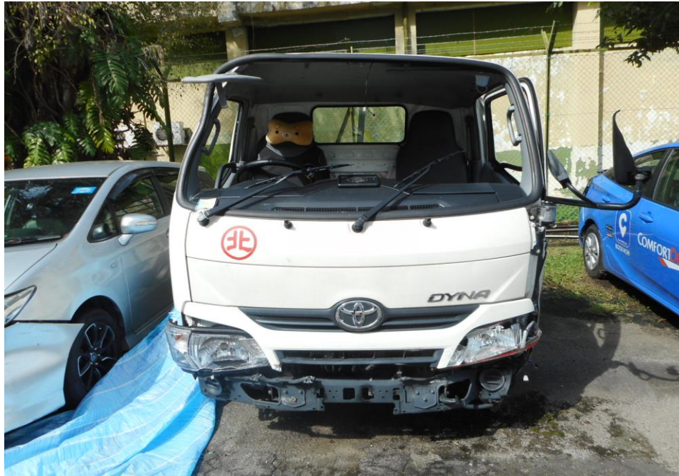
Photo 1 shows a general view of the front windscreen and body panel of the Motor Lorry at the time of our inspection. The Motor Lorry was observed to have sustained damage at its front cabin, front windscreen, front bumper, both front headlamps, left and right doors as well as its rear left body panel were damaged as a result of the accident.
