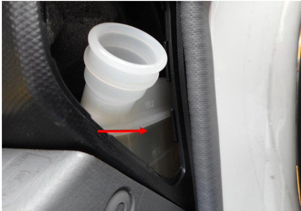
Photo 14 shows the brake fluid reservoir of the Motor Lorry at the time of our inspection. The brake fluid was observed to be of sufficient level and without any visible contamination (arrowed).
