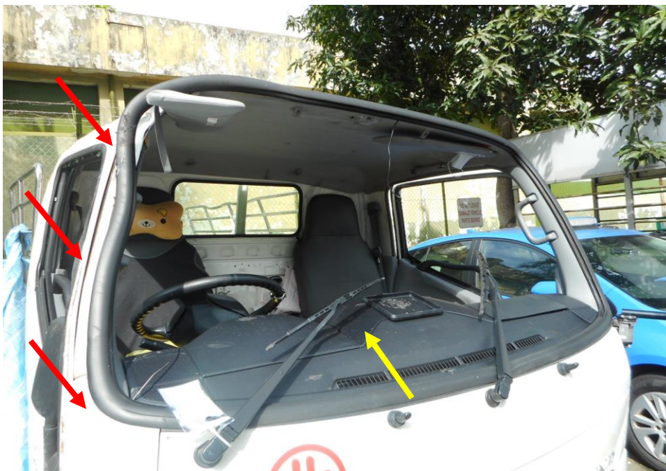
Photo 2 shows the close up view of the front portion of the Motor Lorry at the time of our inspection. The Motor Lorry was observed to have sustained damages to its front cabin (red arrow) and its front windscreen (yellow arrow) due to the accident's impact.
