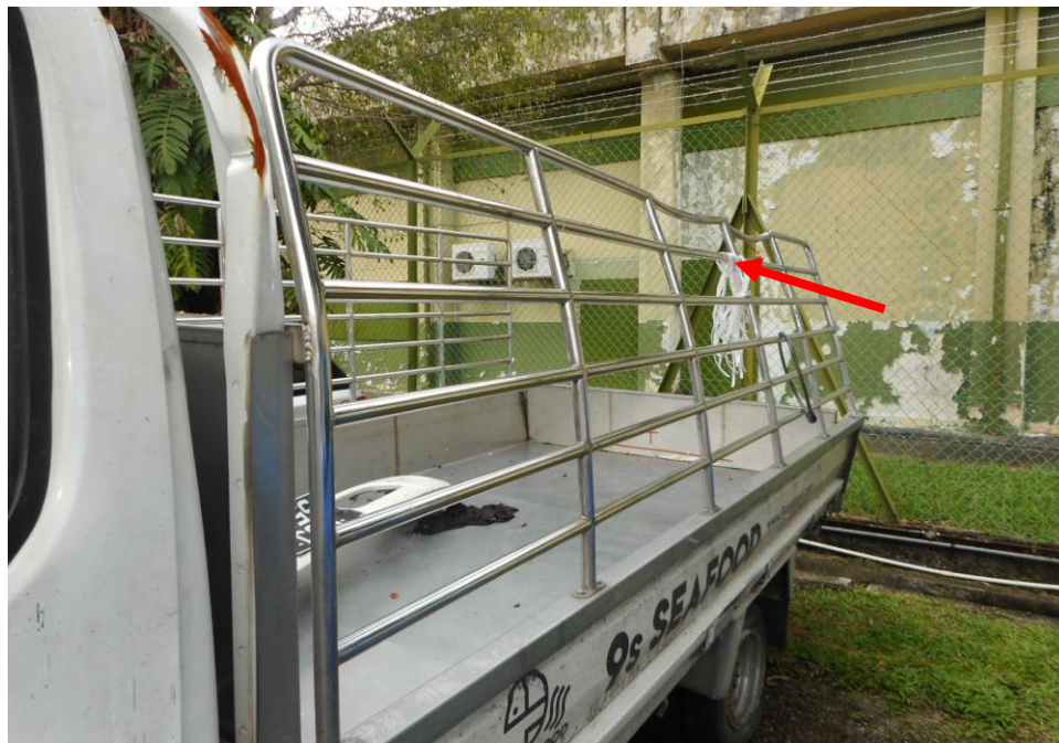
Photo 6 shows a close up view of the Motor Lorry's rear left body at the time of my inspection. The left rear body panel (arrowed) of the Motor Lorry was observed to have been damaged as a result of the accident.
