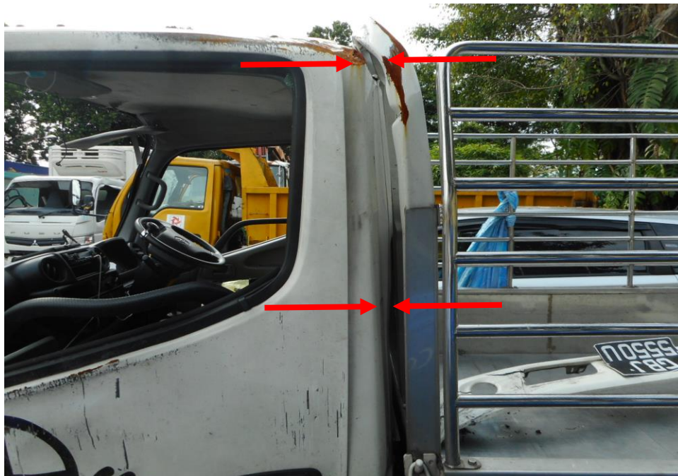
Photo 13 shows the induced damage to the cabin (arrowed) of the Motor Lorry's which immobilised the opening and viewing of the various parts and components inside the engine compartment, a result of the accident.
