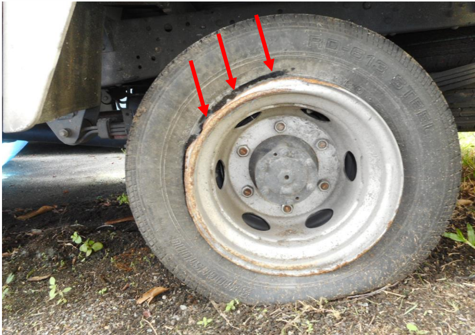
Photo 11 shows the condition of the rear left tyres of the Motor Lorry, which were observed to cut by its rims (arrowed) and deflated as a result of the accident, tread depth of approximately 2.2mm.
