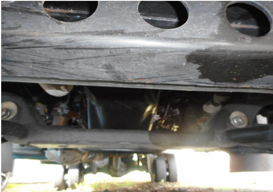
Photo 16 shows the undercarriage of the engine of the Motor Lorry at the time of our inspection. There was no sign(s) and indication(s) of fluid stain within the engine undercarriage area.
