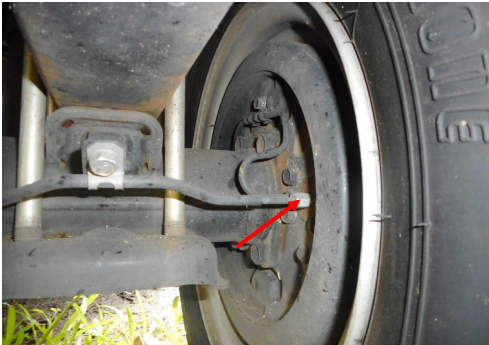
Photo 22 shows the various undercarriage components at the rear right wheel of the Motor Lorry, in particular the brake hose and drum brake (arrowed). The various undercarriage components of the Motor Lorry were all found to be intact without any visible damage. There was also no sign of fluid stain(s) observed on the various undercarriage components.
