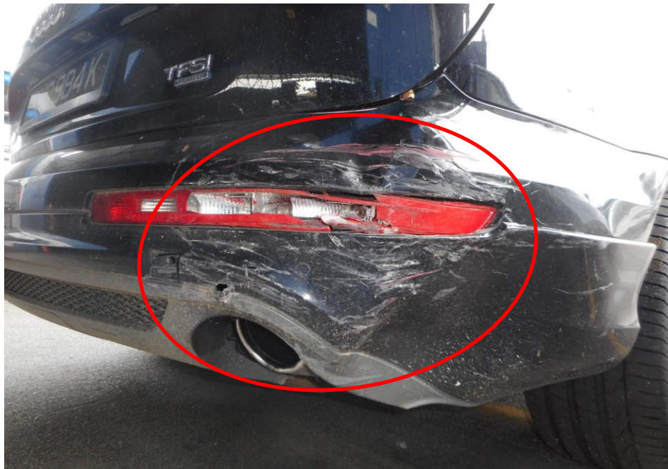
Photo 3 shows a close up view of the rear body of the Motor Car at the time of my inspection. The Motor Car was observed to visually sustain damage at its rear bumper (circled) at the time of inspection.
