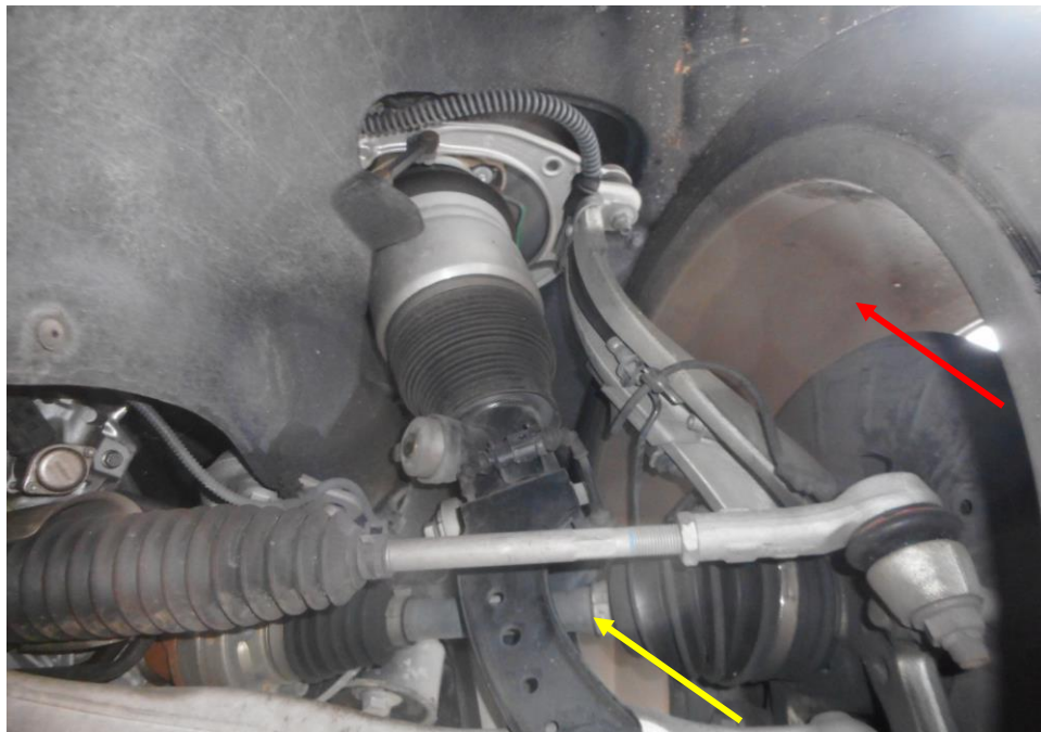
Photo 17 shows the various undercarriage components at the front right wheel of the Motor Car, in particular the steering tie rod end (arrowed) and drive shaft (yellow arrow). The various steering components were all found to be intact, suggesting that the steering system of the Motor Car was likely to be in serviceable condition at the material time of accident. There was also no sign of fluid stain(s) observed on the various undercarriage components.
