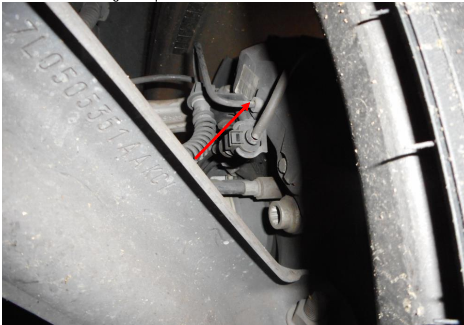
Photo 19 shows the brake pipe (arrowed) at the rear right wheel of the Motor Car. I did not observe any leakage of brake fluid at the time of my inspection of the Motor Car. My static tests of the Motor Car's braking system, along with my visual examination of the various mechanical components in the braking system, had indicated that there was no internal leakage of pressure/vacuum. Hence the braking system of the Motor Car was likely to be in serviceable condition at the material time of accident.
