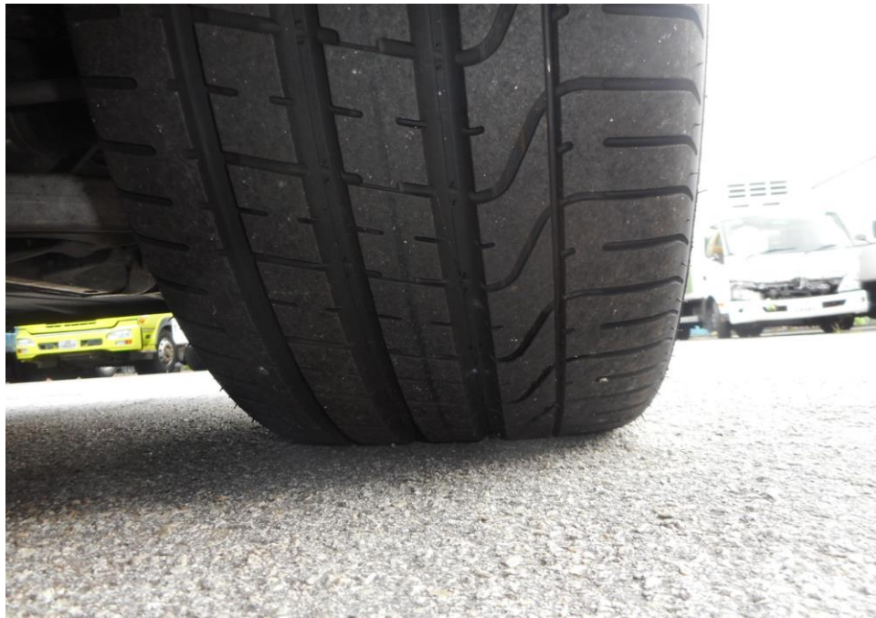
Photo 7 shows the condition of the front right tyre of the Motor Car, which was observed to be in serviceable condition with remaining tread depth of approximately 6.7mm. The tyre, which was wrapped around standard alloy wheel rim, was also observed to be sufficiently inflated for vehicular operation. There was no tear, cut or burst mark(s) on the outer and the inner sidewalls as well as across the tread of the 4 tyres that were fitted on the Motor Car.
