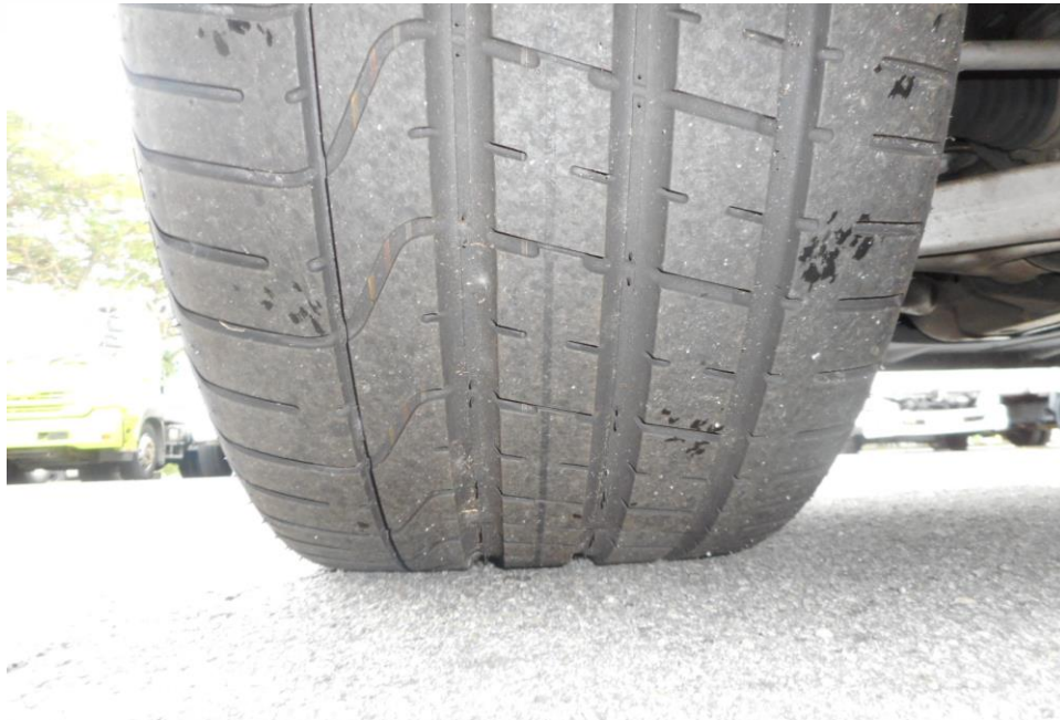
Photo 10 shows the condition of the rear right tyres of the Motor Car, which were observed to be in serviceable condition with remaining, tread depth of approximately 6.5mm. There was also no tear, cut or burst mark(s) on the outer and the inner sidewalls as well as across the tread of the 4 tyres that were fitted on the Motor Car.
