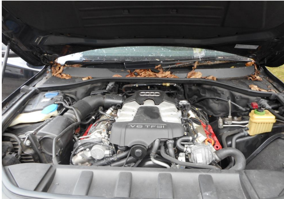
Photo 11 shows a general view of the Motor Car's engine compartment, which was accessed by lifting the front cabin of the Motor Car. The various parts and components inside the engine compartment were unaffected by the accident. There was also no sign(s) or indication(s) of fresh fluid leakage and/or fluid stain within the engine compartment
