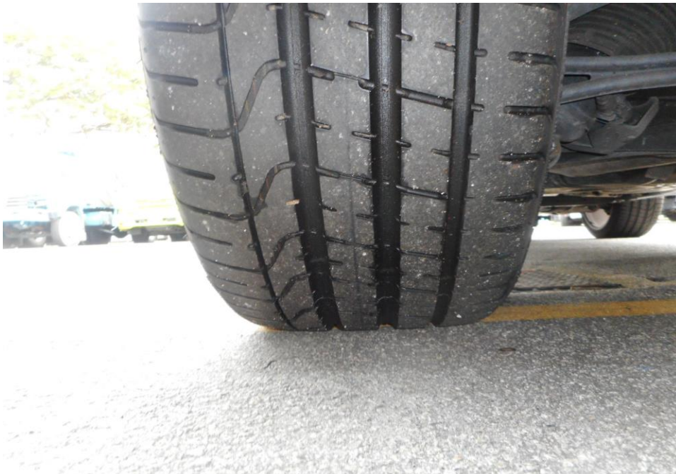
Photo 9 shows the condition of the rear left tyres of the Motor Car, which was observed to be in serviceable condition with remaining tread depth of approximately 6.7mm. The tyres, which were wrapped around standard alloy wheel rim, were also observed to be sufficiently inflated for vehicular operation. There was also no damage found on all 4 alloy wheel rims of the Motor Car.
