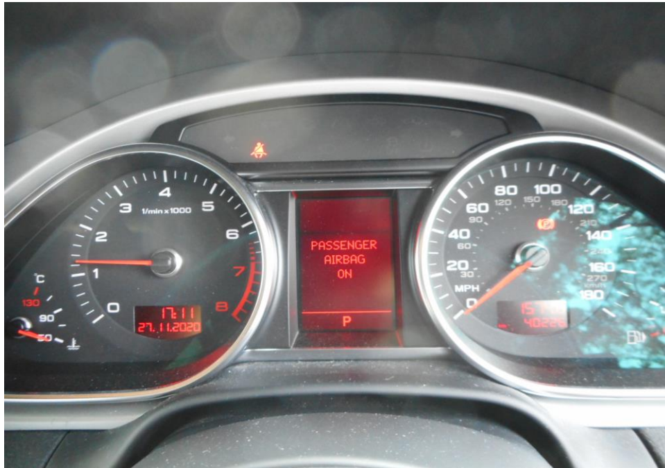
Photo 25 shows no warning lights illuminated on the instrument panel of the Motor Car after the engine was cranked. This would suggest that there was no abnormality to the various electronic operating systems of the Motor Car, like the ABS, SRS and TC.
