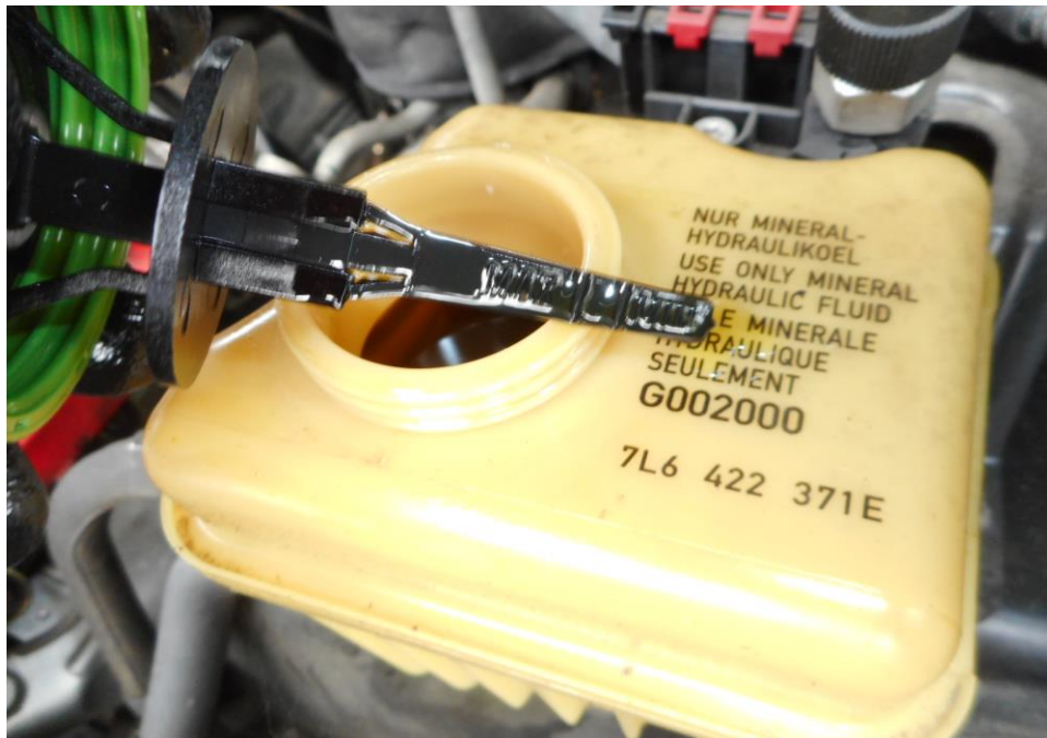
Photo 15 shows the power steering oil dip stick of the Motor Car at the time of my inspection. The power steering oil was observed to be of sufficient level and without any visible contamination.
