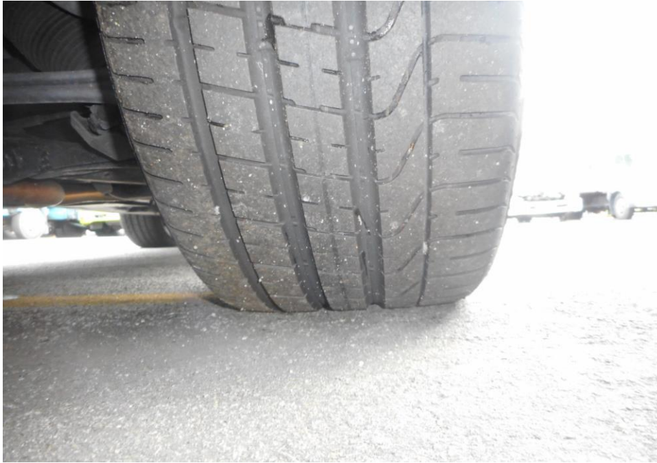
Photo 8 shows the condition of the rear right tyre of the Motor Car, which was observed to be in serviceable condition with remaining tread depth of approximately 6.5mm. The tyre, which was wrapped around standard alloy wheel rim, was also observed to be sufficiently inflated for vehicular operation.
