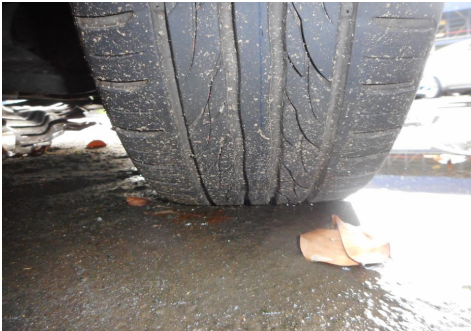
Photo 7 shows the condition of the front right tyre of the Motor Car, which was observed to be in serviceable condition with remaining tread depth of approximately 5.7mm. The tyre was sufficiently inflated for vehicular operation with no tear, cut or burst mark(s) on the outer and the inner sidewalls as well as across the tread. The 4 tyres of the Motor Car were wrapped around standard steel wheel rims without any damage.
