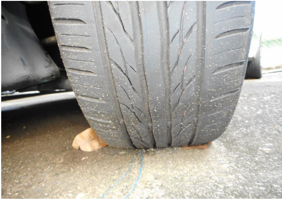
Photo 10 shows the condition of the front left tyre of the Motor Car, which was observed to be in serviceable condition with remaining tread depth of approximately 5.4mm. There was also no tear, cut or burst mark(s) on the outer and the inner sidewalls as well as across the tread of the Motor Car's 4 tyres.
