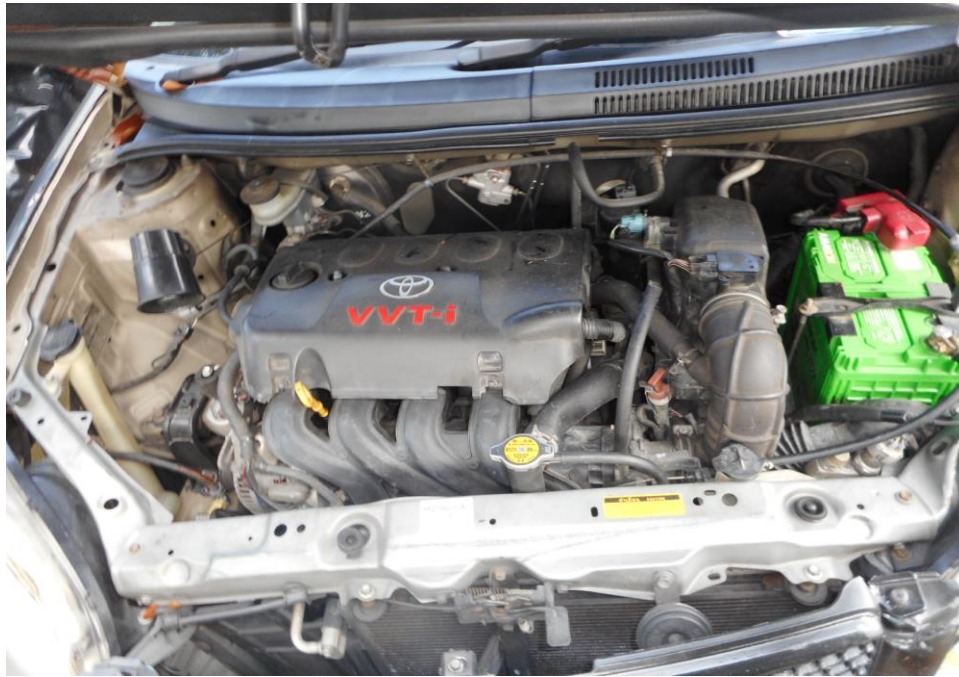
Photo 11 shows a general view of the Motor Car's engine compartment. The front panel of the engine compartment was observed to be damaged as a result of the accident. However, the various parts and components inside the engine compartment were unaffected by the accident. There was also no sign(s) or indication(s) of fluid leakage and/or fluid stain within the engine compartment.
