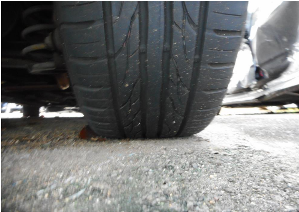
Photo 8 shows the condition of the rear right tyre of the Motor Car, which was observed to be in serviceable condition with remaining tread depth of approximately 6.2mm. The tyre was also observed to be sufficiently inflated for vehicular operation with no tear, cut or burst mark(s).
