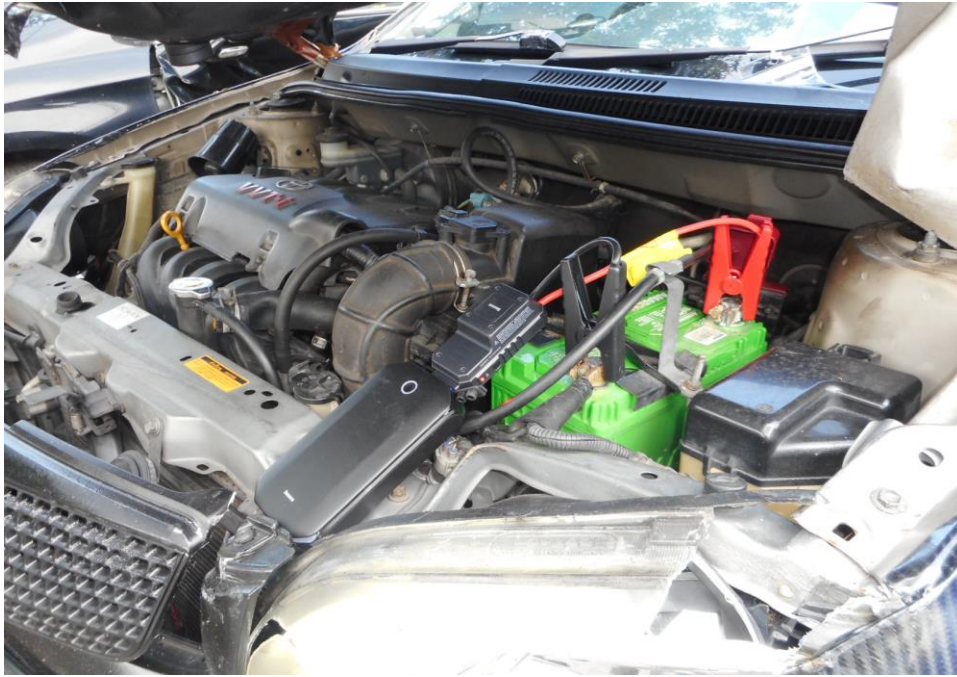
Photo 17 shows the engine of the Motor Car, the engine was not able to be started up despite multiple attempts on jumpstarting it.
