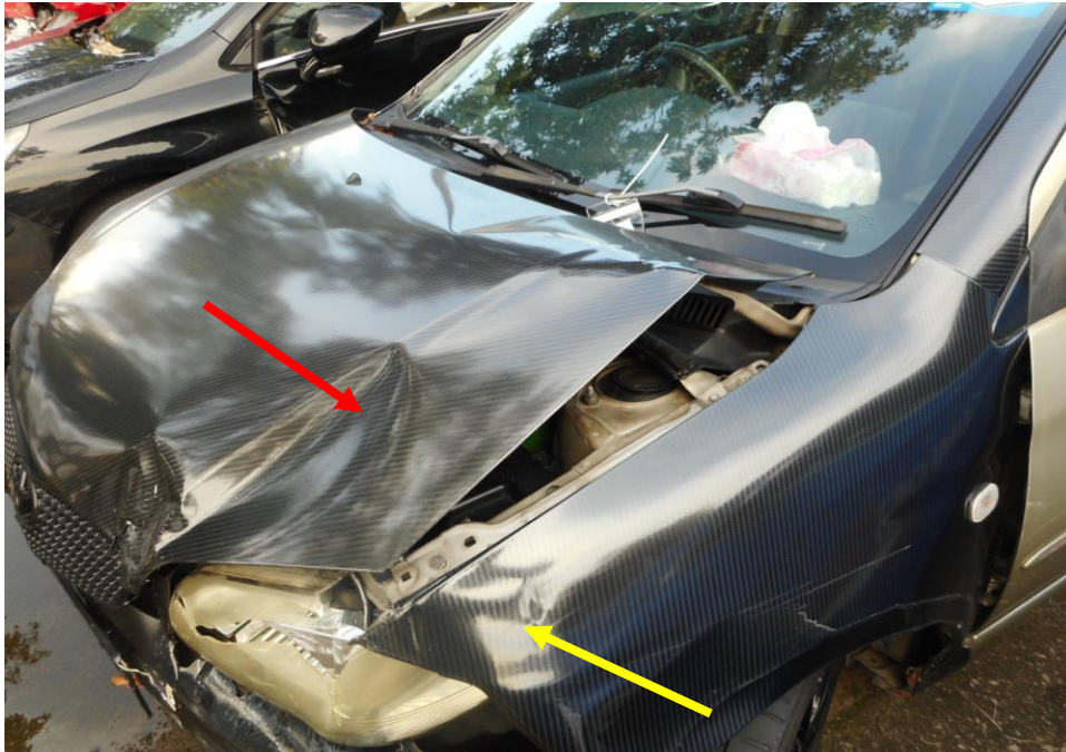
Photo 4 shows the close up view of the Motor Car's front portion at the time of my inspection. Its front bonnet (red arrow) and front left fender (yellow arrow) were amongst the body parts that were damaged as a result of the accident.
