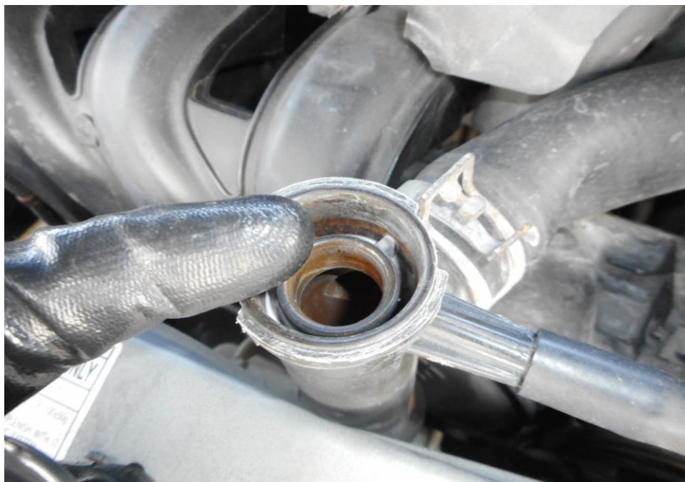
Photo 14 shows checks being carried out to the engine coolant of the Motor Car at the time of my inspection. The engine coolant was observed to be of insufficient level.
