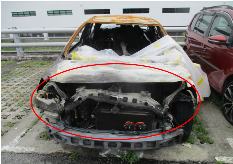
Photo 4 shows the front portion of the Insured Vehicle. Impact damage was observed at its front side (circled). Its front wheels, front support panel, front bumper and front bumper reinforcement were amongst the body parts that were bent/ buckled as a result of the impact force.
