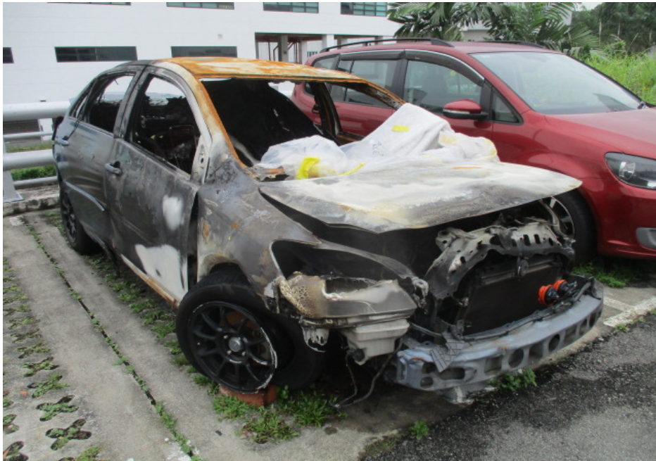
Photo 1 shows the general view of the right body of the Insured Vehicle at the time of our inspection. The Insured Vehicle was observed to have sustained extensive fire damage all around. Its engine compartment and interior compartment were completely burnt. Rust had accumulated all over the Insured Vehicle as a result of exposure to environmental condition for a period of time.
