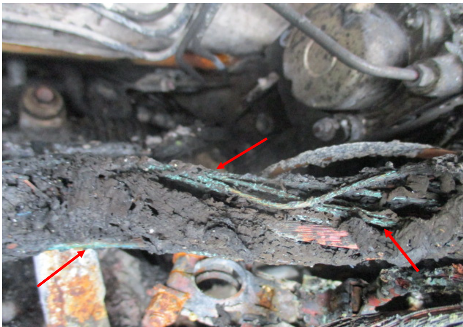
Photo 8 shows a close up view of some of the wirings with greenish residue (arrowed). The presence of such greenish residue suggest occurrence of an electrical short circuit.
