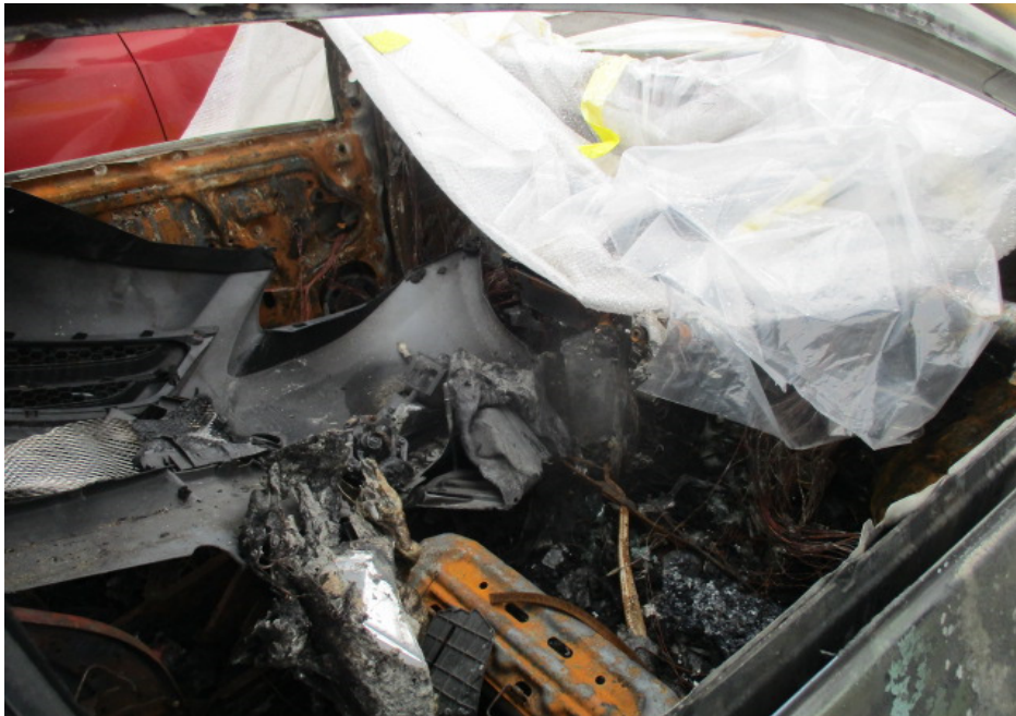
Photo 3 shows the interior compartment of the Insured Vehicle, which was significantly affected by the fire.
