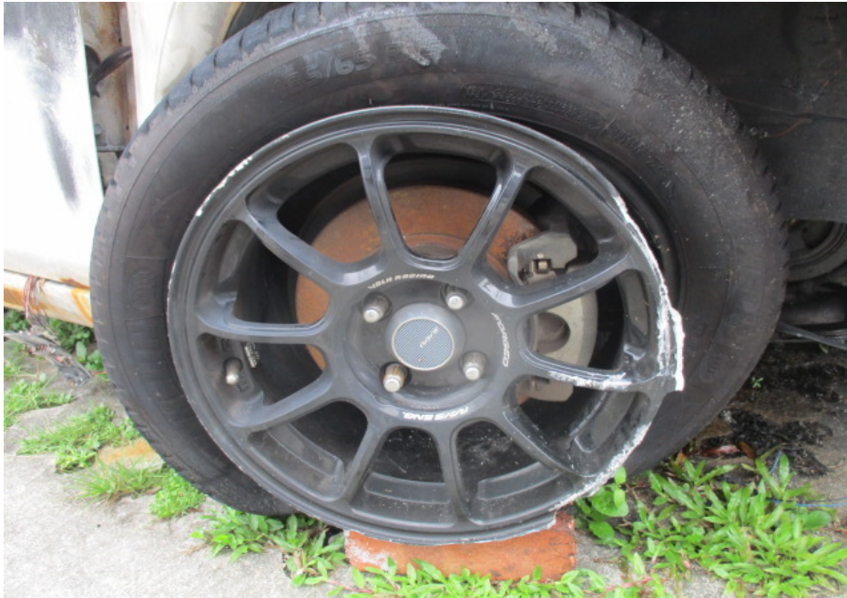
Photo 5 shows the non-standard rim found to be fitted on the Insured Vehicle at the time of our inspection. The 15- inch alloy rims fitted on the Insured Vehicle were not the standard type for the Insured Vehicle.
