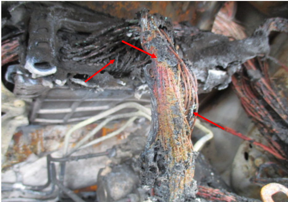
Photo 7 shows a closer view of some of the wirings with greenish residue (red arrows). The presence of such greenish residue suggest occurrence of an electrical short circuit.
