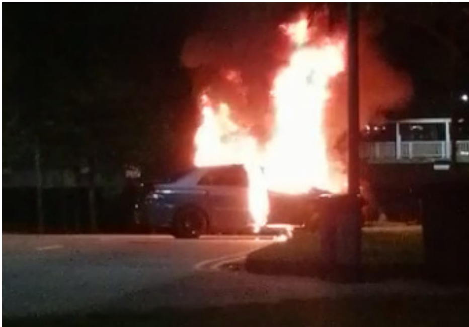
Photo 9 shows the Insured Vehicle on fire after colliding into a centre divider and mounting a kerb, before the arrival of the SCDF. In general, the information that could be gathered from this photograph had corresponded to the events that were related to us by Ms Shalene, which is the fire started from the front bonnet almost immediately after the collision.
