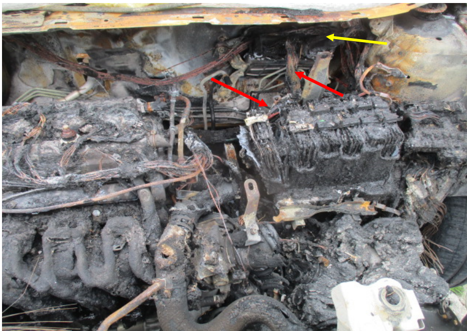
Photo 6 shows the wirings around the rear left portion of the engine compartment. Several stretches of wirings leading towards the Engine Control Module (ECM) (yellow arrow) were found burnt internally to its bare copper state (red arrows). The bright reddish colour of the copper wires suggests that the wirings were exposed to high heat. Such condition normally indicates internal heating of copper wires which is a sign of an electrical short circuit occurring.
