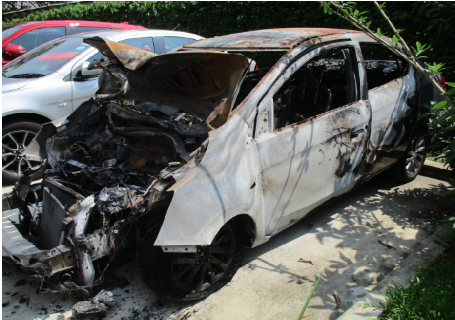
Photo 2 shows the general view of the left body of the Insured Vehicle at the time of our inspection. The Insured Vehicle was observed to have sustained extensive fire damage all around. Rust had accumulated all over the Insured Vehicle as a result of exposure to environmental condition for a period of time.
