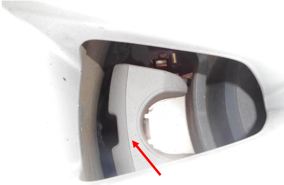
Photo 19 shows the brake caplier (arrowed) at the rear left wheel of the Motor Car. No leakage of brake fluid was observed on the surface. Visual examination of the various components of the braking system like the drum brake, brake booster, brake pedal etc. had revealed all to be intact and without visible damage.
