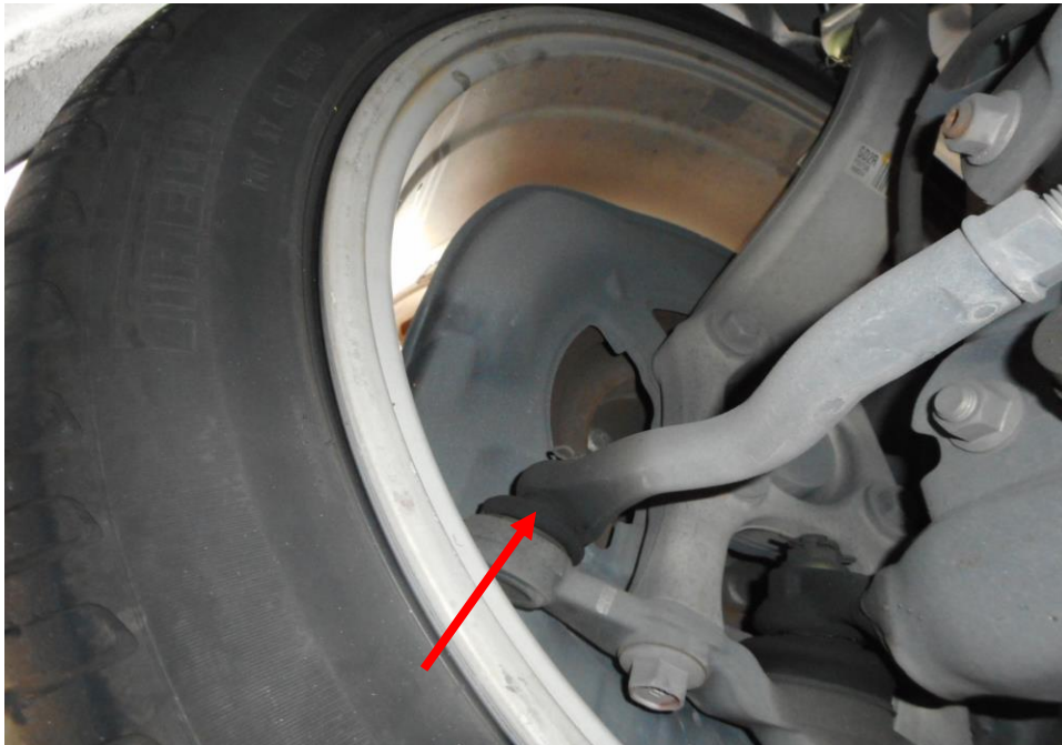
Photo 22 shows the various undercarriage components at the front right wheel of the Motor Car, in particular the steering tie rod, tie rod end and ball joints (arrowed) was observed to be intact and not damaged by the accident. However, old stain was observed on the surface of the tie rod end and ball joint.
