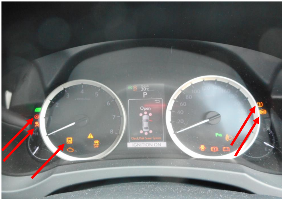
Photo 25 shows the warning light for Anti-Lock Brake System (ABS) and Power Steering System (EPS), Supplemental Restraint System (SRS), Traction Control (TC) and Tyre Pressure Monitoring System (TPMS) (arrowed) appearing on the instrument panel of the Motor Car during the self-test of its various electronic operating systems when its engine was cranked.
