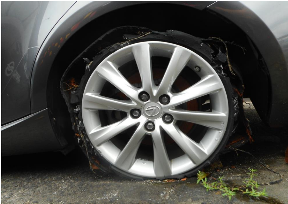
Photo 9 shows the condition of the rear left tyre of the Motor Car, which was observed to be in unserviceable condition. The tyre and alloy wheel rim was observed to be damaged as a result of the accident.
