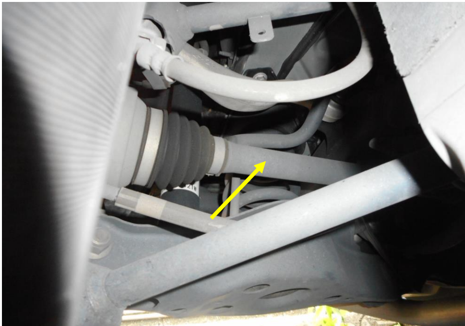
Photo 24 shows the various undercarriage components at the rear left wheel of the Motor Car, in particular the drive shaft (yellow arrow). The various undercarriage components of the Motor Car were all found to be intact without any visible damage. There was also no sign of fluid stain(s) observed on the various undercarriage components.
