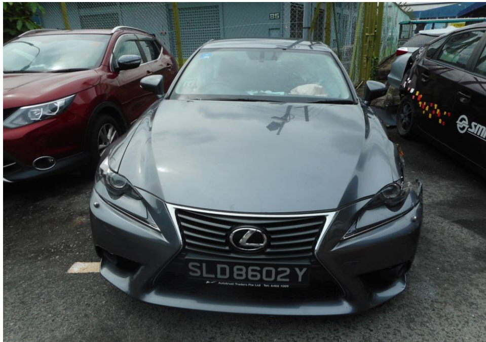
Photo 2 shows a general view of the Motor Car's front body at the time of my inspection. The Motor car was observed to have sustained damage at its front and left portion. Its front windscreen, front bumper, front left fender and front left headlamp were amongst the body parts that were damaged as a result of the accident.
