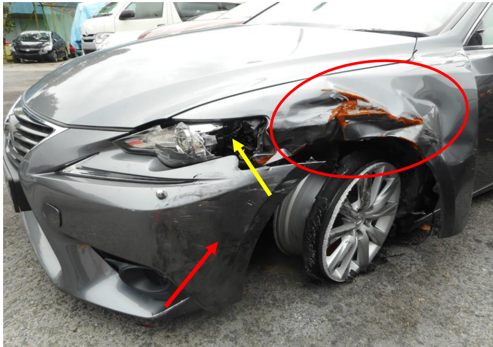
Photo 4 shows a close up view of the Motor Car's front portion at the time of my inspection. The Motor car was observed to have sustained damage at its front portion. Its front bumper (red arrow), front left headlamp (yellow arrow) and front left fender (circled) were amongst the body parts that were damaged as a result of the accident.
