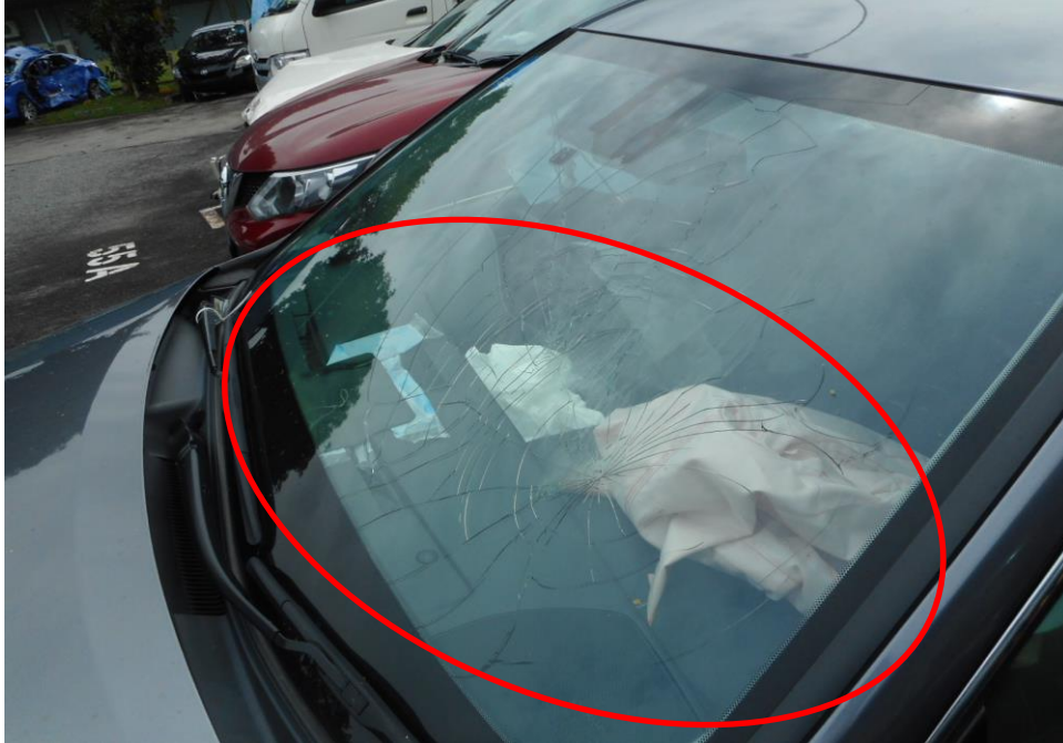
Photo 3 shows the close up view of the Motor Car's front body at the time of my inspection. The Motor car was observed to have sustained damage at its front portion. Its front windscreen (circled) were amongst the body parts that were damaged as a result of the accident.
