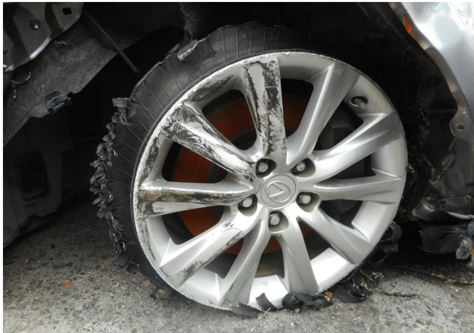
Photo 8 shows the condition of the front left tyre of the Motor Car, which was observed to be in unserviceable condition. The tyre and alloy wheel rim was observed to be damaged as a result of the accident.
