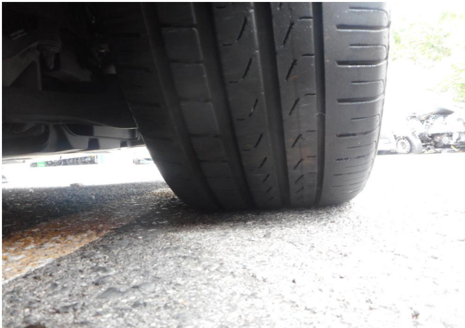
Photo 10 shows the condition of the front right tyre of the Motor Car, which was observed to be in serviceable condition with remaining tread depth of approximately 4.4mm. The tyre was also observed to be sufficiently inflated for vehicular operation with no tear, cut or burst mark(s).
