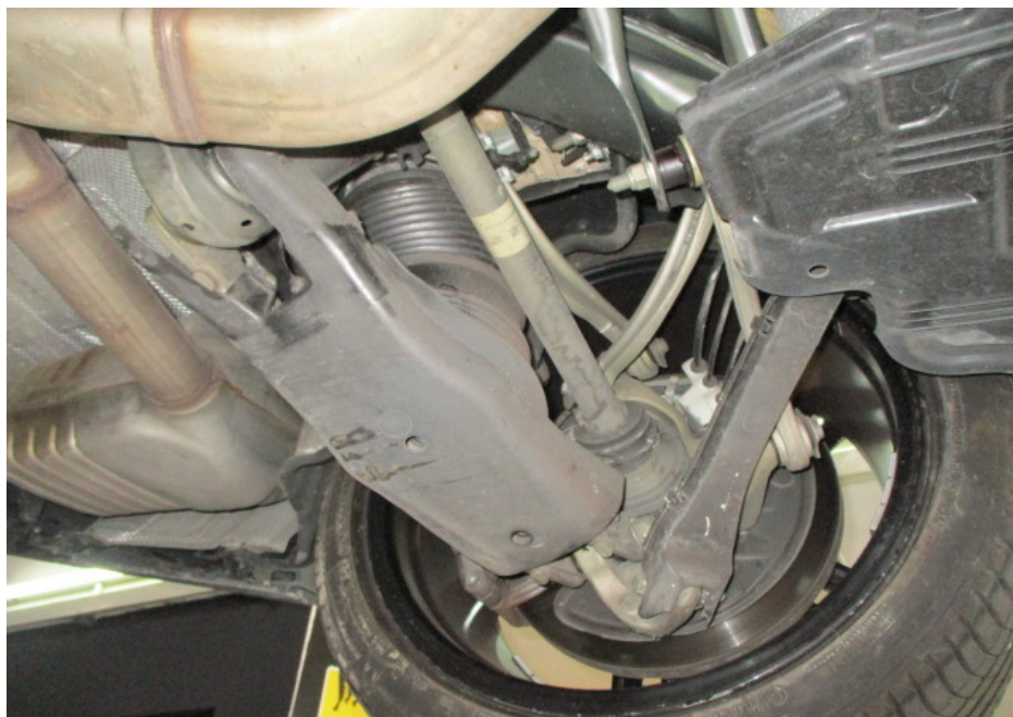
Photo 15 shows a general view of the control arms and linkages at the rear left wheel of the Motor Car. I did not observe any fluid leak and/or fluid stain on the underside of the Motor Car. All the Motor Car's undercarriage components were observed to be intact and secured in an appropriate manner.
