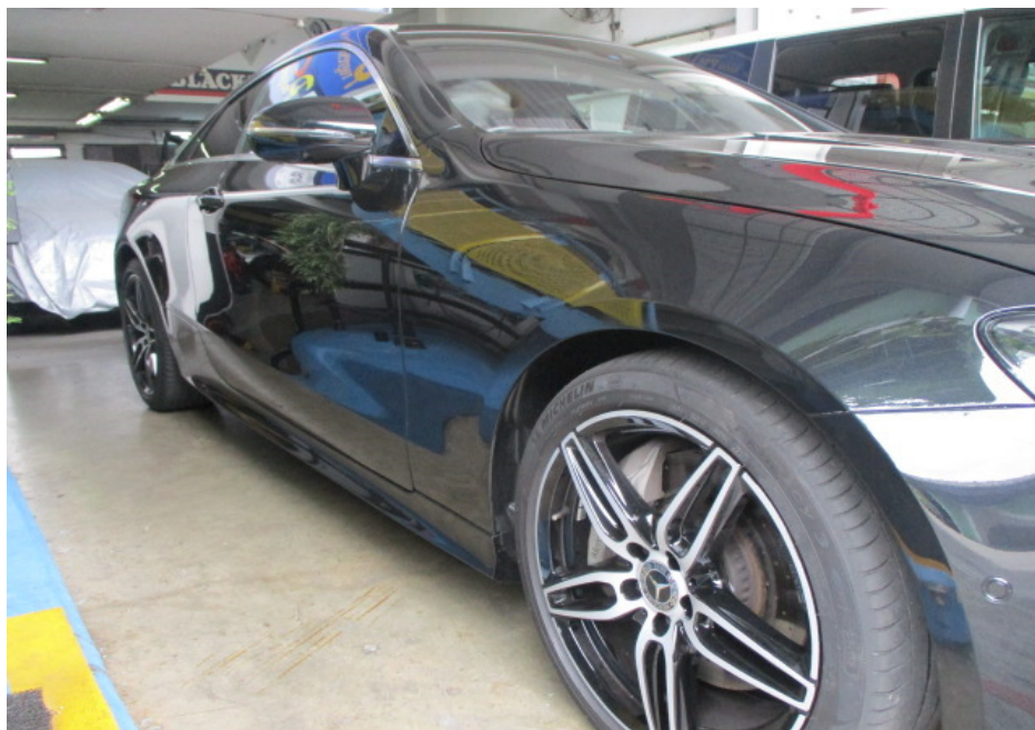
Photo 6 shows a closer view of the Motor Car's front right fender and front right wheel rim. The body parts at the front right portion of the Motor Car were visually examined and it was observed that the repair/restoration works carried out to the damaged area of the Motor Car (refer to photograph 1 & 2 above) were reasonably adequate and in order.
