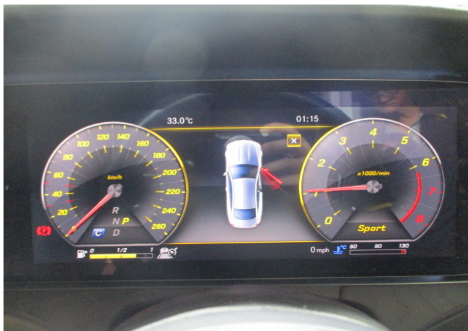
Photo 13 shows the respective warning lights no longer illuminated, indicating that there is no fault detected to the ABS, SRS, EPS and ESP systems of the Motor Car during the self-test. These electronic systems were hence in working condition at the time of my inspection.
