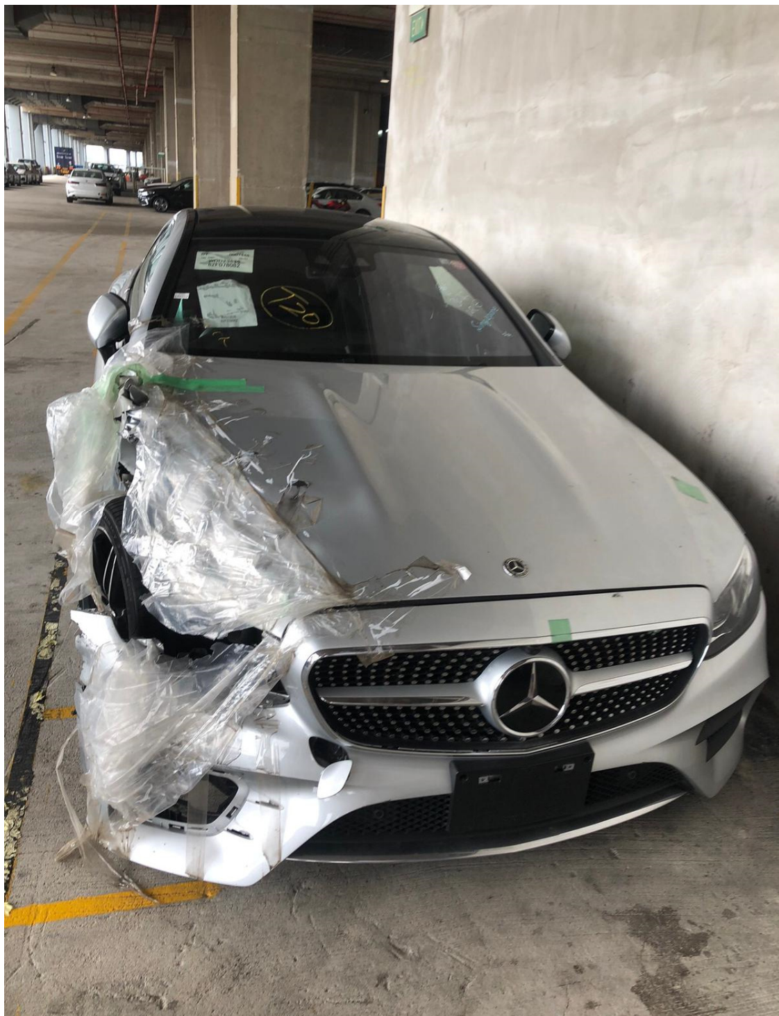
Photo 1 shows the front right body of the Motor Car prior to any repairs being carried out (photograph provided to me). The Motor Car was observed to have sustained damages at its front right portion. The body parts observed to be damaged had include its front bumper, front bumper lower right grille, front right headlamp, front bonnet and front right fender amongst others.
