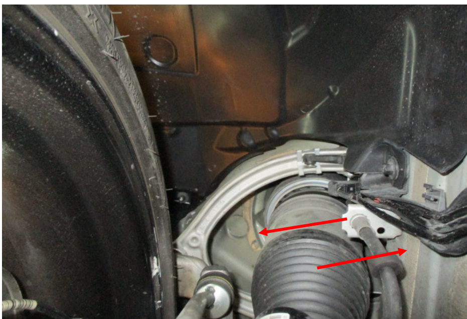
Photo 21 shows the front right wheelhouse panel of the Motor Car. The original factory sealant (arrowed) at the joints along the non-detachable body panels were untouched, indicating no work was done on the non-detachable body panels of the Motor Car. In general, I had found the non-detachable body panels of the Motor Car to be originally fitted at the time of my inspection.
