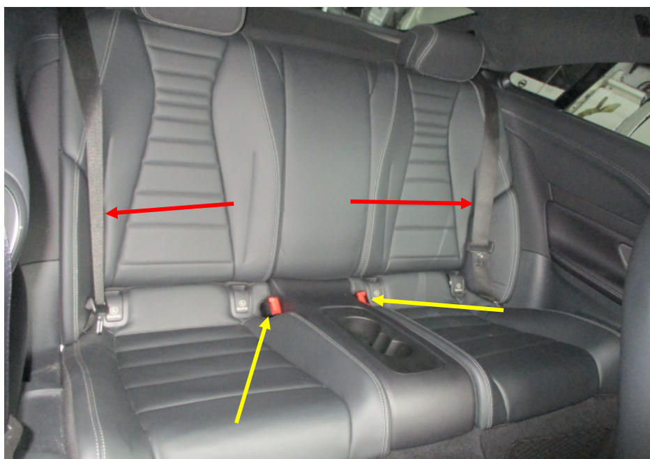
Photo 11 shows the rear seats of the Motor Car. All the seats of the Motor Car were secured via seat rails to the floorboard. They were each fitted with a retractable seat belt reel (red arrow) and a pre-tensioner (yellow arrow). The seat belt reels were tested and able to be fastened into the respective pre-tensioners that were fitted on the side of each individual seat.
