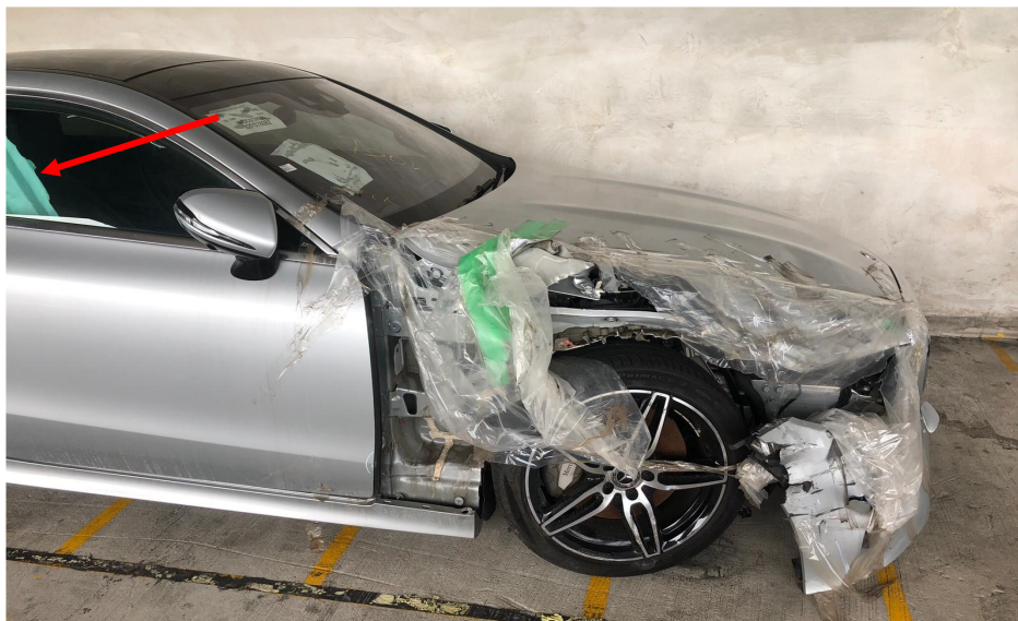
Photo 2 shows the right front portion of the Motor Car prior to any repairs being carried out (photograph provided to me). The front right fender, front right fender inner panel, front right door and right side rocker panel garnish were observed to be damaged. The right side curtain airbag (arrowed) was also observed to be activated.
