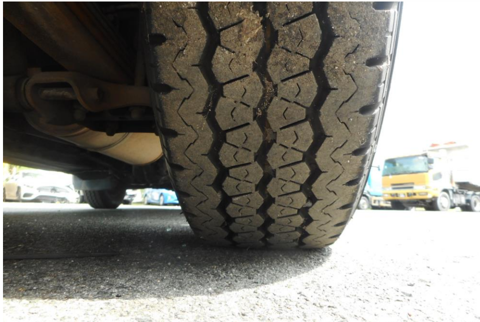
Photo 8 shows the condition of the rear right tyre of the Motor Van, which was observed to be in serviceable condition with remaining tread depth of approximately 5.7mm. The tyre, which was wrapped around standard steel wheel rim, it was observed to be sufficiently inflated for vehicular operation.
