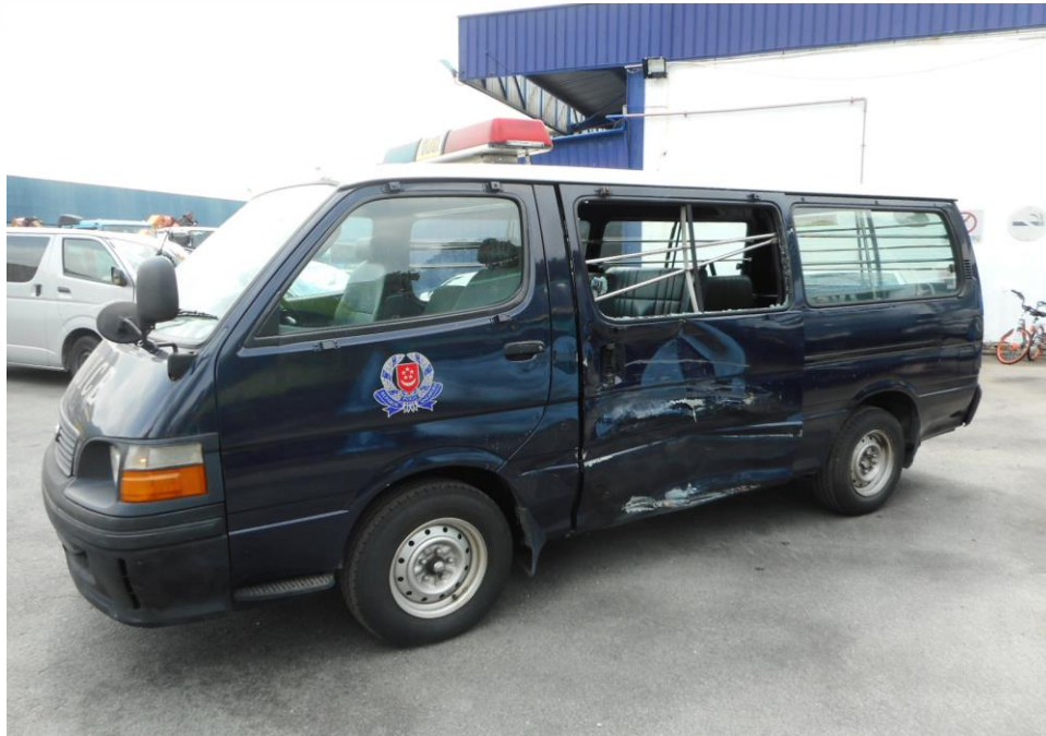
Photo 2 shows a general view of the left body of the Motor Van left portion at the time of my inspection. It appeared to have sustained damage at its left portion. Its left body panel were damaged as a result of the accident.
