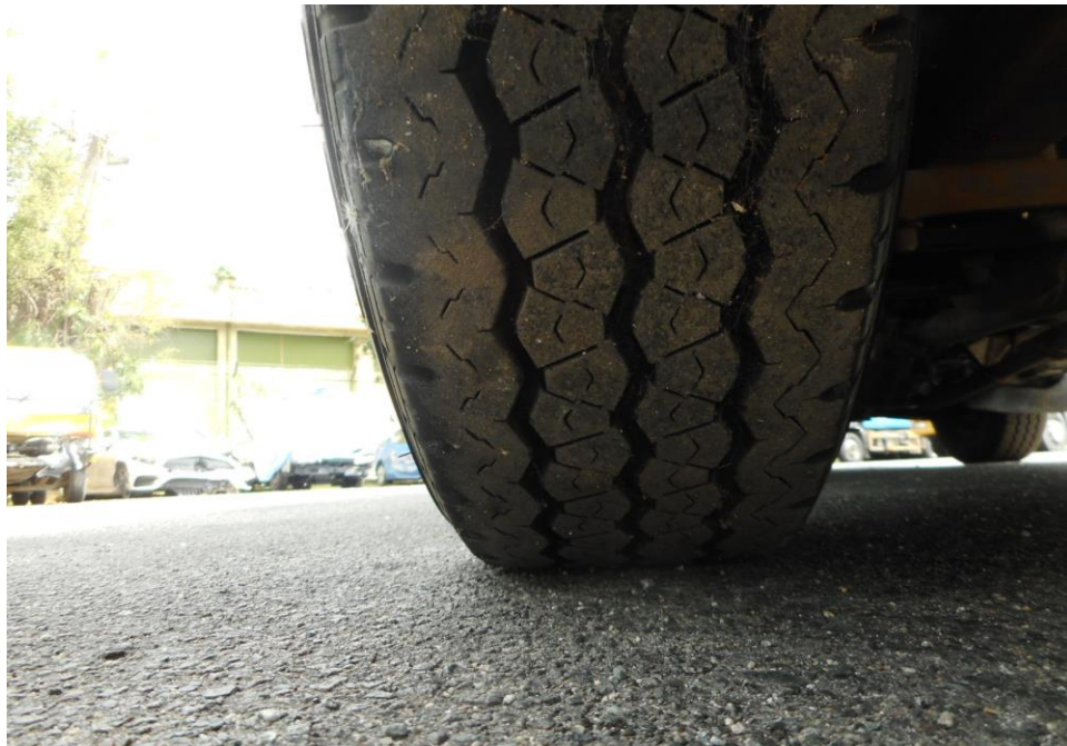
Photo 9 shows the condition of the rear left tyres of the Motor Van, which was observed to be in serviceable condition with remaining tread depth of approximately 6.2mm. The tyres, which were wrapped around standard steel wheel rim, were also observed to be sufficiently inflated for vehicular operation. There was also no damage found on all 4 steel wheel rims of the Motor Van.
