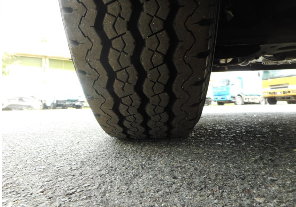
Photo 10 shows the condition of the rear right tyres of the Motor Van, which were observed to be in serviceable condition with remaining, tread depth of approximately 7.1mm. There was also no tear, cut or burst mark(s) on the outer and the inner sidewalls as well as across the tread of the 4 tyres that were fitted on the Motor Van.
