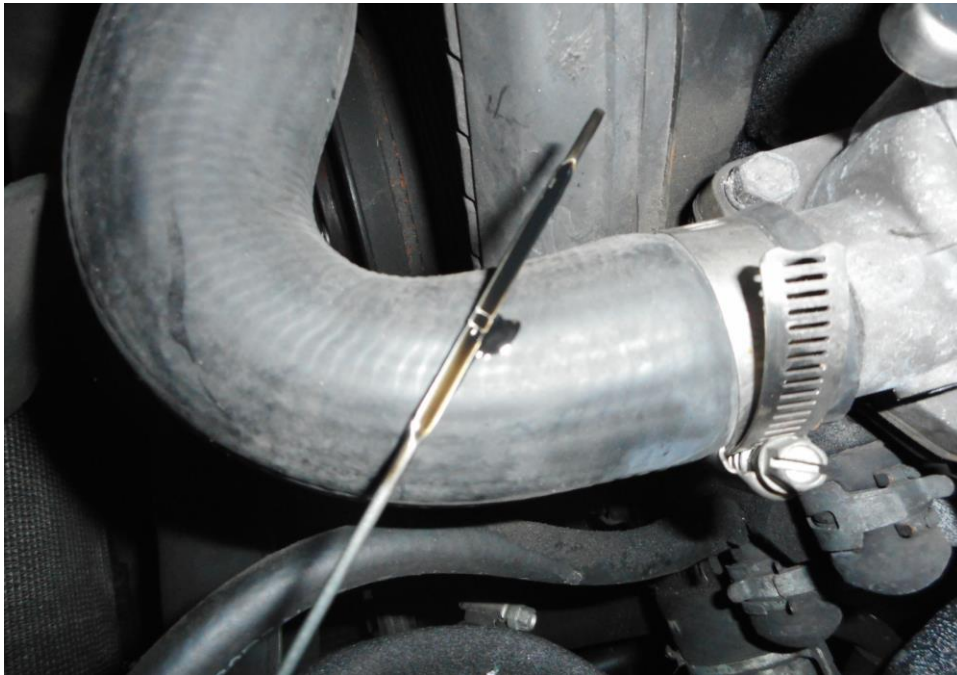
Photo 14 shows the engine oil dip stick of the Motor Van at the time of my inspection. The engine oil was observed to be of sufficient level and without any visible contamination.
