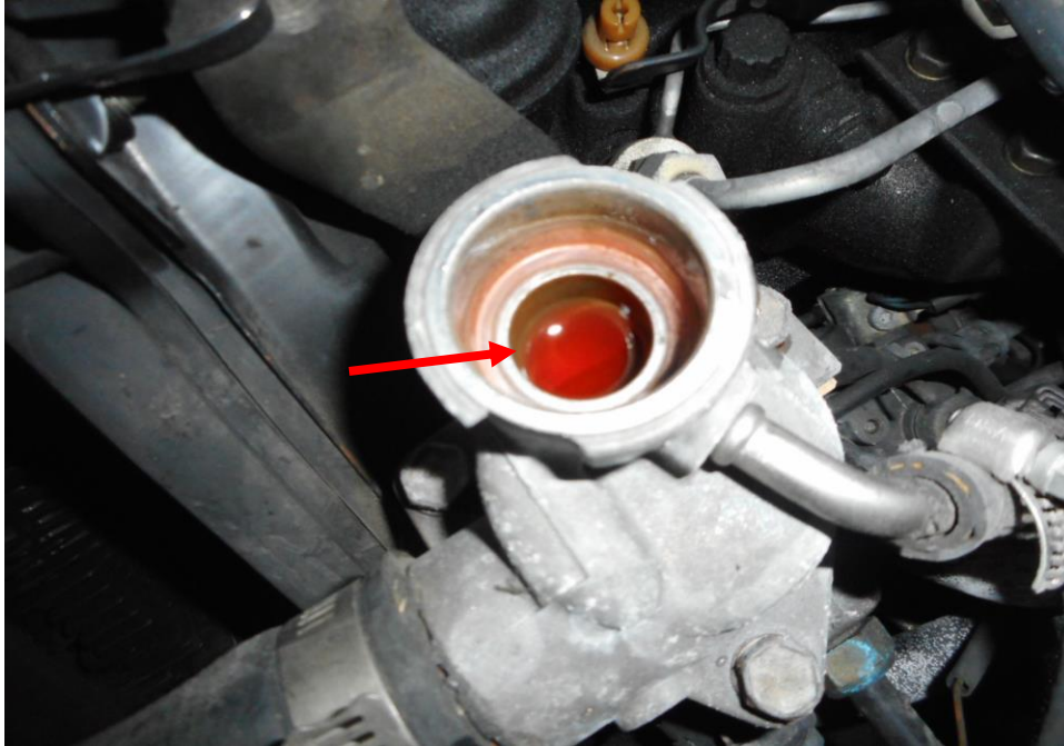
Photo 13 shows the engine coolant reservoir of the Motor Van at the time of my inspection. The engine coolant was observed to be of insufficient level (arrowed).
