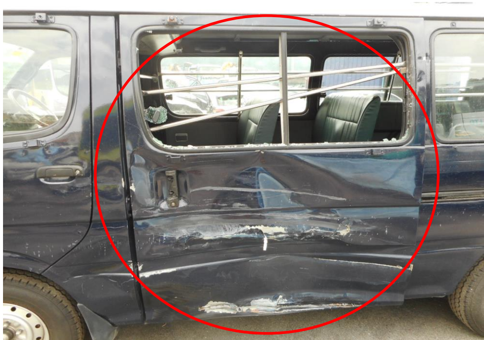
Photo 3 shows a close up view of the left body of the Motor Van left portion at the time of my inspection. It appeared to have sustained damage at its left portion. Its left body panel (circled) were damaged as a result of the accident.
