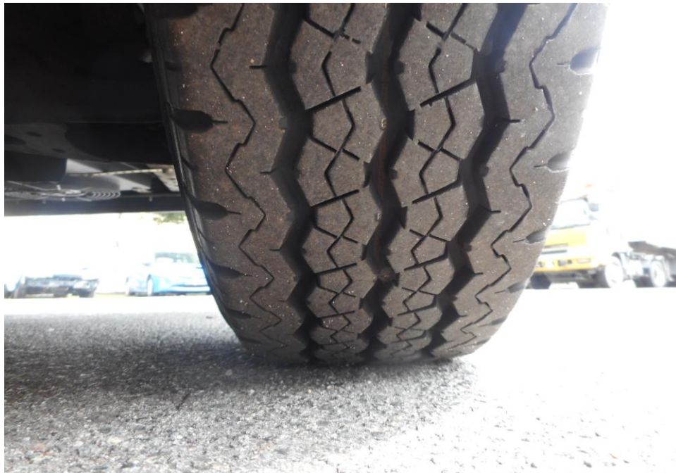
Photo 7 shows the condition of the front right tyre of the Motor Van, which was observed to be in serviceable condition with remaining tread depth of approximately 7.8mm. The tyre, which was wrapped around standard steel wheel rim, was also observed to be sufficiently inflated for vehicular operation. There was no tear, cut or burst mark(s) on the outer and the inner sidewalls as well as across the tread of the 4 tyres that were fitted on the Motor Van.
