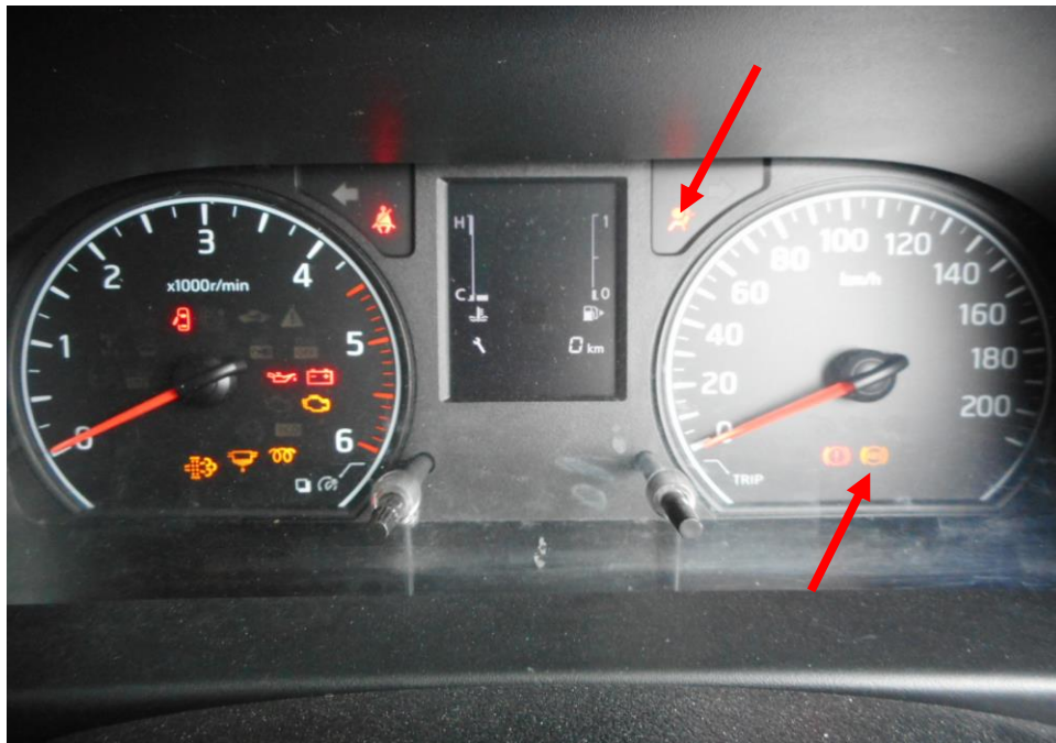
Photo 22 shows the warning light for Anti-Lock Brake System (ABS) and Supplemental Restraint System (SRS) (arrowed) appearing on the instrument panel of the Motor Van during the self-test of its various electronic operating systems when its engine was cranked.
