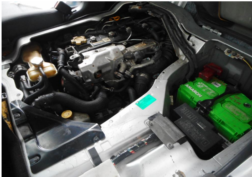
Photo 10 shows a general view of the Motor Van's engine compartment, which was accessed by lifting the front cabin of the Motor Van. The various parts and components inside the engine compartment were unaffected by the accident. There was also no sign(s) or indication(s) of fresh fluid leakage and/or fluid stain within the engine compartment
