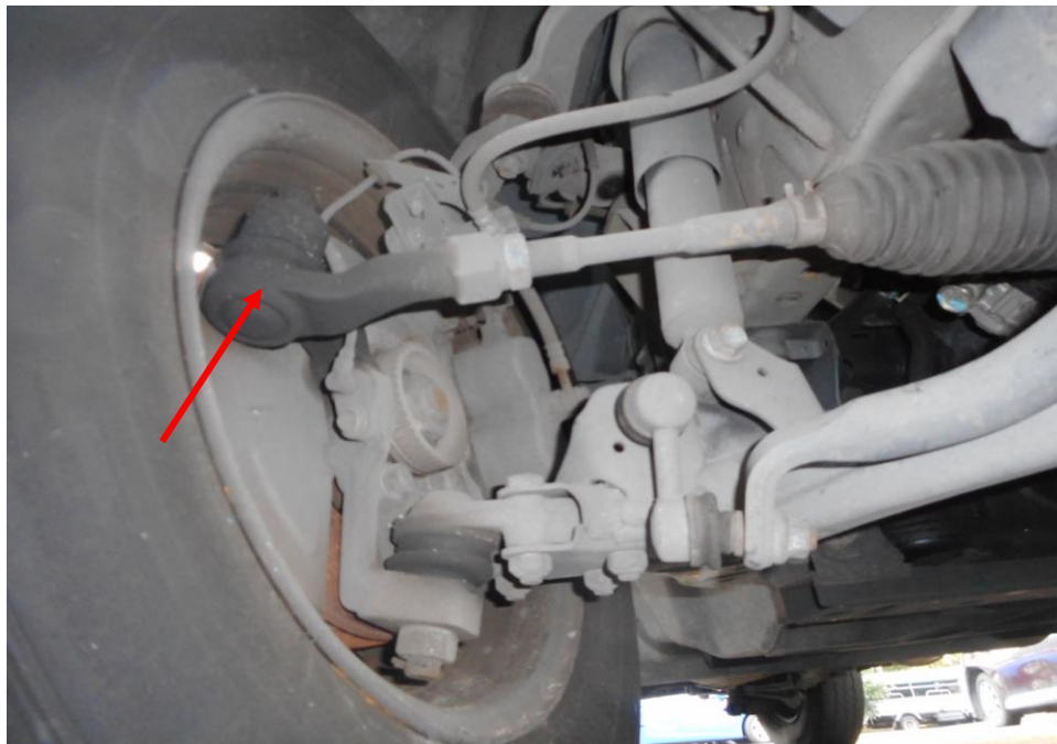
Photo 15 shows the various undercarriage components at the front right wheel of the Motor Van, in particular the steering tie rod end (arrowed). The various steering components were all found to be intact, suggesting that the steering system of the Motor Van was likely to be in serviceable condition at the material time of accident. There was also no sign of fluid stain(s) observed on the various undercarriage components.
