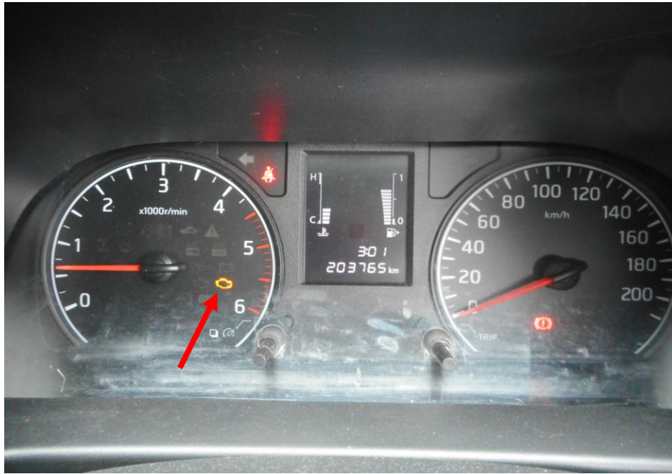
Photo 23 shows no warning lights illuminated on the instrument panel of the Motor Van after the engine was cranked. This would suggest that there was no abnormality to the electronic operating system of the Motor Van, like the ABS and SRS etc. However, only the engine warning light remained illuminated as this is a likely a result of the insufficient engine coolant (arrowed).
