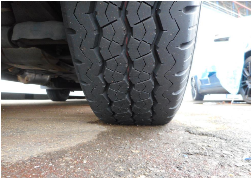
Photo 7 shows the condition of the rear right tyre of the Motor Van, which was observed to be in serviceable condition with remaining tread depth of approximately 7.4mm. The tyre, which was wrapped around standard steel wheel rim, it was observed to be sufficiently inflated for vehicular operation.
