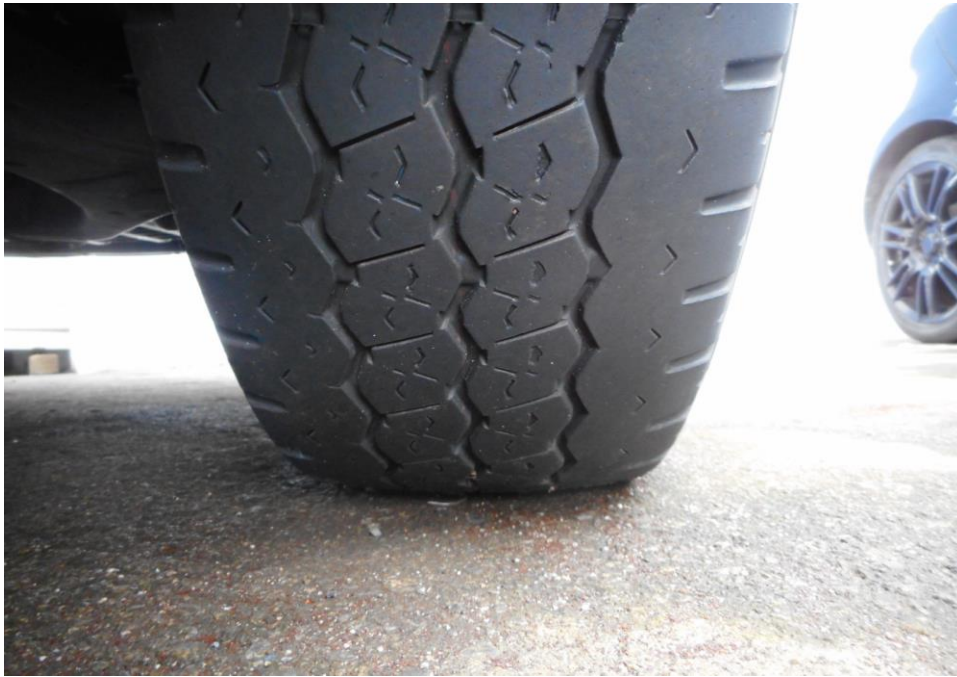
Photo 6 shows the condition of the front right tyre of the Motor Van, which was observed to be in serviceable condition with remaining tread depth of approximately 3.8mm. The tyre, which was wrapped around standard steel wheel rim, was also observed to be sufficiently inflated for vehicular operation. There was no tear, cut or burst mark(s) on the outer and the inner sidewalls as well as across the tread of the 4 tyres that were fitted on the Motor Van.
