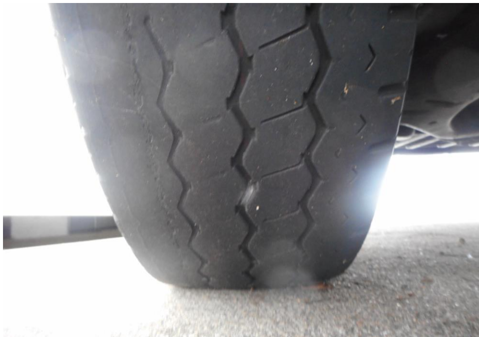
Photo 9 shows the condition of the rear right tyres of the Motor Van, which were observed to be in serviceable condition with remaining, tread depth of approximately 2mm. There was also no tear, cut or burst mark(s) on the outer and the inner sidewalls as well as across the tread of the 4 tyres that were fitted on the Motor Van.
