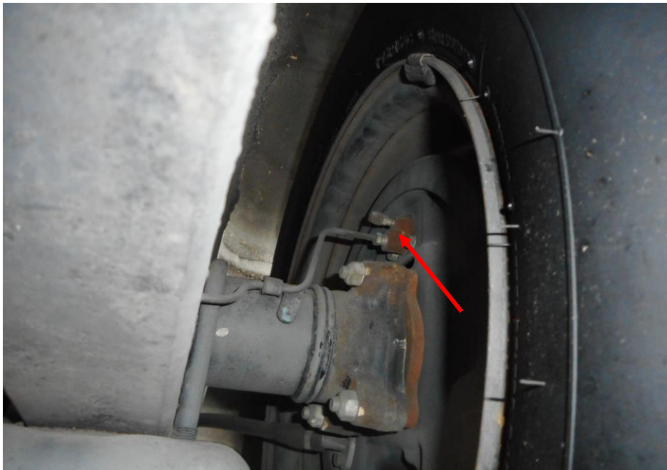
Photo 17 shows the brake pipe (arrowed) at the rear right wheel of the Motor Van. I did not observe any leakage of brake fluid at the time of my inspection of the Motor Van. My static tests of the Motor Van's braking system, along with my visual examination of the various mechanical components in the braking system, had indicated that there was no internal leakage of pressure/vacuum. Hence the braking system of the Motor Van was likely to be in serviceable condition at the material time of accident.
