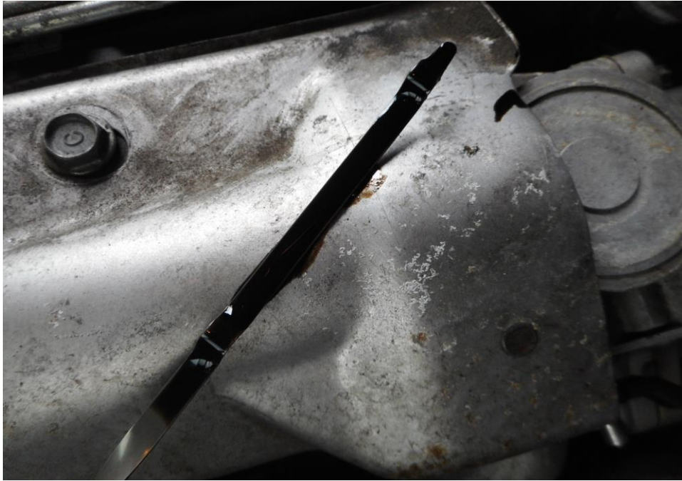
Photo 13 shows the engine oil dip stick of the Motor Van at the time of my inspection. The engine oil was observed to be of sufficient level and without any visible contamination.
