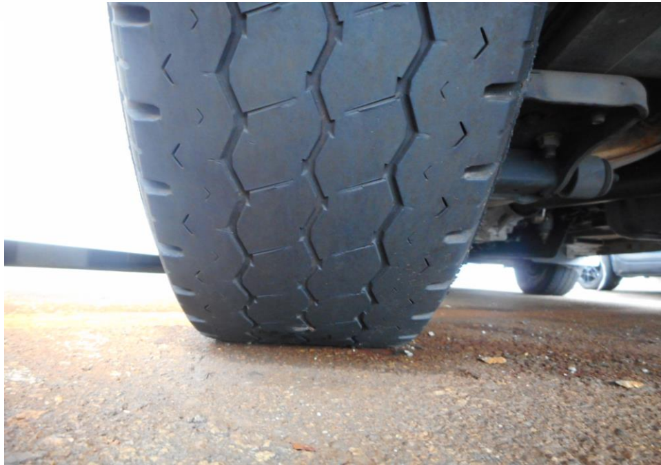
Photo 8 shows the condition of the rear left tyres of the Motor Van, which was observed to be in serviceable condition with remaining tread depth of approximately 1.8mm. The tyres, which were wrapped around standard steel wheel rim, were also observed to be sufficiently inflated for vehicular operation. There was also no damage found on all 4 steel wheel rims of the Motor Van.
