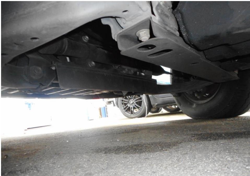
Photo 14 shows the undercarriage of the Motor Van, at the area where the engine housing and transmission housing are located. . I did not find any sign(s) or indication(s) of fluid leak and/or fluid stain(s) on the underside of the Motor Van.
