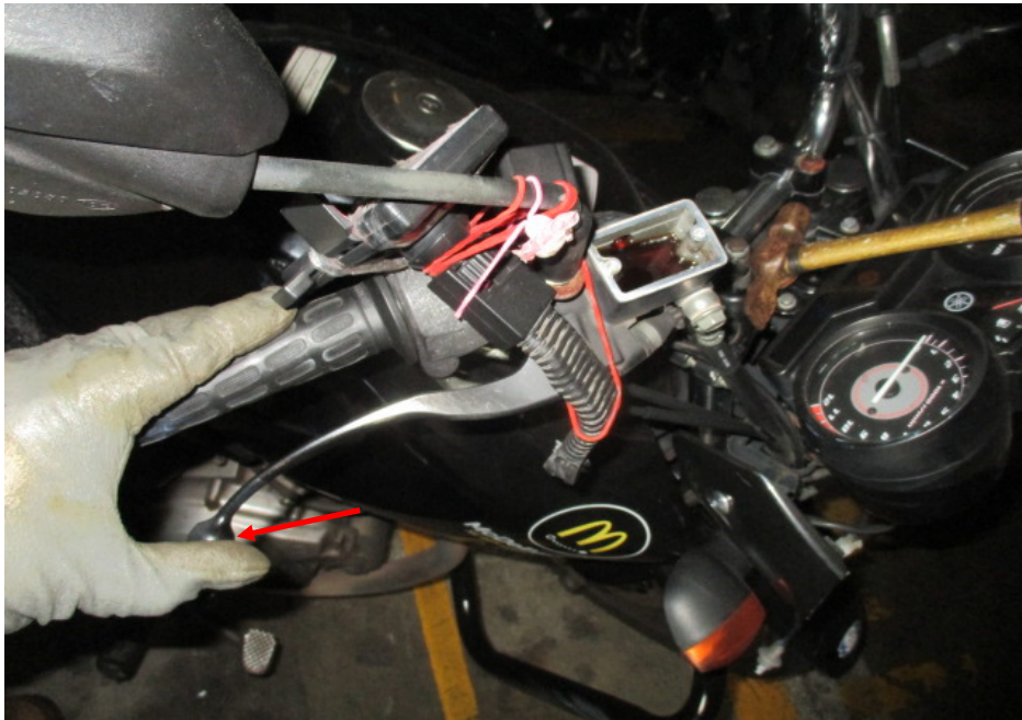
Photo 22 shows the front brake lever being depressed. There was some resistance felt (spongy like feel) upon pressing the front brake lever (arrowed). This would indicate that there is no leakage of pressure/vacuum in the brake system.
