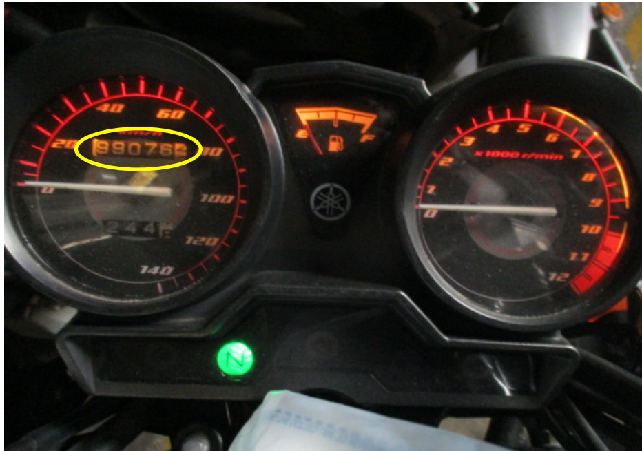
Photo 1 shows the speedometer gauge of the Motorcycle where the mileage recorded at the time of our inspection was 99, 076km (circled).
