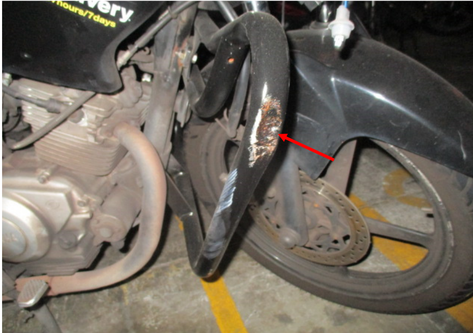
Photo 7 shows a closer view of the deformed right crash bar which was amongst the body parts of the Motorcycle that had sustained damages as a result of the accident (arrowed).
