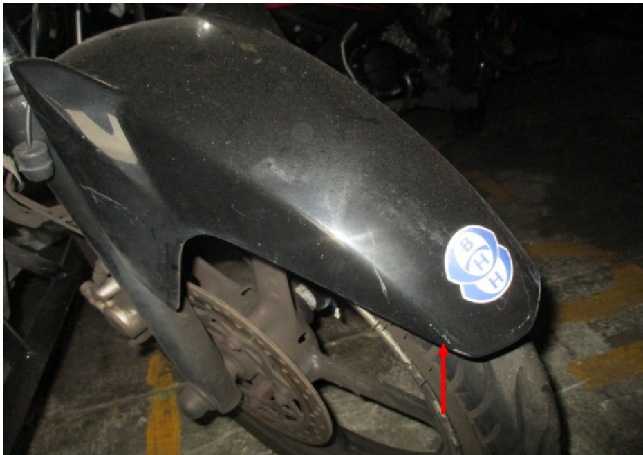
Photo 6 shows a closer view of the front mudguard, which was amongst the body parts of the Motorcycle that had sustained damage as a result of the accident (arrowed).
