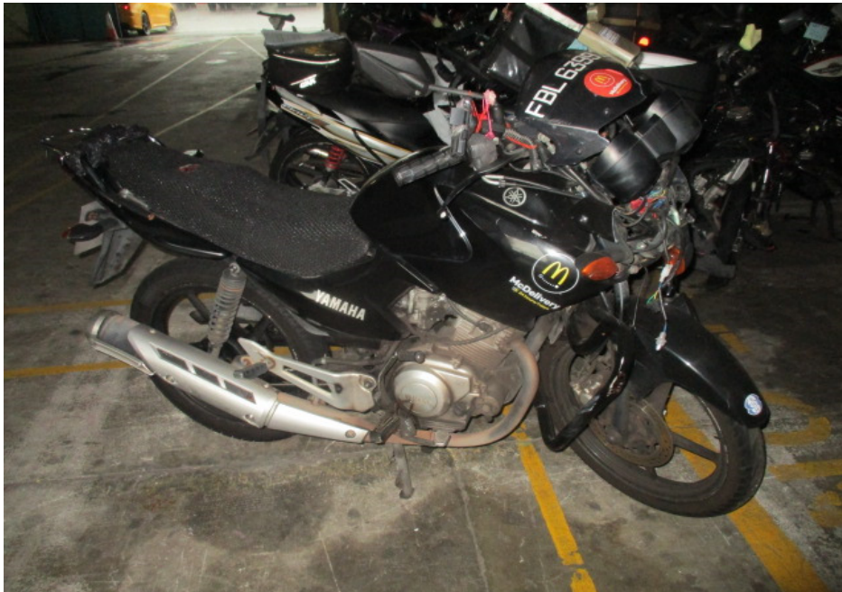
Photo 3 shows a general view of the right body of the Motorcycle at the time of our inspection. The Motorcycle had sustained damages all around. Body parts that were found to have been damaged include its headlight assembly, front fork assembly, front mudguard, left cowl, crash bars, side mirrors, front brake lever, clutch lever, handlebar ends, rear brake pedal, right front footrest and exhaust muffler, amongst others.
