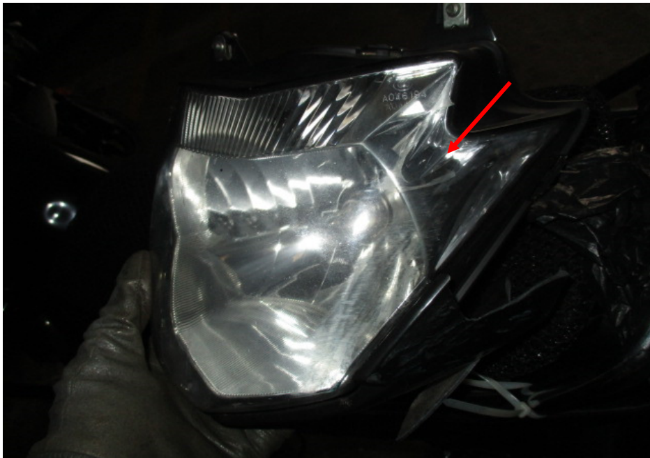
Photo 4 shows a closer view of the cracked headlight assembly of the Motorcycle as a result of the accident (arrowed).
