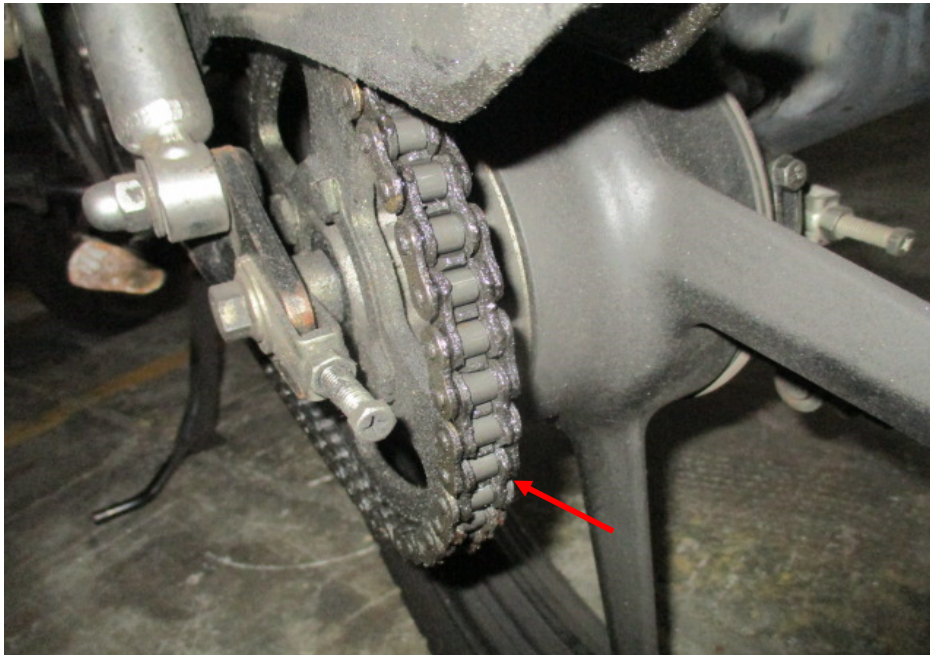
Photo 18 shows the closer view of the gear chain (arrowed) of the Motorcycle, which was observed to be intact with no misalignment. It was also adequately lubricated for operating purposes.
