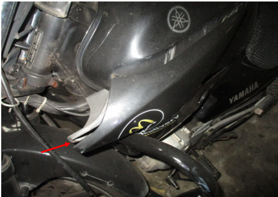
Photo 12 shows the deformed left cowling of the Motorcycle as a result of the accident at the time of our inspection (arrowed).
