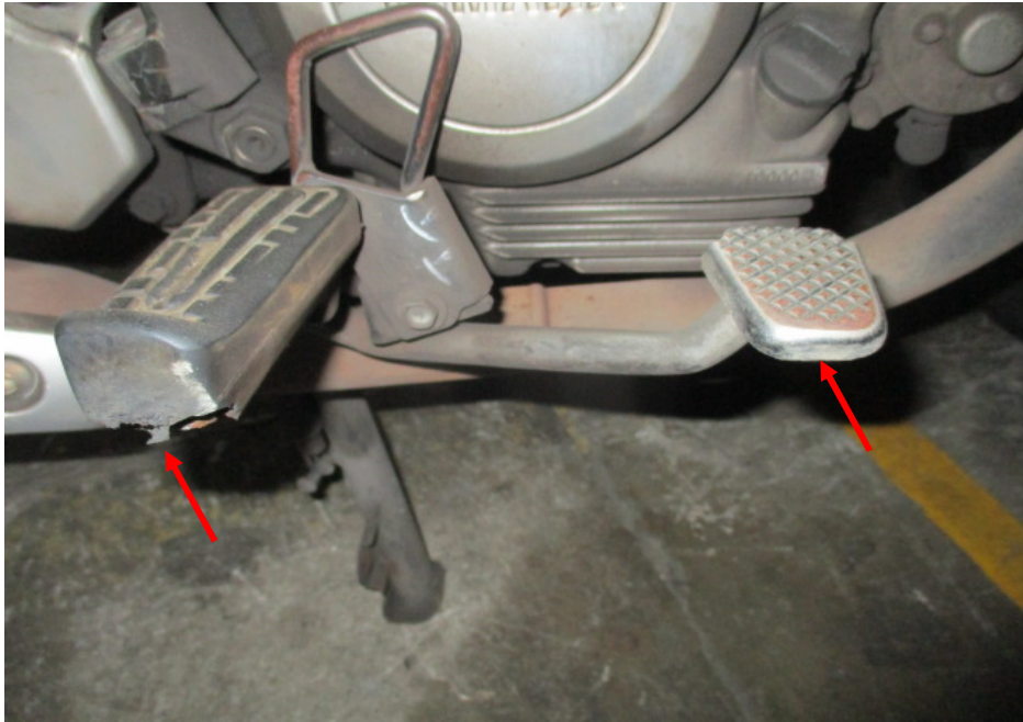
Photo 11 shows the rear brake pedal and right front footrest of the Motorcycle which sustained damages of grazing nature as a result of the accident (arrowed).
