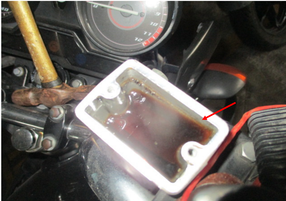
Photo 21 shows the brake fluid reservoir for the front brake of the Motorcycle. The brake fluid was found to be of sufficient level for operating purposes. However the brake fluid was found to be slightly contaminated (arrowed).
