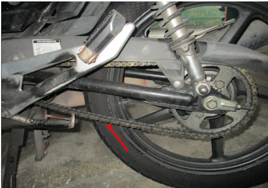
Photo 17 shows the gear chain (arrowed) of the Motorcycle, which was observed to be intact with no misalignment. It was also adequately lubricated for operating purposes. The gear chain rotates the rear wheel of the Motorcycle.
