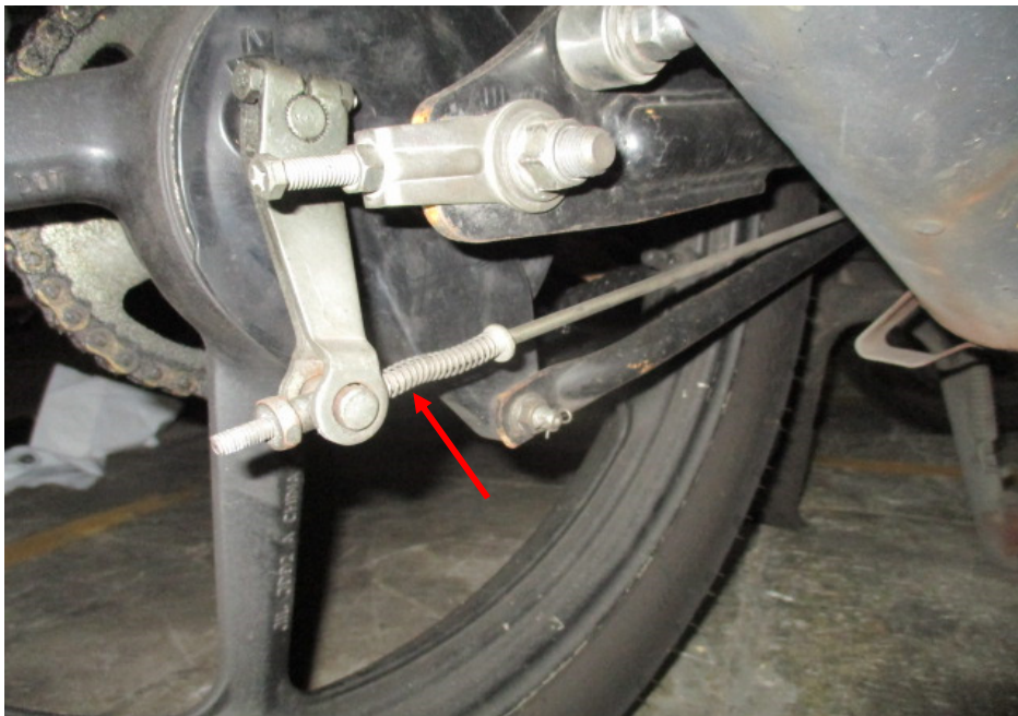
Photo 23 shows the rear wheel of the Motorcycle. The type of brake system for the rear wheel was of a mechanical type, controlled by the brake foot pedal of the Motorcycle. Our checks of the cable (arrowed), spring and drum which are all part of the components in the rear brake system of the Motorcycle reveal all to be intact and without damage.
