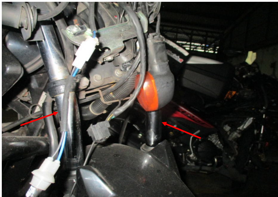
Photo 19 shows the front forks of the Motorcycle. The front forks were observed to be bent inwards as a result of the accident (arrowed). We were hence not able to conduct any tests on the steering system of the Motorcycle.
