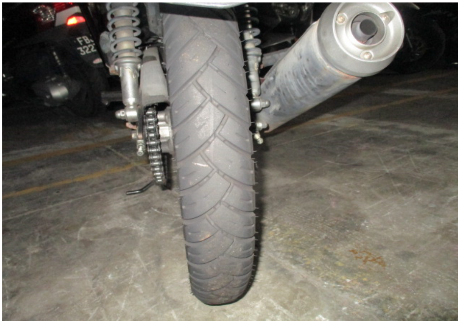
Photo 14 shows the condition of the Motorcycle's rear tyre. The rear tyre was observed to be in serviceable condition with remaining tread depth of approximately 4mm. The tyre was also observed to be sufficiently inflated for vehicular operation. We did not observe any tear, burst mark(s) and/or punctured hole(s) on the sidewalls as well as across the tread of the rear tyre.
