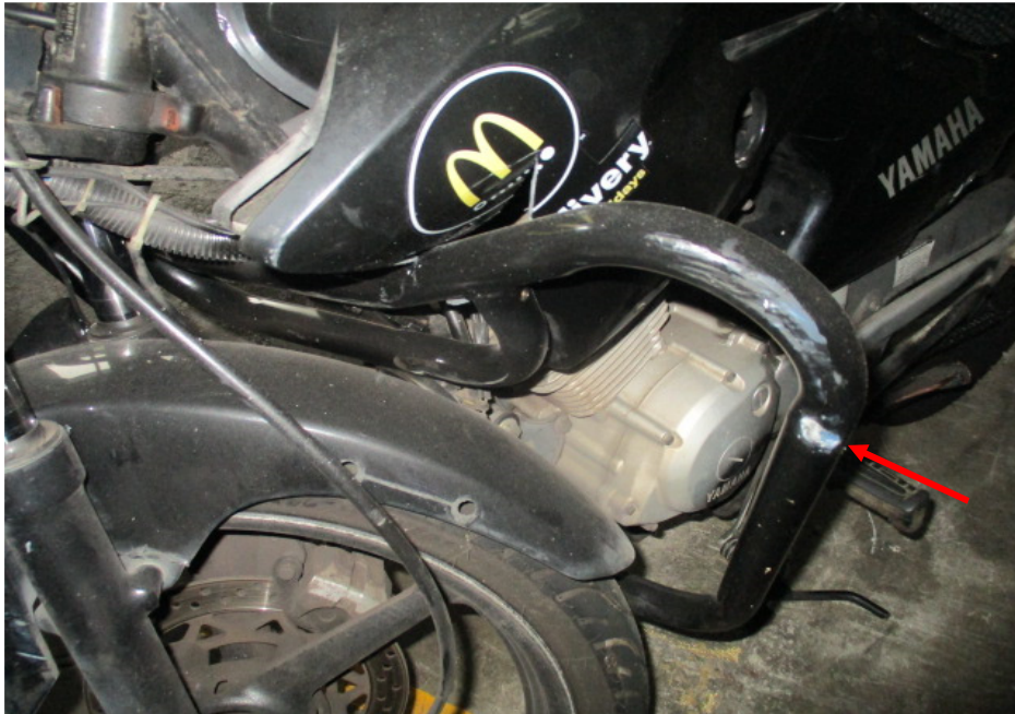
Photo 8 shows a closer view of the deformed left crash bar which was amongst the body parts of the Motorcycle that had sustained damages as a result of the accident (arrowed).
