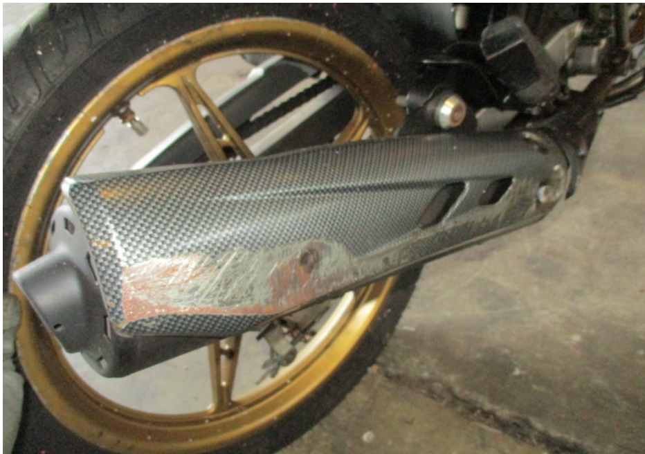
Photo 15 shows the exhaust muffler heat shield of the Motorcycle that had sustained damages of grazing nature as a result of the accident.
