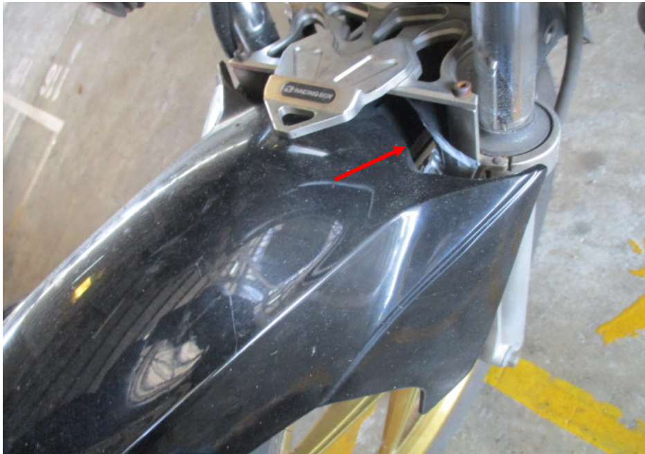
Photo 5 shows a closer view of the cracked front mudguard which was amongst the body parts of the Motorcycle that had sustained damage as a result of the accident.
