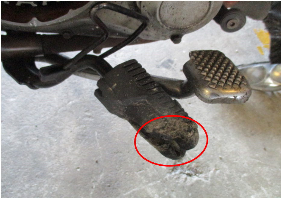
Photo 12 shows a closer view of the right front footrest which was amongst the body parts of the Motorcycle that had sustained damages as a result of the accident (circled).
