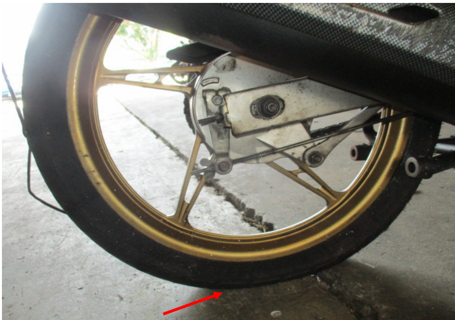
Photo 19 shows a closer view of the deflated rear tyre of the Motorcycle as a result of the accident (arrowed).
