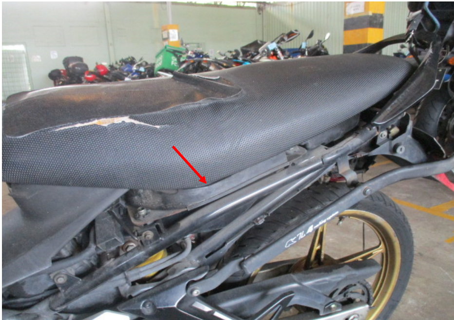
Photo 10 shows a closer view of the missing left rear side cover of the Motorcycle as a result of the accident (arrowed).
