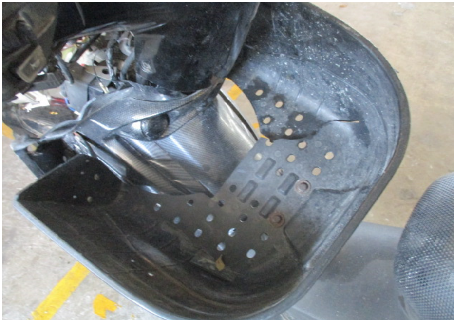
Photo 9 shows a closer view of the cracked front basket of the Motorcycle as a result of the accident.
