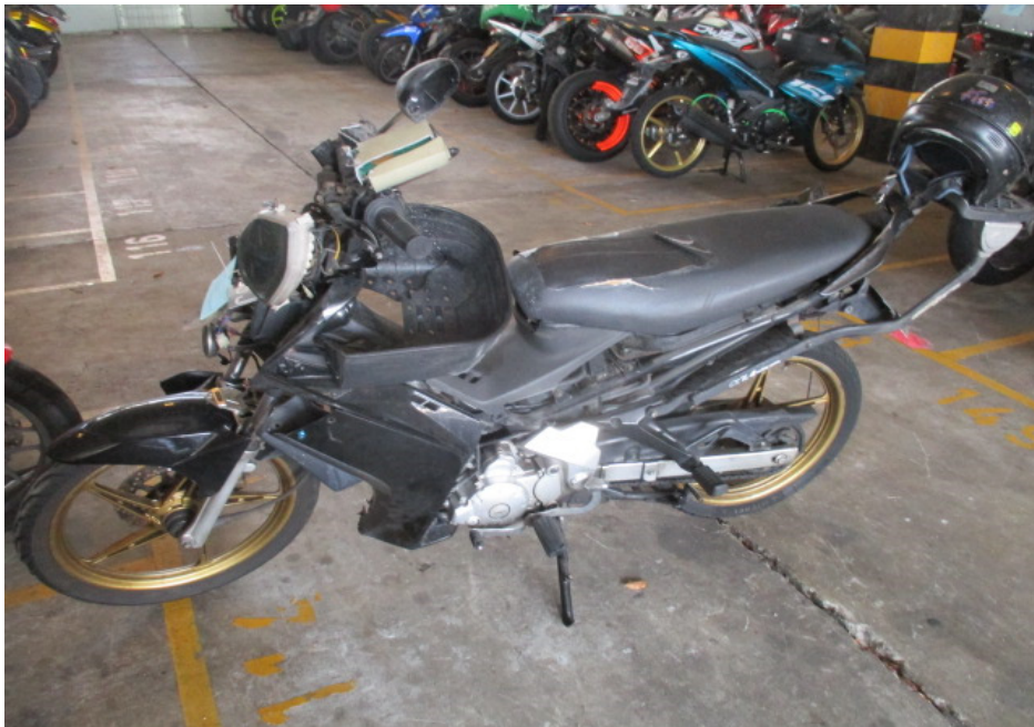
Photo 3 shows a general view of the left body of the Motorcycle at the time of our inspection. The Motorcycle was observed to have sustained damages all around body. Amongst the body parts that were found to have been damaged include its headlight assembly, front cowlings, front mudguard, side cowlings, front brake lever, clutch lever, rear side covers and tail light assembly, amongst others.
