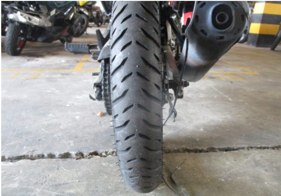
Photo 18 shows the condition of the Motorcycle's rear tyre. The rear tyre was observed to be in serviceable condition with remaining tread depth of approximately 4mm. The rear tyre was observed to be deflated as a result of the accident. We did not observe any tear, burst mark(s) and/or punctured hole(s) on the sidewalls as well as across the tread of the rear tyre.
