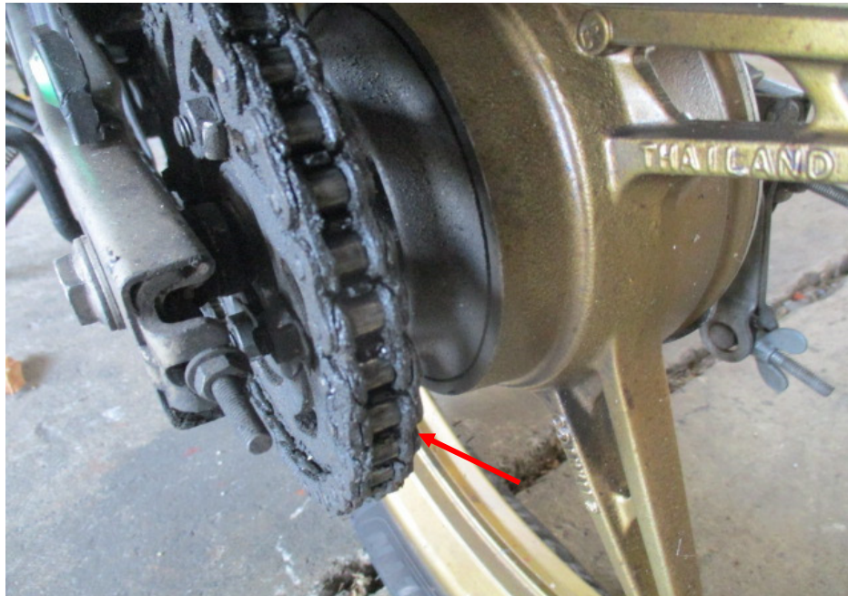
Photo 23 shows a closer view of the gear train (arrowed) of the Motorcycle, which was observed to be intact with no misalignment. It was also adequately lubricated for operating purposes.
