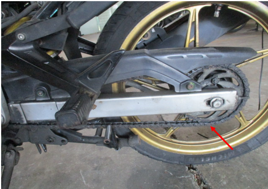
Photo 22 shows the general view of the gear train (arrowed) of the Motorcycle, which was observed to be intact with no misalignment. It was also adequately lubricated for operating purposes.
