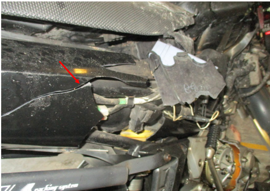
Photo 11 shows a closer view of the cracked right rear side cover of the Motorcycle as a result of the accident (arrowed).
