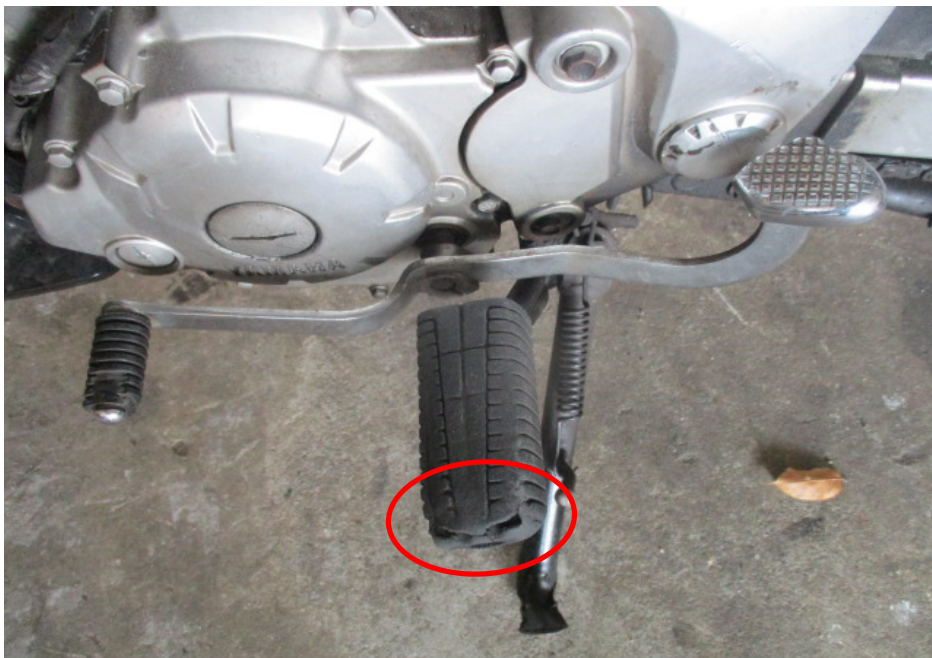
Photo 13 shows the left front footrest of the Motorcycle that had sustained damage as a result of the accident (circled).
