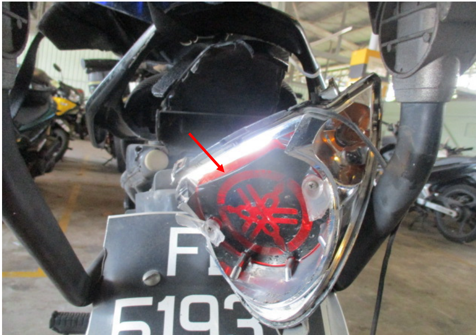
Photo 16 shows a closer view of the cracked tail light assembly of the Motorcycle as a result of the accident (arrowed).
