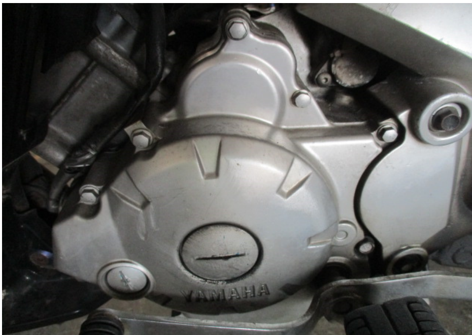
Photo 20 shows the left side of the engine of the Motorcycle at the time of our inspection. The various engine related parts and components were found to be intact with no visible damage. There was also no sign(s) or indication(s) of fluid leak observed around the left engine area of the Motorcycle.
