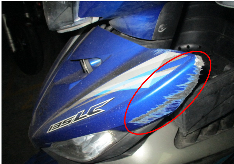
Photo 5 shows a closer view of the front cowling which was amongst the body parts of the Motorcycle that had sustained damage as a result of the accident (circled).
