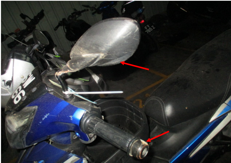
Photo 7 shows the left handlebar end and left side mirror (arrowed), which were amongst the body parts of the Motorcycle that had sustained damage as a result of the accident.
