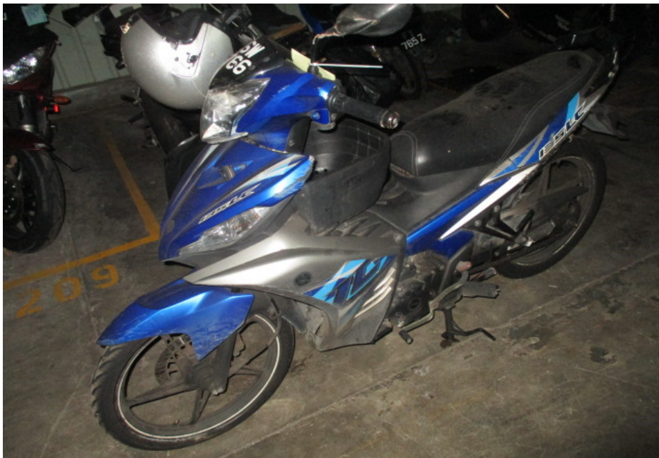
Photo 3 shows a general view of the left body of the Motorcycle at the time of our inspection. The Motorcycle was observed to have sustained damages at its frontal portion and left body. Amongst the body parts that were found to have been damaged include its windshield, headlight assembly, head cowl, front cowl, front mudguard, left cowl, left handlebar end, left side mirror, gear shift pedal, left front footrest, left rear side cover and pillion grab rail, amongst others.
