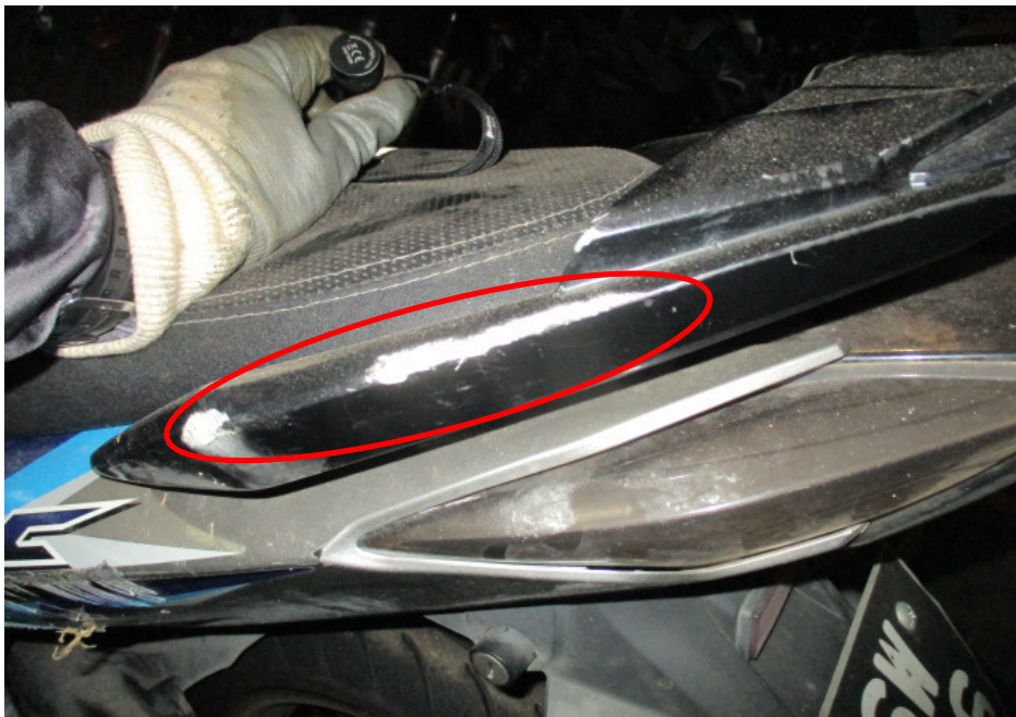
Photo 11 shows the pillion grab rail of the Motorcycle that had sustained damage as a result of the accident (circled).
