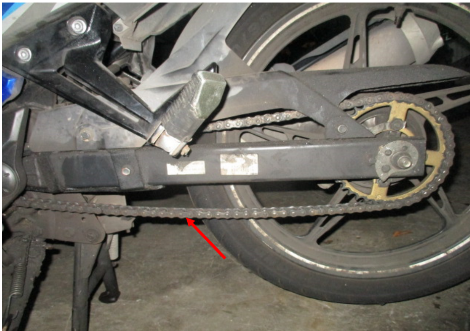
Photo 16 shows the general view of the gear train (arrowed) of the Motorcycle, which was observed to be intact with no misalignment. It was also adequately lubricated for operating purposes.
