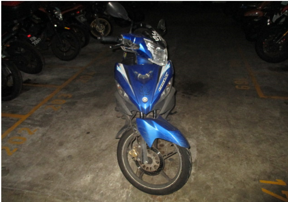
Photo 19 shows the front wheel of the Motorcycle turned towards its full left. Turning the Motorcycle's handle bar towards the left did not produce any abnormal free play and/or resistance. This would indicate that the steering system of the Motorcycle was in serviceable condition at the time of our inspection.
