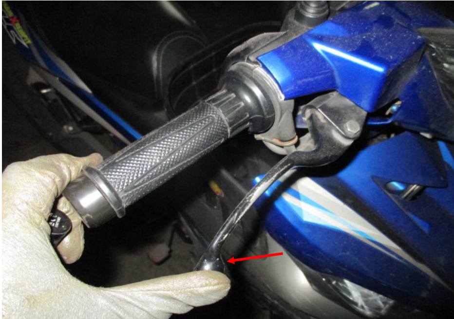
Photo 23 shows the front brake lever being depressed. There was some resistance felt (spongy like feel) upon pressing the front brake lever (arrowed). This would indicate that there is no leakage of pressure/vacuum in the front brake system.
