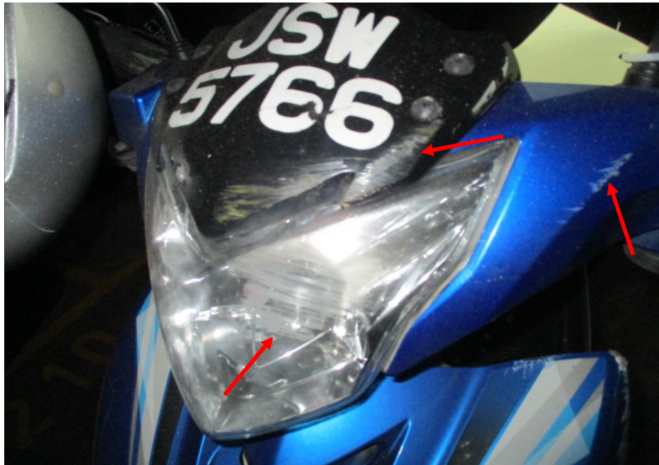
Photo 4 shows a close up view of the windshield, headlight assembly and head cowl which was amongst the body parts at the front of the Motorcycle that had sustained damage as a result of the accident (arrowed).
