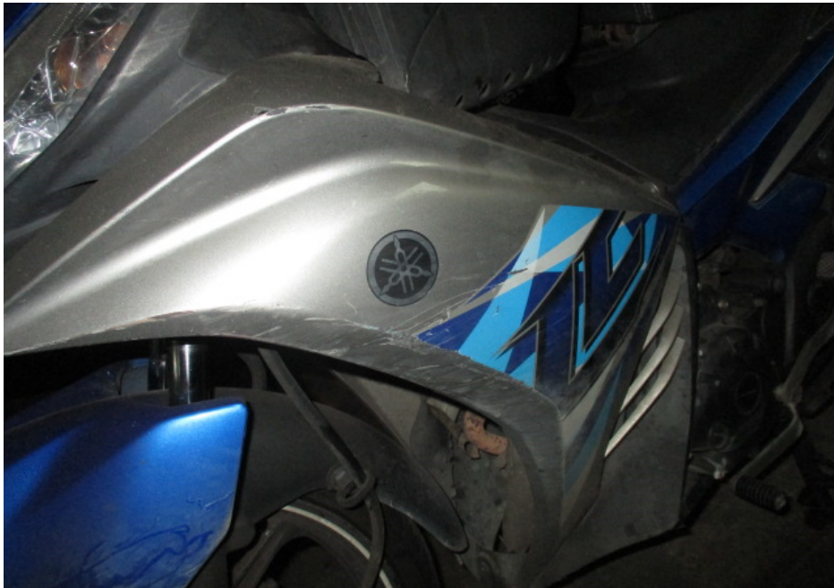
Photo 8 shows the left cowling which was amongst the body parts of the Motorcycle that had sustained damage as a result of the accident.
