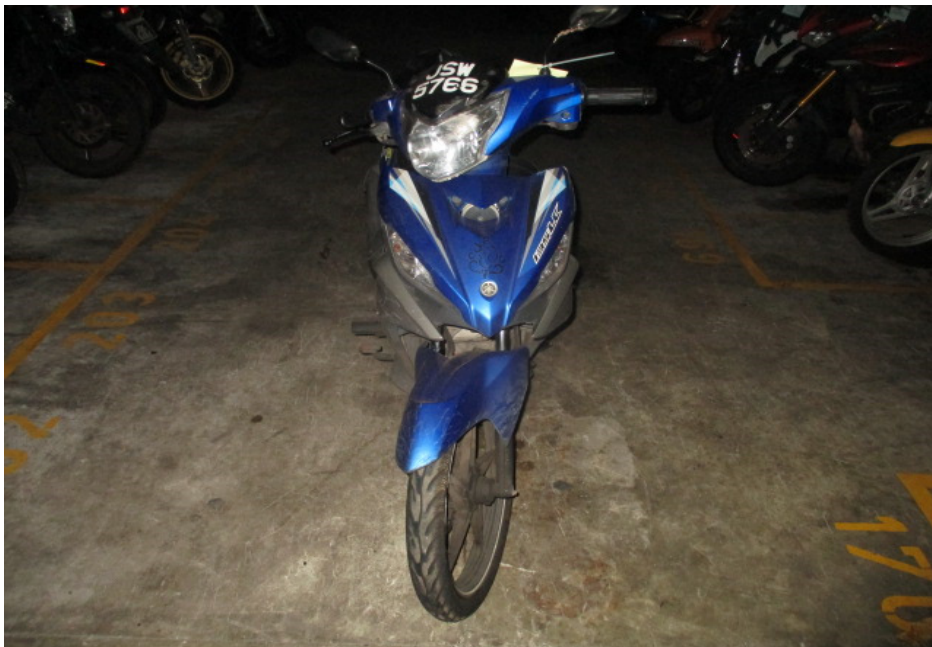
Photo 20 shows the front wheel of the Motorcycle turned towards its full right. Turning the Motorcycle's handle bar towards the right did not produce any abnormal free play and/or resistance. This would indicate that the steering system of the Motorcycle was in serviceable condition at the time of our inspection.
