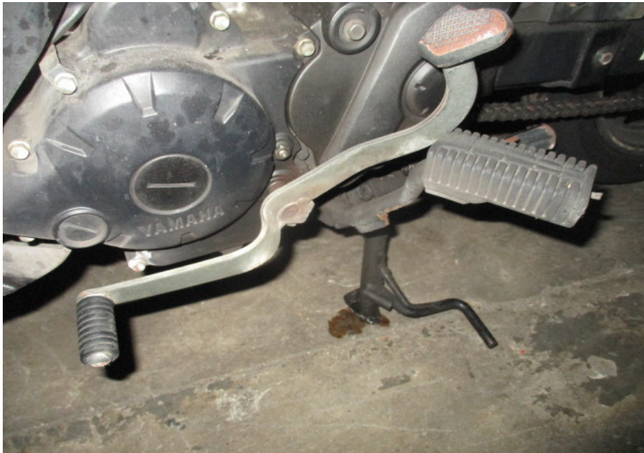
Photo 10 shows the gear shift pedal and left front footrest of the Motorcycle that had sustained damage as a result of the accident.
