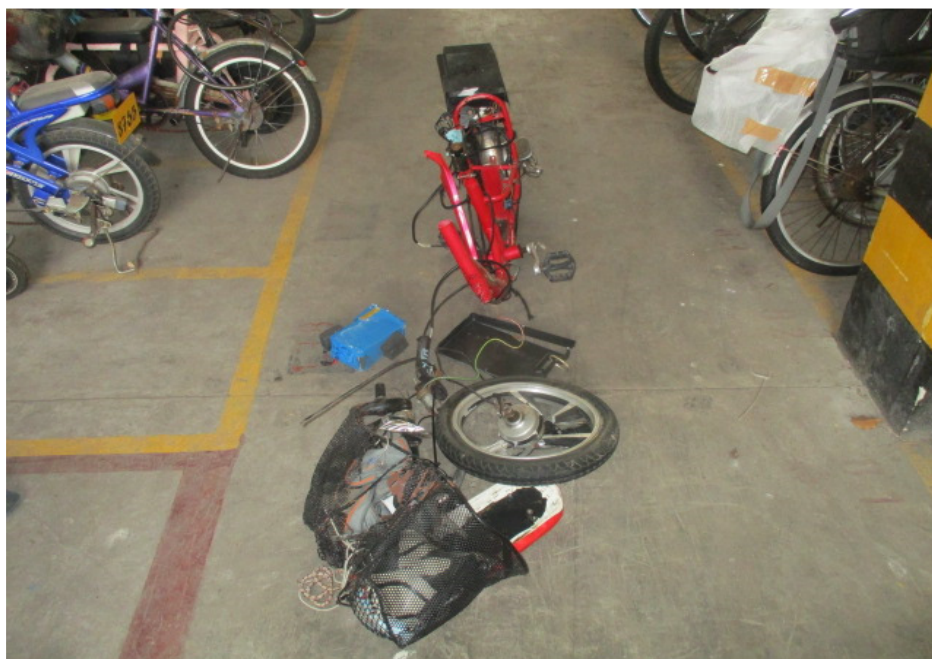
Photo 2 shows the frontal portion of the E-bike at the time of our inspection. The E-bike was observed to have sustained damages all around.
