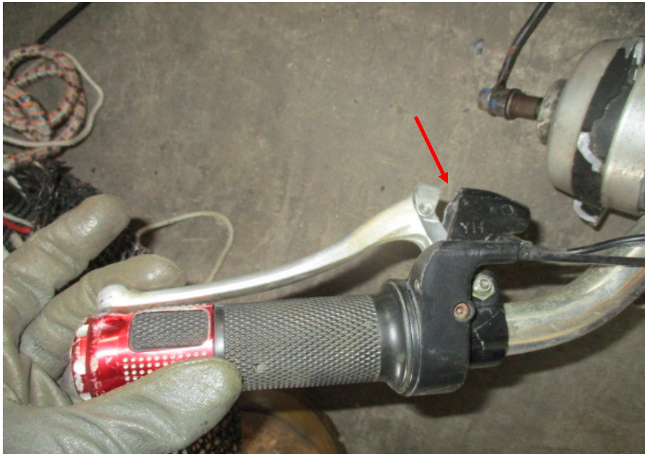
Photo 19 shows the right hand brake lever of the E-bike when depressed. The brake cable was observed to be dislodged as a result of the accident (arrowed). Hence a static brake test could not be conducted on the E-bike's braking system.
