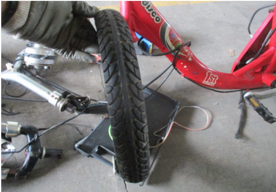
Photo 11 shows the front tyre of the E-bike at the time of our inspection. The front tyre was observed to be in serviceable condition with remaining tread depth of approximately 3mm. The tyre was also observed to be sufficiently inflated for vehicular operation. We did not observe any tear, burst mark(s) and/or punctured hole(s) on the sidewalls as well as across the tread of the front tyre.
