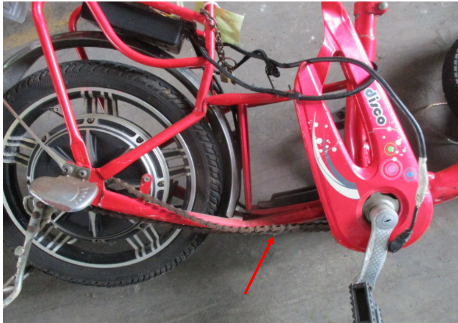
Photo 16 shows the general view of the gear train of the E-bike, which was observed to be intact with no misalignment. It was also adequately lubricated for operating purposes. However the chain was observed to be dislodged from the gear train most likely as a result of the accident (arrowed).
