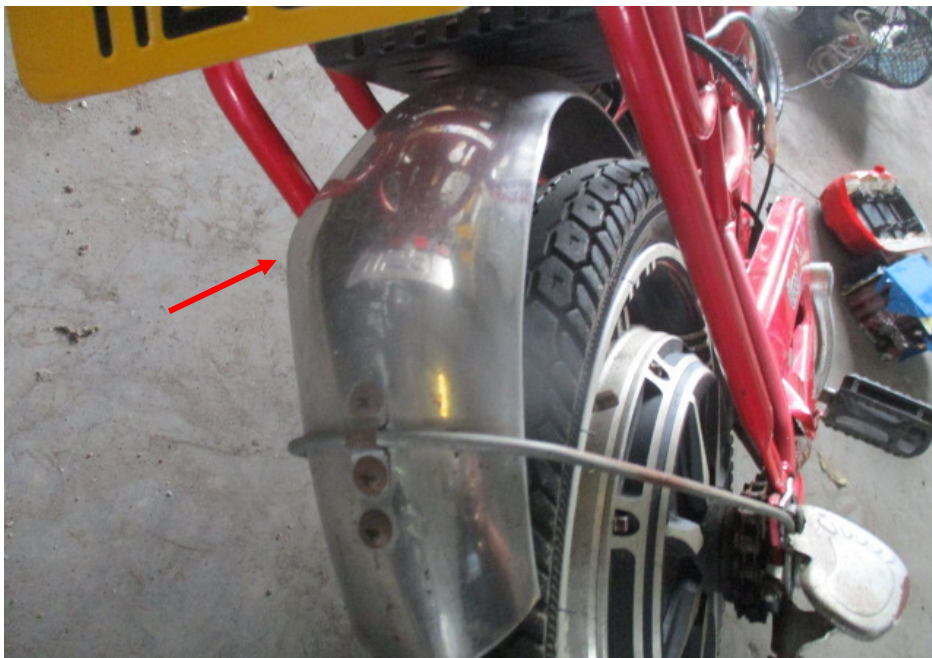
Photo 10 shows the deformed rear mudguard of the E-bike as a result of the accident (arrowed).
