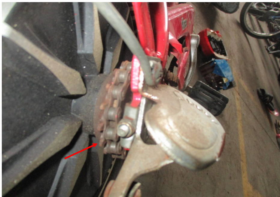
Photo 17 shows a closer view of the dislodged chain from the gear train of the E-bike, most likely as a result of the accident (arrowed). It was found to be adequately lubricated for operating purposes.
