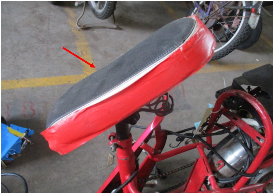
Photo 9 shows the deformed seat of the E-bike as a result of the accident (arrowed).
