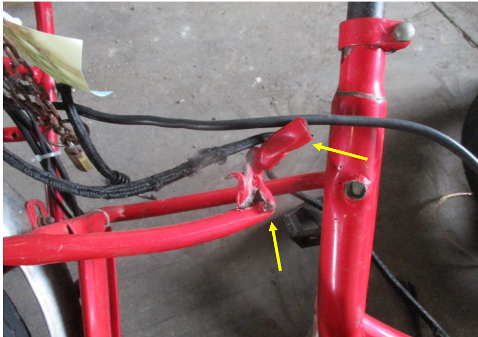
Photo 7 shows the damages on the body frame of the E-bike as a result of the accident (arrowed).
