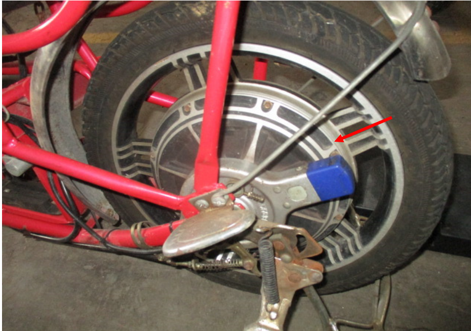
Photo 14 shows the general view of the drive motor (arrowed) of the E-bike which was observed to be intact with no misalignment. However it was observed not to be in operational condition due to the dislodged battery as a result of the accident.
