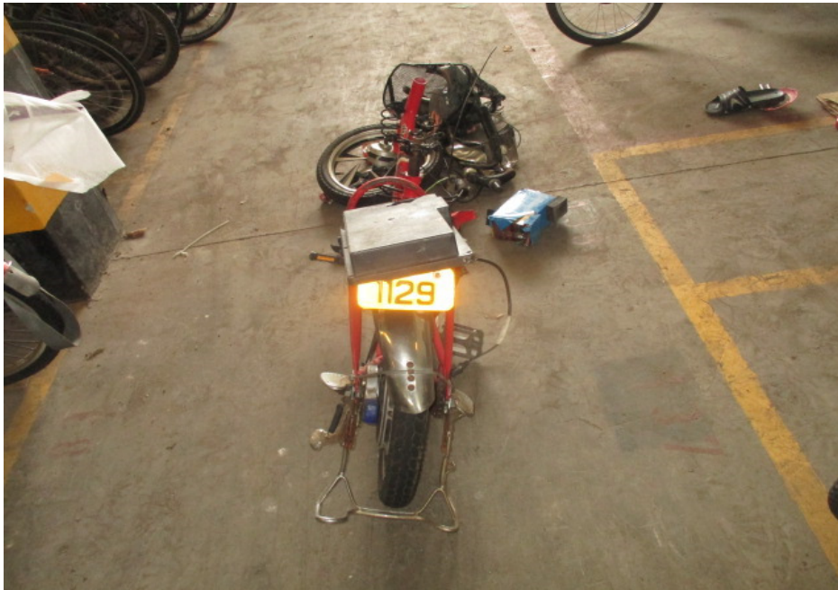
Photo 5 shows the rear portion of the E-bike at the time of our inspection. The E-bike was observed to have sustained damages all around. The body parts that were found to have been damaged include its fork assembly, hand brake levers, handlebar, basket, front wheel rim, seat, body frame and rear mudguard, amongst others as a result of the accident.
