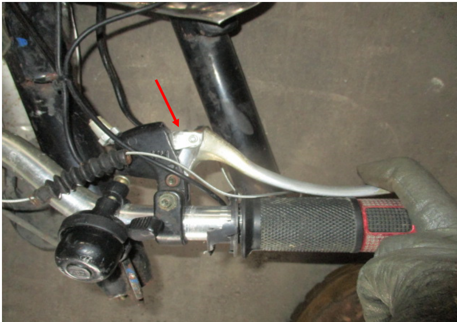
Photo 20 shows the bent left hand brake lever of the E-bike as a result of the accident (arrowed). Hence a static brake test could not be conducted on the E-Bike's braking system.
