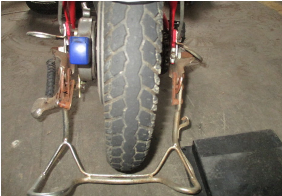
Photo 12 shows the rear tyre of the E-bike at the time of our inspection. The rear tyre was observed to be in serviceable condition with remaining tread depth of approximately 3mm. We did not observe any tear, burst mark(s) and/or punctured hole(s) on the sidewalls as well as across the tread of the rear tyre. The tyre was also observed to be sufficiently inflated for vehicular operation.
