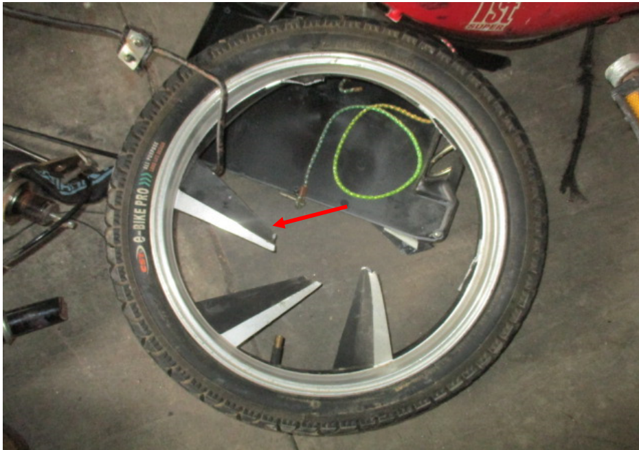
Photo 13 shows the broken front wheel rim of the E-bike as a result of the accident (arrowed).
