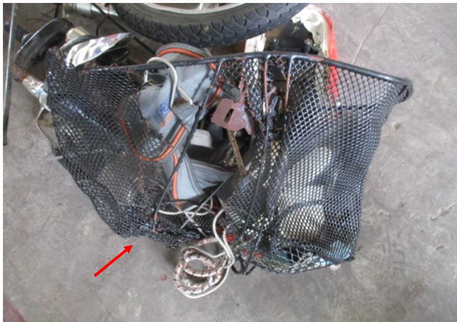
Photo 8 shows the deformed basket of the E-bike as a result of the accident (arrowed).
