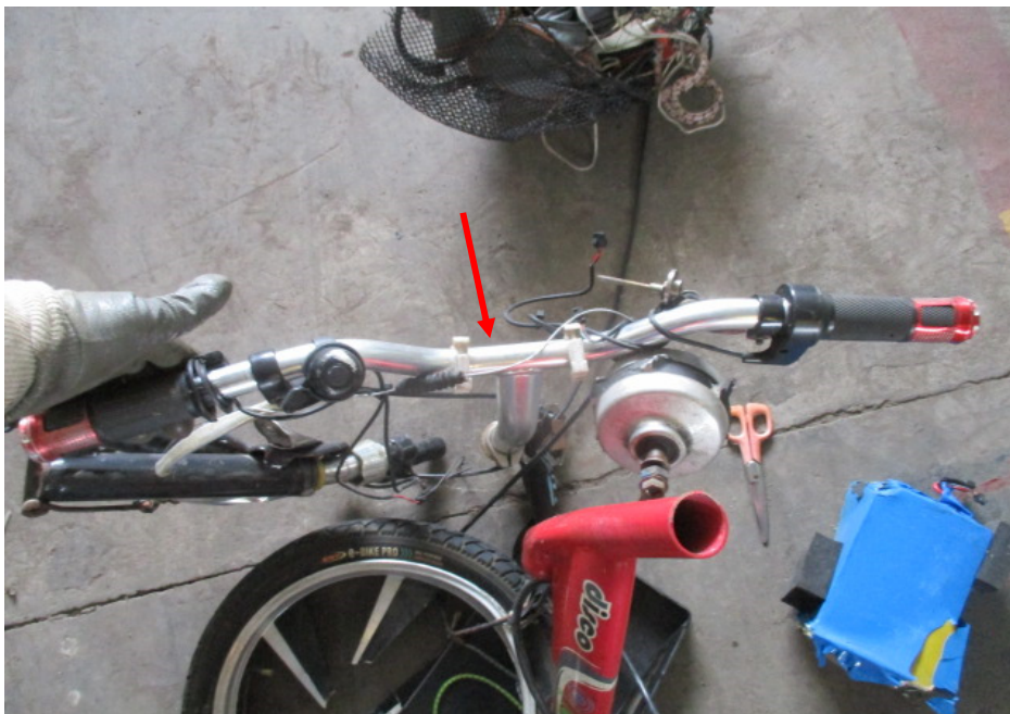
Photo 6 shows the dislodged handlebar (arrowed) of the E-bike as a result of the accident.
