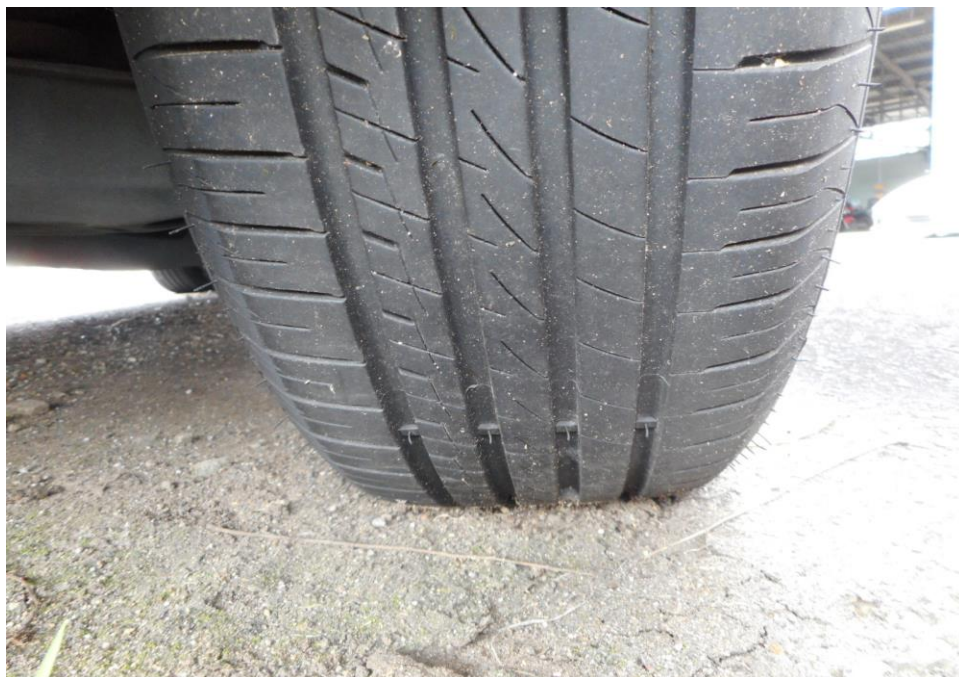
Photo 9 shows the condition of the rear right tyre of the Motor Car, which was observed to be in serviceable condition with remaining tread depth of approximately 6.3mm. The tyre was also observed to be sufficiently inflated for vehicular operation with no tear, cut or burst mark(s).
