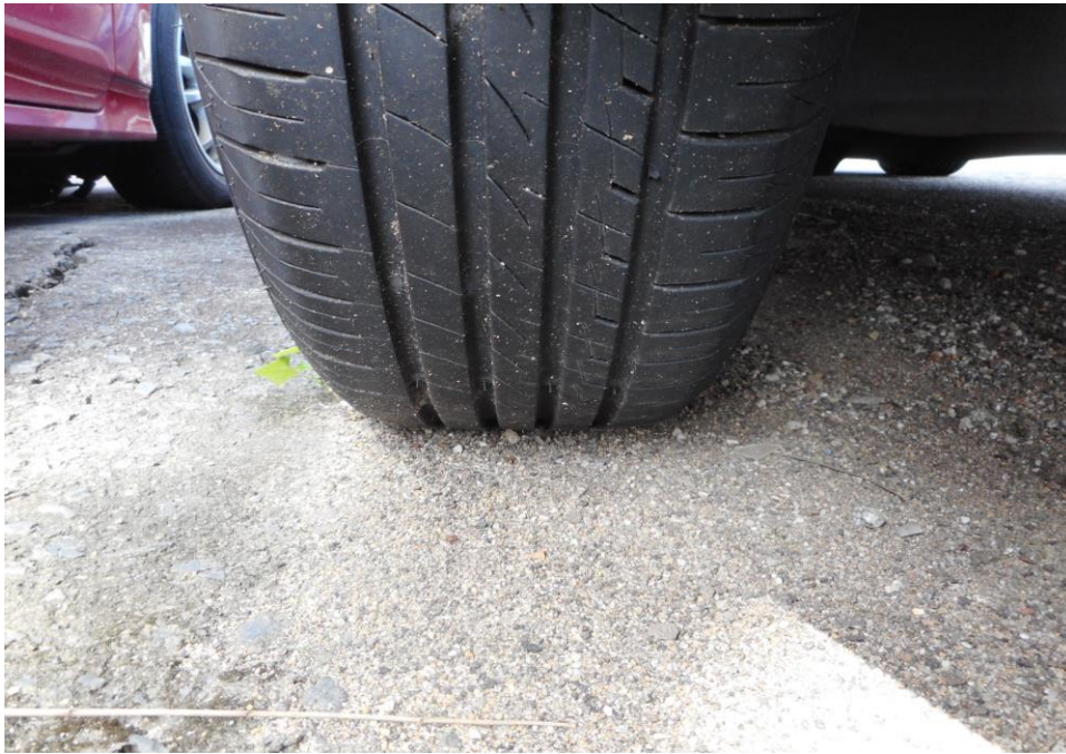
Photo 10 shows the condition of the rear left tyre of the Motor Car, which was observed to be in serviceable condition with remaining tread depth of approximately 6mm. The tyre, which was wrapped around steel wheel rim, was also observed to be sufficiently inflated for vehicular operation. The 4 tyres of the Motor Car were wrapped around standard steel wheel rims.
