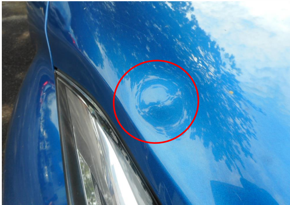
Photo 4 shows the close up view of the Motor Car's front body at the time of my inspection. The Motor Car was observed to have sustained damage at its front bonnet (circled) as a result of the accident.
