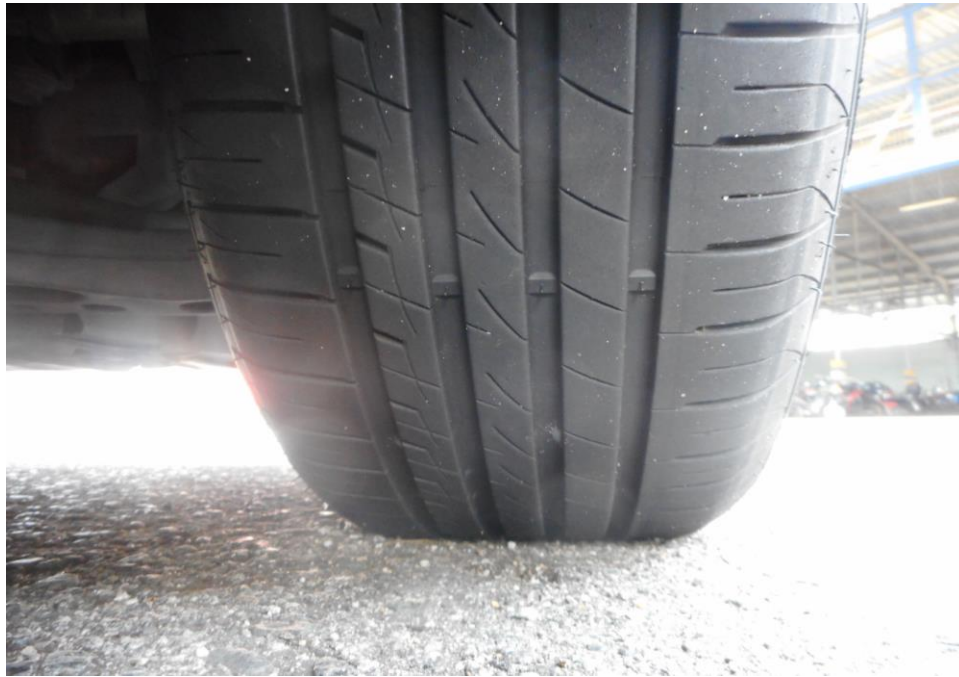
Photo 8 shows the condition of the front right tyre of the Motor Car, which was observed to be in serviceable condition with remaining tread depth of approximately 6.5mm. The tyre was sufficiently inflated for vehicular operation with no tear, cut or burst mark(s) on the outer and the inner sidewalls as well as across the tread. The 4 tyres of the Motor Car were wrapped around standard steel wheel rims without any damage.
