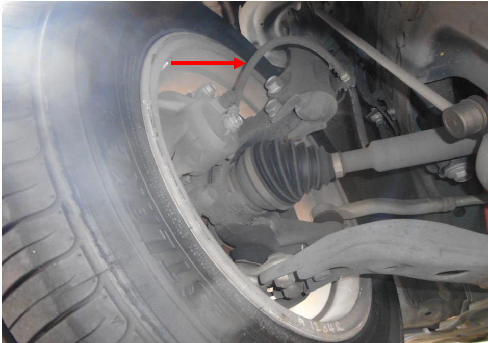
Photo 18 shows the brake hose/pipe (arrowed) at the front right wheel of the Motor Taxi. I did not observe any leakage of brake fluid at the time of my inspection of the Motor Taxi. Static tests of the Motor Taxi's braking system had indicated that there was no internal leakage of pressure/vacuum. The undercarriage components of the Motor Taxi were also all found to be intact and without any visible damage.
