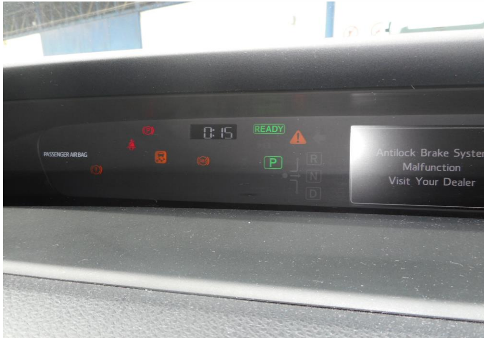
Photo 23 However, the Anti-Lock Brake System (ABS) and Traction Control System (arrowed) lights remained illuminated on the instrument panel of the Motor Taxi after the engine was cranked. This was likely caused by the result of the accident.
