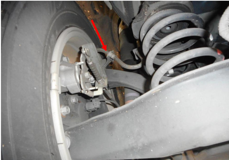
Photo 17 shows the brake hose/pipe (arrowed) at the rear left wheel of the Motor Taxi. I did not observe any leakage of brake fluid at the time of my inspection of the Motor Taxi. Static tests of the Motor Taxi's braking system had indicated that there was no internal leakage of pressure/vacuum. The undercarriage components of the Motor Taxi were also all found to be intact and without any visible damage.
