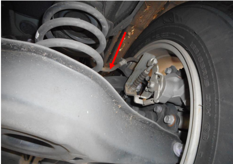
Photo 16 shows the brake hose/pipe (arrowed) at the rear right wheel of the Motor Taxi. No leakage of brake fluid was observed. Visual examination of the various components of the braking system like the drum brake, brake booster, brake pedal etc. had revealed all to be intact and without visible damage.
