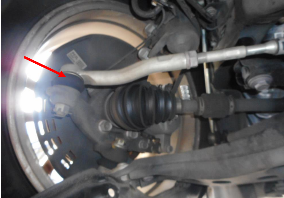
Photo 21 shows the various undercarriage components at the front left wheel of the Motor Taxi, in particular the steering tie rod (red arrow) and drive shaft (yellow arrow). The various steering components were all found to be intact, suggesting that the steering system of the Motor Taxi was likely to be in serviceable condition at the material time of accident. There was also no sign of fluid stain observed on the various undercarriage components at the front left wheel of the Motor Taxi.
