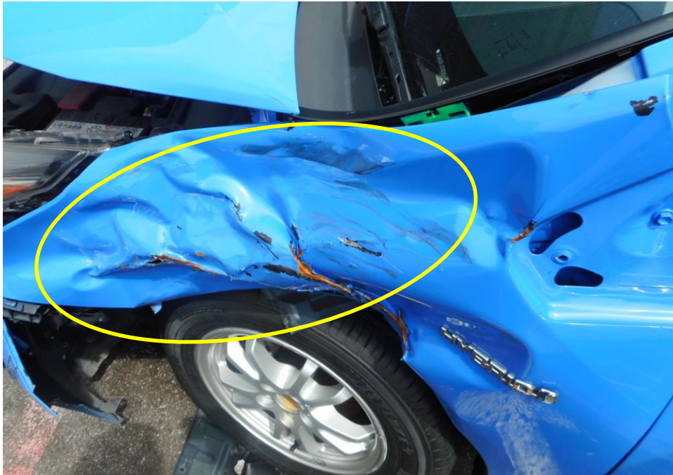
Photo 4 shows the close up view of the Motor Taxi's front left body at the time of my inspection. The Motor Taxi was observed to have sustained damage at its front left fender (circled) were amongst the body parts that were damaged as a result of the accident.
