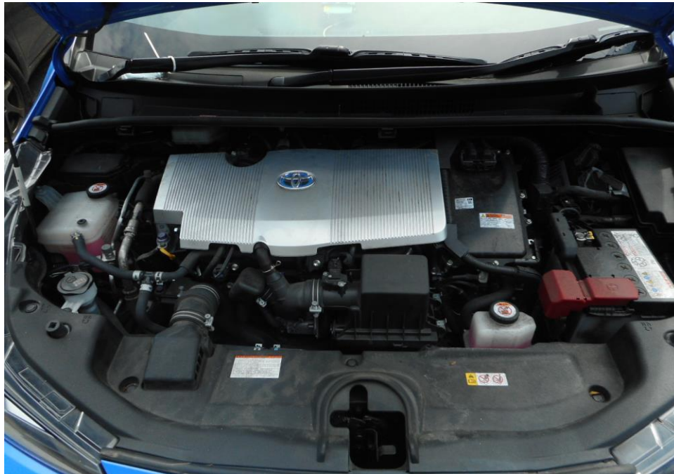
Photo 11 shows a general view of the Motor Taxi's engine compartment. The various parts and components inside the engine compartment were unaffected by the accident. There was also no sign(s) or indication(s) of fluid leakage and/or fluid stain within the engine compartment.
