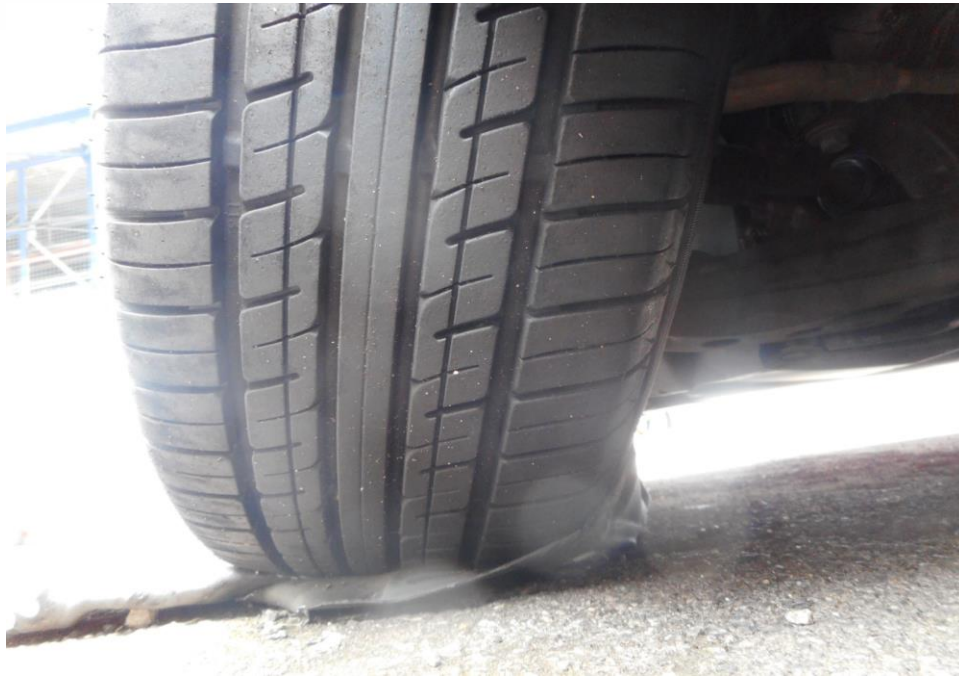
Photo 10 shows the condition of the front left tyre of the Motor Taxi, which was observed to be in serviceable condition with remaining tread depth of approximately 6.1mm. There was also no tear, cut or burst mark(s) on the outer and the inner sidewalls as well as across the tread of the Motor Taxi's 4 tyres.
