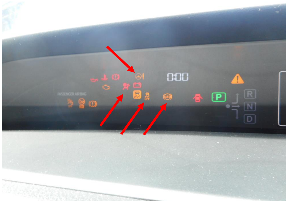
Photo 22 shows the warning light for the Supplemental Restraint System (SRS), Electric Power Steering System (EPS), Anti-Lock Brake System (ABS) and Traction Control System (arrowed) appearing on the instrument panel of the Motor Taxi during the self-test of its various electronic operating systems when its engine was cranked.
