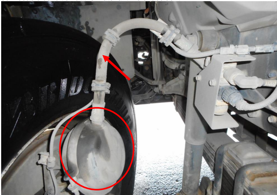
Photo 24 shows the brake hose/pipe (arrowed) at the front left wheel of the Motor Lorry. I did not observe any leakage of brake fluid at the time of my inspection of the Motor Lorry. My static tests of the Motor Lorry's braking system, along with my visual examination of the various mechanical components in the braking system had indicated that there was no internal leakage of pressure/vacuum. Hence the braking system of the Motor Lorry was likely to be in serviceable condition at the material time of accident.
