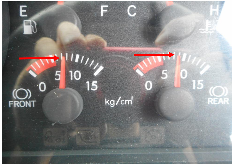
Photo 14 shows the air-brake reservoir of the Motor Lorry at the time of my inspection. The air-brake was observed to be of sufficient level (arrowed) and without any visible contamination.
