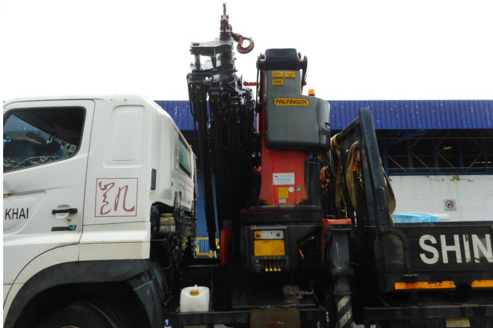
Photo 11 shows a general view of the Motor Lorry's Crane from the right side at the time of my inspection. The Crane was observed to be intact and unaffected by the accident.
