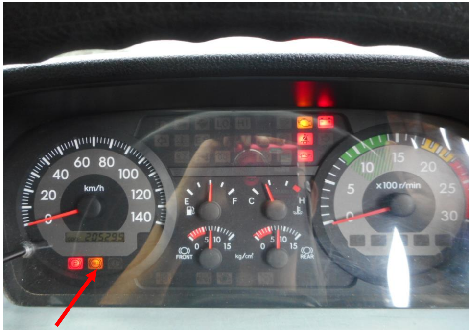
Photo 27 shows the warning light for Anti-Lock Brake System (ABS) appearing on the instrument panel of the Motor Lorry during the self-test of its various electronic operating systems when its engine was cranked.
