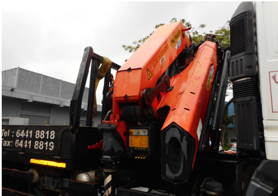
Photo 10 shows a general view of the Motor Lorry's Crane from the right side at the time of my inspection. The Crane was observed to be intact and unaffected by the accident.
