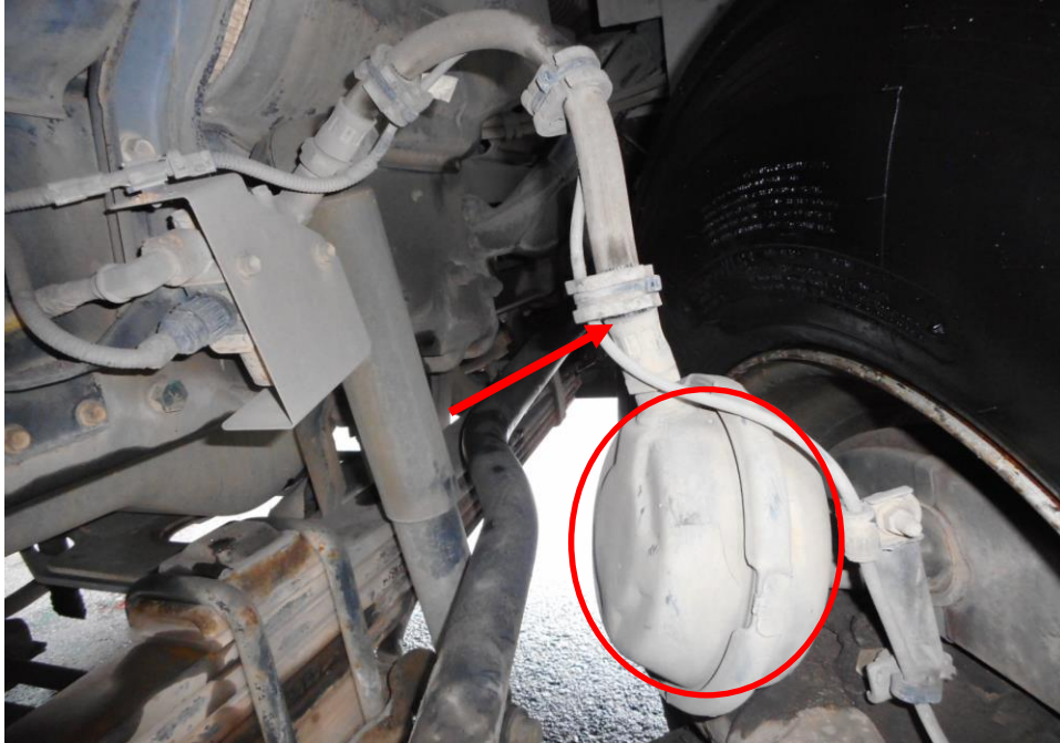
Photo 23 shows the brake hose/pipe (arrowed) at the front right wheel of the Motor Lorry. I did not observe any leakage of brake fluid at the time of my inspection of the Motor Lorry. My static tests of the Motor Lorry's braking system, along with my visual examination of the various mechanical components in the braking system had indicated that there was no internal leakage of pressure/vacuum. Hence the braking system of the Motor Lorry was likely to be in serviceable condition at the material time of accident.
