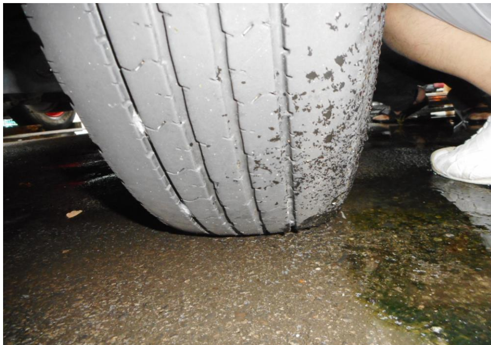
Photo 9 shows the condition of the rear right tyres of the Motor Lorry, which were observed to be in serviceable condition with remaining, tread depth of approximately 4.5mm. There was also no tear, cut or burst mark(s) on the outer and the inner sidewalls as well as across the tread of the 10 tyres that were fitted on the Motor Lorry.
