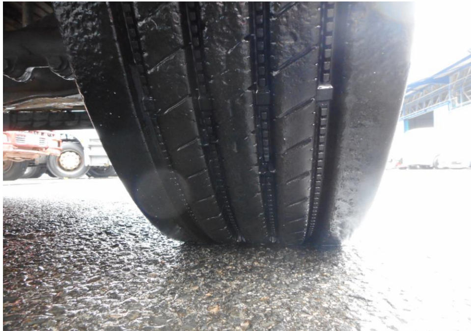
Photo 6 shows the condition of the front right tyre of the Motor Lorry, which was observed to be in serviceable condition with remaining tread depth of approximately 13.5mm. The tyre, which was wrapped around standard steel wheel rim, was also observed to be sufficiently inflated for vehicular operation. There was no tear, cut or burst mark(s) on the outer and the inner sidewalls as well as across the tread of the 10 tyres that were fitted on the Motor Lorry.
