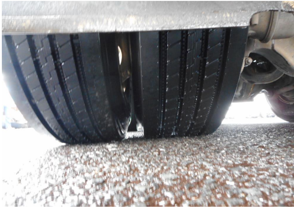
Photo 8 shows the condition of the rear left tyres of the Motor Lorry, which was observed to be in serviceable condition with remaining tread depth of approximately 11.4mm. The tyres, which were wrapped around standard steel wheel rim, were also observed to be sufficiently inflated for vehicular operation. There was also no damage found on all 10 steel wheel rims of the Motor Lorry.
