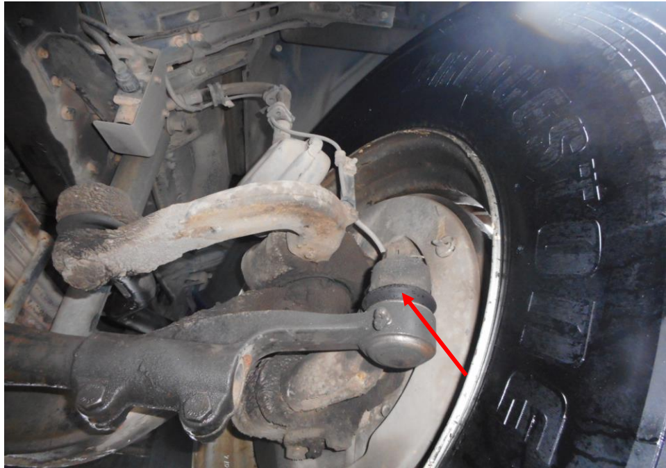
Photo 19 shows the various undercarriage components at the front right wheel of the Motor Lorry, in particular the steering tie rod end (arrowed). The various steering components were all found to be intact, suggesting that the steering system of the Motor Lorry was likely to be in serviceable condition at the material time of accident. There was also no sign of fluid stain(s) observed on the various undercarriage components.
