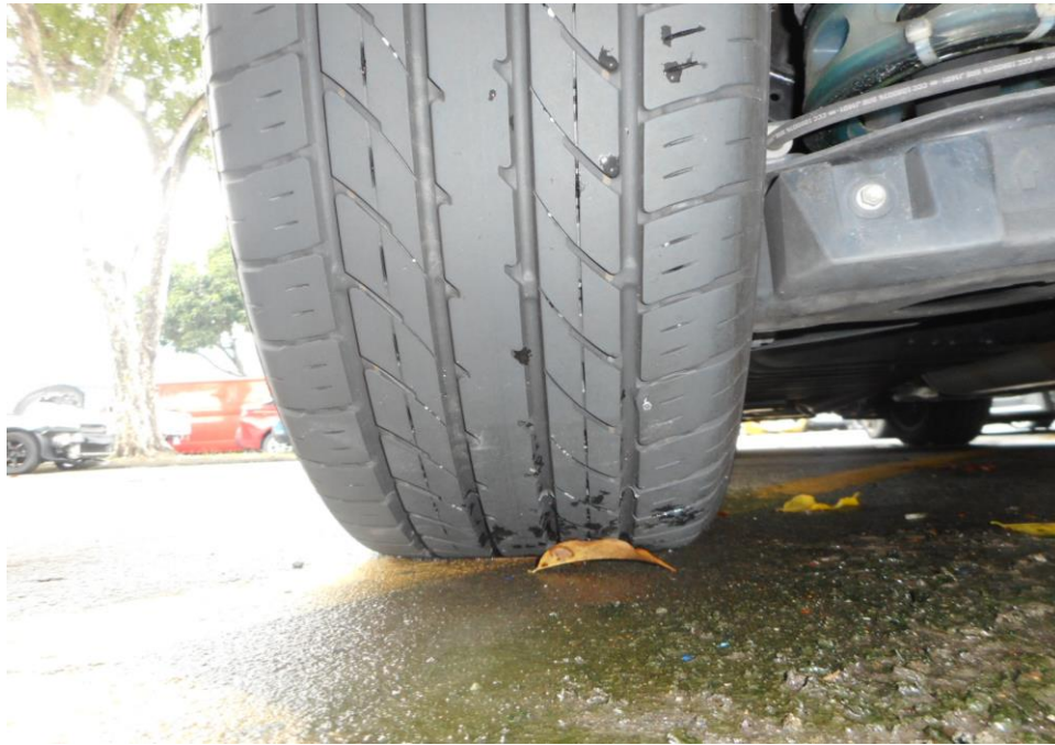
Photo 10 shows the condition of the rear left tyre of the Motor Car, which was observed to be in serviceable condition with remaining tread depth of approximately 5.4mm. The tyre, which was wrapped around steel wheel rim, was also observed to be sufficiently inflated for vehicular operation. The 4 tyres of the Motor Car were wrapped around standard steel wheel rims.
