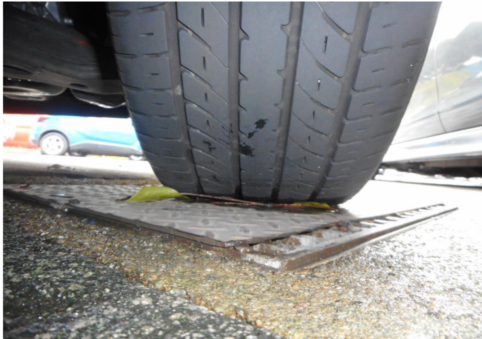
Photo 8 shows the condition of the front right tyre of the Motor Car, which was observed to be in serviceable condition with remaining tread depth of approximately 3.2mm. The tyre was sufficiently inflated for vehicular operation with no tear, cut or burst mark(s) on the outer and the inner sidewalls as well as across the tread. The 4 tyres of the Motor Car were wrapped around standard steel wheel rims without any damage.
