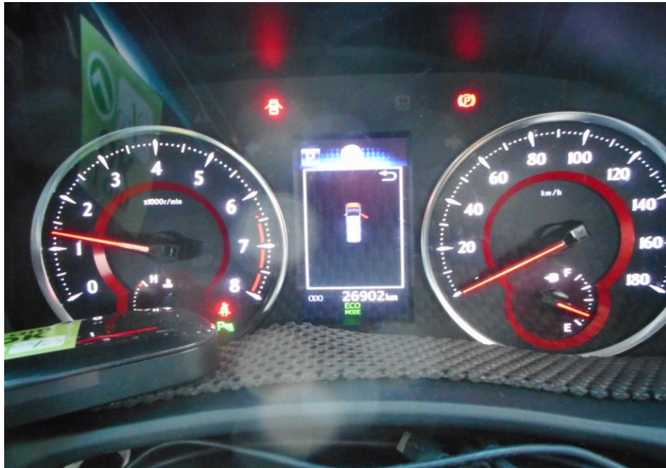
Photo 25 shows no warning lights illuminated on the instrument panel of the Motor Car after the engine was cranked. This would suggest that there was no abnormality to the electronic operating system of the Motor Car, like the ABS, EPS, TC and SRS etc.
