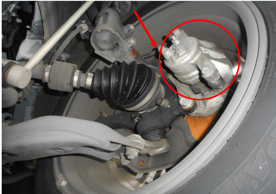
Photo 20 shows the brake hose/pipe (arrowed) at the front left wheel of the Motor Car. No leakage of brake fluid was observed. Visual examination of the various components of the braking system like the brake caliper (circled), brake booster, brake pedal etc had revealed all to be intact and without visible damage.
