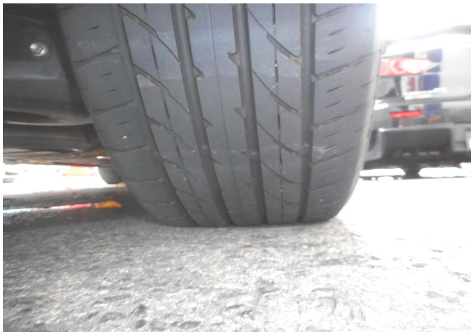
Photo 9 shows the condition of the rear right tyre of the Motor Car, which was observed to be in serviceable condition with remaining tread depth of approximately 6mm. The tyre was also observed to be sufficiently inflated for vehicular operation with no tear, cut or burst mark(s).
