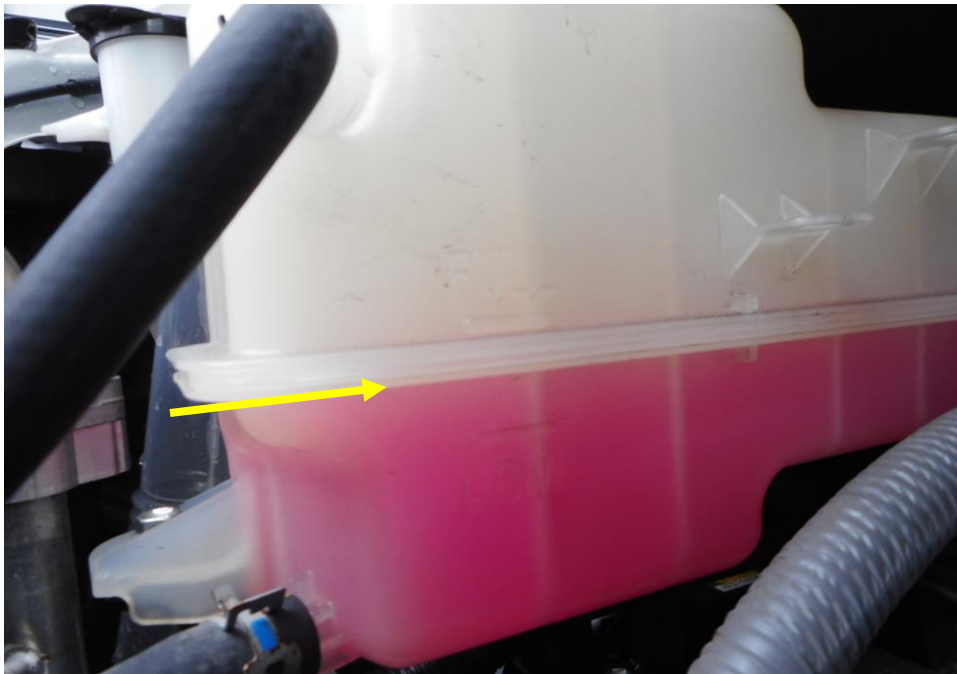
Photo 14 shows checks being carried out to the engine coolant of the Motor Car at the time of my inspection. The engine coolant was observed to be of insufficient level (arrowed) likely due to the damaged to the front radiator which caused the leakage of coolant.
