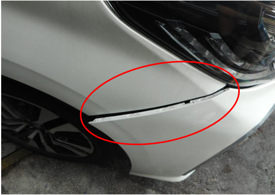
Photo 4 shows the close up view of the Motor Car's front body at the time of my inspection. The Motor Car was observed to have sustained damage at its front bumper (circled) as a result of the accident.
