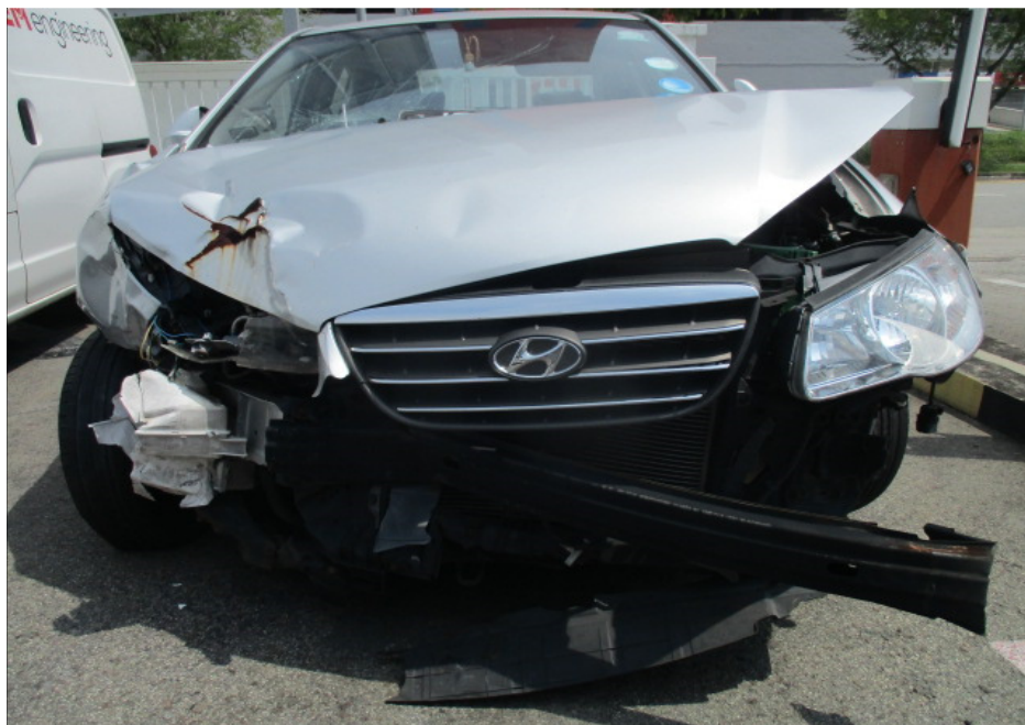
Photo 4 shows a general view of the front right portion of the Motor Car at the time of our inspection. The Motor Car was also observed to have sustained extensive impact damage at its frontal portal, damaged parts had included its front bonnet, front bumper, right fender, engine system, radiator and front right headlamp were amongst the body parts that were observed to have been damaged as a result of the accident.
