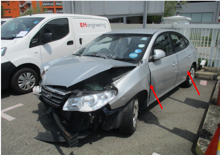
Photo 7 shows a general view of the front left portion of the Motor Car at the time of our inspection. The front left fender and the rear left body panel (arrowed) of the Motor Car was observed to have been damaged as a result of the accident.
