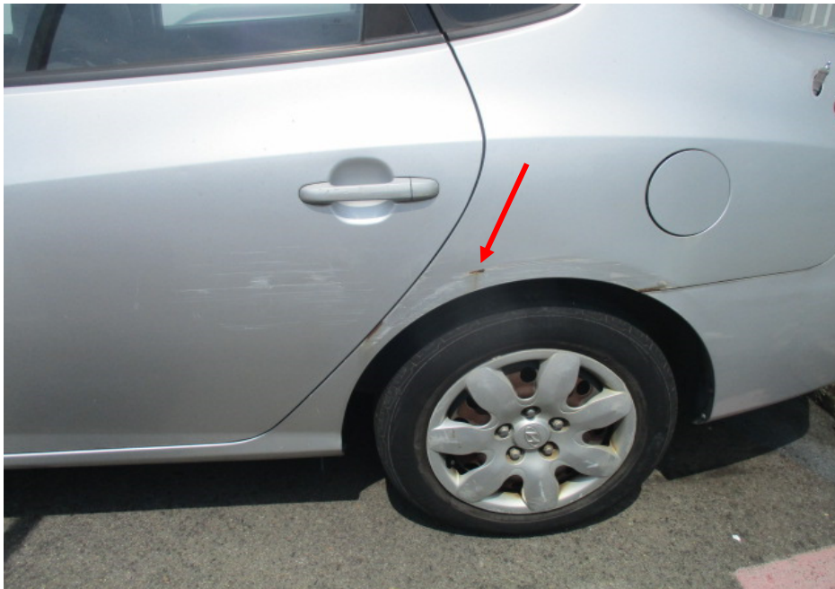
Photo 8 shows the close up view of the rear left panel portion of the Motor Car at the time of our inspection. The left rear body panel (arrowed) of the Motor Car was observed to have been damaged as a result of the accident.
