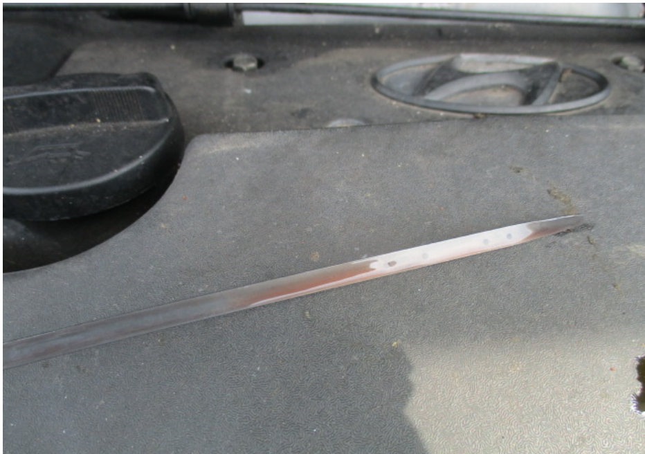
Photo 19 shows the ATF dip stick of the Motor Car at the time of our inspection. The ATF was observed to be of sufficient level for operational purposes and without any visible contamination.
