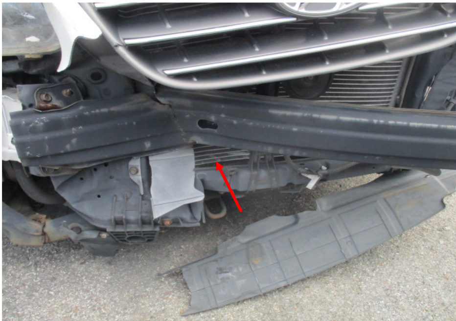
Photo 6 shows a close up view of the front portion of the Motor Car at the time of our inspection. The radiator of the Motor Car was observed to have been damaged by an induced impact as a result of the accident (arrowed).
