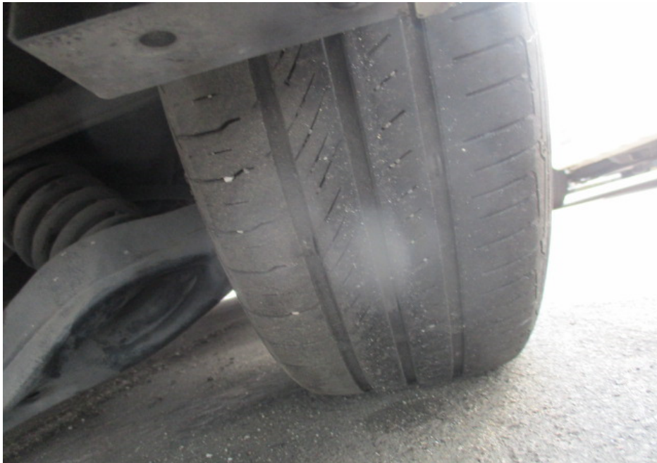
Photo 15 shows the condition of the rear right tyre of the Motor Car, which were observed to be in serviceable condition with remaining tread depth of approximately 7mm. There was also no tear, cut or burst mark(s) on the outer and the inner sidewalls as well as across the tread of the 4 tyres that were fitted on the Motor Car.
