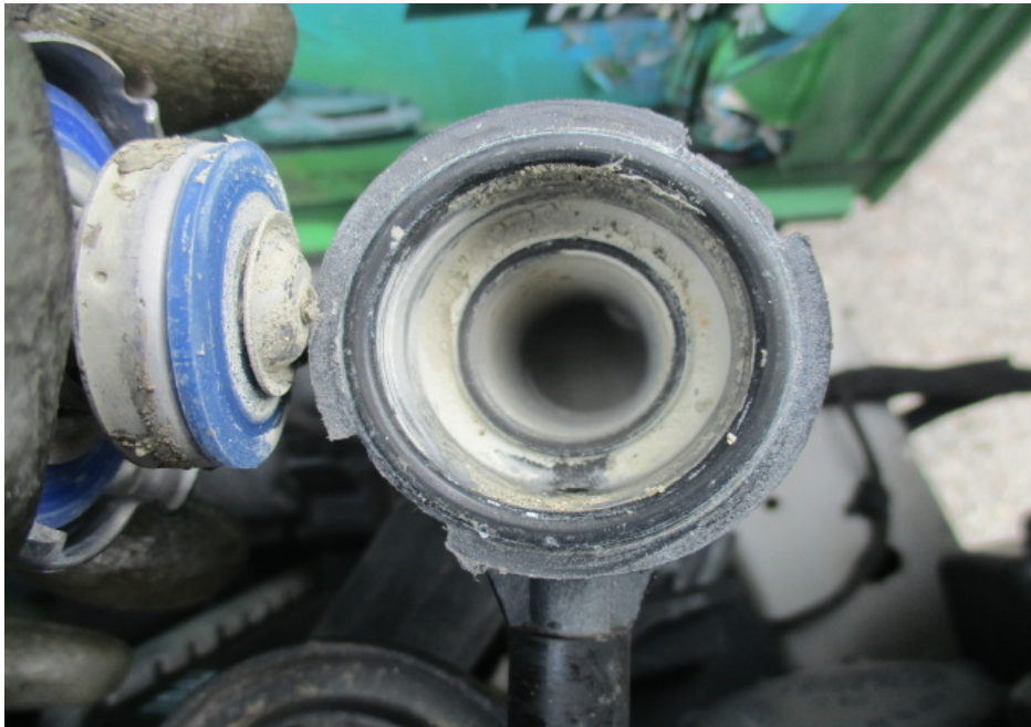
Photo 20 shows the radiator of the Motor Car at the time of our inspection. The radiator was observed to be empty most likely due to damages sustained as a result of the accident.
