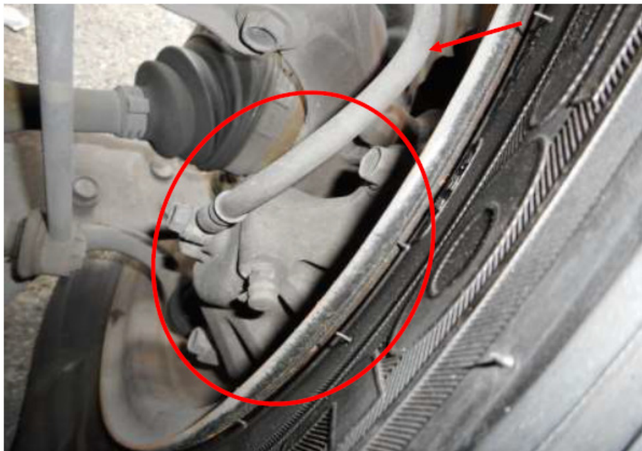
Photo 24 shows the brake hose (arrowed) at the front right wheel of the Motor Car. We did not observe any leakage of brake fluid at the 4 wheels of the Motor Car. Our visual inspection of the various mechanical components of the Motor Car's braking system, including its brake caliper (circled), revealed all to be intact and without visible damage.
