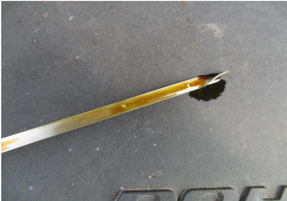
Photo 18 shows the engine oil dip stick of the Motor Car at the time of our inspection. The engine oil was observed to be of sufficient level for operational purposes and without any visible contamination.
