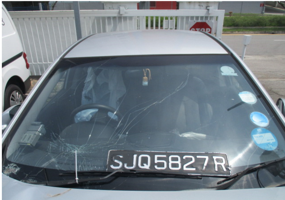
Photo 3 shows a close up view of the front windscreen of the Motor Car at the time of our inspection. The front windscreen of the Motor Car was observed to have been damaged as a result of the accident.
