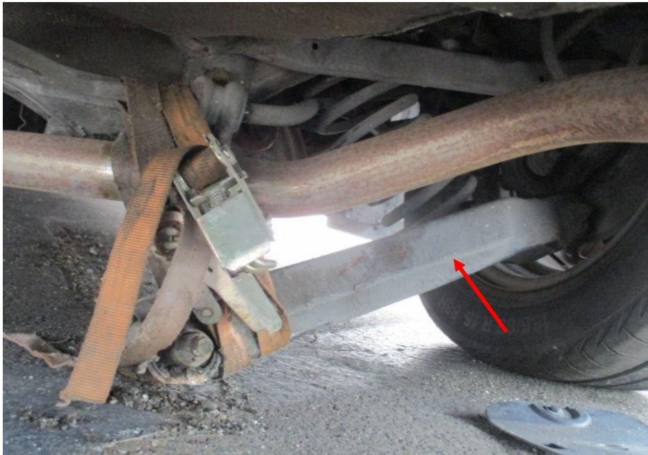
Photo 9 shows the close up view of the rear right suspension system of the Motor Car at the time of our inspection. The rear right lower arm (arrowed) of the Motor Car was observed to have been damaged as a result of the accident.
