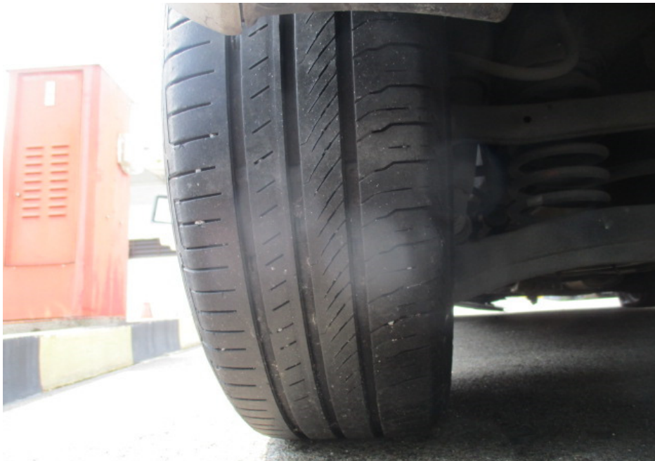
Photo 14 shows the condition of the rear left tyre of the Motor Car, which was observed to be in serviceable condition with remaining tread depth of approximately 5mm. There was no tear, cut or burst mark(s) on the outer and the inner sidewalls as well as across the tread of this tyre.
