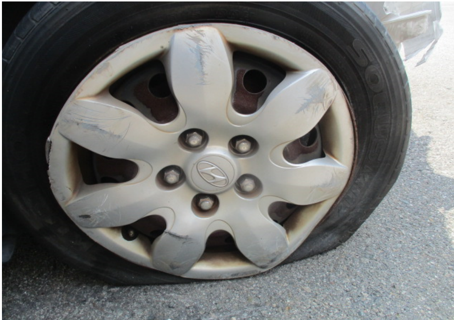
Photo 13 shows the condition of the front right wheel rim of the Motor Car, The right front tyre was observed to sustained damage, dislodged from the rim and deflated as a result of the accident.
