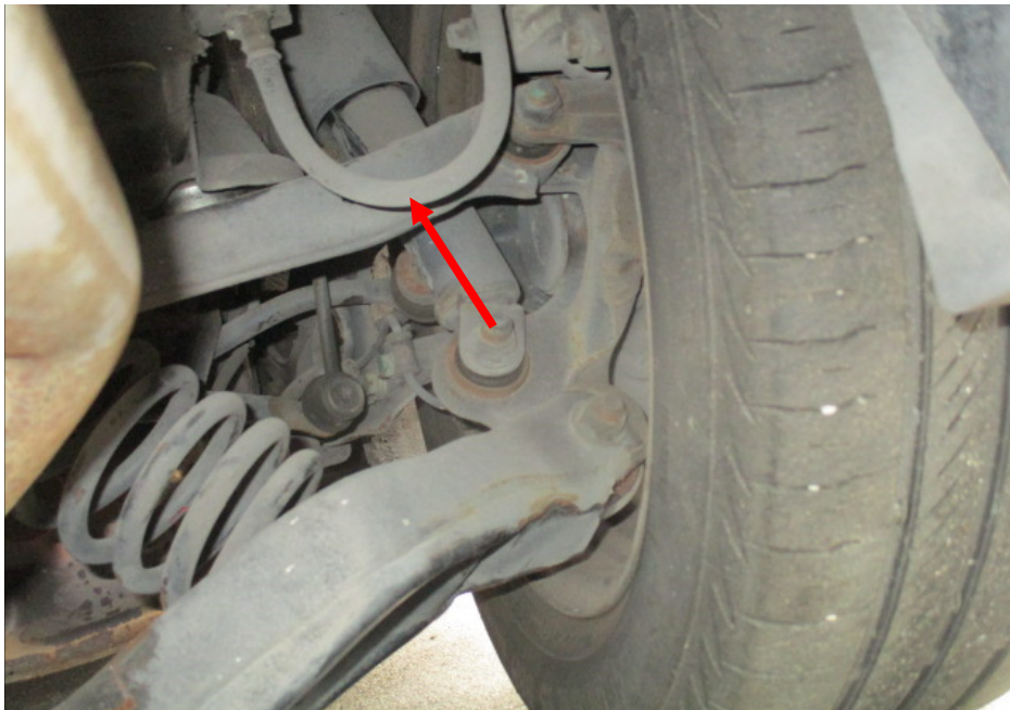
Photo 26 shows the various undercarriage components at the rear right wheel of the Motor Car, in particular the brake hose (arrowed). We did not observe any leakage of brake fluid at the 4 wheels of the Motor Car. Our visual inspection of the various mechanical components of the Motor Car's braking system revealed all to be intact and without visible damage.
