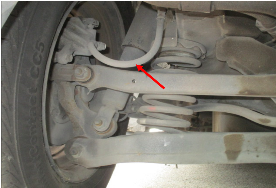
Photo 27 shows the various undercarriage components at the rear left wheel of the Motor Car, in particular the brake hose (arrowed). We did not observe any leakage of brake fluid at the 4 wheels of the Motor Car. Our visual inspection of the various mechanical components of the Motor Car's braking system revealed all to be intact and without visible damage.
