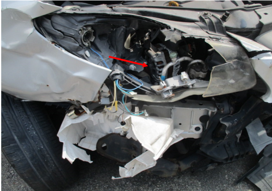
Photo 5 shows a close up view of the front portion of the Motor Car at the time of our inspection. The engine system (arrowed) of the Motor Car was observed to have been damaged as a result of the accident.
