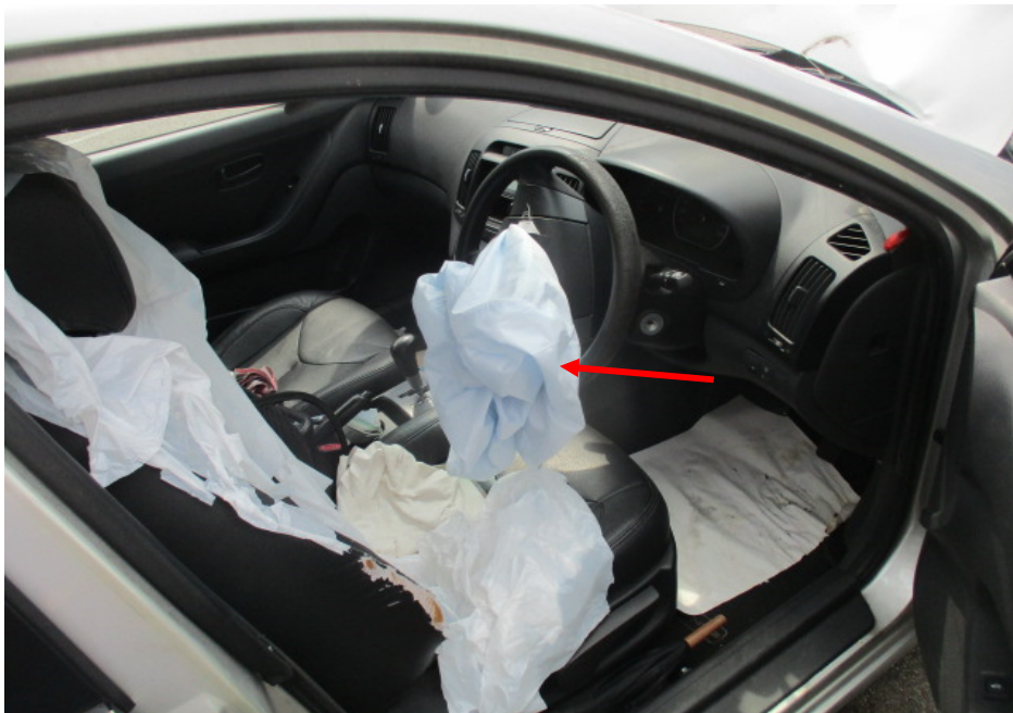
Photo 10 shows a general view of the Motor Car's interior compartment. The driver's air bag was also deployed as a result of the accident (arrowed).
