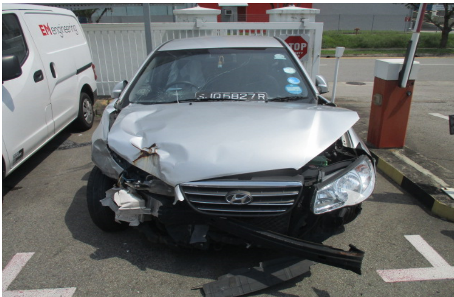
Photo 2 shows a general view of the front portion of the Motor Car at the time of our inspection. The Motor Car was also observed to have sustained extensive impact damage at its frontal and undercarriage portion.
