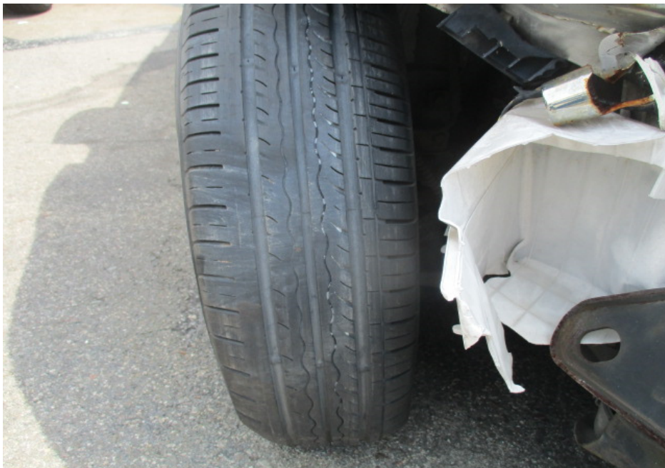
Photo 12 shows the condition of the front right tyre of the Motor Car, which was observed to be in serviceable condition with remaining tread depth of approximately 4mm. The tyre, which was wrapped around standard alloy wheel rim, was also observed to be deflated as a result of the accident.
