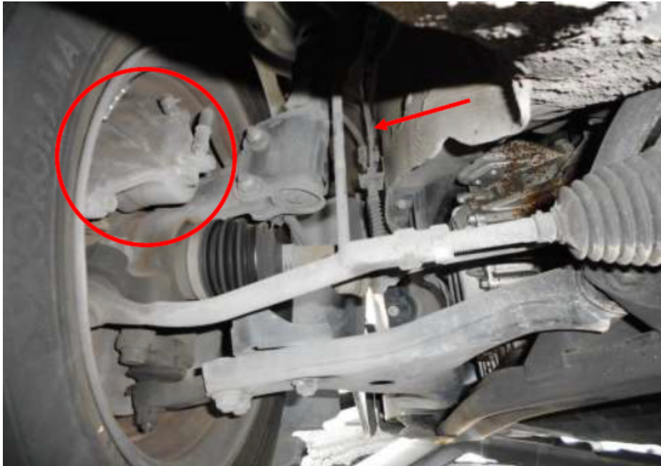
Photo 25 shows the brake hose (arrowed) at the front left wheel of the Motor Car. We did not observe any leakage of brake fluid at the 4 wheels of the Motor Car. Our visual inspection of the various mechanical components of the Motor Car's braking system, including its brake caliper (circled), revealed all to be intact and without visible damage.
