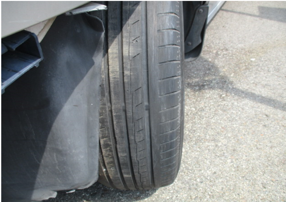
Photo 11 shows the condition of the front left tyre of the Motor Car, which was observed to be in serviceable condition with remaining tread depth of approximately 4mm. There was no tear, cut or burst mark(s) on the outer and the inner sidewalls as well as across the tread of this tyre.
