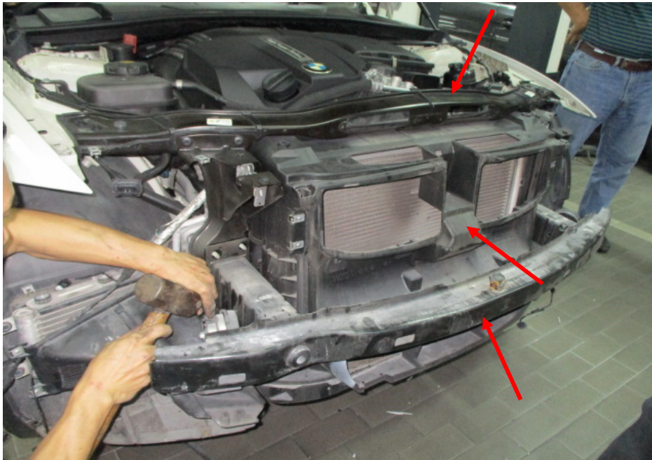
Photo 7 shows the Insured Vehicle during partial dismantling of the parts at its frontal portion on 20 January 2020. The front bumper reinforcement, radiator air guide and front support panel were amongst the parts (arrowed) that were found to be damaged.
