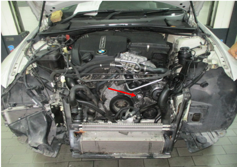
Photo 13 shows the Insured Vehicle during the re-inspection on 21 January 2020. The aircon condenser, radiator and radiator fan were dismantled and removed. The engine block of the Insured Vehicle, at the location where the idler pulley as mounted (arrowed), was observed to be broken/chipped off.
