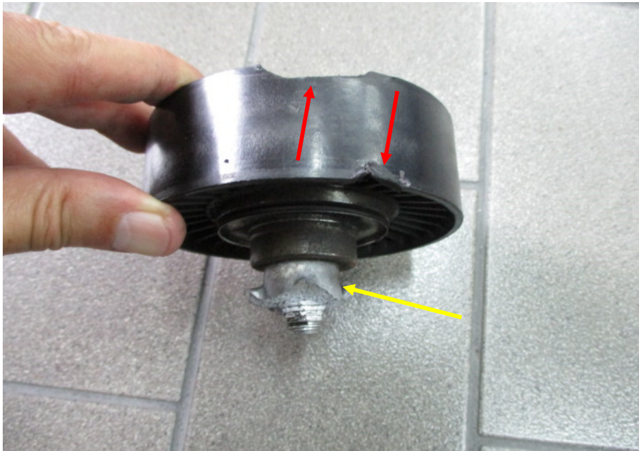
Photo 6 shows the rear side of the idler pulley of the Insured Vehicle. A section of the circumference edge was observed to be broken at both the front side and rear side (red arrow). The rear side of this idler pulley was mounted onto the engine housing of the Insured Vehicle and I had noted that a small part of the engine housing had chipped off (yellow arrow).
