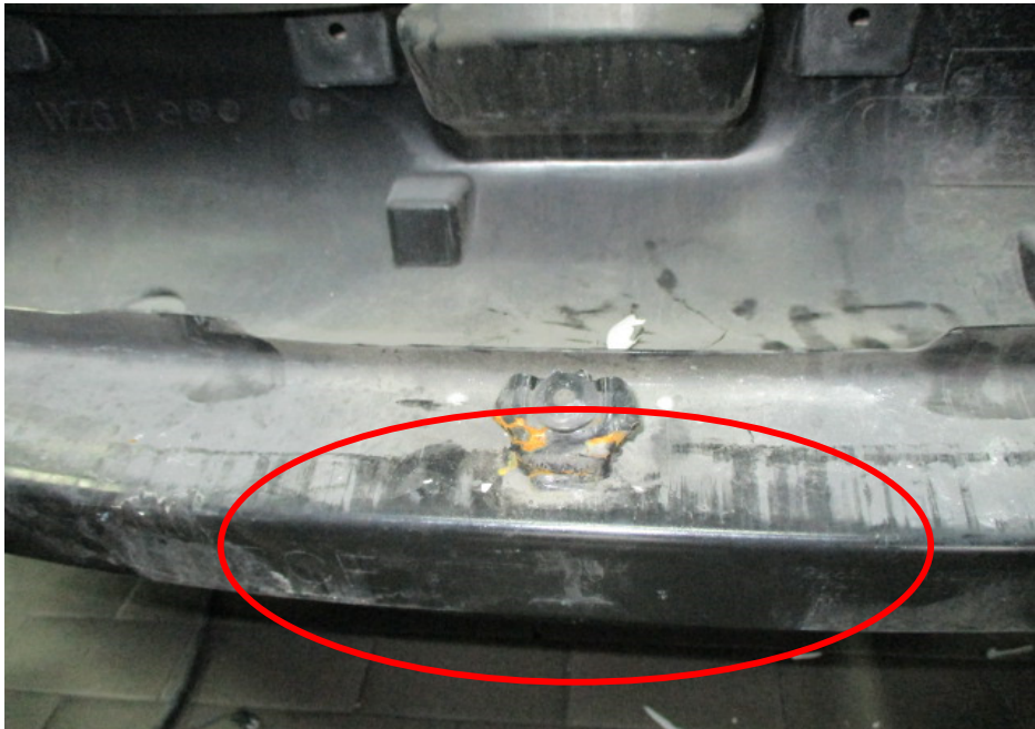
Photo 8 shows the front bumper reinforcement of the Insured Vehicle, which was observed to be dented (circled) at the centre. The indentation was inwards of the Insured Vehicle.
