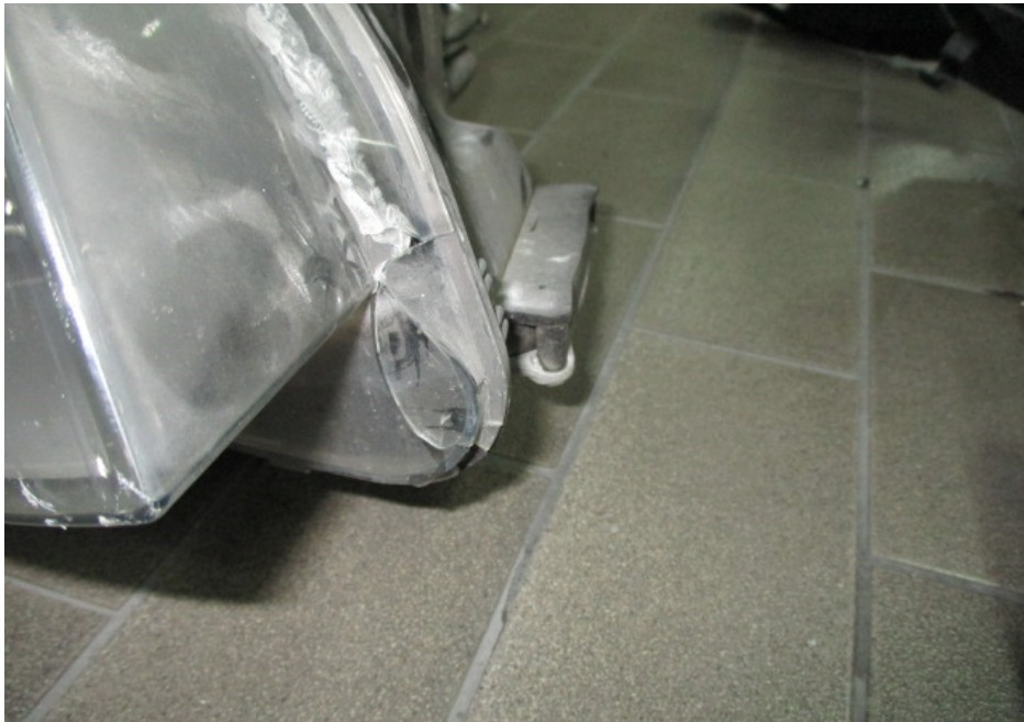
Photo 10 shows the front right headlamp of the Insured Vehicle, which was found to be cracked/broken at the corner edge. When fitted on the Insured Vehicle, this corner edge is located slightly towards the right from the centre of the Insured Vehicle.
