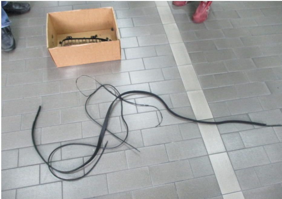
Photo 4 shows the drive belt of the Insured Vehicle, which was observed to be torn/shredded.
