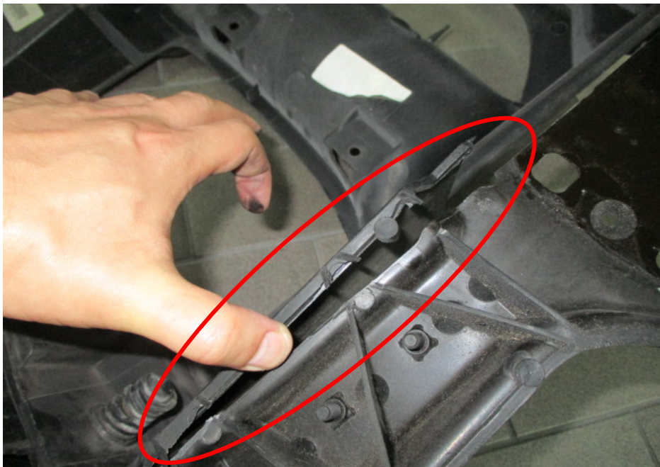
Photo 11 shows the front support panel of the Insured Vehicle, which was observed to be broken (circled). When fitted on the Insured Vehicle, this broken area is located slightly towards the left from the centre of the Insured Vehicle.
