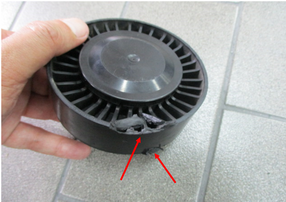
Photo 5 shows the front side of the idler pulley of the Insured Vehicle. A section of the circumference edge was observed to be broken at both the front side and rear side (arrowed).
