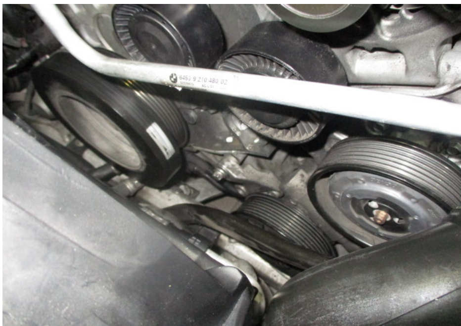
Photo 20 shows no contact between the drive belt system of the Insured vehicle and the parts directly in front.
