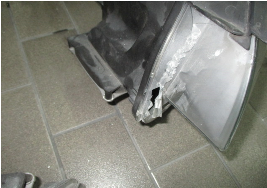
Photo 9 shows the front left headlamp of the Insured Vehicle, which was found to be cracked/broken at the corner edge. When fitted on the Insured Vehicle, this corner edge is located slightly towards the left from the centre of the Insured Vehicle.
