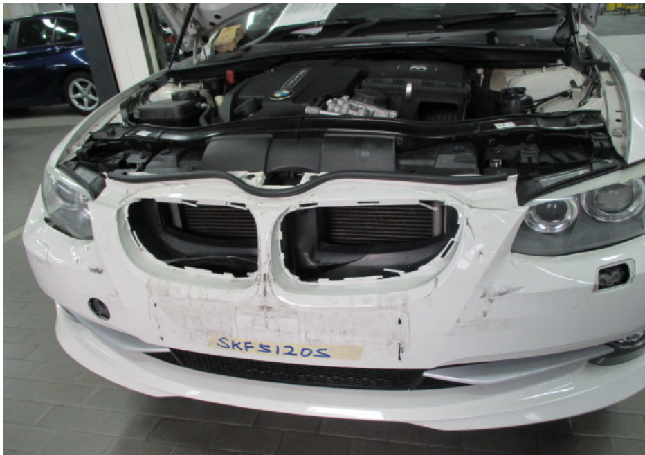
Photo 2 shows a closer view of the frontal portion of the Insured Vehicle. The front bumper, front grilles, front bonnet and front number plate were amongst the exterior body parts that were found to be with visible damage.
