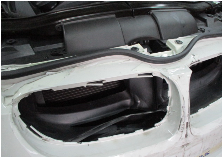
Photo 3 shows another view of the frontal portion of the Insured Vehicle. The front bumper, front grilles, front bonnet and front number plate were amongst the exterior body parts that were found to be with visible damage.
