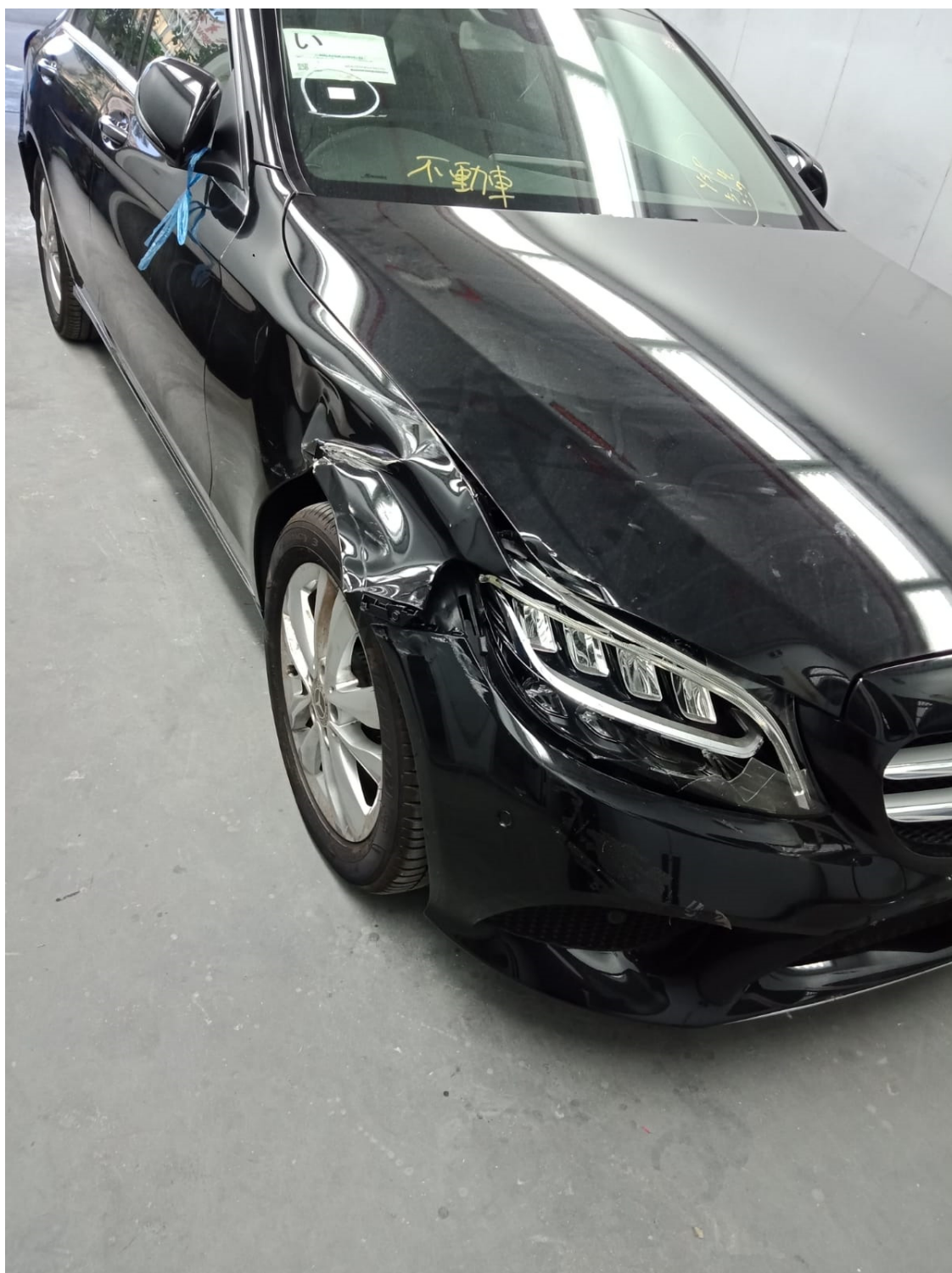
Photo 1 shows the front right body of the Motor Car prior to any repairs being carried out (photograph provided to me). The Motor Car had sustained damages at its front right portion and rear portion. For the front right portion, the body parts observed to be damaged include its front bumper, front right headlamp, front bonnet and front right fender amongst others. The airbags of the Motor Car were not activated, as seen from the photographs that were provided to me.
