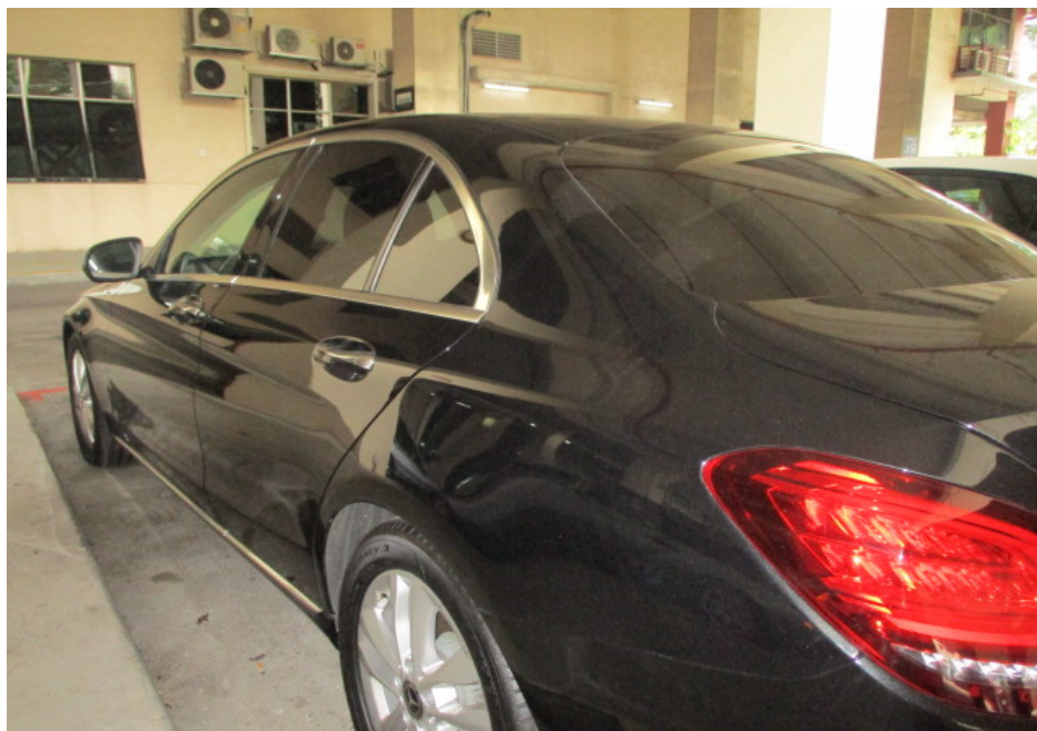
Photo 10 shows the rear left fender and rear left taillamp of the Motor Car at the time of my inspection. The body parts at the rear portion of the Motor Car were visually examined and it was observed that the repair/restoration works carried out to the damaged area of the Motor Car (refer to photograph 1 & 2 above) were reasonably adequate and in order.
