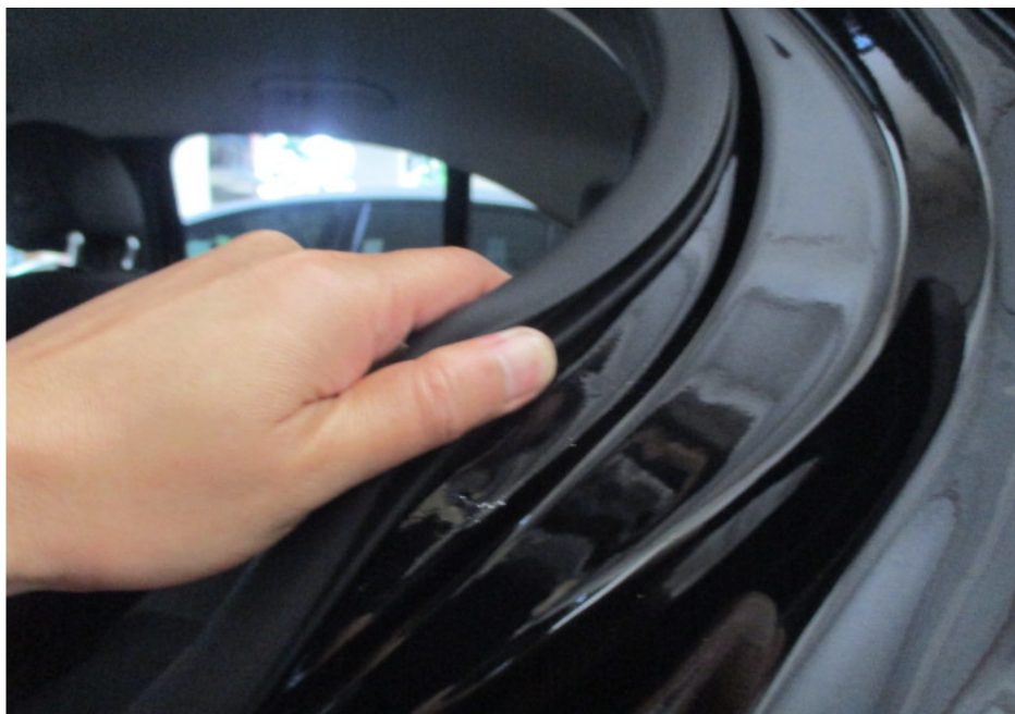
Photo 25 shows the left side "C" pillar of the Motor Car. I did not find any original weld marks at the left side "C" pillar of the Motor Car, indicating that the rear left fender of the Motor Car was replaced. The lack of original weld marks seen was due to replacement work when the replaced rear left fender was re-welded onto the Motor Car and smoothen for re-spraying work.
