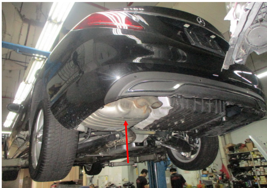
Photo 20 shows the Motor Car's rear muffler (arrowed). My examination of the Motor Car's exhaust system revealed no sign(s) or indication(s) of any cut or weld marks along its exhaust pipes and on its catalytic convertor.
