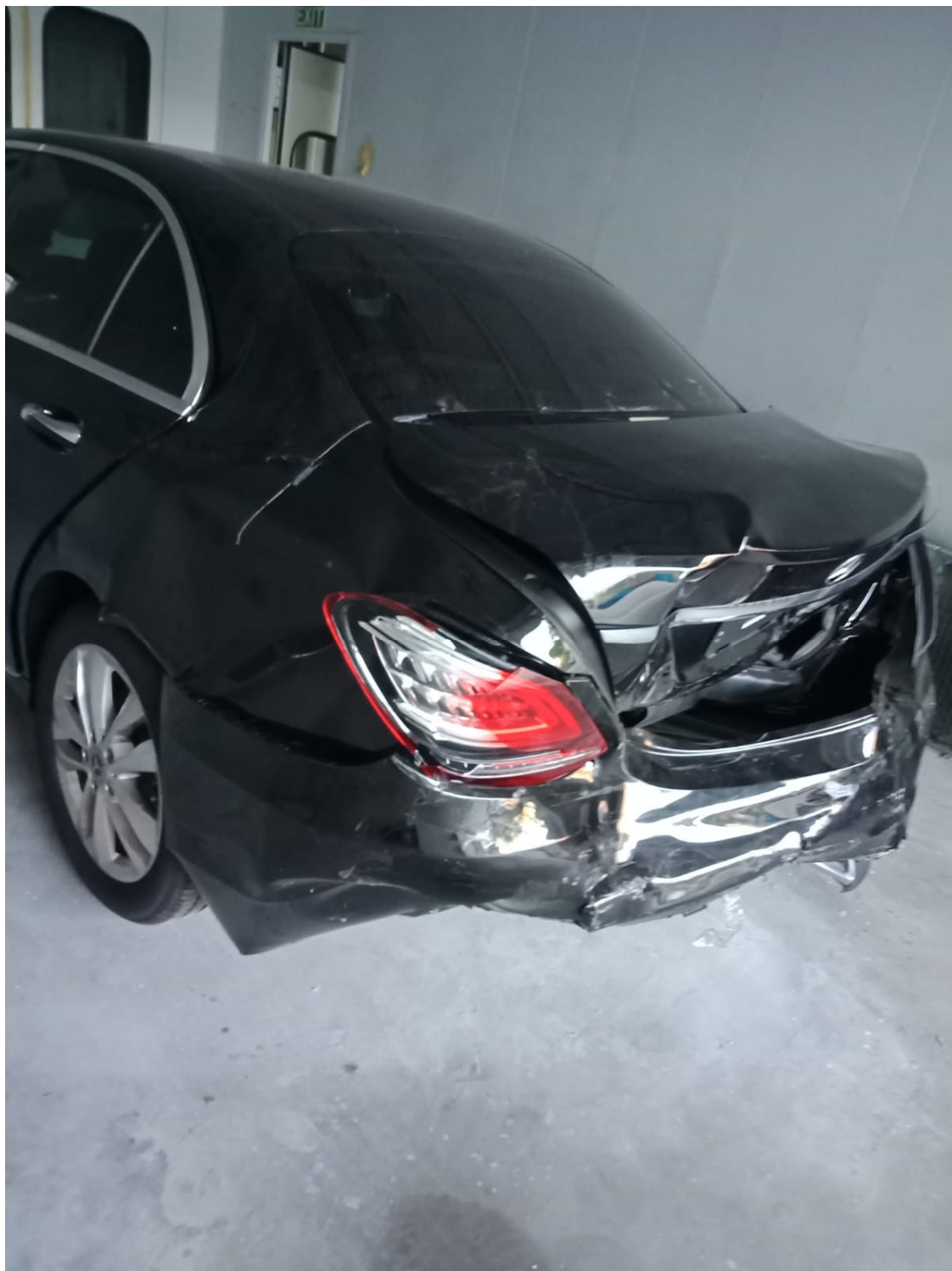
Photo 3 shows the rear left portion of the Motor Car prior to any repairs being carried out (photograph provided to me). Apart for the front right portion, the Motor Car had also sustained damage at its rear portion. The body parts observed to be damaged at the rear portion include the rear bumper, rear bootlid, rear left taillamp and rear left fender amongst others.
