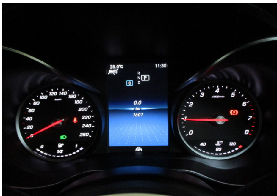
Photo 15 shows the respective warning lights no longer illuminated, indicating that there is no fault detected to the ABS, SRS, EPS and TCS lights systems of the Motor Car during the self-test. These electronic systems were hence in working condition at the time of my inspection.
