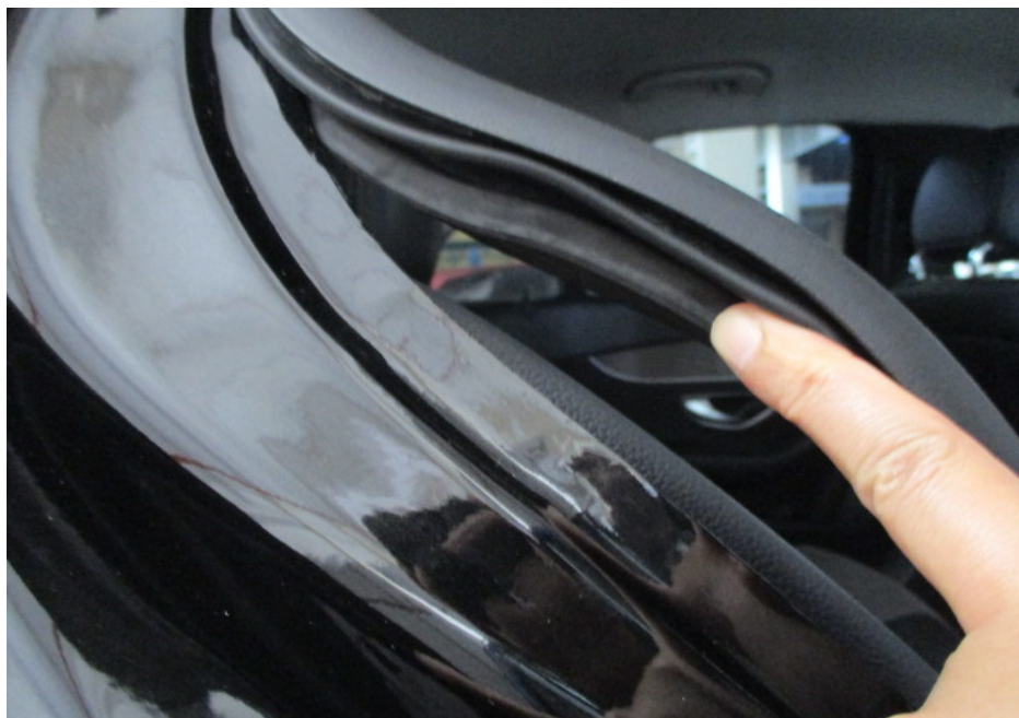
Photo 26 shows the right side "C" pillar of the Motor Car. I did not find any original weld marks at the right side "C" pillar of the Motor Car, indicating that the rear right fender of the Motor Car was replaced. The lack of original weld marks seen was due to replacement work when the replaced rear right fender was re-welded onto the Motor Car and smoothen for re-spraying work.
