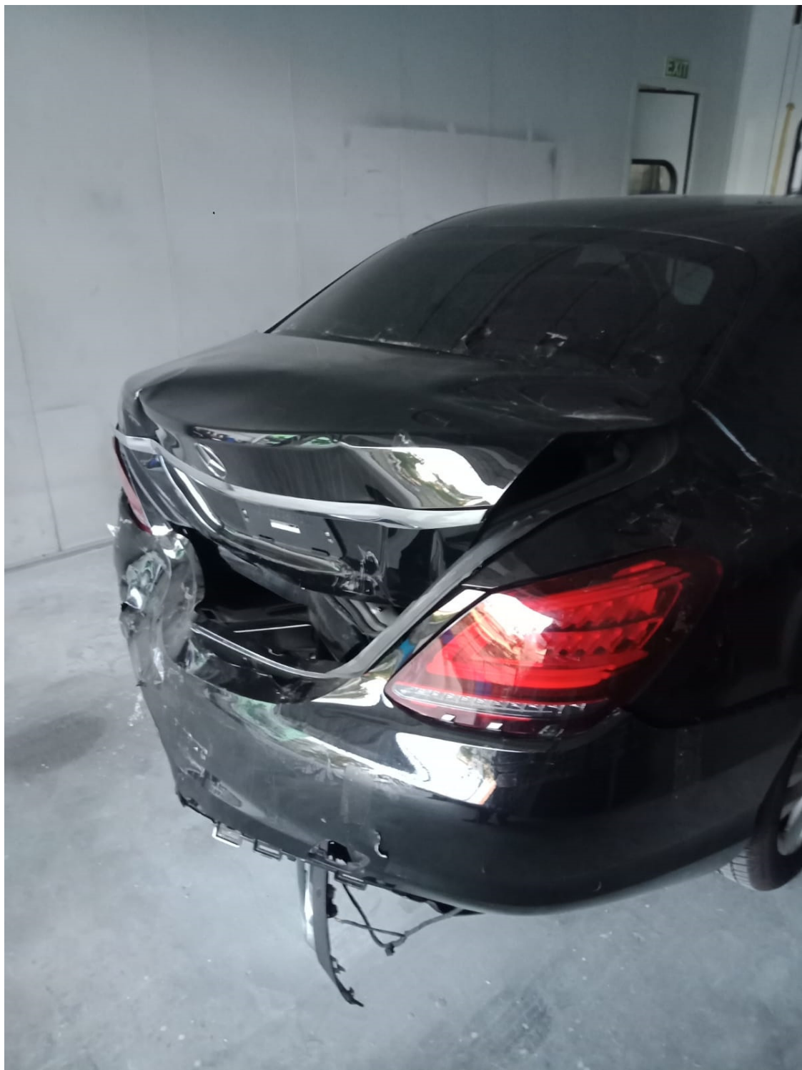
Photo 2 shows the rear right portion of the Motor Car prior to any repairs being carried out (photograph provided to me). Apart for the front right portion, the Motor Car had also sustained damage at its rear portion. The body parts observed to be damaged at the rear portion include the rear bumper, rear bootlid, rear bootlid chrome moulding and rear exhaust muffler amongst others.
