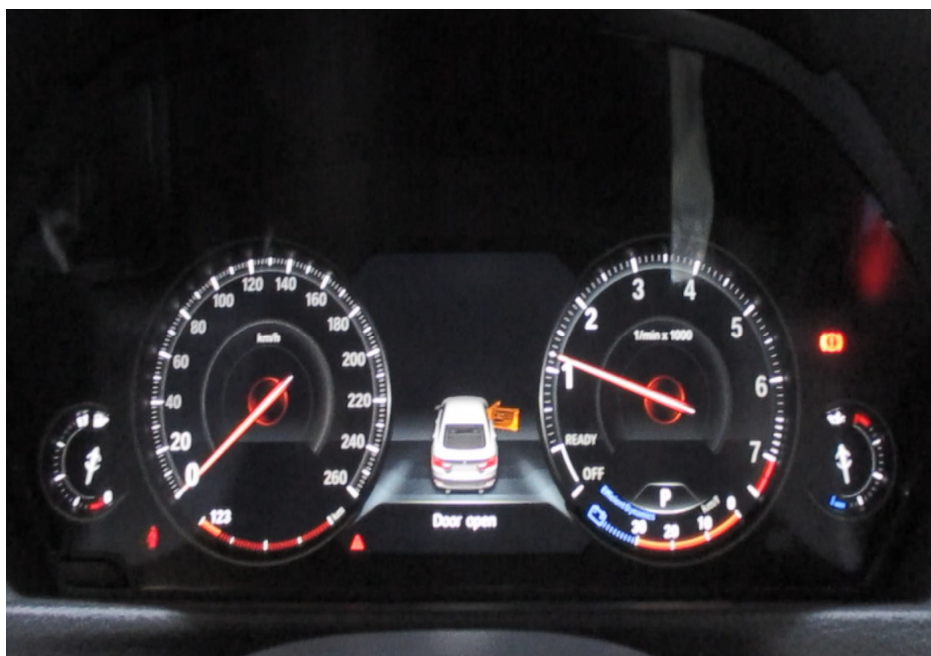
Photo 12 shows the respective warning lights no longer illuminated, indicating that there is no fault detected to the ABS, SRS, IAS, TPM and DSC systems of the Motor Car during the self-test. These electronic systems were hence in working condition at the time of my inspection.
