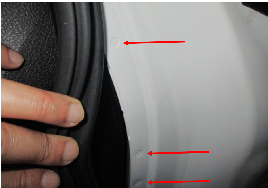
Photo 20 shows the right side "A" pillar of the Motor Car. I did not find any weld marks other than original spot weld marks (arrowed) on the non-detachable body panels of the Motor Car, indicating that there was no re-welding works carried out; and that the non-detachable body panels of the Motor Car were originally fitted.
