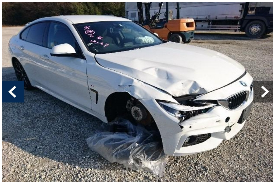
Photo 1 shows the front right body of the Motor Car prior to any repairs being carried out (photograph provided to me). The Motor Car was observed to have sustained damages at its front right portion. The body parts observed to be damaged had include its front bumper, front right headlamp, front bonnet and front right fender amongst others. The front right wheel rim and front right tyre were observed to be missing, as seen from the photographs that were provided to me.
