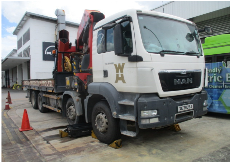
Photo 3 shows the right side view of the Insured Vehicle at the time of our inspection. The fire damage to the Insured Vehicle was confined to its interior compartment. The right body was observed to have been unaffected by the fire.
