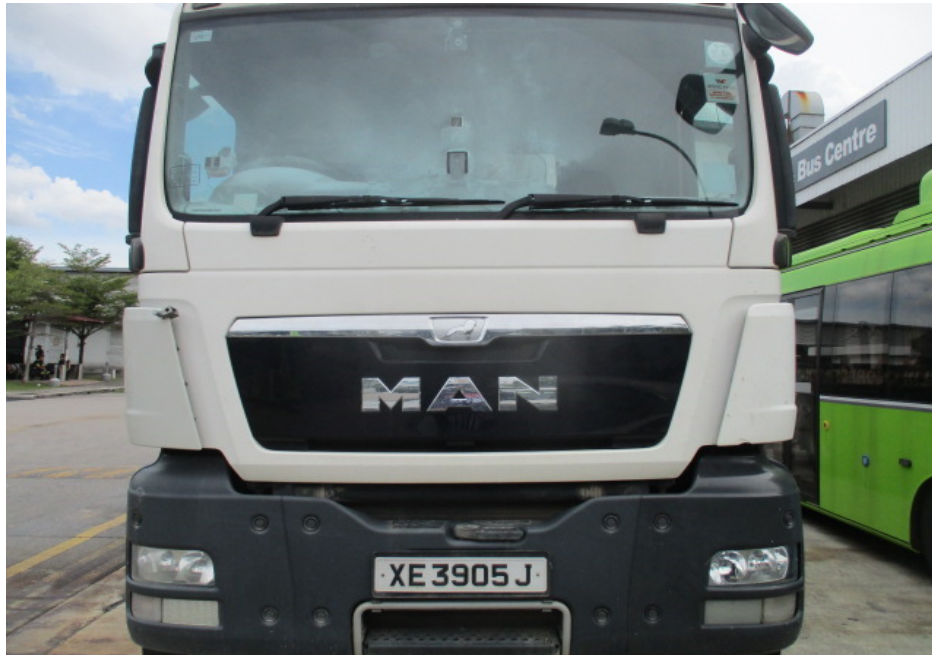
Photo 1 shows the front view of the Insured Vehicle at the time of our inspection. The fire damage to the Insured Vehicle was confined to its interior compartment. Most parts of the front portion were unaffected by the fire except for the front windscreen.
