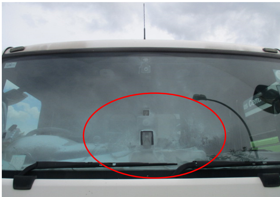
Photo 2 shows the general view of the front windscreen of the Insured Vehicle. The centre portion of the windscreen seemed to have sustained visible fire damage (circled).
