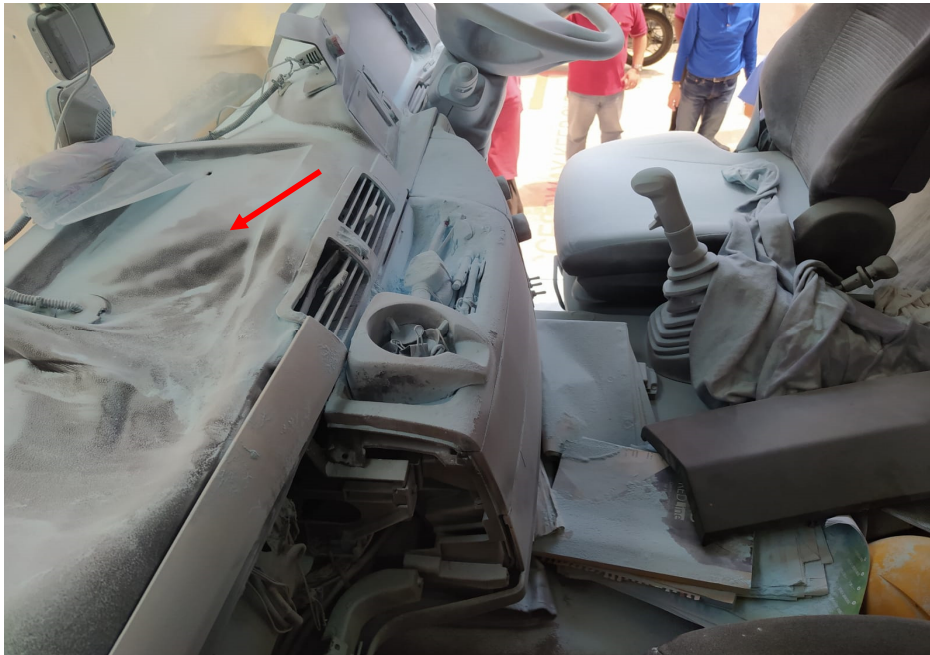
Photo 14 shows interior compartment of the Insured Vehicle at the incident scene after the fire was put out. Generally, the information that could be gathered from the incident scene photographs provided by Mr Yong had corresponded to the events that he had related to us, which is the fire had started from the centre portion of the dashboard of the Insured Vehicle (arrowed)
