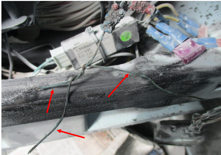
Photo 10 shows greenish residue on some wirings leading to a component that belonged to the mobile crane of the Insured Vehicle (arrowed). The presence of such greenish residue suggests occurrence of an electrical short circuit.
