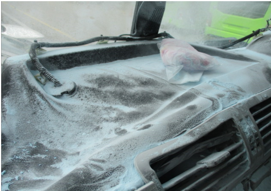
Photo 7 shows the centre of the dashboard of the Insured Vehicle. The fire seemed to have originated from the centre portion of the instrument panel basing on the area where the extent of fire damage was most severe. Various components of the instrument panel were observed to have been burnt and/or partly melted from prolonged exposure to high heat intensity which included the upper and central parts of the instrument panel assembly, air outlet assembly, beaker holder assembly and carrier assembly, amongst others.
