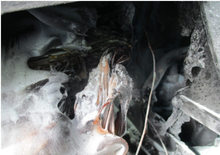
Photo 9 shows a close up view of the centre portion of the instrument panel. Most of the components of the instrument panel were observed to have been burnt and/or partly melted from prolonged exposure to high heat intensity.
