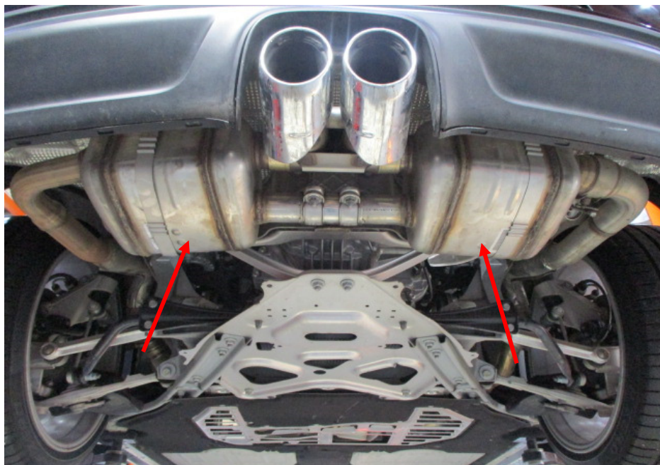
Photo 19 shows the Motor Car's rear mufflers (arrowed). My examination of the Motor Car's exhaust system revealed no sign(s) or indication(s) of any cut or weld marks along its exhaust pipes and on its catalytic converters.
