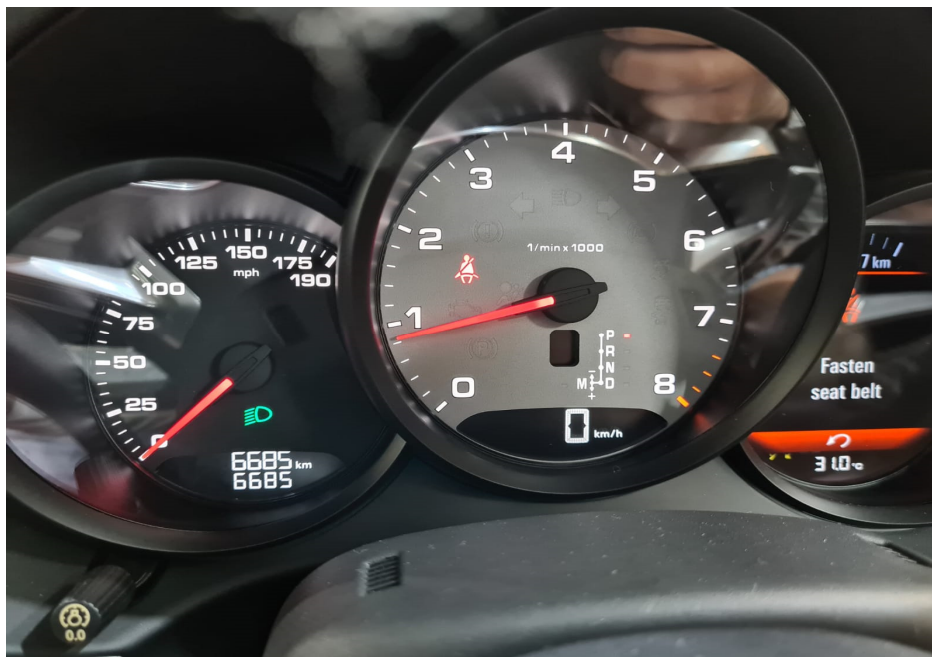
Photo 13 shows the respective warning lights no longer illuminated, indicating that there is no fault detected to the ABS, SRS, TPM and TCS systems of the Motor Car during the self-test. These electronic systems were hence in working condition at the time of my inspection.
