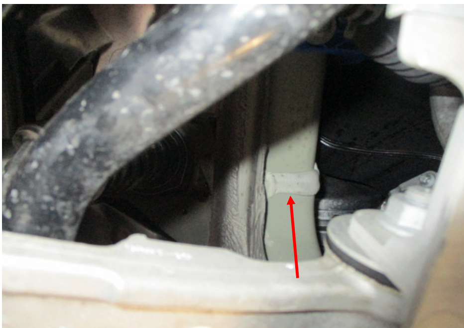
Photo 22 shows the chassis/structural body at the underside front right of the Motor Car. The original factory sealant (arrowed) at the joints along the chassis/structural body was observed to be untouched, indicating no work was done on the chassis/structural body of the Motor Car and that the chassis/structural body was originally fitted.
