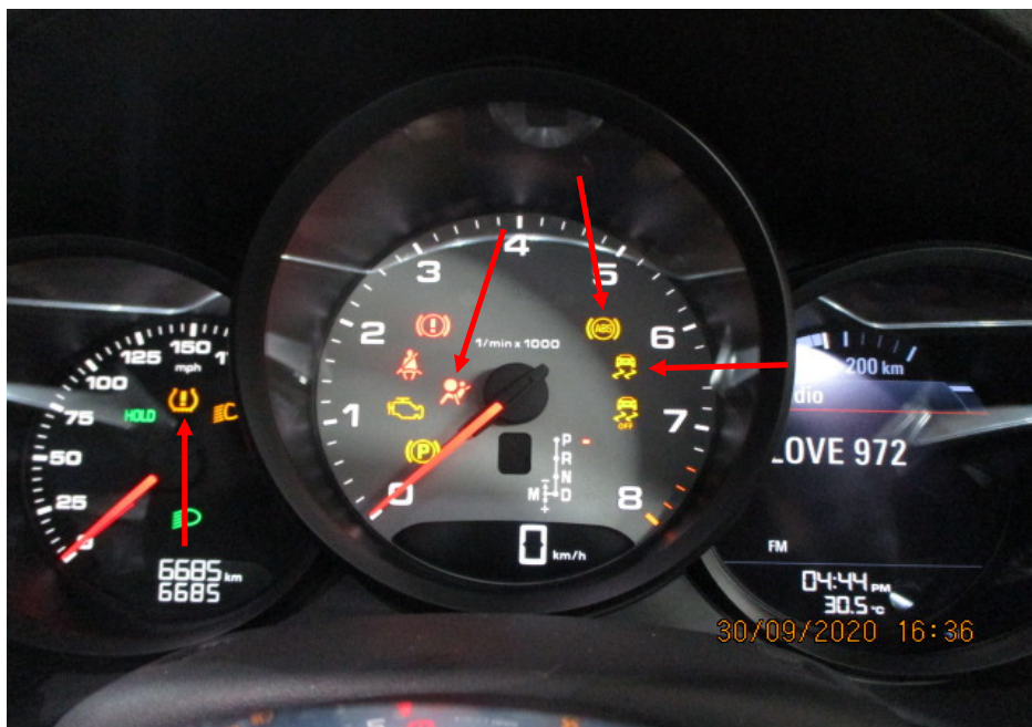
Photo 12 shows the warning lights for the various electronic safety features appearing on the instrument panel of the Motor Car during its self-test when the engine is cranked, in particular the ABS, SRS, TPM and TCS lights (arrowed).
