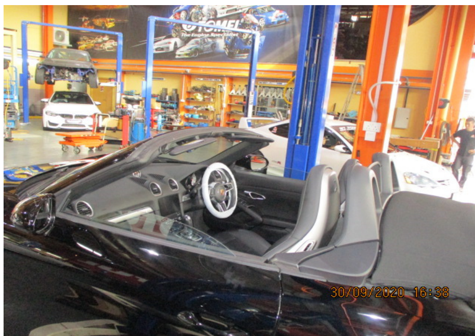
Photo 9 shows the Motor Car with its soft top roof folded. During my inspection of the Motor Car, I had tested the soft top roof and it was observed that the soft top roof was able to fold and unfold without any difficulty. It was also observed that during the folding and unfolding process, the soft top roof did not extend laterally beyond the Motor Car's body. In general, the soft top roof of the Motor Car was found to be in a normal working condition.
