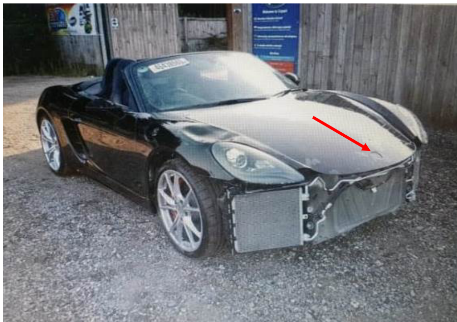
Photo 1 shows the front right body of the Motor Car (photograph provided to me). There appears to be no visible damage observed to the Motor Car as seen from the photographs that were provided to me. I had however observed that the Motor Car's front bumper and its related attachments were dislodged/missing. The front bonnet emblem (arrowed) was also missing.
