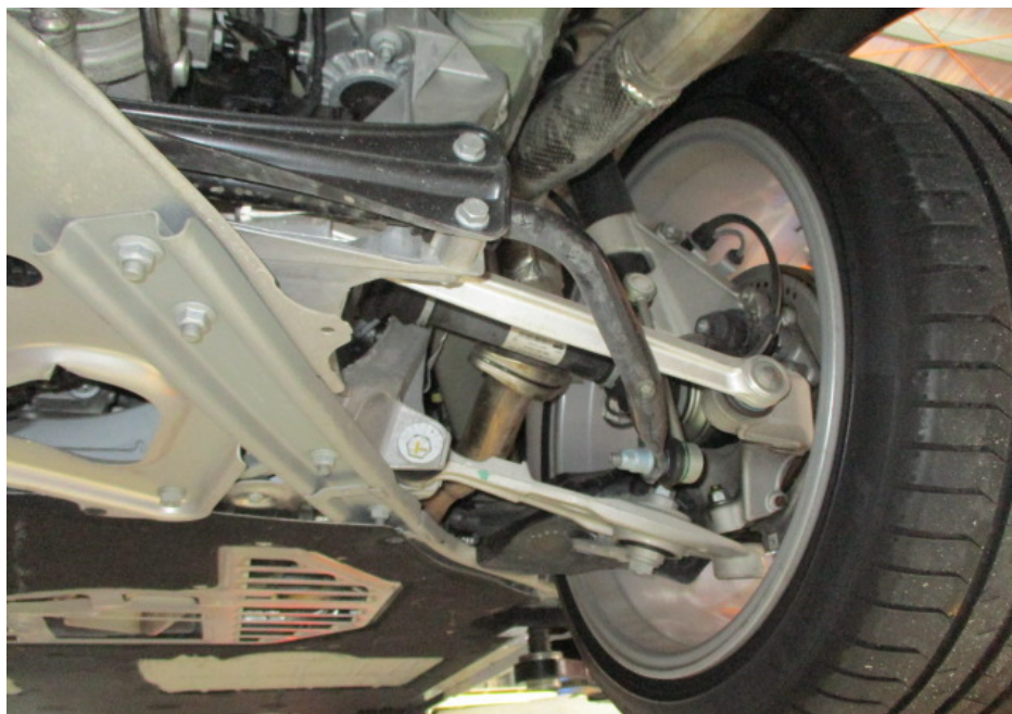
Photo 15 shows a general view of the control arms and linkages at the rear right wheel of the Motor Car. I did not observe any fluid leak and/or fluid stain on the underside of the Motor Car. All the Motor Car's undercarriage components were observed to be intact and secured in an appropriate manner.
