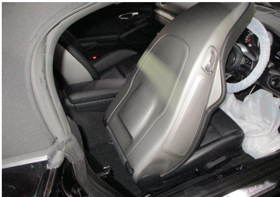
Photo 11 shows the seats of the Motor Car, which were secured via seat rails to the floorboard. All the seats of the Motor Car were fitted with a retractable seat belt reel and pre-tensioner. The seat belts were tested and able to be fastened into the respective pre-tensions that were fitted on the side of each individual seat.
