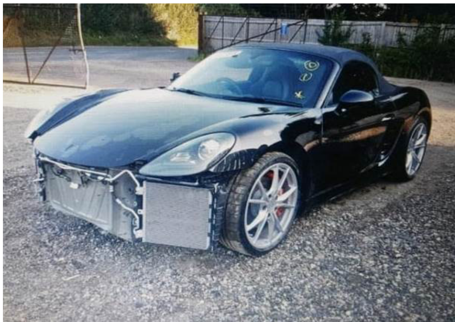
Photo 2 shows the front left body of the Motor Car (photograph provided to me). There appears to be no visible damage observed to the Motor Car as seen from the photographs that were provided to me. I had however observed that the Motor Car's front bumper and its related attachments were dislodged/missing.
