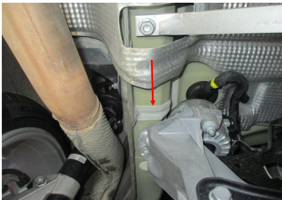
Photo 20 shows the chassis/structural body at the underside rear left of the Motor Car. The original factory sealant (arrowed) at the joints along the chassis/structural body was observed to be untouched, indicating no work was done on the chassis/structural body of the Motor Car and that the chassis/structural body was originally fitted.
