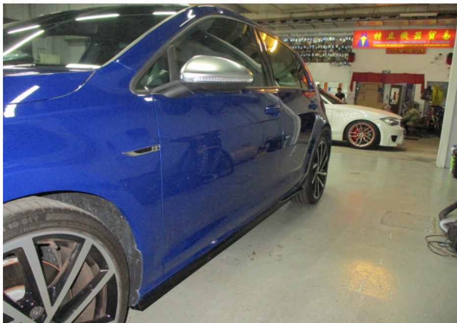
Photo 5 shows the front left fender, front left door and left side rocker panel garnish of the Motor Car at the time of my inspection. The body parts at the left body of the Motor Car were visually examined and it was observed that the repair/restoration works carried out to the damaged area of the Motor Car (refer photograph 1 & 2 above) were reasonably adequate and in order.
