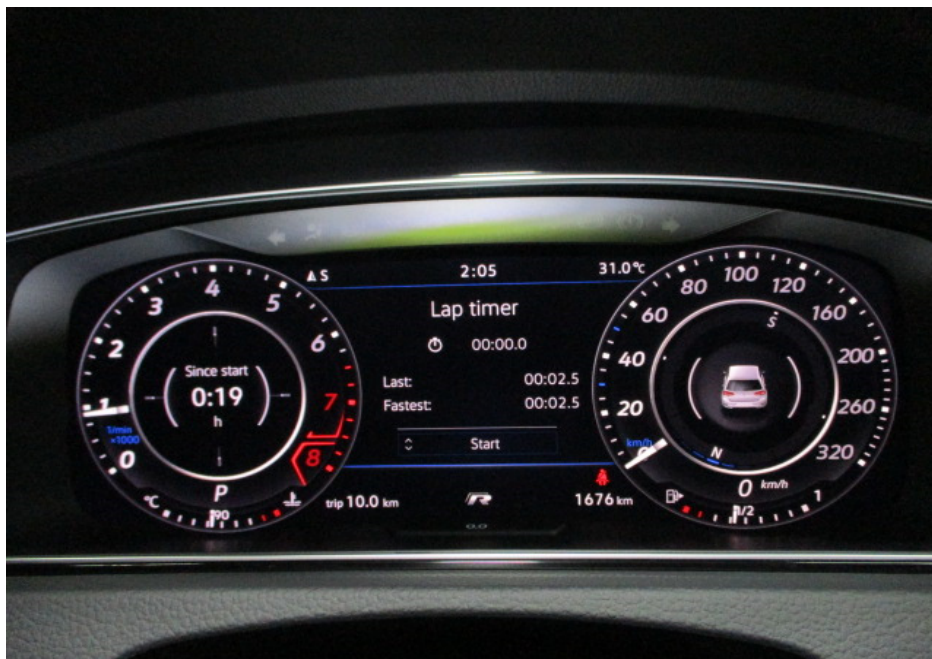
Photo 12 shows the respective warning lights no longer illuminated, indicating that there is no fault detected to the ABS, SRS, EPS, ESP and TPM systems of the Motor Car during the self-test. These electronic systems were hence in working condition at the time of my inspection.
