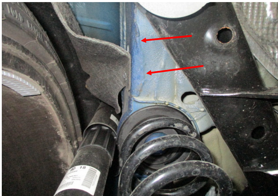
Photo 19 shows the chassis/structural body at the underside rear left of the Motor Car. The original factory sealant (arrowed) at the joints along the chassis/structural body was untouched, indicating no work was done on the chassis/structural body of the Motor Car and that the chassis/structural body was originally fitted.
