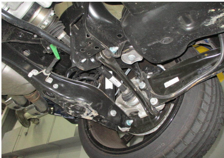
Photo 14 shows a general view of the control arms and linkages at the rear left wheel of the Motor Car. I did not observe any fluid leak and/or fluid stain on the underside of the Motor Car. All of the Motor Car's undercarriage components were observed to be intact and secured in an appropriate manner.
