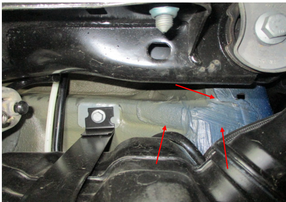
Photo 20 shows the floorboard at the underside rear of the Motor Car. The original factory sealant (arrowed) at the joints along the non-detachable body panels were untouched, indicating no work was done on the non-detachable body panels of the Motor Car; and that these body panels were originally fitted.
