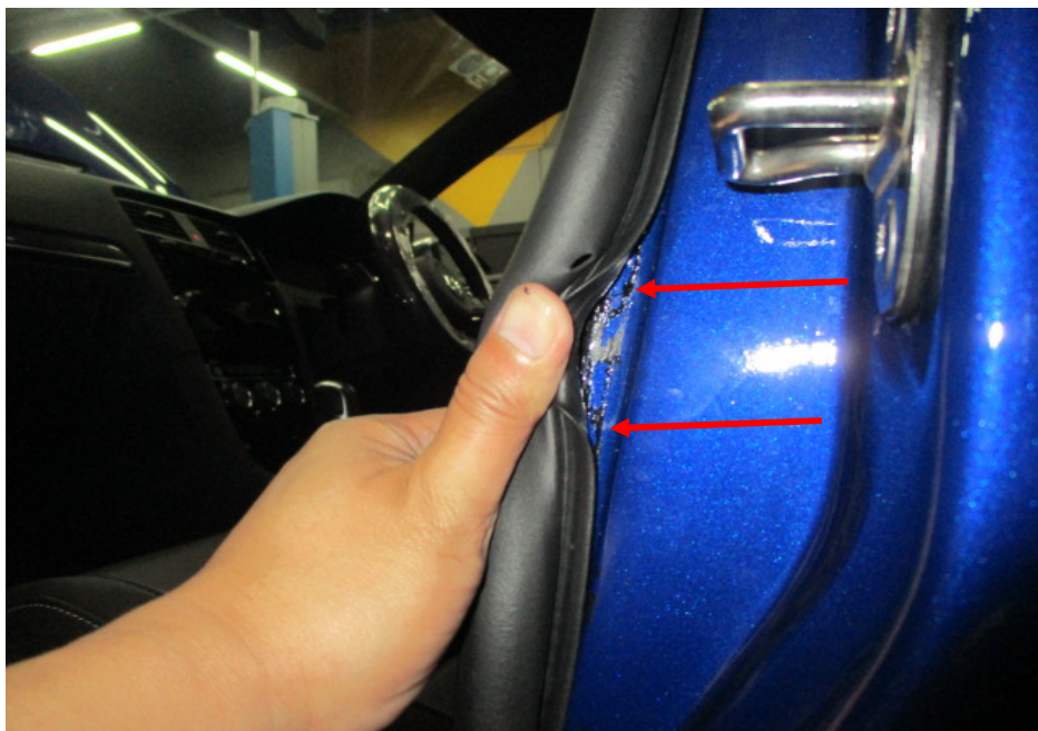
Photo 21 shows the left side "B" pillar of the Motor Car. The original rubber gum (arrowed) was seen at the left side "B" pillar when the front left door weatherstrip was pulled aside, indicating that the left side "B" pillar was originally fitted. In general, I had found the non-detachable body panels of the Motor Car to be originally fitted at the time of my inspection.
