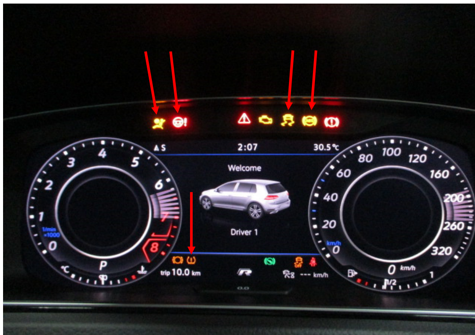
Photo 11 shows the warning lights for the various electronic safety features appearing on the instrument panel of the Motor Car during its self-test when the engine is cranked, in particular the ABS, SRS, EPS, ESP and TPM lights (arrowed).
