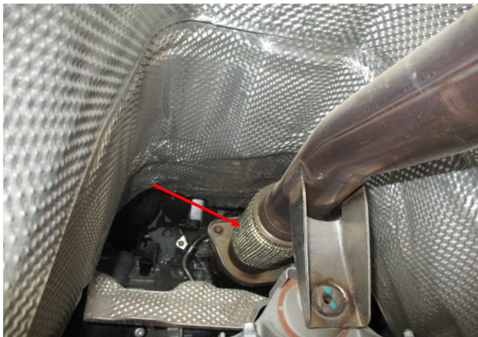
Photo 17 shows the Motor Car's catalytic converter (arrowed). My examination of the Motor Car's exhaust system revealed no sign(s) or indication(s) of any cut or weld marks along its exhaust pipes and on its rear muffler.
