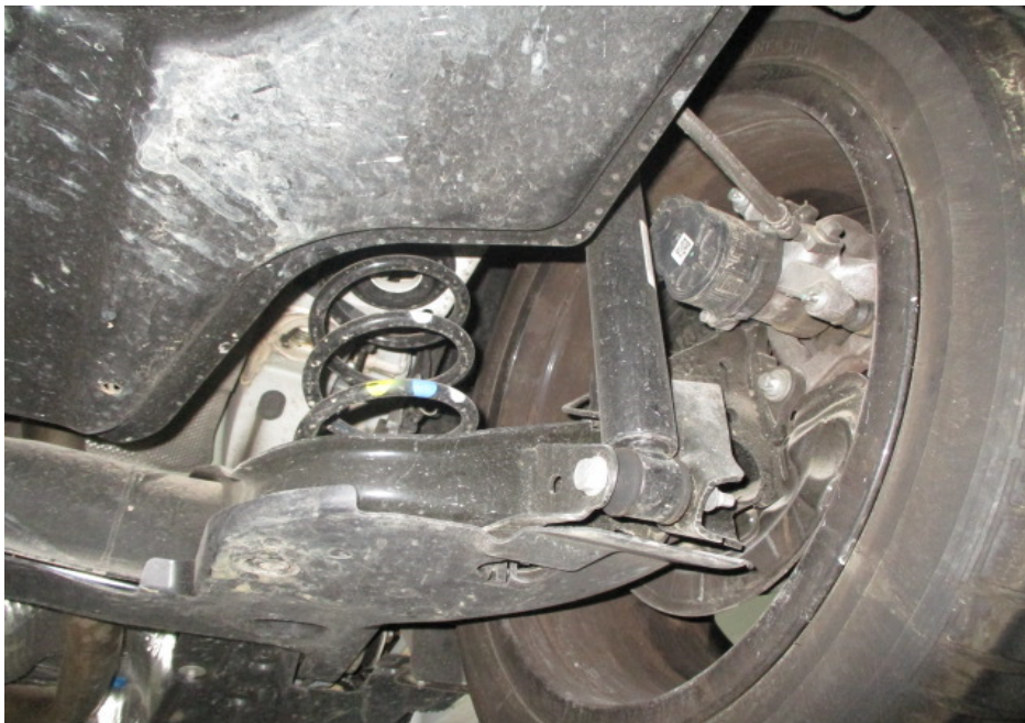
Photo 14 shows a general view of the control arms and linkages at the rear right wheel of the Motor Car. I did not observe any fluid leak and/or fluid stain on the underside of the Motor Car. All the Motor Car's undercarriage components were observed to be intact and secured in an appropriate manner.
