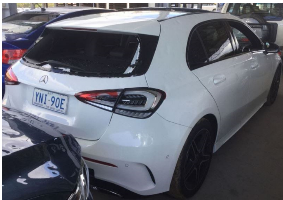
Photo 2 shows the rear right body of the Motor Car prior to any repairs being carried out (photograph provided to me). Relatively minor indentation damage was seen on the rear right fender and other exterior body parts of the Motor Car. The rear right taillamps were also observed to be broken.
