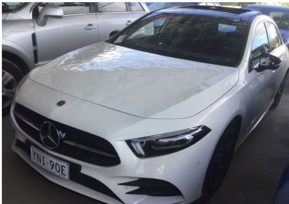
Photo 1 shows the front left body of the Motor Car prior to any repairs being carried out (photograph provided to me). The Motor Car was observed to have sustained damages of indentation nature to multiple exterior body parts like its front bumper and front bonnet. As seen from the photographs provided, the indentation was relatively minor. The panoramic sunroof glass was also observed to be broken.
