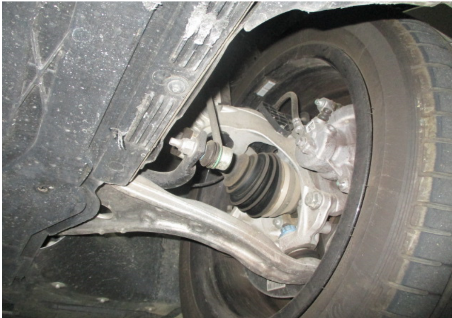
Photo 15 shows the various undercarriage components at the front left wheel of the Motor Car. The mechanical components, control arms and linkages were all found to be intact and secured in an appropriate manner.
