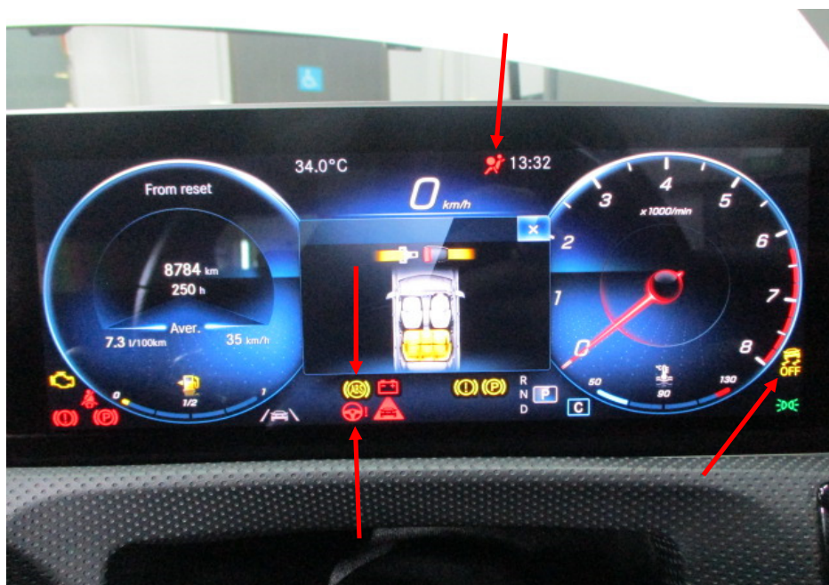
Photo 11 shows the warning lights for the various electronic safety features appearing on the instrument panel of the Motor Car during its self-test when the engine is cranked, in particular the ABS, SRS, EPS and ESP lights (arrowed).
