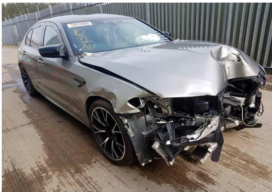
Photo 2 shows the front right body of the Motor Car prior to any repairs being carried out (photograph provided to me). The Motor Car was observed to have sustained damages at its frontal portion. The body parts observed to be damaged had included the front bumper, front bonnet, front right headlamp and front right fender amongst others.
