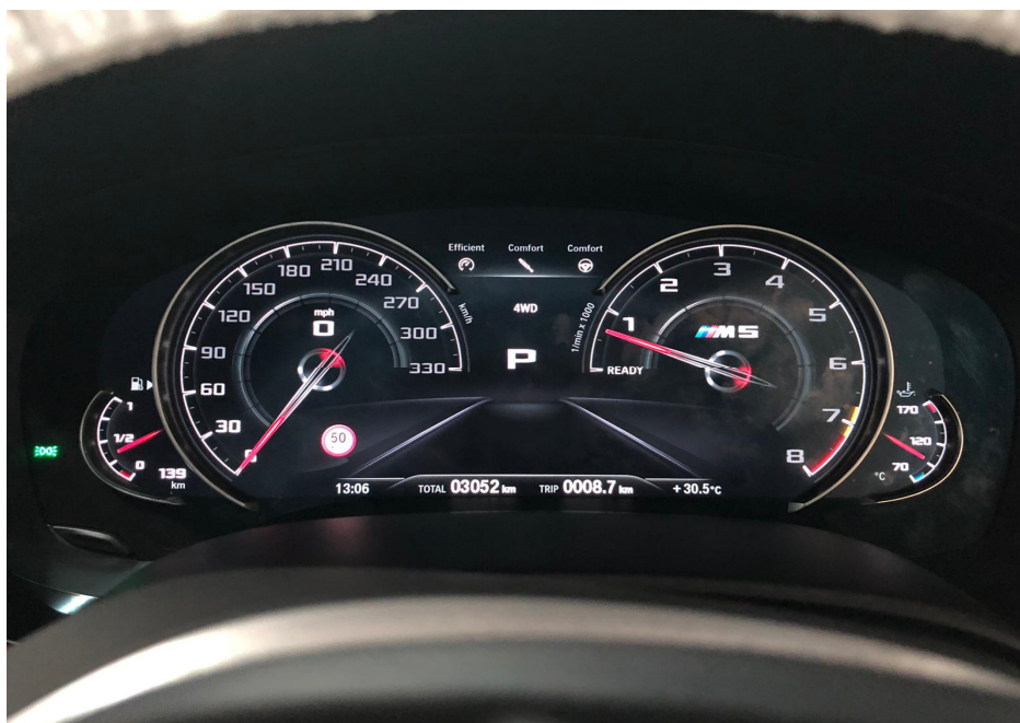
Photo 12 shows the respective warning lights no longer illuminated after the engine was started, indicating that there was no fault detected to the ABS, SRS, IAS, TPM and DSC systems of the Motor Car during the self-test. These electronic systems were hence in working condition at the time of my inspection.
