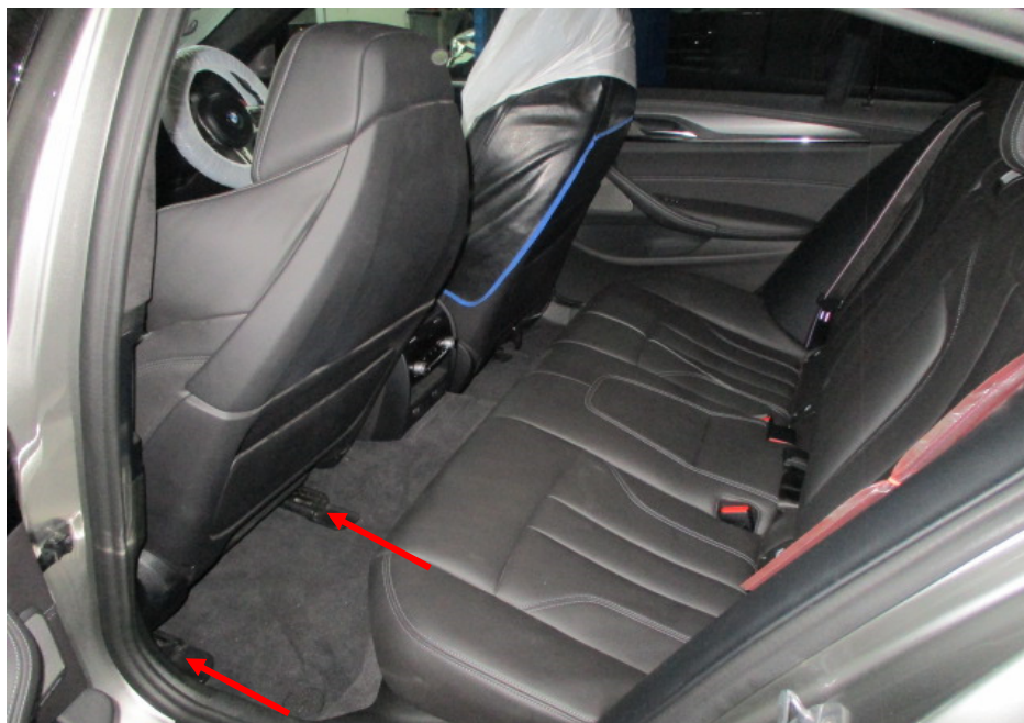
Photo 10 shows the seats of the Motor Car, which were secured via seat rails (arrowed) to the floorboard. All the seats of the Motor Car were fitted with a retractable seat belt reel and pre-tensioner. The seat belt reels were tested and were able to be fastened securely into the respective pre-tensioners that were fixed to the side of all the seats.
