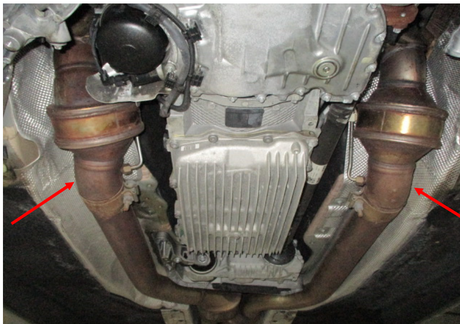
Photo 17 shows the Motor Car's 2 exhaust downpipes (arrowed) from the exhaust manifold to the rear mufflers. My examination of the Motor Car's exhaust system revealed no sign(s) or indication(s) of any cut or weld marks along its exhaust pipes and on its rear mufflers.
