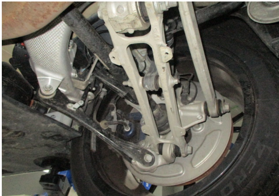
Photo 14 shows a general view of the control arms and linkages at the rear right wheel of the Motor Car. I did not observe any fluid leak and/or fluid stain on the underside of the Motor Car. All of the Motor Car's undercarriage components were observed to be intact and secured in an appropriate manner.
