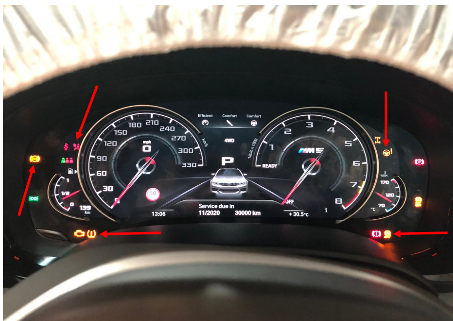
Photo 11 shows the warning lights for the various electronic safety features appearing on the instrument panel of the Motor Car during its self-test when the engine is cranked, in particular the ABS, SRS, IAS, TPM and DSC lights (arrowed).
