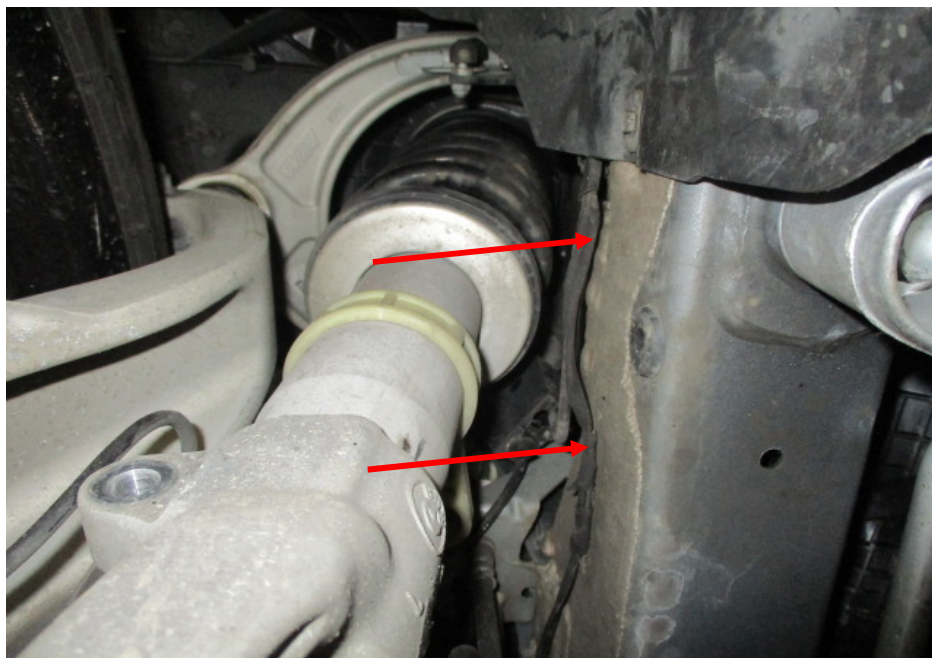
Photo 18 shows the chassis/structural body at the underside front left of the Motor Car. I did not find any weld marks other than original spot weld marks on the chassis/structural body of the Motor Car. The original factory sealant (arrowed) at the joints along the chassis/structural body was also untouched, indicating no work was done on the chassis/structural body of the Motor Car and that the chassis/structural body was originally fitted.
