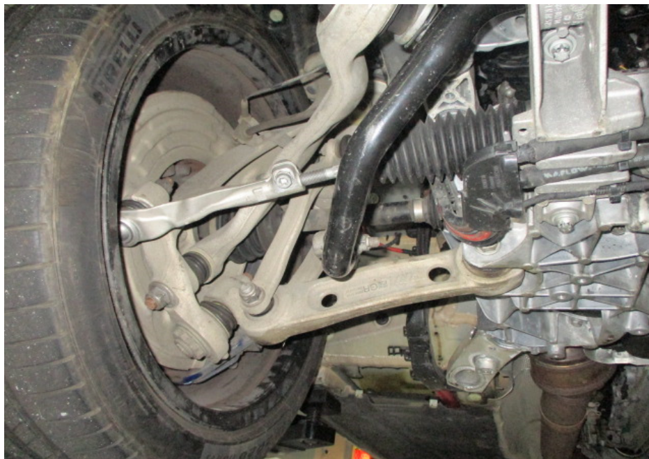
Photo 16 shows the various undercarriage components at the front right wheel of the Motor Car. I did not observe any fluid leak and/or fluid stain on the underside of the Motor Car. All of the Motor Car's undercarriage components were observed to be intact and secured in an appropriate manner.
