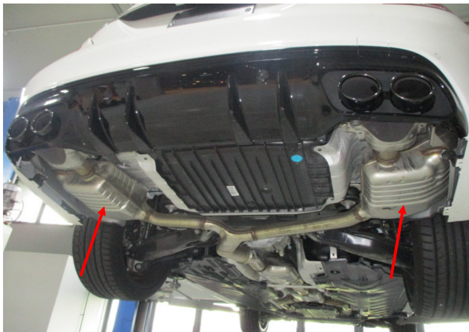
Photo 18 shows the Motor Car's rear mufflers (arrowed). My examination of the Motor Car's exhaust system revealed no sign(s) or indication(s) of any cut or weld marks along its exhaust pipes and on its catalytic converters.
