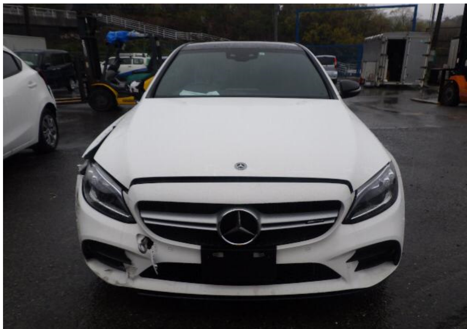
Photo 1 shows the frontal portion of the Motor Car prior to any repairs being carried out (photograph provided to me). The Motor Car was observed to have sustained damages at its front right portion. Body parts observed to have been damaged include its front bumper and front right fender.
