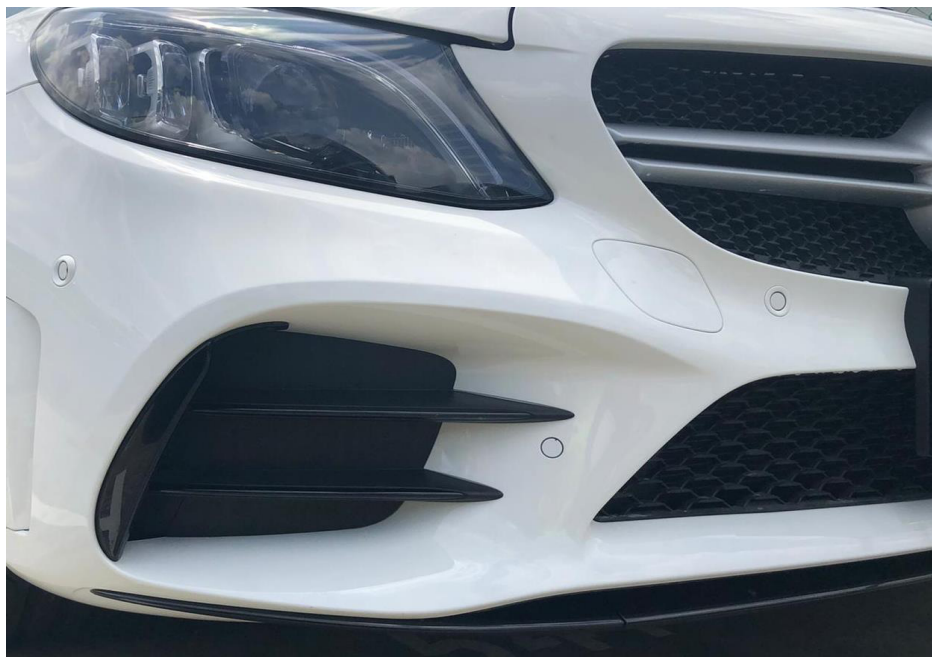
Photo 5 shows a closer view of the front right portion of the Motor Car. The body parts at the front right portion of the Motor Car were visually examined and it was observed that the repair/restoration works carried out to the damaged area of the Motor Car (refer photograph 1 above) were reasonably adequate and in order
