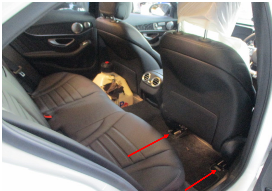
Photo 11 shows the seats of the Motor Car, which were secured via seat rails (arrowed) to the floorboard. All the seats of the Motor Car were fitted with a retractable seat belt reel and pre-tensioner. The seat belt reels were tested and able to be fastened into the respective pre-tensions that were fitted on the side of each individual seat.
