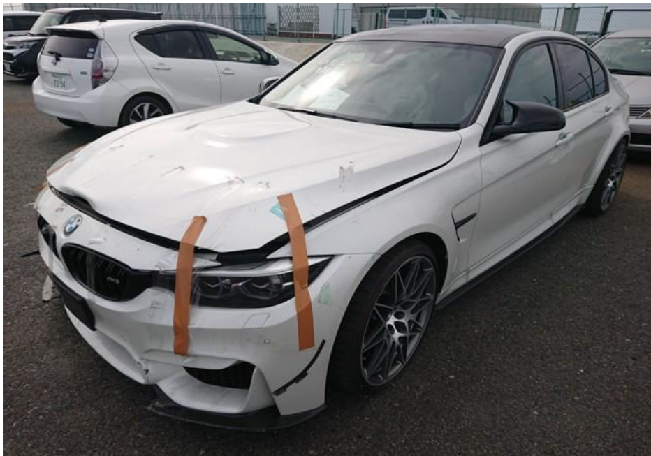
Photo 1 shows the front left body of the Motor Car prior to any repairs being carried out (photograph provided to me). The Motor Car was observed to have sustained damages at its frontal portion. The body parts observed to be damaged had included the front bumper, front grille and front bonnet. The airbags of the Motor Car were not activated as seen from the photograph.
