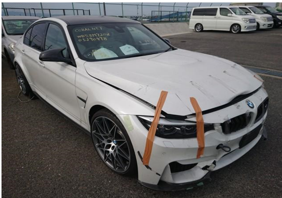
Photo 2 shows the front right body of the Motor Car prior to any repairs being carried out (photograph provided to me). The Motor Car was observed to have sustained damages at its frontal portion. The body parts observed to be damaged had included the front bumper, front grille and front bonnet. The airbags of the Motor Car were not activated as seen from the photograph.
