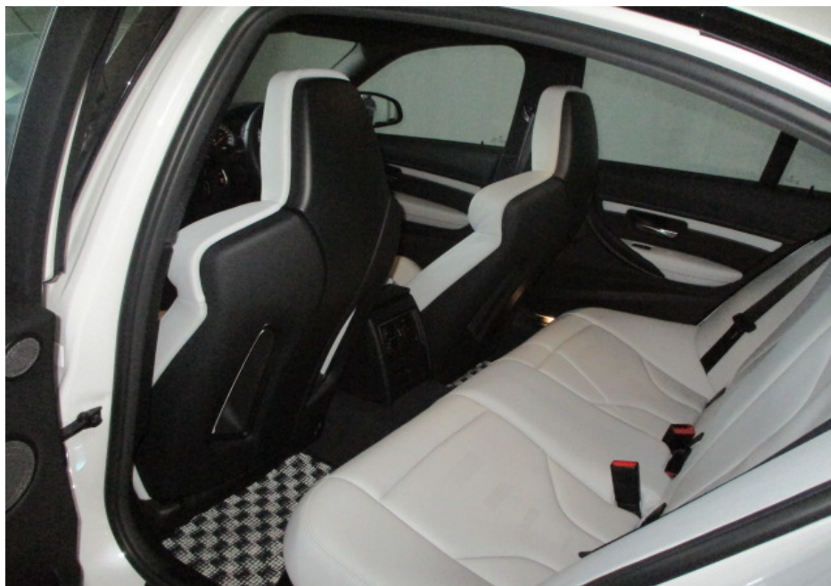
Photo 10 shows the seats of the Motor Car, which were secured via seat rails to the floorboard. All the seats of the Motor Car were fitted with a retractable seat belt reel and pre-tensioner. The seat belts were tested and able to be fastened into the respective pre-tensions that were fitted on the side of each individual seat.
