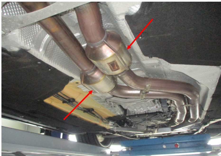
Photo 17 shows the Motor Car's centre catalytic converters (arrowed). My examination of the Motor Car's exhaust system revealed no sign(s) or indication(s) of any cut or weld marks along its exhaust pipes and on its rear mufflers.
