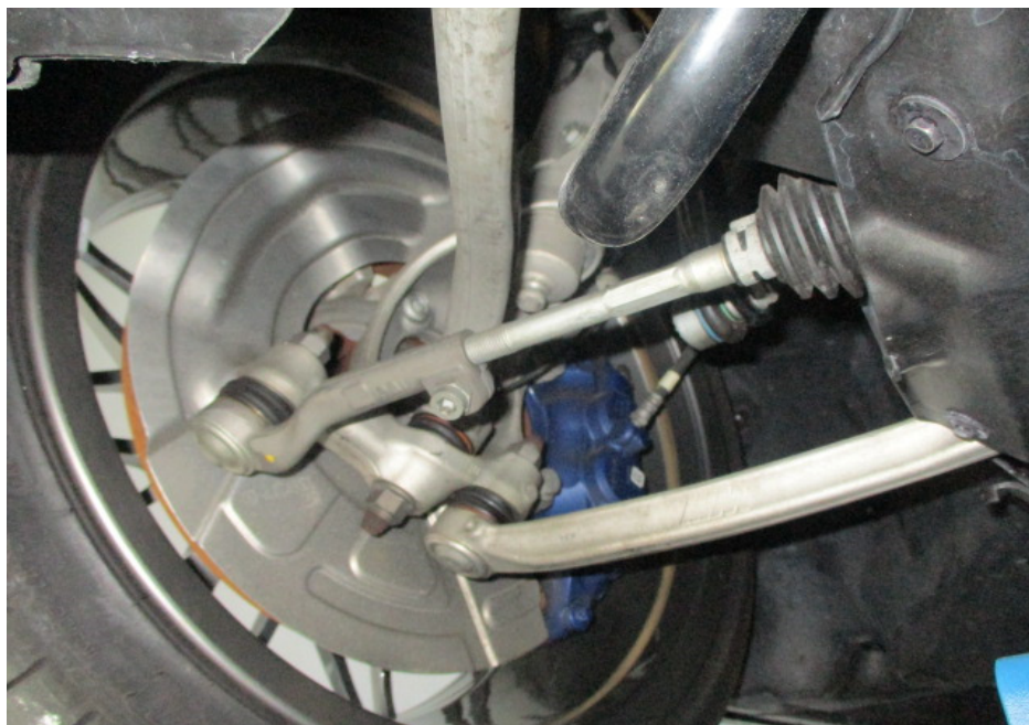
Photo 16 shows the various undercarriage components at the front right wheel of the Motor Car. The mechanical components, control arms and linkages were all found to be intact and secured in an appropriate manner. I also did not observe any fluid leak and/or fluid stain on the underside of the Motor Car.
