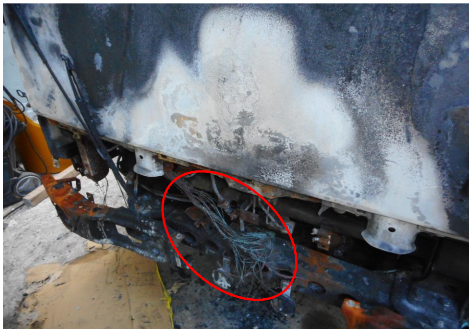
Photo 13 shows a general view of the original wiring harness leading to the fuse box into the front cabin compartment from the front of the Insured Vehicle. The original wiring harness (red circle) was observed with greenish residue on the surface. The presence of greenish residue indicates internal heating of copper wires, a sign of an electrical short circuit occurring. The greenish residue is normally left behind from oxidation as a result of chemical reaction involving the copper wires.
