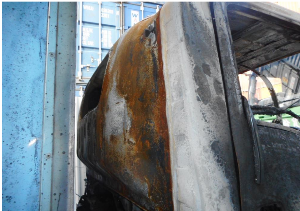
Photo 9 the close up view of the rear of the front cabin's exterior of the Insured Vehicle. The front cabin body panel have been badly burnt by the fire.
