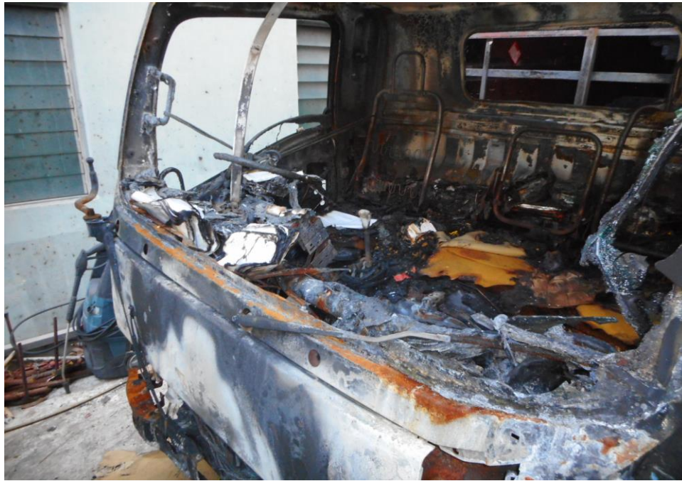
Photo 5 shows the general view of the interior compartment of the Insured Vehicle. The entire windscreen and the interior compartment have been badly burnt by the fire.
