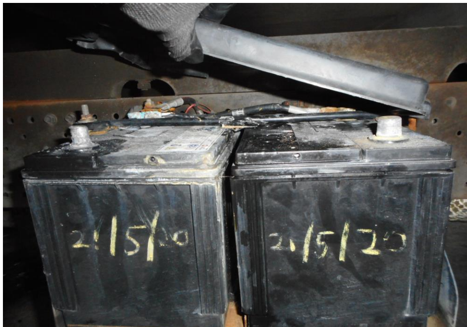
Photo 16 shows a close up view of the batteries of the Insured Vehicle at the time of our inspection. The fire damage to the Insured Vehicle was confined to its front portion and did not affect its batteries as it was mounted in the middle of the Insured Vehicle.
