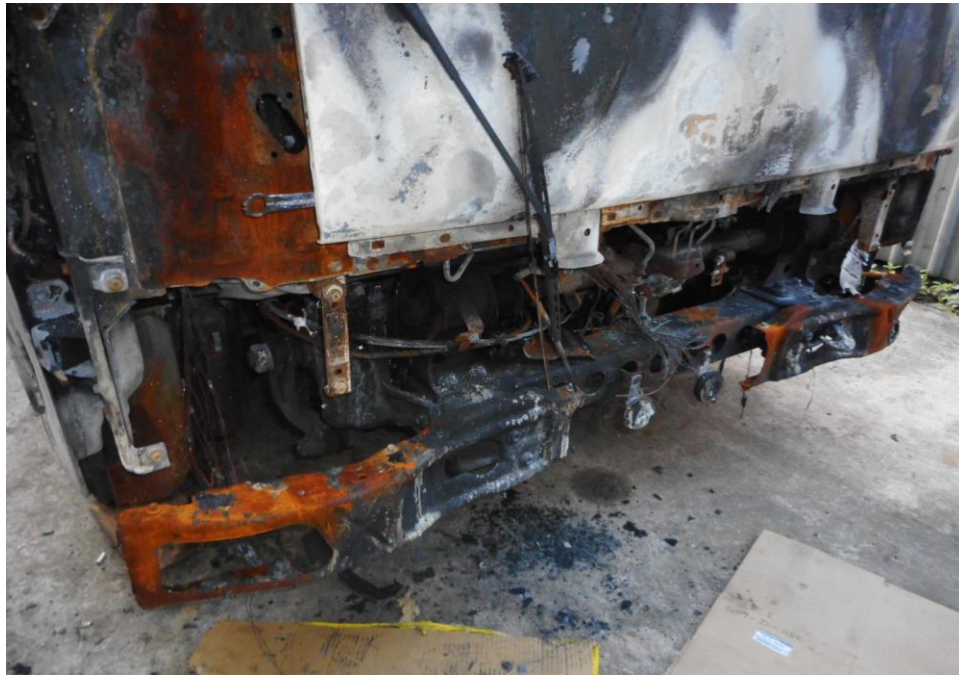
Photo 8 shows the close up view of the front cabin's exterior of the Insured Vehicle. The exterior compartment have been badly burnt by the fire.
