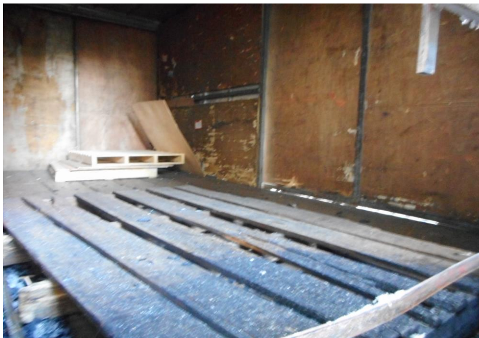
Photo 11 shows the inside of the rear cabin of the Insured Vehicle from the right side at the time of our inspection. The goods in the rear cabin that the Insured Vehicle was carrying were amongst the parts that were observed to have sustained heat & smoke damage.
