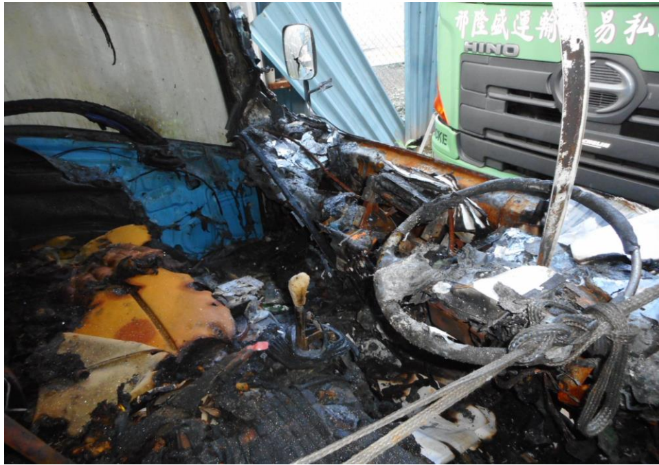
Photo 7 shows the close up view of the interior compartment of the Insured Vehicle. The interior compartment have been badly burnt by the fire.
