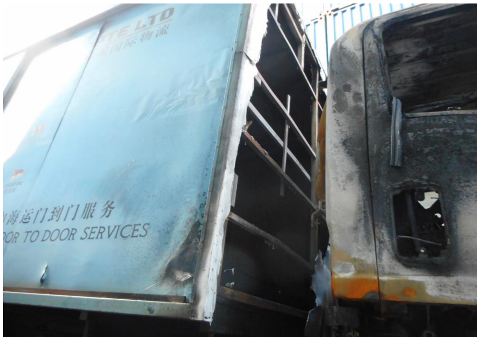
Photo 10 shows the rear cabin of the Insured Vehicle from the right side at the time of our inspection. The fire damage to the Insured Vehicle had burnt down the body panel of the rear portion and were amongst the parts that were observed to have been affected by the fire.
