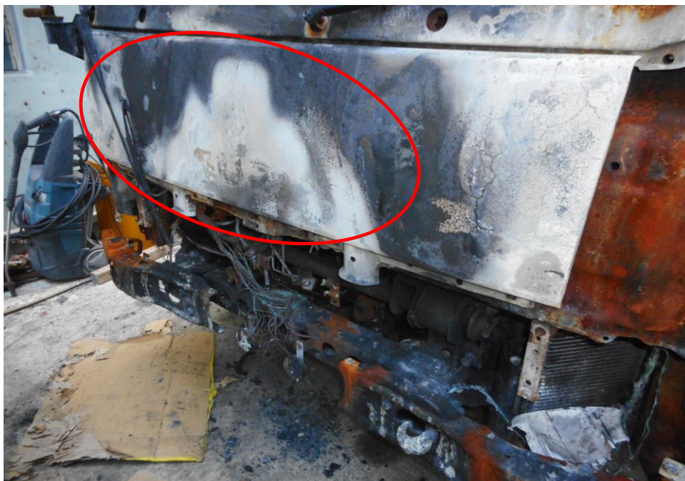
Photo 12 shows the front portion body panel of the Insured Vehicle at the time of our inspection. The high heat intensity burn marks (whitish burn marks) and rust that had development found on the exterior surface of the bonnet indicates that the fire had originated from the front portion of the Insured Vehicle.
