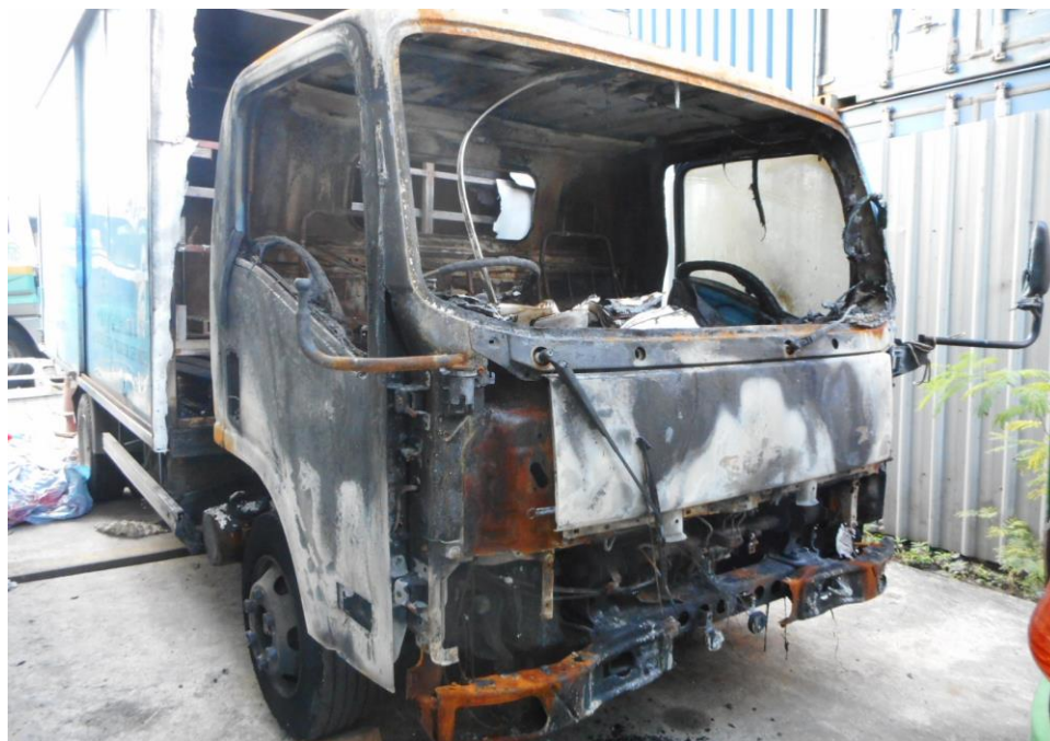
Photo 4 shows the front view of the Insured Vehicle at the time of our inspection. The fire damage to the Insured Vehicle had affected the whole front & rear cabin of the Insured Vehicle.
