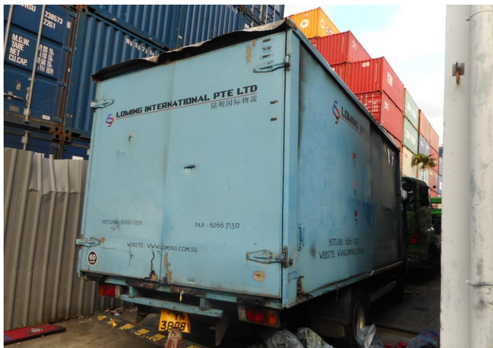
Photo 2 shows the general view of the right portion of the Insured Vehicle at the time of our inspection. The fire damage to the Insured Vehicle was confined to its front portion. Its right portion is observed to be unaffected by the fire.
