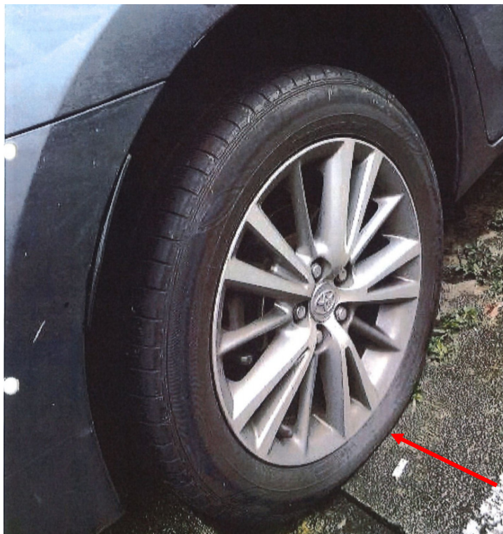
Photo 2 shows the rear right tyre of the Defendant Vehicle (photograph exhibited at page 19 of DAEIC). The rear right tyre of the Defendant's Vehicle was observed to be punctured as seen from the bulge at the area of the tyre that is resting on the ground (arrowed). The tyre was however still intact and wrapped around the rear right wheel rim.
