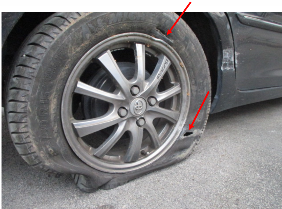
Photo 3 shows a tyre that has its outer sidewall torn (arrowed). Such physical condition is typically seen when a tyre burst. Rapid loss of pressurized air occurs when the pressurized air gushes out from the hole. A driver can lose control of a vehicle due to the sudden and rapid loss of pressurized air. Note the physical difference between this tyre and the rear right tyre of the Defendant Vehicle as shown in photograph 2 above, and other photographs exhibited in page 18, 19, 25 and 27 of DAEIC.
