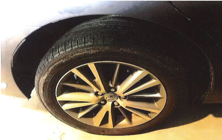
Photo 1 shows the rear right tyre of the Defendant Vehicle (photograph exhibited at page 25 of DAEIC). The rear right tyre of the Defendant's Vehicle was observed to be punctured. The rear right tyre was not torn/shredded. No hole and/or cut mark(s) was observed on the outer sidewall of the tyre.
