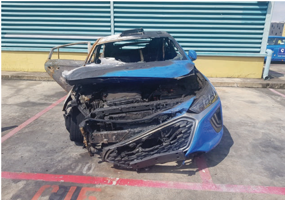
Photo 2 shows the general view of the frontal portion of the Insured Vehicle at the time of our inspection. The fire damage to the Insured Vehicle was confined to its frontal portion and right body. The entire engine compartment of the Insured Vehicle was observed to be severely burnt while the interior compartment was observed to be severely affected by the fire.
