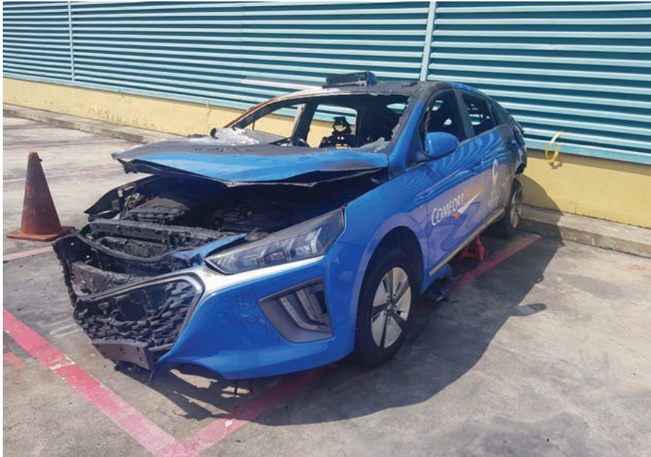
Photo 1 shows the general view of the left frontal portion of the Insured Vehicle at the time of our inspection. The left body of the Insured Vehicle was relatively unaffected by the fire.
