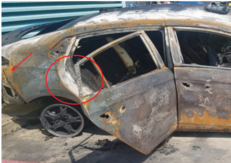
Photo 7 shows the fire damage at the right rear portion of the Insured Vehicle. The high heat intensity burn marks (whitish burn marks) found on the exterior surface of its right rear fender (circled) and rust that had developed on the right rear fender (arrowed) indicates that the fire to the Insured Vehicle had originated from the exterior of the Insured Vehicle.
