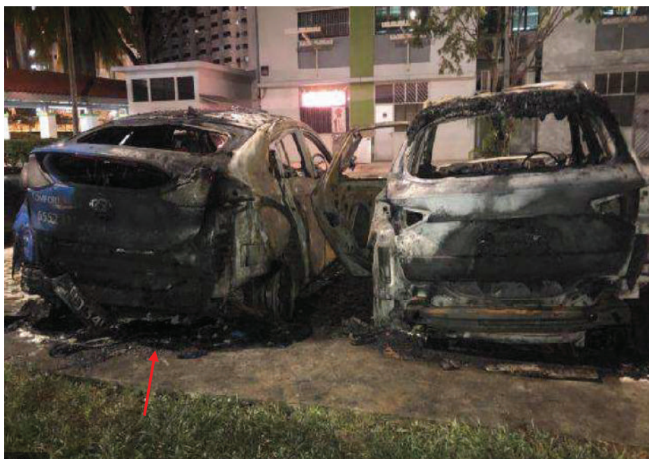
Photo 14 shows the rear portion of the Insured Vehicle and the other parked car at the incident scene after the fire was extinguished by SCDF personnel. The raised kerb directly behind the rear portion of the Insured Vehicle was observed to be burnt (arrowed).
