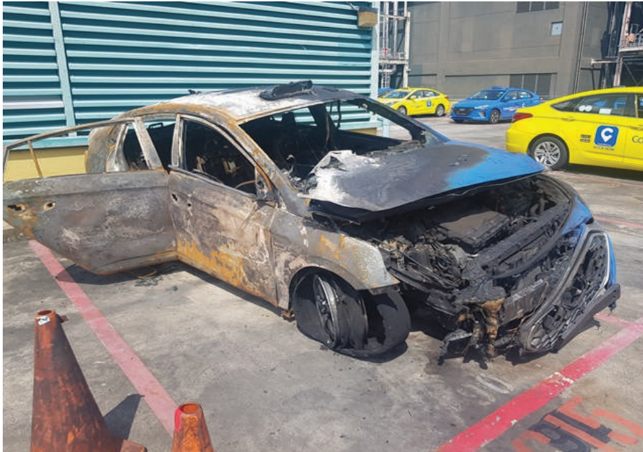
Photo 3 shows the closer view of the right front body of the Insured Vehicle at the time of our inspection. The fire damage to the Insured Vehicle was confined to its frontal portion and right body. Its front bumper, front bonnet, front support panel, front grille, front headlamps, front windscreen, right rims, right body and right tyres were amongst the body parts that were found to have been affected by the fire.
