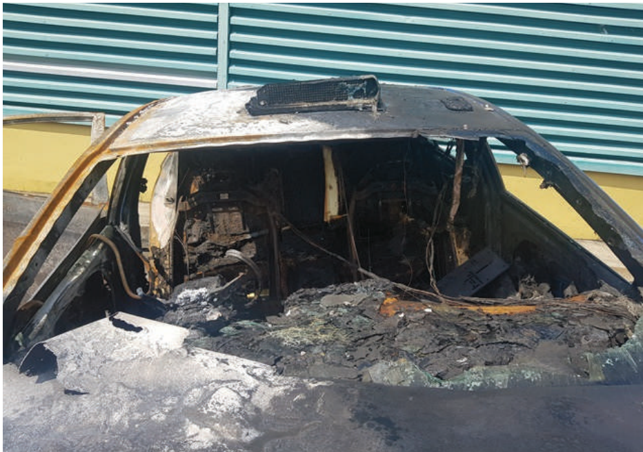
Photo 4 shows the general view of the front windscreen of the Insured Vehicle at the time of our inspection. The fire damage to the front windscreen was extensive.
