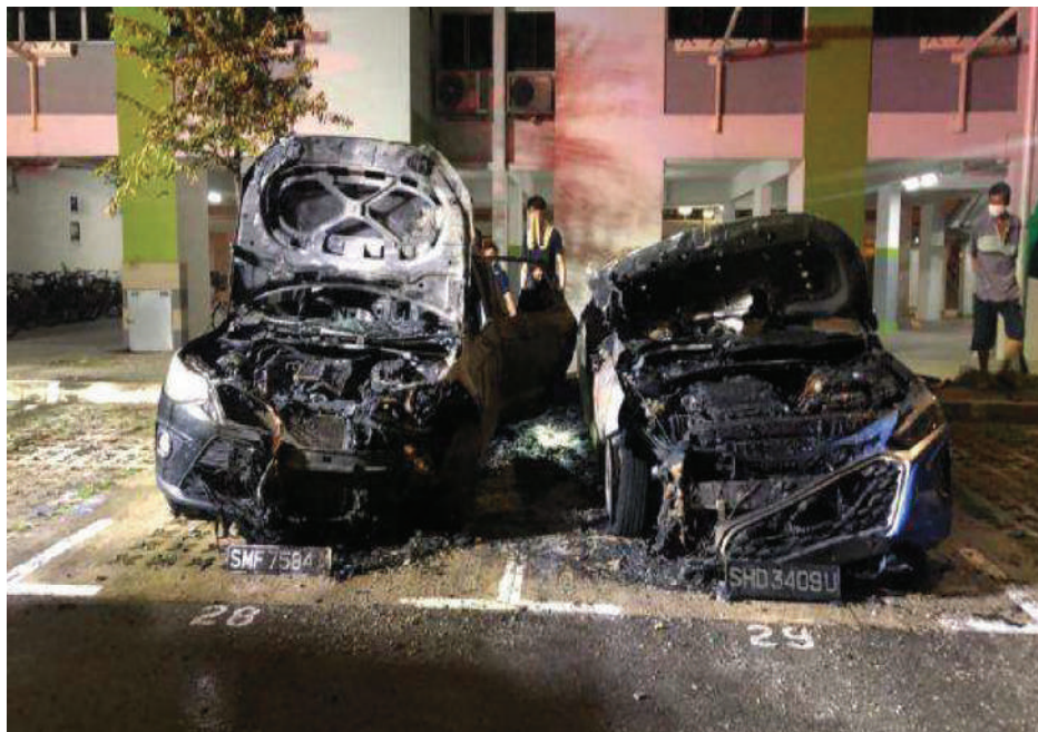
Photo 13 shows the Insured Vehicle and the other parked car at the incident scene after the fire was extinguished by SCDF personnel. The extent of damage and burn pattern to the Insured Vehicle was observed to be similar to what we had observed during our inspection of the Insured Vehicle.
