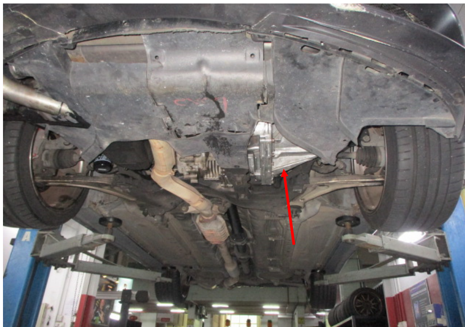
Photo 2 shows a general view of the transmission assembly (arrowed) that was fitted on the Motor Car. This was the input side of the transmission, which houses the main shaft and various gear sets. It is bolted to the crankshaft side of the engine block.
