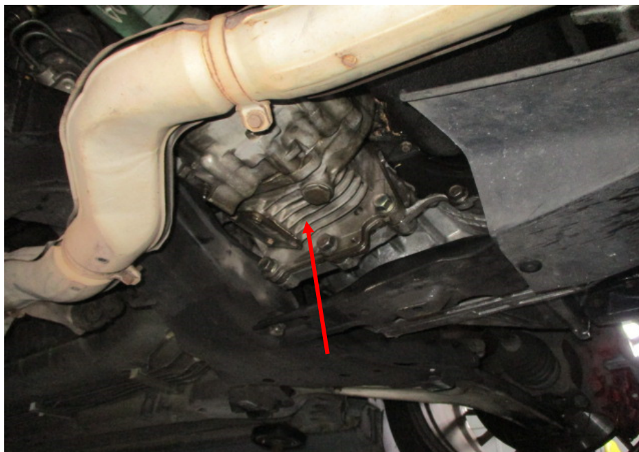
Photo 5 shows another view of the transfer case (arrowed) that was fitted on the Motor Car. The transfer case is the output side of the transmission. There was no crack and/or hole observed on the housing of the transfer case.
