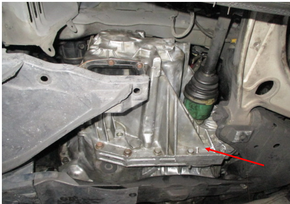
Photo 3 shows another view of the transmission assembly (arrowed) that was fitted on the Motor Car. This was the input side of the transmission, which houses the main shaft and various gear sets. There was no crack and/or hole observed on the transmission housing.
