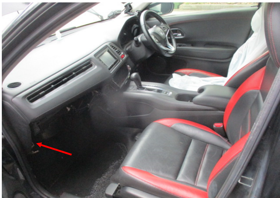
Photo 6 shows the interior compartment of the Insured Vehicle at the time of our inspection. The left portion of the interior compartment of the Insured Vehicle had sustained minimal fire damage (arrowed).
