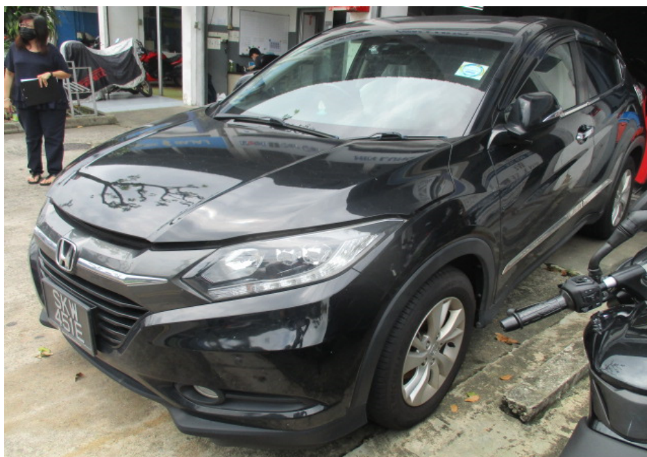
Photo 2 shows the general view of the left front portion of the Insured Vehicle at the time of our inspection. The exterior body of the Insured Vehicle had sustained visible fire damage. This included its front windscreen, wiper panel, left 'A' pillar, left side panel and instrument panel.
