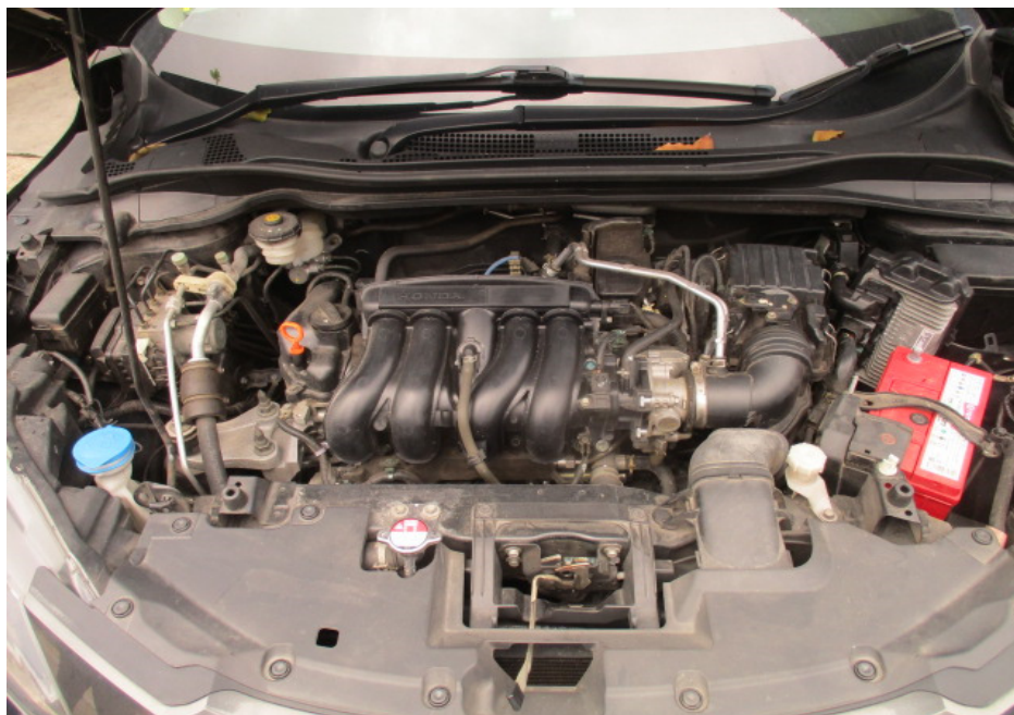
Photo 5 shows a general view of the engine compartment of the Insured Vehicle at the time of our inspection. The engine compartment was relatively unaffected by the fire.
