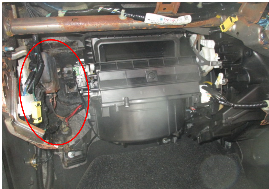
Photo 7 shows a closer view of the left portion of the interior compartment (after removing the glove compartment) of the Insured Vehicle at the time of our inspection. The left portion of the interior compartment of the Insured Vehicle had sustained fire damage (circled).
