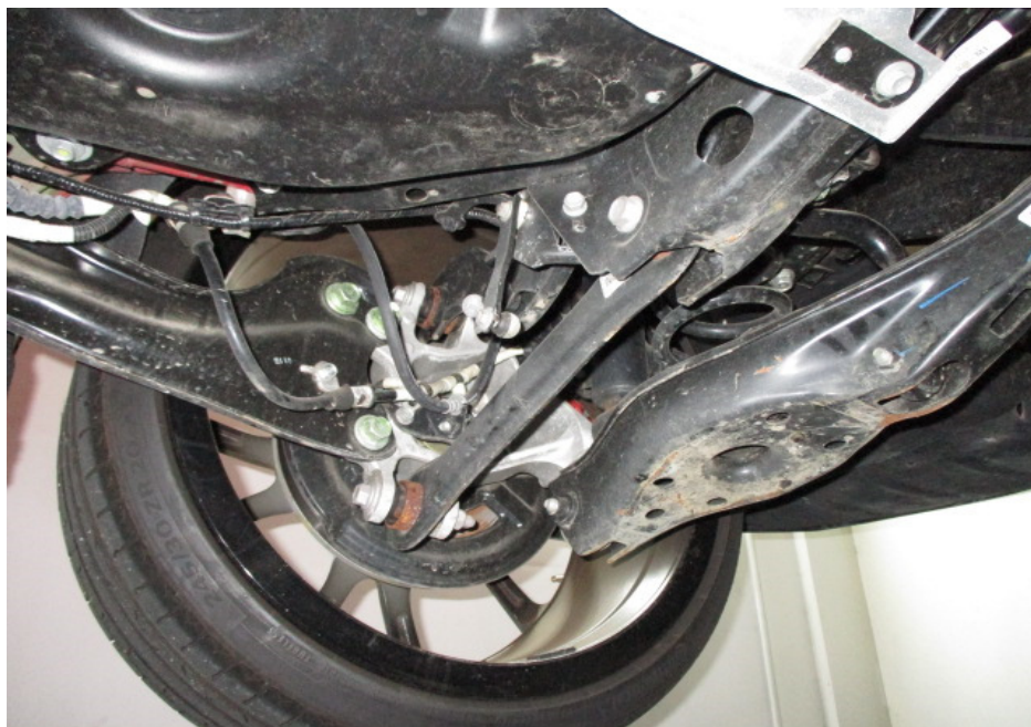
Photo 12 shows a general view of the control arms and linkages at the rear right wheel of the Motor Car. I did not observe any fluid leak and/or fluid stain on the underside of the Motor Car. All of the Motor Car's undercarriage components were observed to be intact and secured in an appropriate manner.
