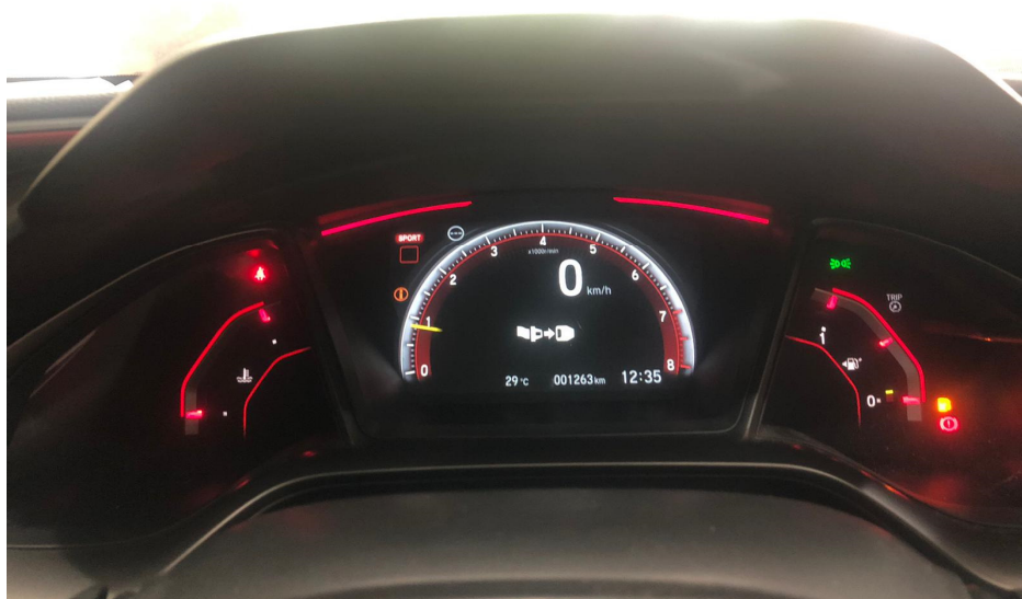
Photo 10 shows the respective warning lights no longer illuminated after the engine was started, indicating that there was no fault detected to the ABS, SRS, EPS and VSA systems of the Motor Car during the self-test. These electronic systems were hence in working condition at the time of my inspection.
