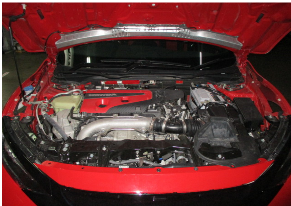
Photo 7 shows a general view of the engine compartment of the Motor Car at the time of my inspection. The damaged parts within the engine compartment of the Motor Car (refer photograph 2 above) were visually examined and it was observed that the repair/restoration works carried out were reasonably adequate and in order. Overall, I had found the various parts and components inside the engine compartment to be intact and properly fitted. There was also no sign(s) or indication(s) of fluid leak and/or fluid stain found inside the engine compartment.
