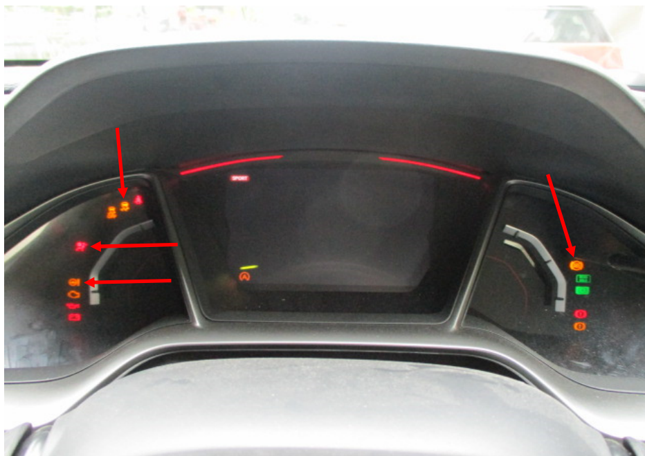
Photo 9 shows the warning lights for the various electronic safety features appearing on the instrument panel of the Motor Car during its self-test when the engine is cranked, in particular the ABS, SRS, EPS and VSA lights (arrowed).
