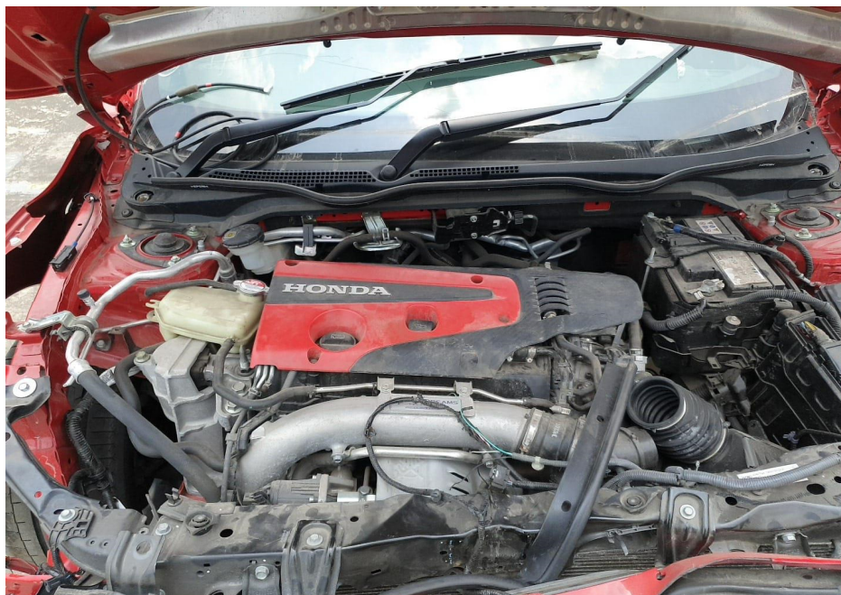
Photo 2 shows the engine compartment of the Motor Car prior to any repairs being carried out (photograph provided to me). The front support panel, air hose, aircon condenser and radiator were amongst the parts within the engine compartment that were observed to be damaged.
