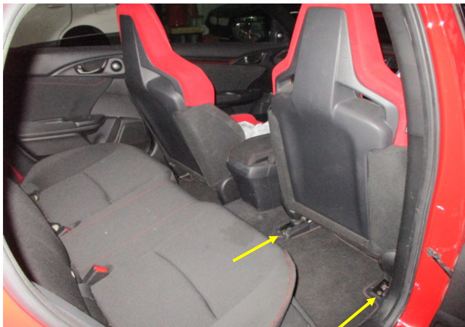
Photo 8 shows the seats of the Motor Car, which were secured via seat rails (arrowed) to the floorboard. All the seats of the Motor Car were fitted with a retractable seat belt reel and pre-tensioner. The seat belts were tested and able to be fastened into the respective pre-tensions that were fitted on the side of each individual seat.
