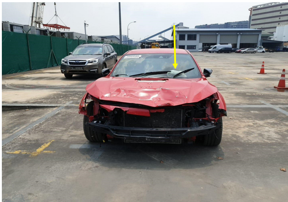
Photo 1 shows the Motor Car prior to any repairs being carried out (photograph provided to me). The Motor Car was observed to have sustained damages at its frontal portion. The body parts observed to be damaged include the front bumper, front fenders, front bonnet, front bumper reinforcement and front headlamps amongst others. The front left passenger seat belt (arrowed) was also deployed.
