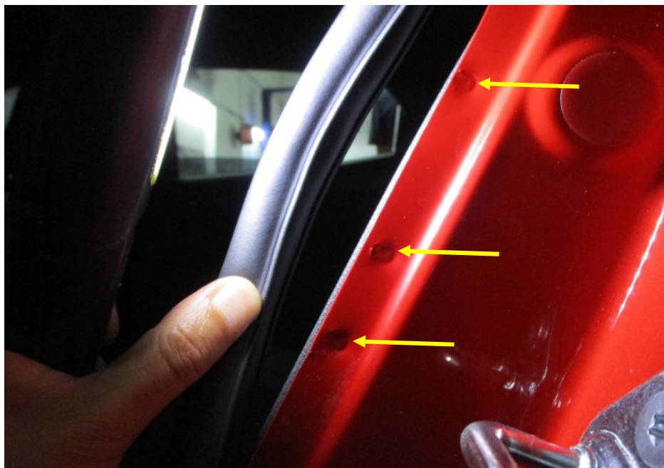
Photo 18 shows the rear left "C" pillar of the Motor Car. I did not find any weld marks other than original spot weld marks (arrowed) on the non-detachable body panels of the Motor Car, indicating that there was no re-welding works carried out; and that the non-detachable body panels of the Motor Car were originally fitted.
