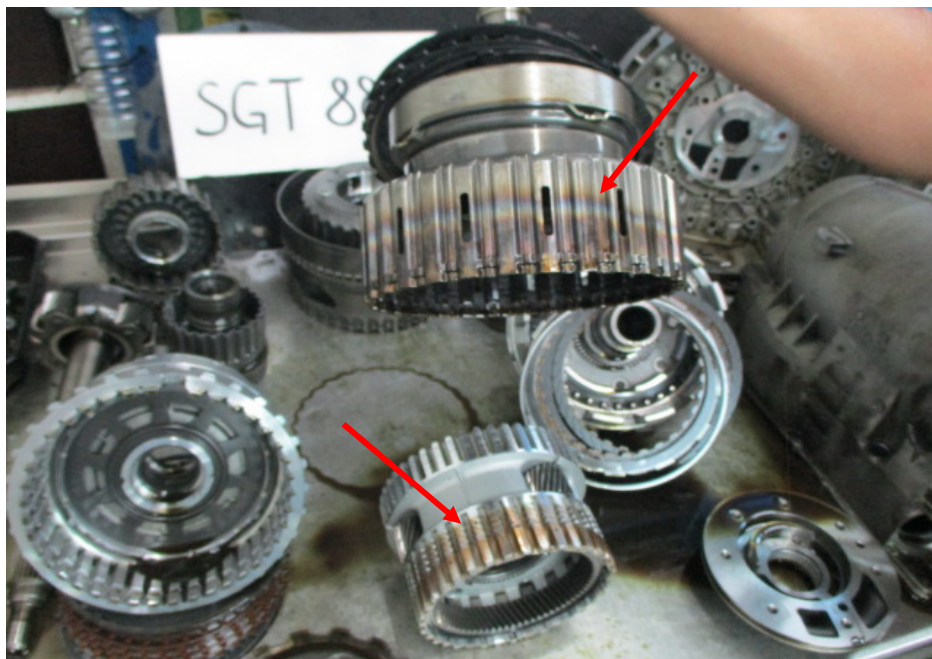
Photo 11 shows burnt marks (arrowed) found on several transmission gear set. This is an indication of an overheated transmission.
