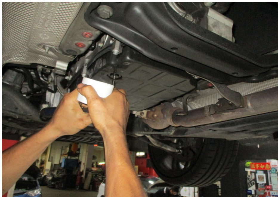
Photo 8 shows removal of the transmission fluid drain plug for checks on the transmission fluid of the Motor Car. This was during my inspection of the Motor Car.
