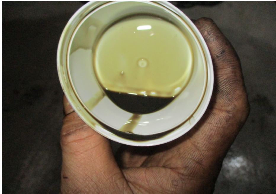
Photo 9 shows the transmission fluid that was collected from the Motor Car. The transmission fluid of the Motor Car was observed to be burnt/blackened. A typical automatic transmission fluid colour is reddish.
