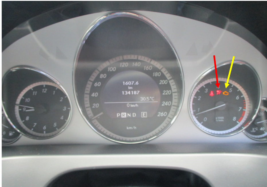
Photo 4 shows the check engine light (yellow arrow) and SRS light (red arrow) illuminated on the Motor Car's instrument panel. The illumination of these lights indicates a fault(s) in the engine system and a fault(s) in the Supplemental Restraint System of the Motor Car.
