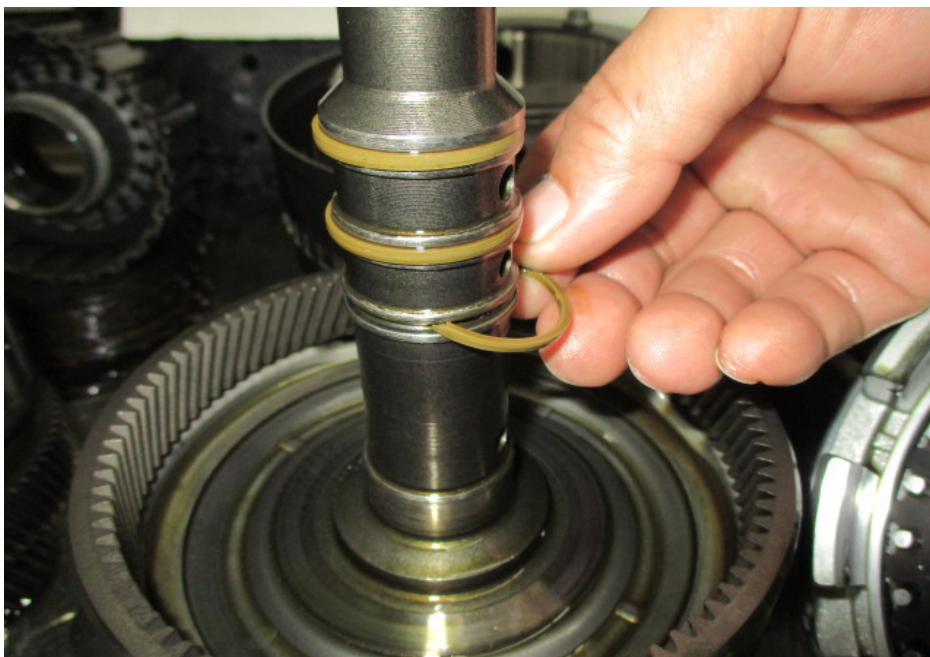
Photo 15 shows one of the diaphragms attached to the transmission input shaft broken.
