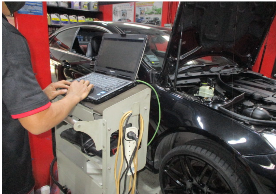
Photo 5 shows the OBD scan being carried out to the Motor Car to establish the cause(s) of the check engine light and the SRS light that were illuminated on the instrument panel of the Motor Car. The result at the end of the OBD scan revealed transmission gear slippage in the Motor Car's transmission system causing the check engine light to be illuminated, and a faulty front right seat belt buckle, causing the SRS light to be illuminated.
