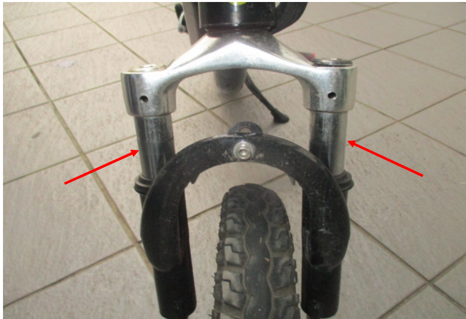
Photo 17 shows the front fork (arrowed) of the Electric Scooter. The front fork and fork bracket of the Electric Scooter were both found to be intact and undamaged. Turning the Electric Scooter's handle bar towards the left and right did not produce any abnormal free play. The steering system of the Electric Scooter was in serviceable condition at the time of our inspection.
