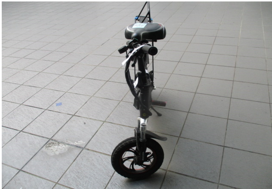
Photo 18 shows the front wheel of the Electric Scooter turned towards its full right. Turning the Electric Scooter's handle bar towards the right did not produce any abnormal free play and/or resistance. This would indicate that the steering system of the Electric Scooter was in serviceable condition at the time of our inspection.
