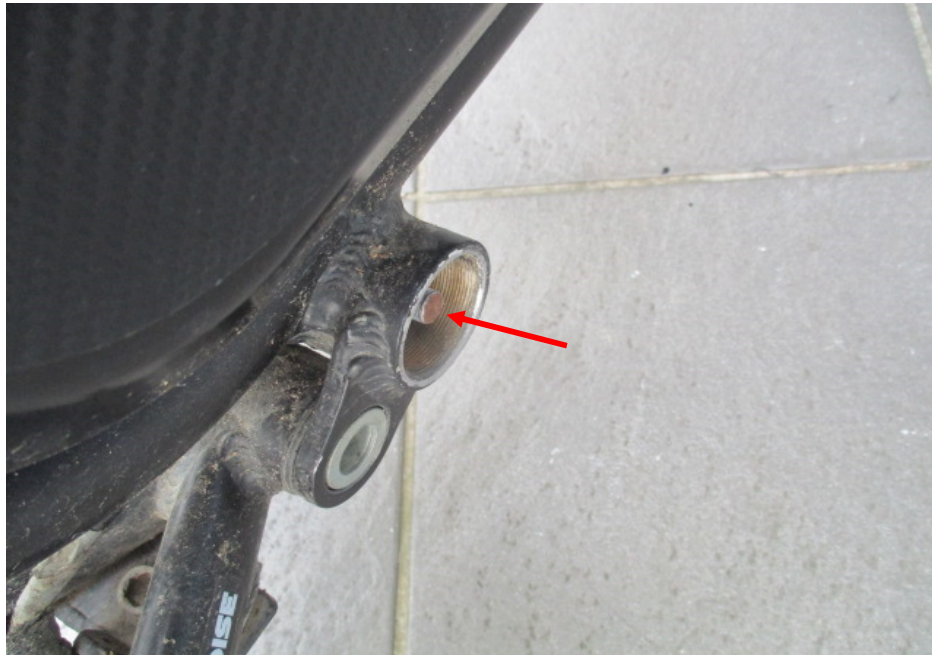
Photo 11 shows the missing right foot peg of the Electric Scooter at the time of our inspection (arrowed).
