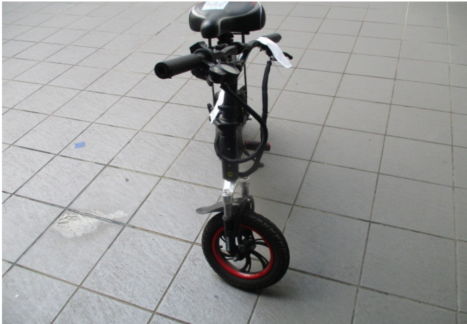
Photo 19 shows the front wheel of the Electric Scooter turned towards its full left. Turning the Electric Scooter's handle bar towards the left did not produce any abnormal free play and/or resistance. This would indicate that the steering system of the Electric Scooter was in serviceable condition at the time of our inspection.
