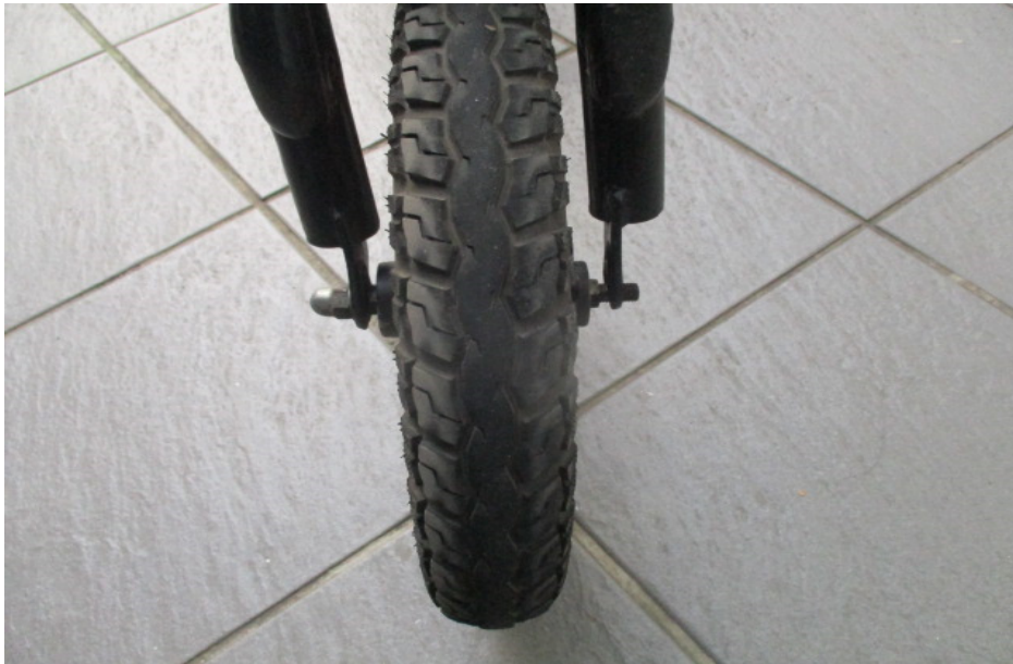
Photo 13 shows the front tyre of the Electric Scooter at the time of our inspection. The front tyre was observed to be in serviceable condition with remaining tread depth of approximately 3mm. The tyre was also observed to be sufficiently inflated for vehicular operation. We did not observe any tear, burst mark(s) and/or punctured hole(s) on the sidewalls as well as across the tread of the front tyre.
