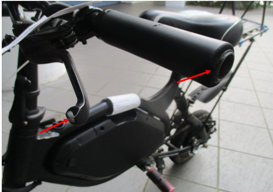
Photo 7 shows the damages on the left handlebar end and left hand brake lever (arrowed) of the Electric Scooter as a result of the accident.
