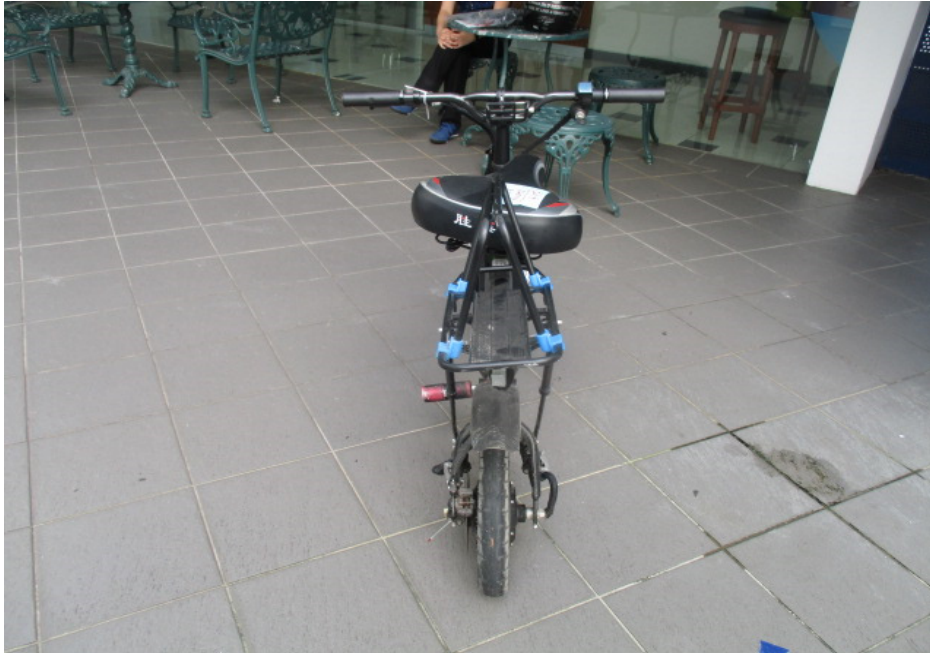
Photo 5 shows the rear portion of the Electric Scooter at the time of our inspection. The Electric Scooter was observed to have sustained damages all around. The body parts that were found to have been damaged include its handlebar ends, left hand brake lever, seat, right foot peg, right cowling and top rack, amongst others as a result of the accident.
