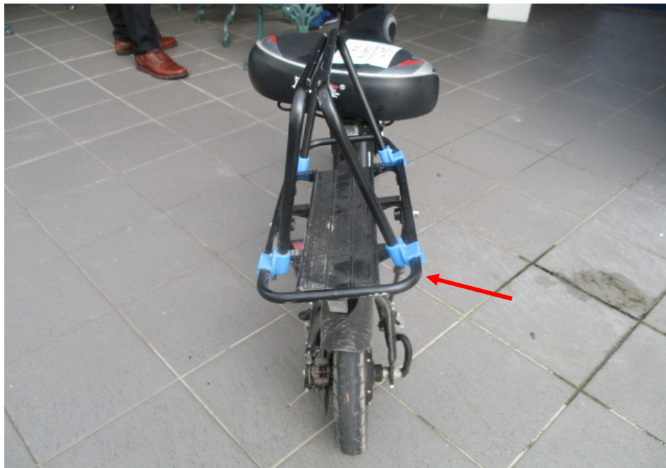
Photo 12 shows the deformed top rack of the Electric Scooter at the time of our inspection (arrowed).
