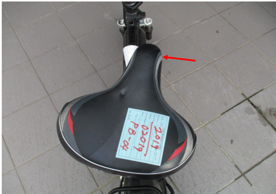
Photo 10 shows the deformed seat of the Electric Scooter (arrowed) at the time of our inspection.
