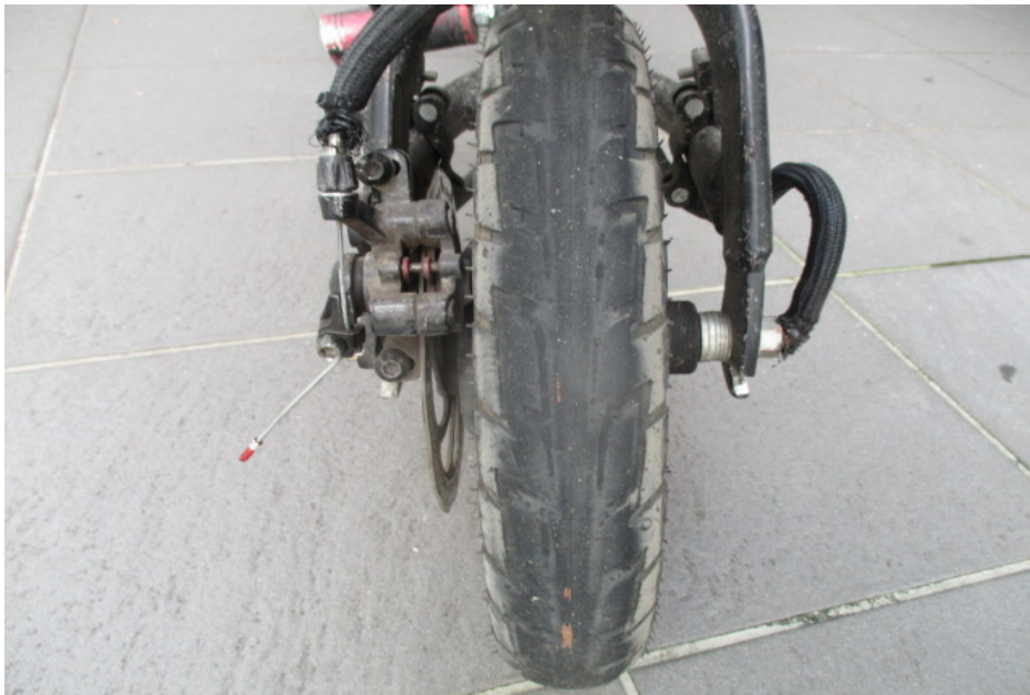
Photo 14 shows the rear tyre of the Electric Scooter at the time of our inspection. The rear tyre was observed to be in serviceable condition with remaining tread depth of approximately 3mm. The tyre was also observed to be sufficiently inflated for vehicular operation. We did not observe any tear, burst mark(s) and/or punctured hole(s) on the sidewalls as well as across the tread of the rear tyre.
