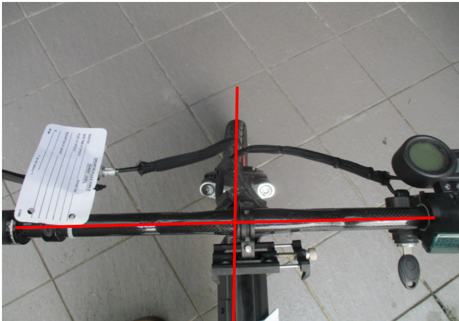
Photo 6 shows the frontal portion of the Electric Scooter (top view) at the time of our inspection. A slight misalignment of the handle bar & front tyre was observed.
