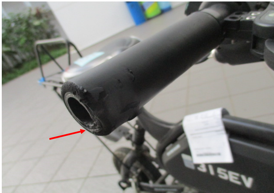
Photo 8 shows damages on the right handlebar end (arrowed) of the Electric Scooter as a result of the accident.
