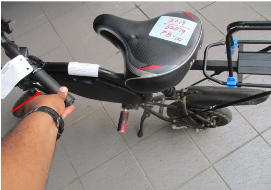
Photo 20 shows a static brake test conducted on the Electric Scooter's rear brake. There was some resistance felt upon pressing the left hand brake lever (arrowed).
