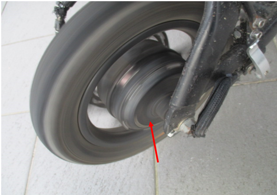
Photo 16 shows the general view of the drive motor of the Electric Scooter which was observed to be in operational condition (arrowed).
