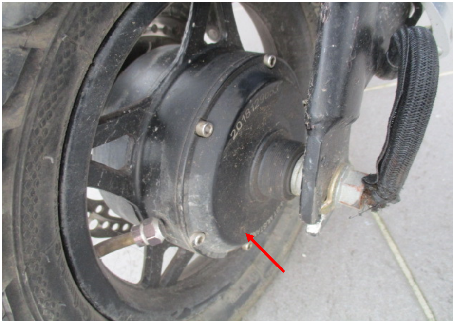
Photo 15 shows the general view of the drive motor (arrowed) of the Electric Scooter which was observed to be intact with no misalignment.
