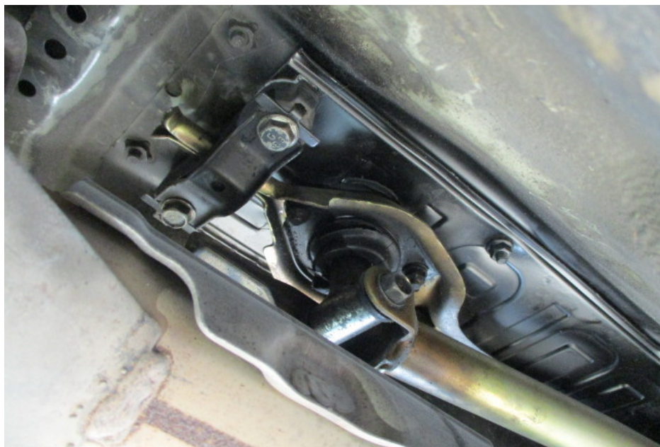
Photo 8 shows the gear selector fork, at the side where it connects to the gear shifter in the interior compartment of the Motor Car through the floorboard.
