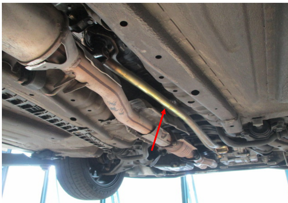
Photo 7 shows the gear selector fork (arrowed) from the transmission to the gear shifter of the Motor Car. The gear selector fork was observed to be securely fitted on the underside of the Motor Car. This gear selector fork connects to the gear shifter in the interior compartment of the Motor Car through the floorboard
