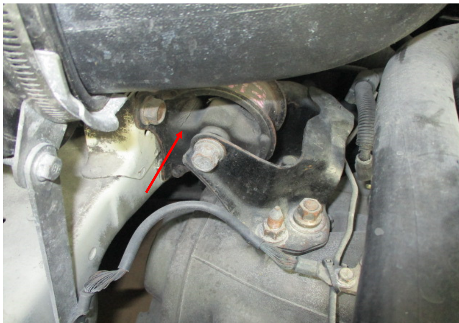
Photo 6 shows the bracket supporting the right side of the Motor Car's transmission. This bracket was mounted onto the right side front chassis, adjacent to the right side front wheel house. The bracket was with rubber bushings (arrowed) that absorbs any vibrations arising from the rotation of the transmission gears, minimising any stress to the bracket and correspondingly also minimise any stress to the right side front chassis member.
