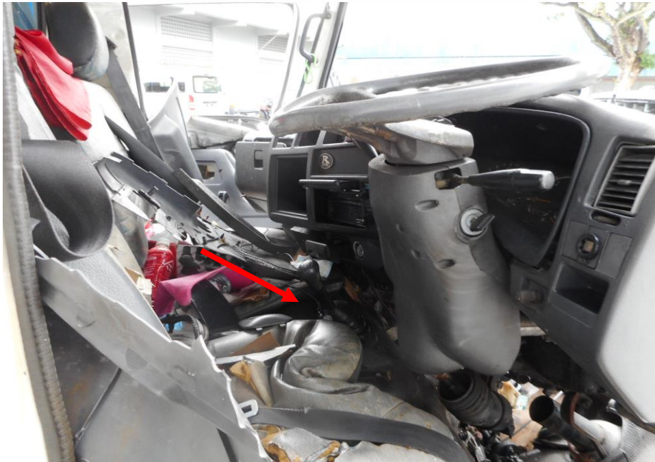
Photo 8 shows the close up view of the interior cabin of the Motor Lorry. It was observed to have sustained extensive induced damages to the dashboard, foot well as a result of the accident.
