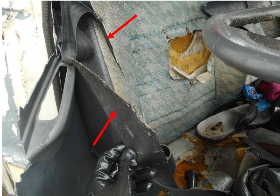
Photo 23 shows that the seat belt on the right seat was worn at the material time of accident as the safety pre-tensioners was activated at the moment of impact and caused the seat belts to be locked into the last position of the user and there was signs an extrication conducted (arrowed)
