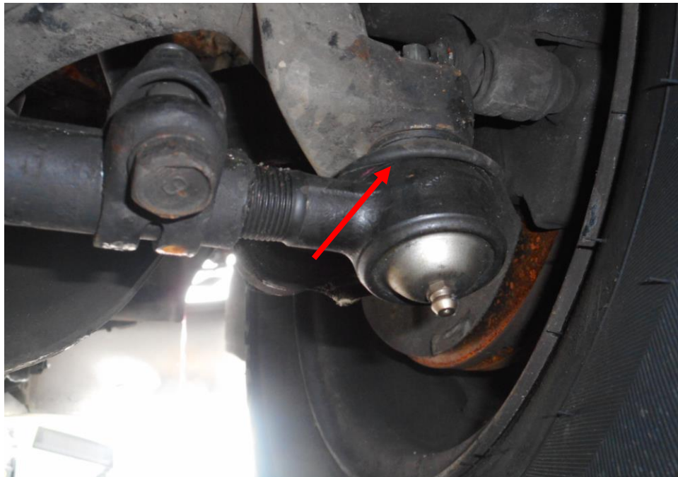
Photo 17 shows the various undercarriage components at the front right wheel of the Motor Lorry, in particular the steering tie rod end and ball joints (arrowed). The various undercarriage components of the Motor Lorry were all found to be intact without any visible damage. There was also no sign of fluid stain(s) observed on the various undercarriage components.
