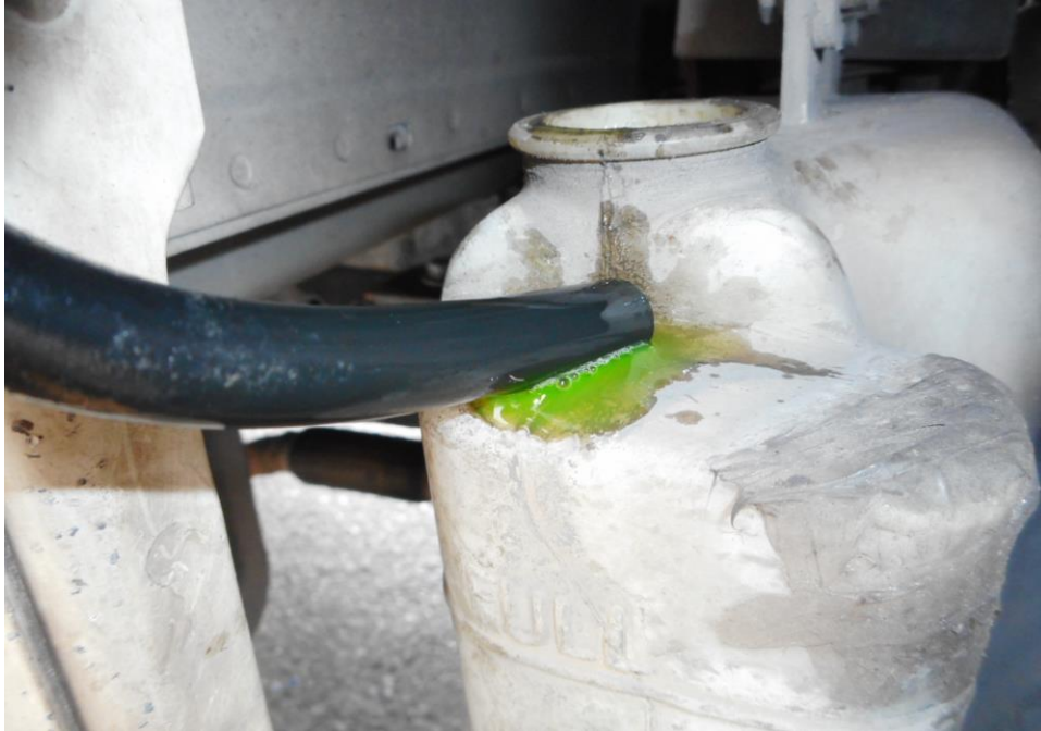
Photo 15 shows the engine coolant reservoir of the Motor Lorry at the time of our inspection. The coolant fluid was observed to be of sufficient level and without any visible contamination (arrowed).
