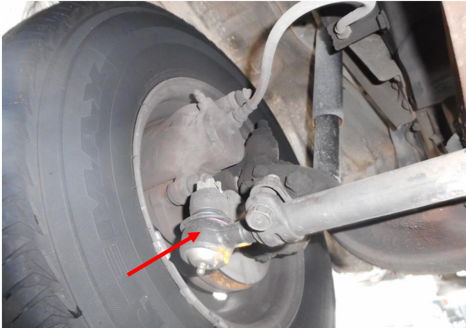
Photo 18 shows the various undercarriage components at the front left wheel of the Motor Lorry, in particular the steering tie rod end and ball joints (arrowed) were observed to be damaged.
