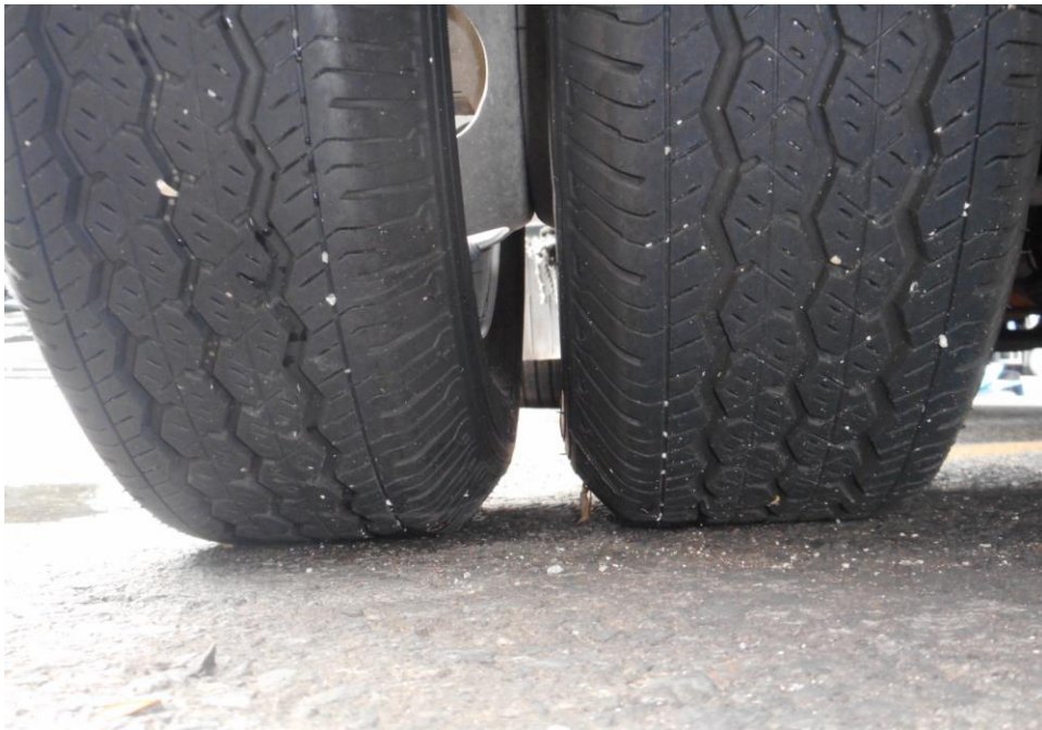
Photo 11 shows the condition of the rear left tyres of the Motor Lorry, which were observed to be in serviceable condition with remaining, tread depth of approximately 1.7mm. See above.
