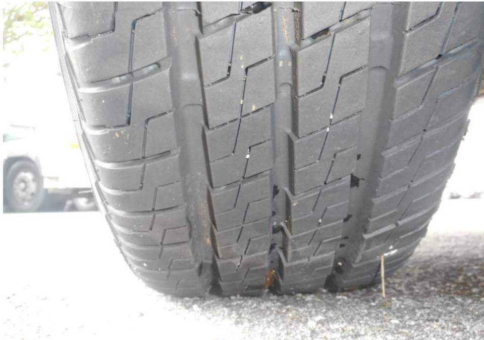
Photo 12 shows the condition of the front right tyre of the Motor Lorry, which was observed to be in serviceable condition with remaining tread depth of approximately 7.6mm. The tyre, which was wrapped around standard steel wheel rim, was also observed to be sufficiently inflated for vehicular operation.
