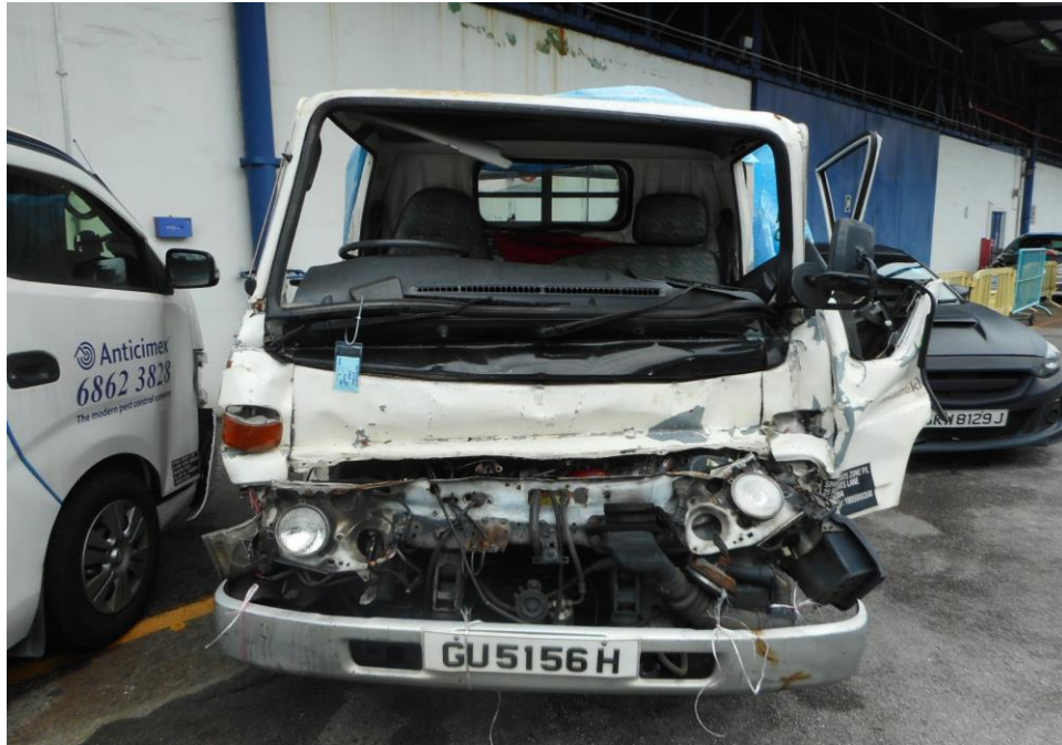
Photo 2 shows a general view of the front windscreen and body panel of the Motor Lorry at the time of our inspection. The Motor Lorry was observed sustained major damages to its frontal likely due to the accident's impact.
