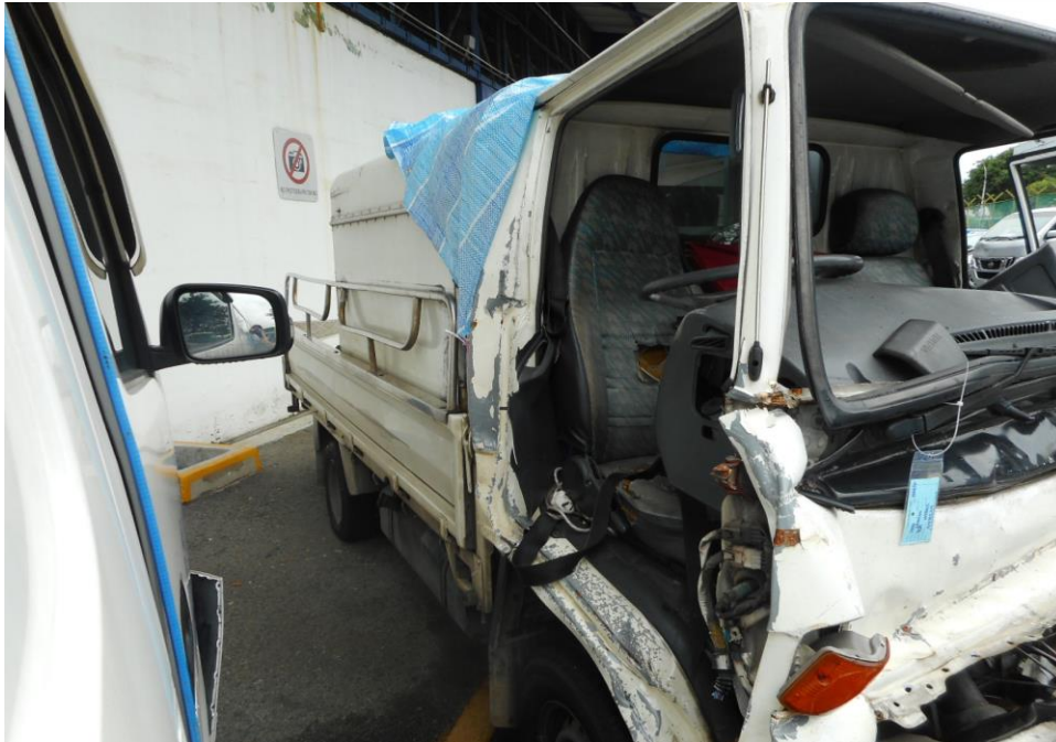
Photo 4 shows the close up view of the right door of the Motor Lorry at the time of our inspection. The Motor Lorry was observed to have sustained major damages to its doors that was crushed and dislodged due to the accident's impact.
