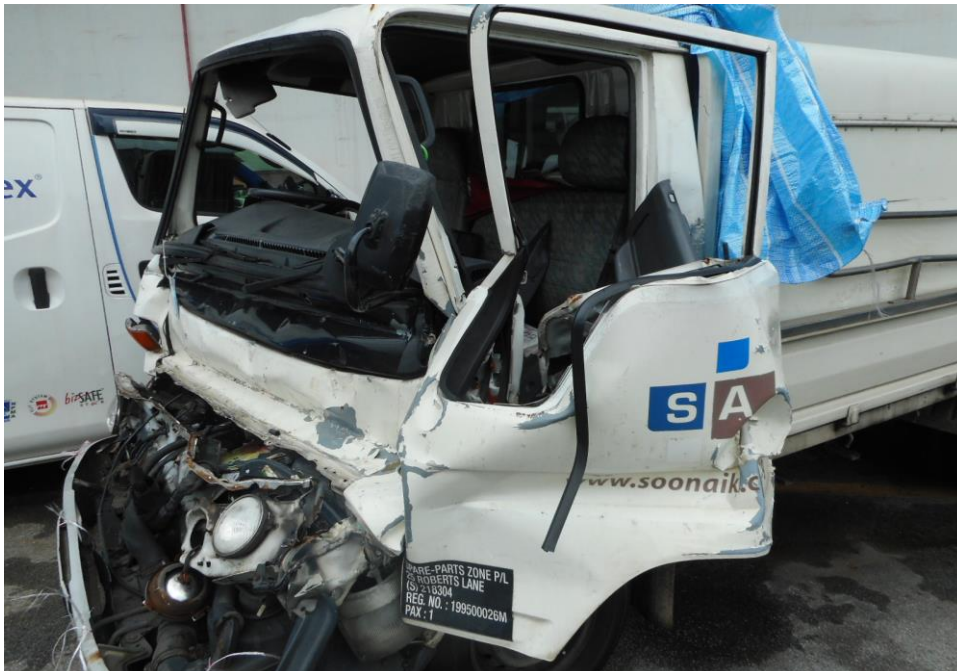
Photo 3 shows the close up view of the left door of the Motor Lorry at the time of our inspection. The Motor Lorry was observed to have sustained major damages to its doors that was crushed due to the accident's impact.
