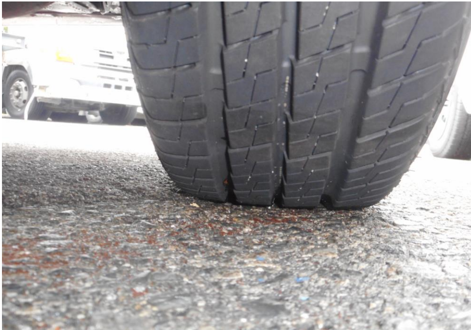
Photo 9 shows the condition of the front right tyre of the Motor Lorry, which was observed to be in serviceable condition with remaining tread depth of approximately 7.4mm. The tyre, which was wrapped around standard steel wheel rim, was also observed to be sufficiently inflated for vehicular operation.
