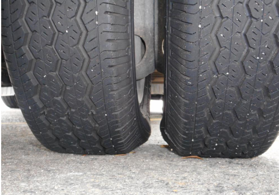
Photo 10 shows the condition of the rear right tyres of the Motor Lorry, which observed to be in serviceable condition with remaining tread depth of approximately 4.6mm. The tyres, which were wrapped around standard steel wheel rim, were also observed to be sufficiently inflated for vehicular operation.
