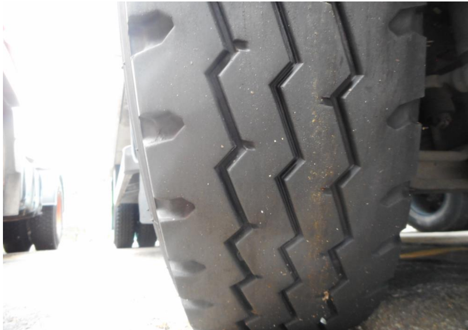
Photo 7 shows the condition of the front right tyre of the Motor Lorry, which was observed to be in serviceable condition with remaining tread depth of approximately 5.3mm. The tyre, which was wrapped around standard steel wheel rim, was also observed to be sufficiently inflated for vehicular operation. There was no tear, cut or burst mark(s) on the outer and the inner sidewalls as well as across the tread of the 6 tyres that were fitted on the Motor Lorry.
