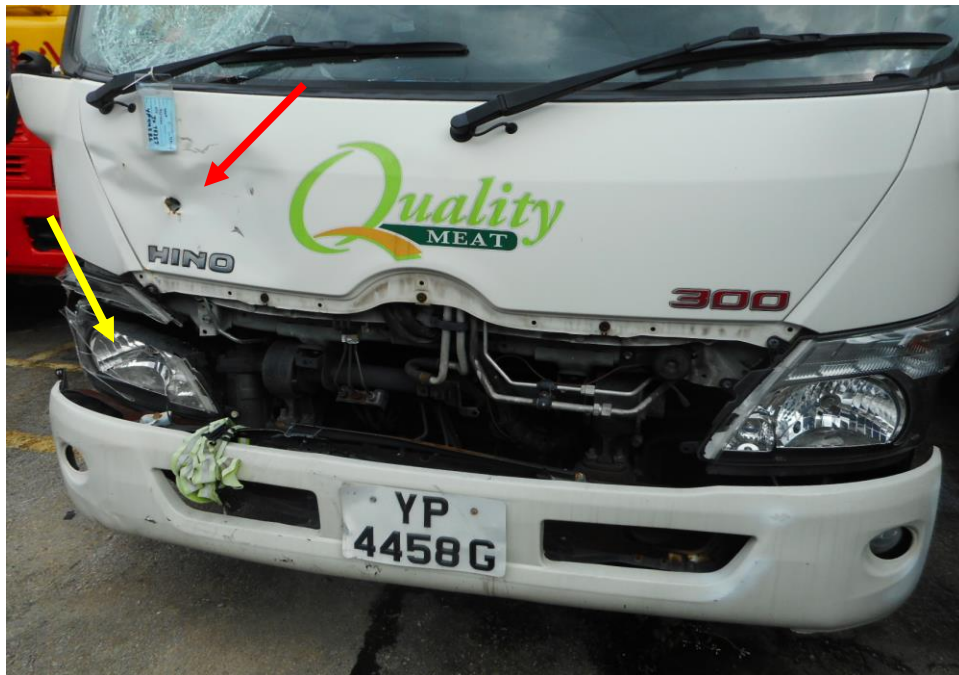
Photo 3 shows a close up view of the Motor Lorry's frontal portion at the time of my inspection. The Motor Lorry was observed to sustained damage at its front portion. Its front body panel (red arrow) and front right headlamp (yellow arrow) were damaged as a result of the accident.
