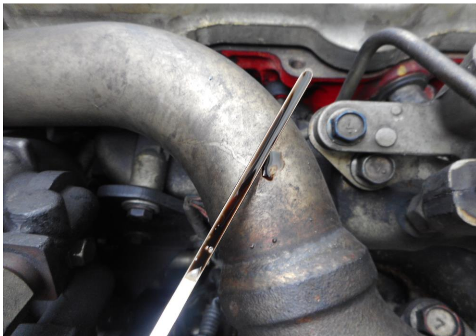
Photo 14 shows the engine oil dip stick of the Motor Lorry at the time of my inspection. The engine oil was observed to be of sufficient level and without any visible contamination.
