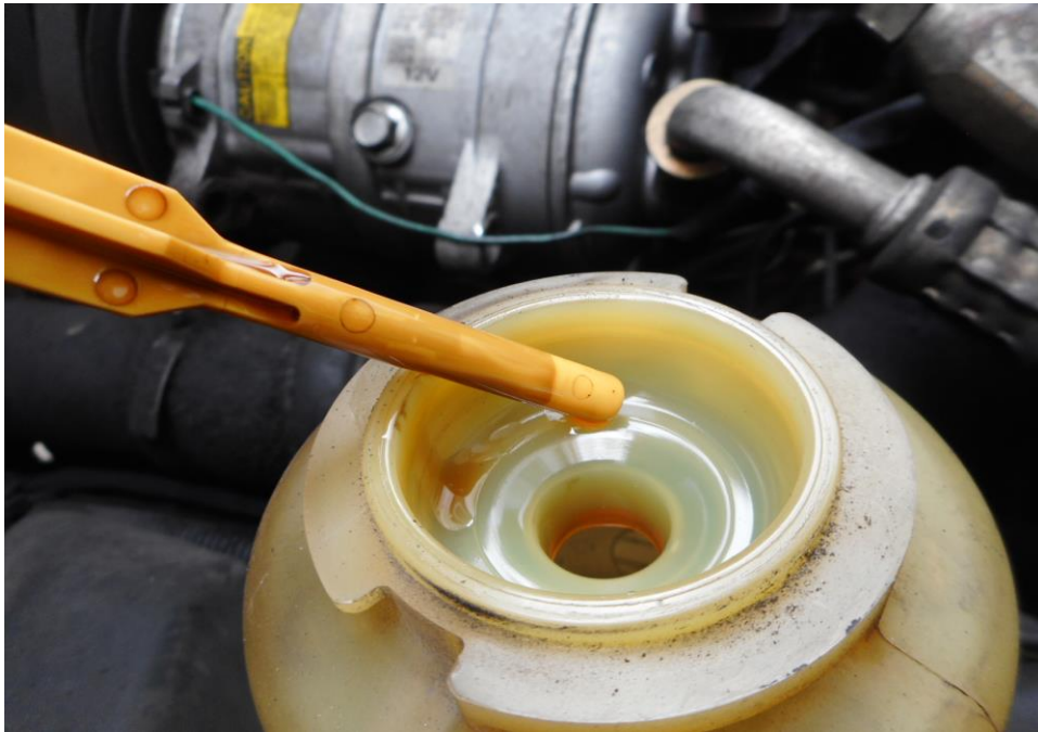
Photo 15 shows the power steering fluid dip stick of the Motor Lorry at the time of my inspection. The power steering fluid was observed to be of sufficient level and without any visible contamination.
