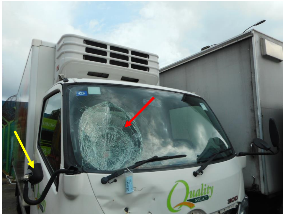
Photo 2 shows a close up view of the Motor Lorry's frontal portion at the time of my inspection. The Motor Lorry was observed to sustained damage at its front portion. Its front windscreen (red arrow) and front right rear view mirror (yellow arrow) were damaged as a result of the accident.
