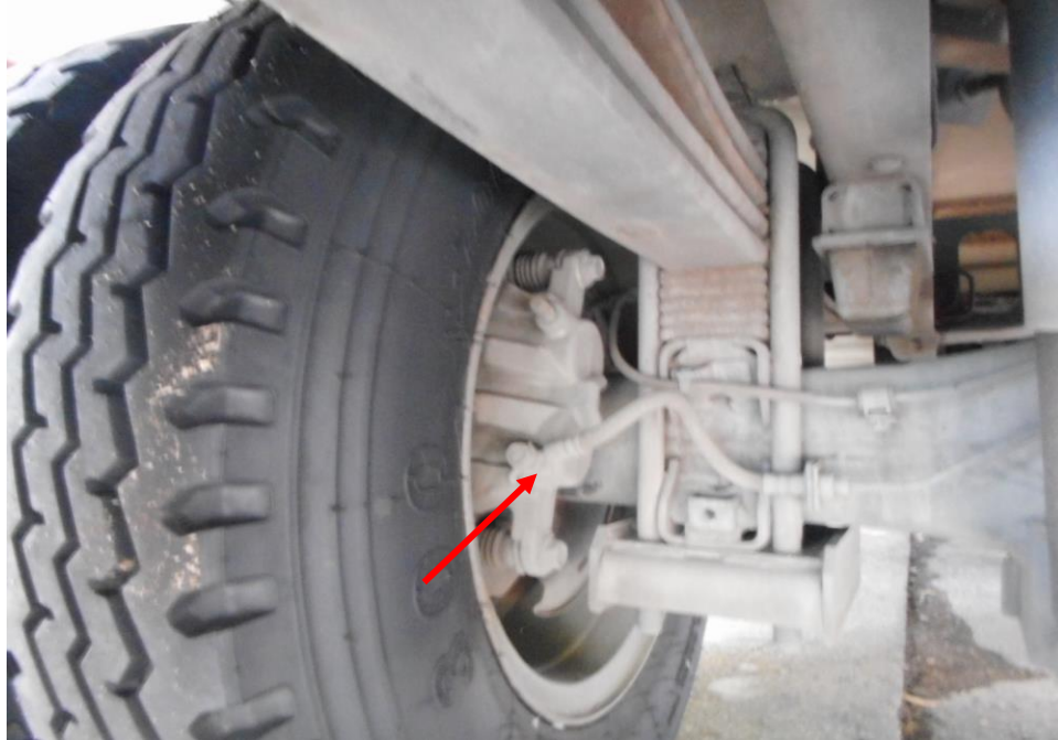
Photo 20 shows the brake pipe (arrowed) at the rear left wheel of the Motor Lorry. I did not observe any leakage of brake fluid at the time of my inspection of the Motor Lorry. My static tests of the Motor Lorry's braking system, along with my visual examination of the various mechanical components in the braking system had indicated that there was no internal leakage of pressure/vacuum. Hence the braking system of the Motor Lorry was likely to be in serviceable condition at the material time of accident.
