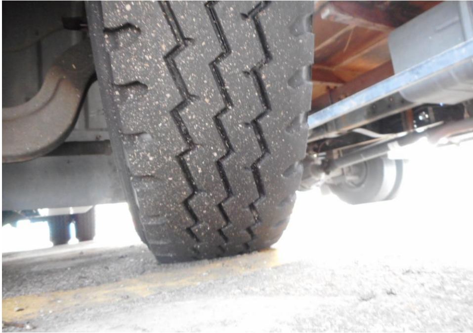
Photo 10 shows the condition of the front left tyre of the Motor Lorry, which were observed to be in serviceable condition with remaining, tread depth of approximately 8.2mm. There was also no tear, cut or burst mark(s) on the outer and the inner sidewalls as well as across the tread of the 6 tyres that were fitted on the Motor Lorry.
