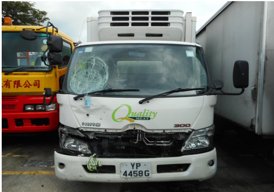
Photo 1 shows a general view of the Motor Lorry's frontal portion at the time of my inspection. The Motor Lorry was observed to sustained damage at its front portion. Its front windscreen, front body panel, front right rear view mirror and front right headlamp were damaged as a result of the accident.
