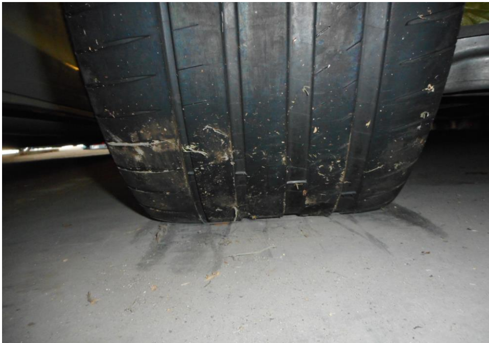
Photo 11 shows the condition of the rear left tyre of the Motor Car, which was observed to be in serviceable condition with remaining tread depth of approximately 3mm. The tyre, which was wrapped around steel wheel rim, was also observed to be sufficiently inflated for vehicular operation. The 4 tyres of the Motor Car were wrapped around standard steel wheel rims.
