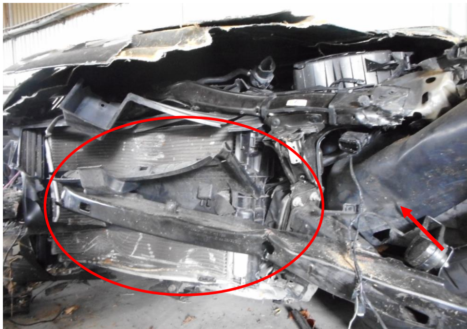
Photo 5 shows a close up view of the Motor Car's front body at the time of my inspection. Its front bumper (arrowed), radiator (circled) and various engine components were amongst the body parts that were damaged as a result of the accident.
