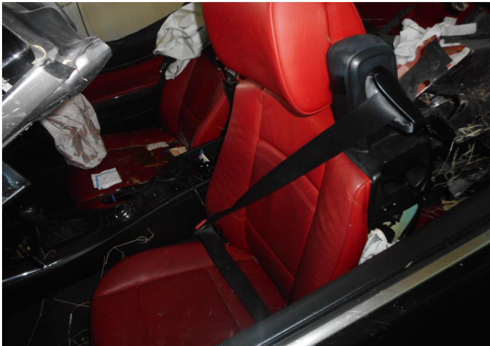
Photo 22 shows that the seat belt on the left seat were able to be fastened securely into the respective pre-tensioners that were fitted at the sides of each seat.
