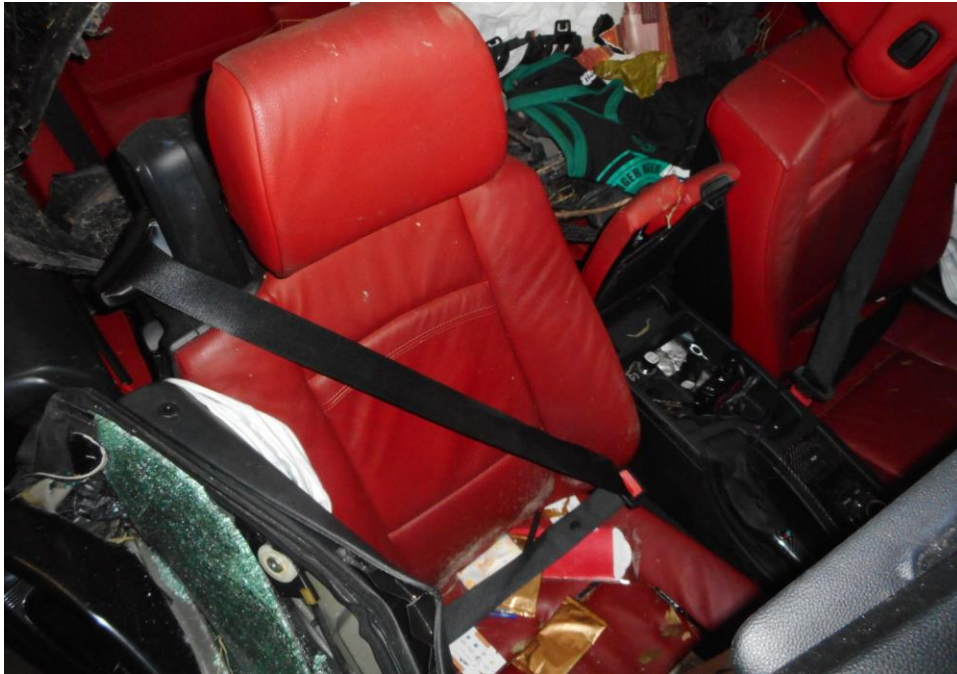
Photo 21 shows that the seat belt on the right seat were able to be fastened securely into the respective pre-tensioners that were fitted at the sides of each seat.
