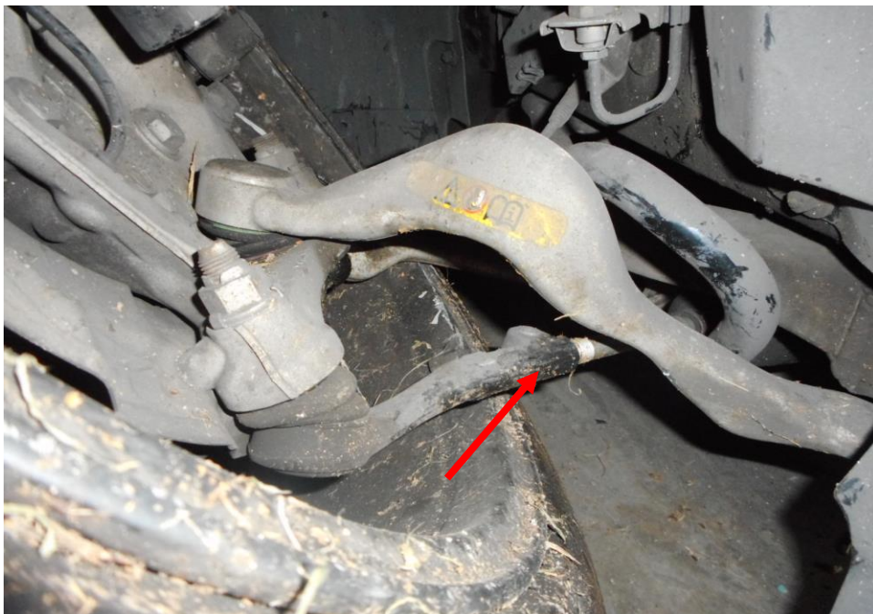
Photo 19 shows the various undercarriage components at the front right wheel of the Motor Car, in particular the steering tie rod (red arrow) and various steering components were all found to be damaged as a result of the accident.
