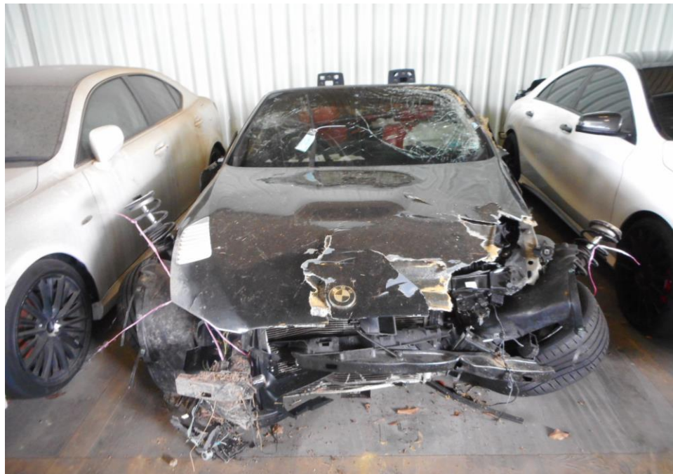
Photo 3 shows a general view of the Motor Car's front body at the time of my inspection. The Motor Car was observed to have sustained damage all around. Its front windscreen, front bonnet, front bumper, both front headlamps, its left and right body panels and rear bumper were amongst the body parts that were damaged as a result of the accident. The Supplemental Restraint System (SRS) was activated as a result of the accident.
