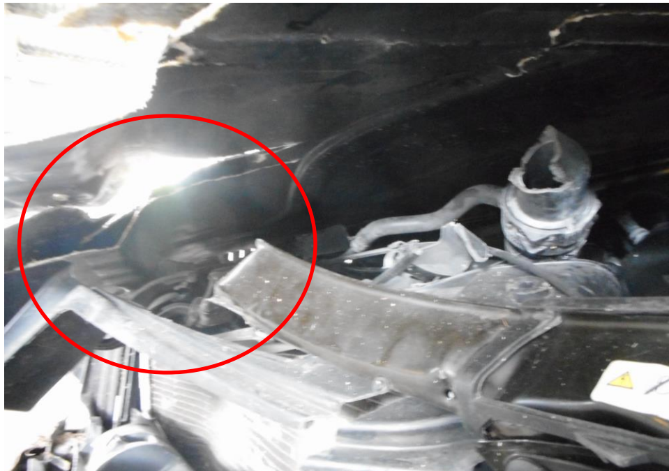
Photo 14 shows a close up view of the damaged front bonnet lock mechanism and the structure of the engine compartment of the Motor Car at the time of my inspection resulting it unable to open a result of the accident. (circled) (Unable to open)
