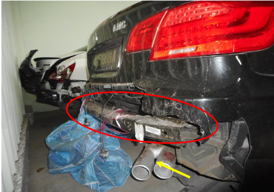
Photo 2 shows the general view of the Motor Car's rear body at the time of my inspection, its rear bumper (red arrow) and exhaust piping (yellow arrow) were amongst the body parts that were damaged as a result of the accident.
