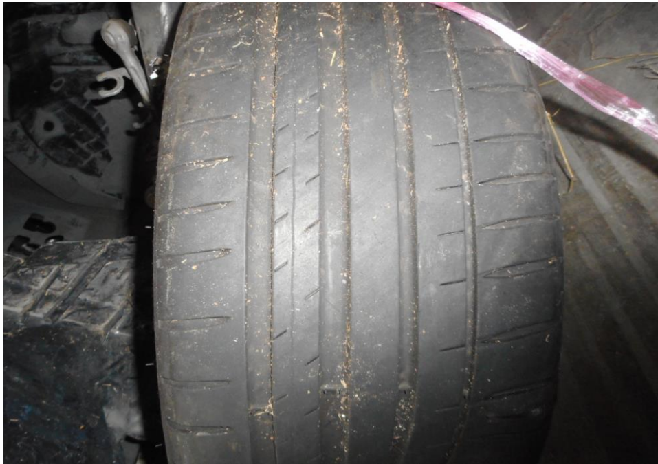
Photo 12 shows the condition of the front left tyre of the Motor Car, which was observed to be in serviceable condition with remaining tread depth of approximately 5.3mm. The tyre, which was wrapped around steel wheel rim, was also observed to be sufficiently inflated for vehicular operation. The 4 tyres of the Motor Car were wrapped around standard steel wheel rims.
