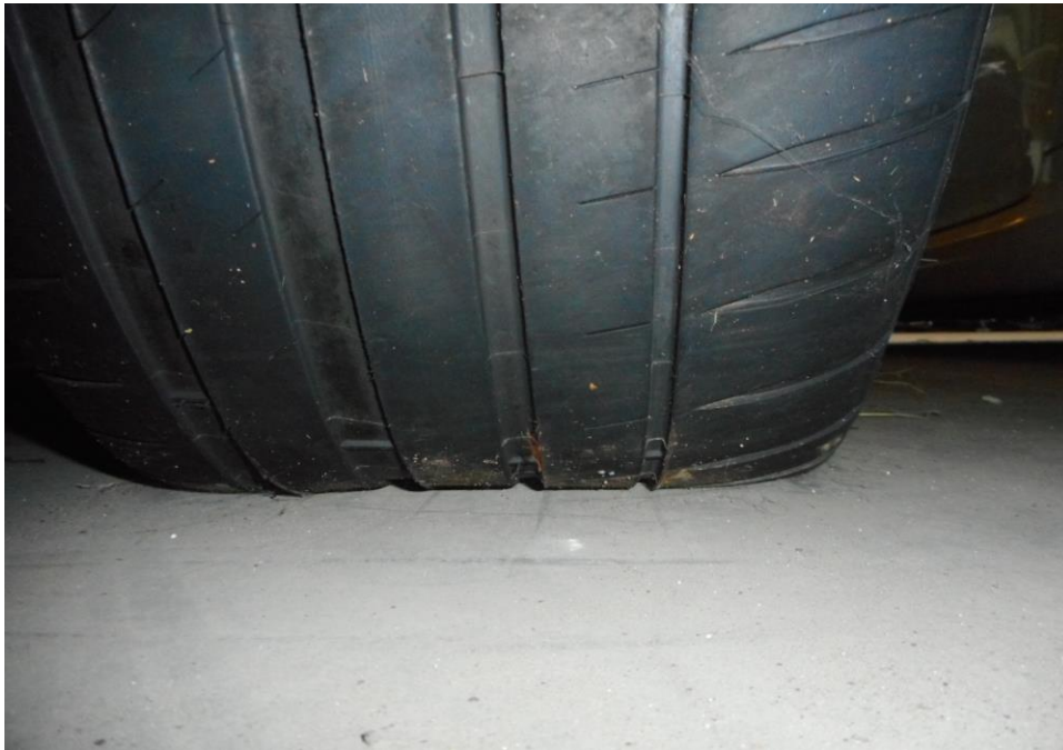
Photo 10 shows the condition of the rear right tyre of the Motor Car, which was observed to be in serviceable condition with remaining tread depth of approximately 3.4mm. The tyre was also observed to be sufficiently inflated for vehicular operation with no tear, cut or burst mark(s).
