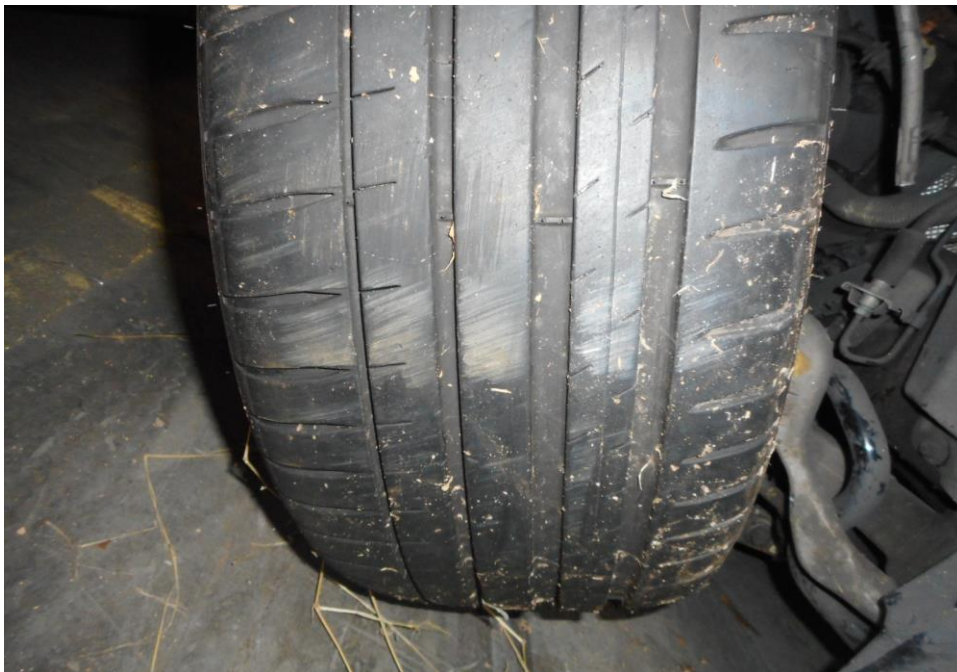
Photo 9 shows the condition of the front right tyre of the Motor Car, which was observed to be in serviceable condition with remaining tread depth of approximately 5.5mm. The tyre was sufficiently inflated for vehicular operation with no tear, cut or burst mark(s) on the outer and the inner sidewalls as well as across the tread. The 4 tyres of the Motor Car were wrapped around standard steel wheel rims without any damage.
