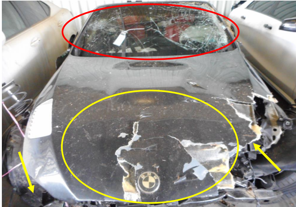
Photo 4 shows a close up view of the Motor Car's front body at the time of my inspection. Its front windscreen (red circle), front bonnet (yellow circle) and both front headlamps (yellow arrow) were amongst the body parts that were damaged as a result of the accident.
