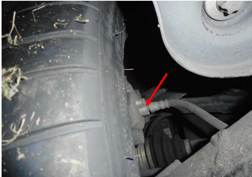
Photo 16 shows the brake hose/pipe (arrowed) at the rear left wheel of the Motor Car. I did not observe any leakage of brake fluid at the time of my inspection of the Motor Car and found to be intact and without any visible damage.
