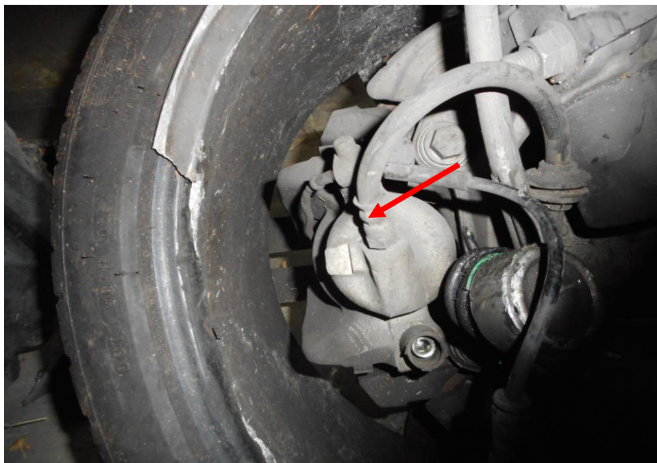
Photo 17 shows the brake hose/pipe (arrowed) at the front right wheel of the Motor Car. I did not observe any leakage of brake fluid at the time of my inspection of the Motor Car and found to be intact and without any visible damage.
