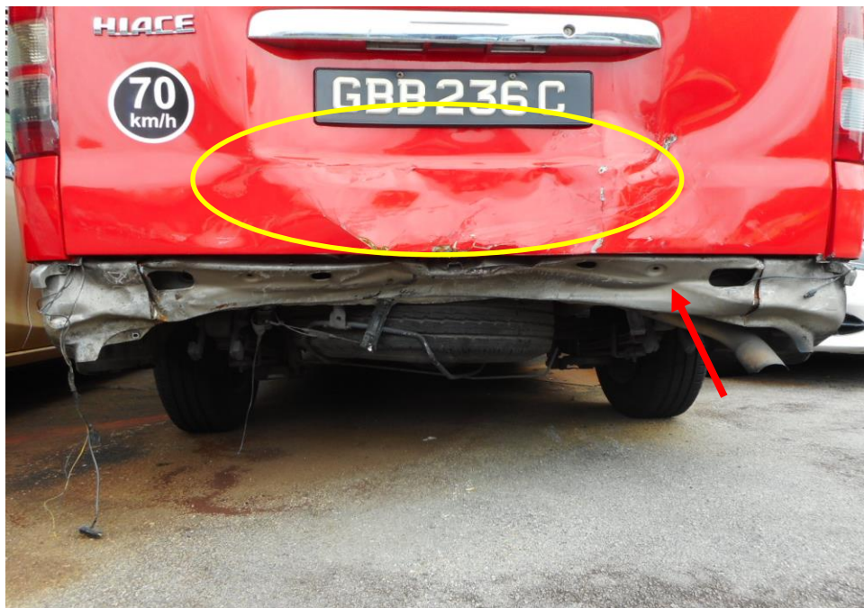
Photo 3 shows a close up view of the Motor Van's rear portion at the time of my inspection. It appeared to have sustained damage at its rear portion. Its rear body panel (circled) and rear bumper (arrowed) was damage at the time of my inspection as a result of the accident.
