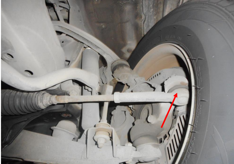
Photo 18 shows the various undercarriage components at the front left wheel of the Motor Van, in particular the steering tie rod end (arrowed). The various undercarriage components of the Motor Van were all found to be intact without any visible damage. There was also no sign of fluid stain(s) observed on the various undercarriage components.
