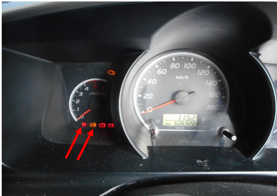
Photo 24 shows the warning light for Anti-Lock Brake System (ABS) and Supplemental Restraint System (SRS) (arrowed) appearing on the instrument panel of the Motor Van during the self-test of its various electronic operating systems when its engine was cranked.
