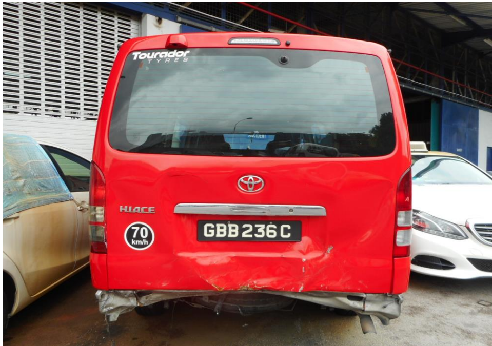
Photo 2 shows a general view of the Motor Van's rear portion at the time of my inspection. It appeared to have sustained damage at its rear portion. Its rear body panel and rear bumper were damage at the time of my inspection.
