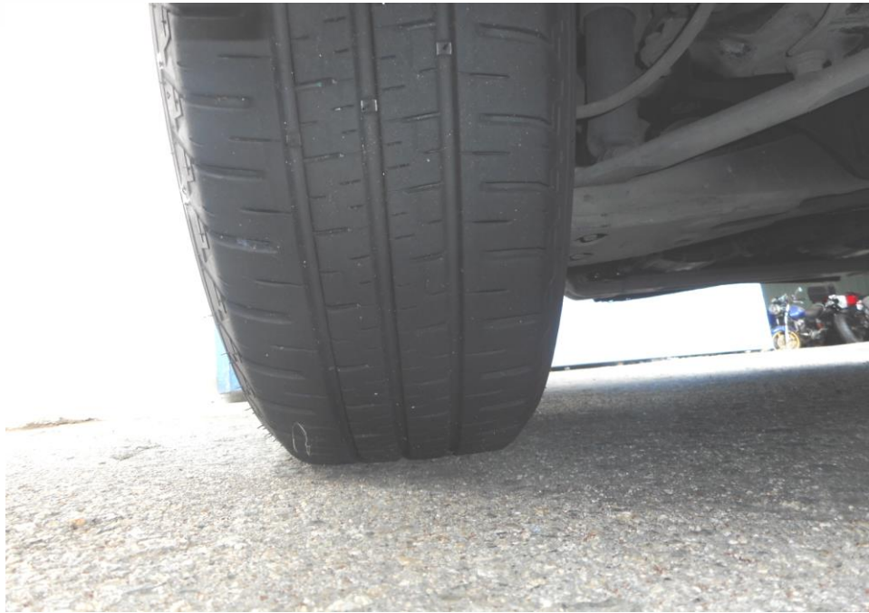
Photo 10 shows the condition of the rear right tyres of the Motor Van, which were observed to be in serviceable condition with remaining, tread depth of approximately 6.2mm. There was also no tear, cut or burst mark(s) on the outer and the inner sidewalls as well as across the tread of the 4 tyres that were fitted on the Motor Van.
