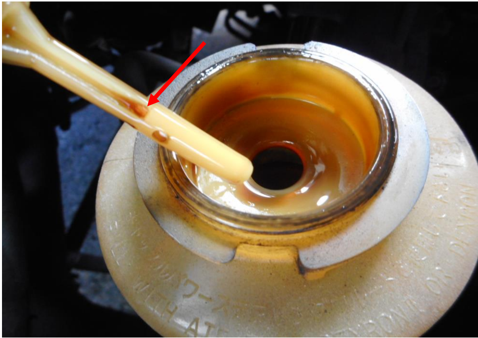
Photo 15 shows the power steering fluid reservoir of the Motor Van at the time of my inspection. The steering fluid was observed to be of sufficient level (arrowed) and without any visible contamination.
