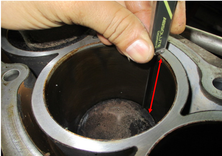
Photo 18 shows measurement being carried out to the stroke (arrowed) of cylinder 3 of the Toyota engine. The bore and stroke measurements of the Toyota engine were carried out using a digital Vernier Caliper that was calibrated before the start of the measurements.
