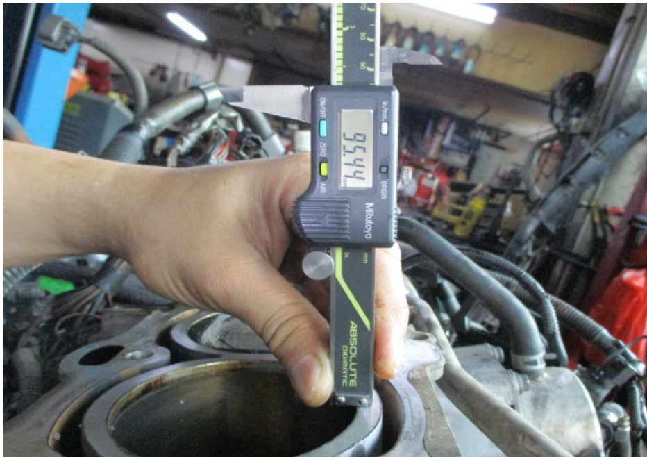
Photo 19 shows the stroke measurement of cylinder 3, which was recorded to be 95.44mm.
