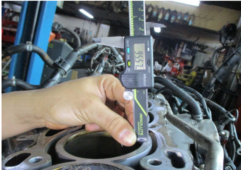
Photo 14 shows the stroke measurement of cylinder 2, which was recorded to be 95.57mm.
