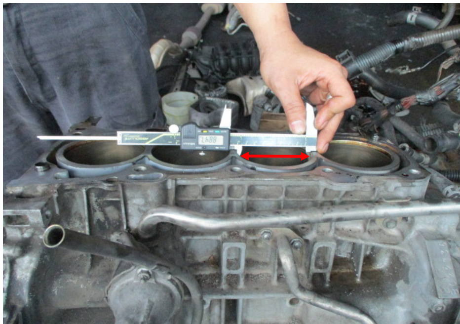
Photo 15 shows measurement being carried out to the bore (arrowed) of cylinder 3 of the Toyota engine. The bore and stroke measurements of the Toyota engine were carried out using a digital Vernier Caliper that was calibrated before the start of measurements. The bore measurement of cylinder 3 was recorded to be 88.47mm.
