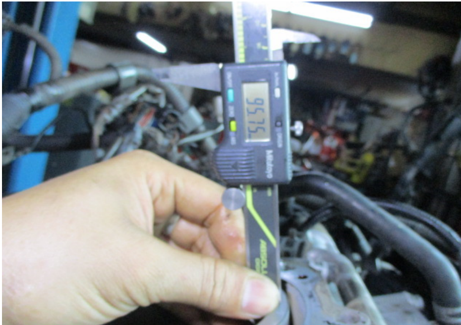
Photo 22 shows the stroke measurement of cylinder 4, which was recorded to be 95.75mm.
