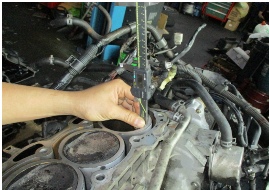
Photo 21 shows measurement being carried out to the stroke of cylinder 4 of the Toyota engine. The bore and stroke measurements of the Toyota engine were carried out using a digital Vernier Caliper that was calibrated prior to the start of measurements.
