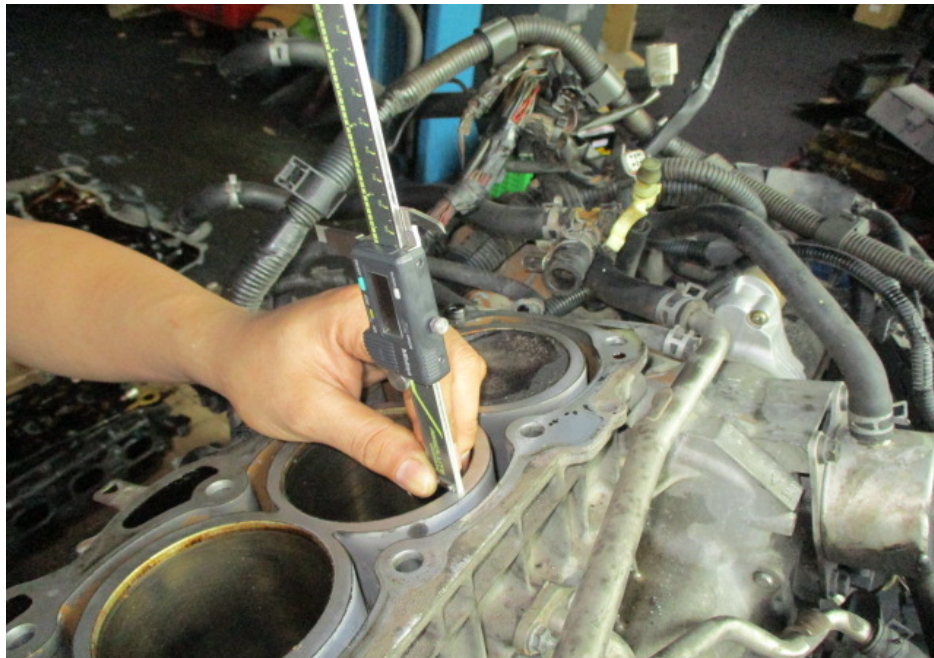
Photo 17 shows measurement of the stroke for cylinder 3 of the Toyota engine that I had inspected. The bore and stroke measurements of the Toyota engine were carried out using a digital Vernier Caliper that was calibrated before the start of measurements.
