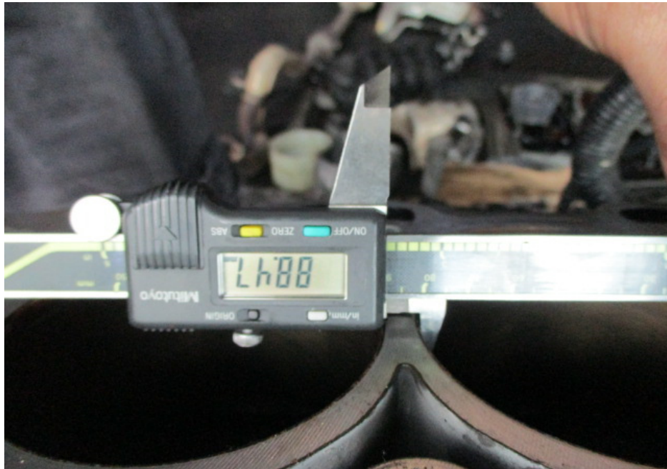
Photo 16 shows the bore (arrowed) measurement of cylinder 3, which was recorded to be 88.47mm.
