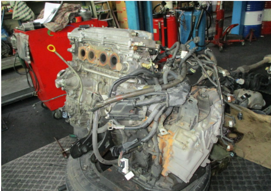
Photo 4 shows a general view of the Toyota engine that I had inspected. The Toyota engine was observed to be a used engine and complete assembly with all mechanical parts still intact, within the engine housing.
