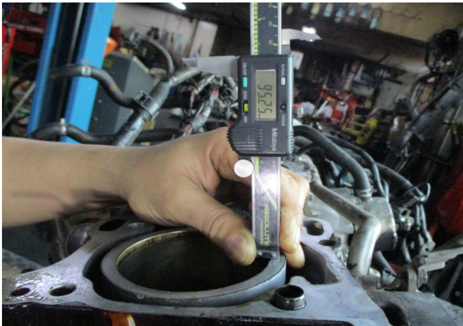
Photo 11 shows the stroke measurement of cylinder 1, which was recorded to be 95.25mm.
