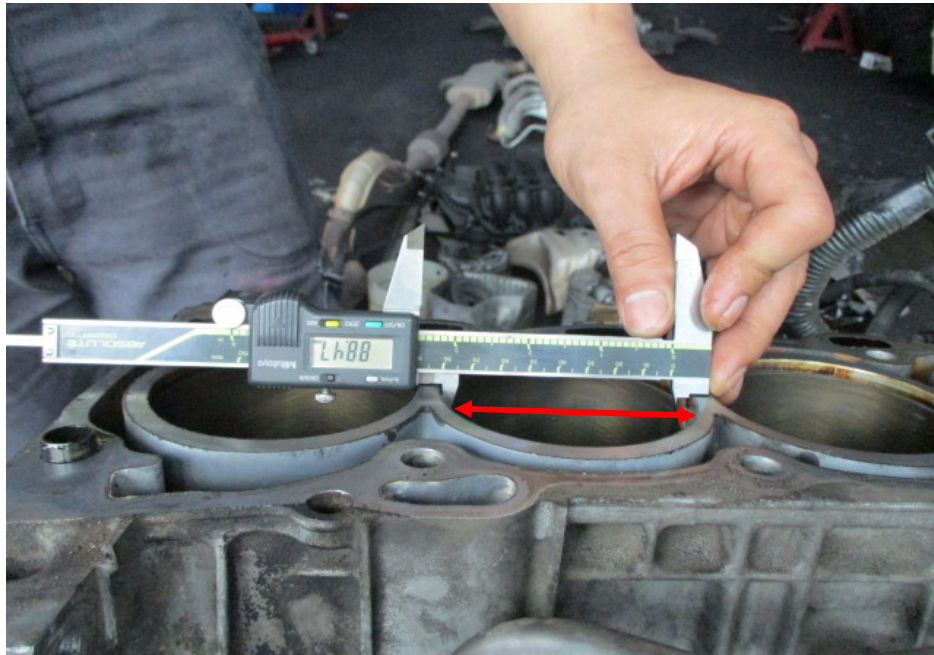
Photo 12 shows measurement being carried out to the bore (arrowed) of cylinder 2 of the Toyota engine. The bore measurement of cylinder 2 was recorded to be 88.47mm.
