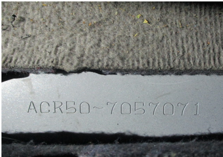
Photo 2 shows the chassis number of the Toyota Estima Aeras 2.4A with registration number SJE 1221C. The chassis number engraved on the driver's side floorboard was ACR50-7057071. This corresponds to the chassis number indicated in the LTA log card of the motor car SJE 1221C.
