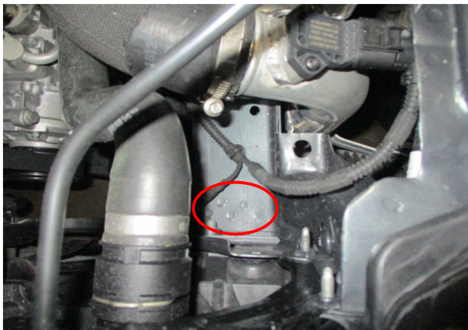
Photo 20 shows the chassis/structural body at the front left of the Motor Car (as viewed from the engine compartment). This was at the section where the front left member joins the front left chassis. I did not find any weld marks other than original spot weld marks (circled) on the chassis/structural body of the Motor Car, indicating no work was done on the chassis/structural body of the Motor Car and that the chassis/structural body was originally fitted.
