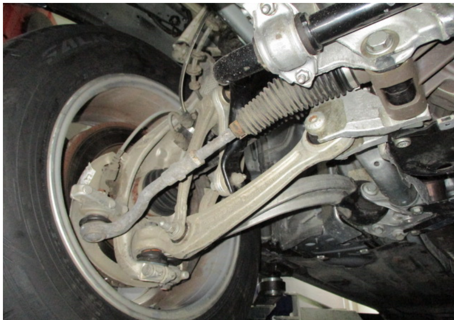
Photo 18 shows the various undercarriage components at the front right wheel of the Motor Car. The mechanical components, control arms and linkages were all found to be intact and secured in an appropriate manner. I did not observe any fluid leak and/or fluid stain on the underside of the Motor Car.
