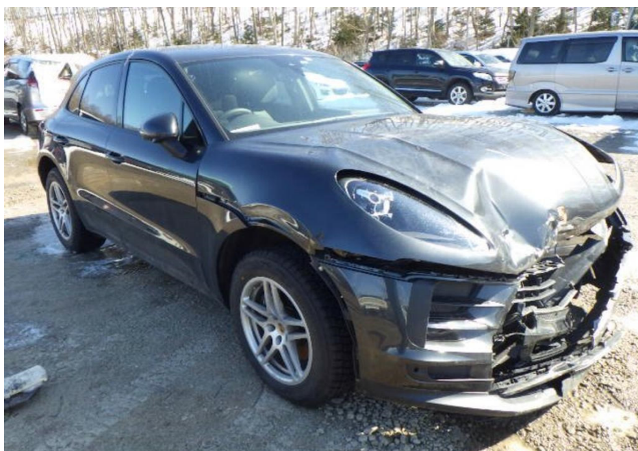
Photo 2 shows the front right body of the Motor Car prior to any repairs being carried out (photograph provided to me). The Motor Car was observed to have sustained damages at its frontal portion. The body parts observed to be damaged had included the front bumper, front bonnet and front right headlamp amongst others.
