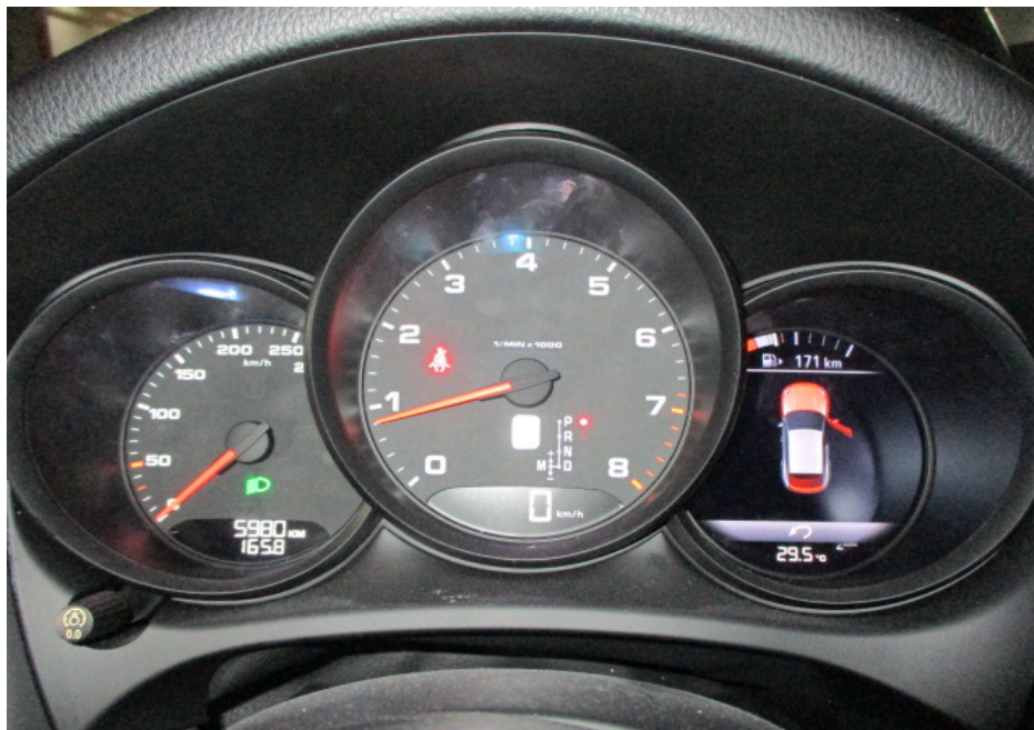
Photo 14 shows the respective warning lights no longer illuminated after the engine was started, indicating that there was no fault detected to the ABS, SRS, TPM and TCS systems of the Motor Car during the self-test. These electronic systems were hence in working condition at the time of my inspection.
