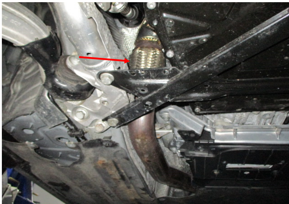
Photo 19 shows the Motor Car's catalytic converter (arrowed). My examination of the Motor Car's exhaust system revealed no sign(s) or indication(s) of any cut or weld marks along its exhaust pipes and on its rear mufflers.
