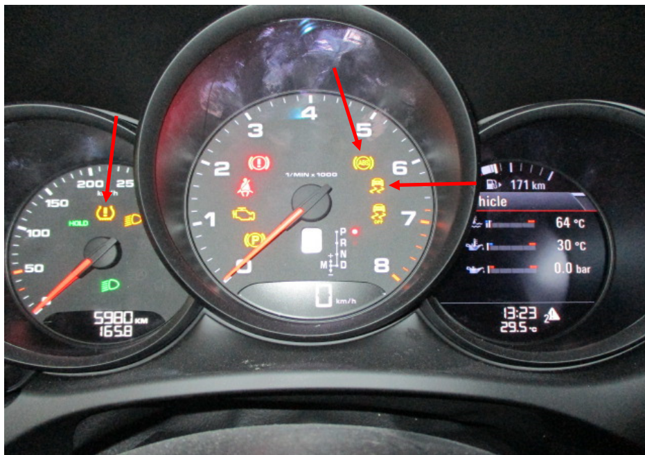
Photo 13 shows the warning lights for the various electronic safety features appearing on the instrument panel of the Motor Car during its self-test when the engine is cranked, in particular the ABS, SRS, TPM and TCS lights (arrowed).
