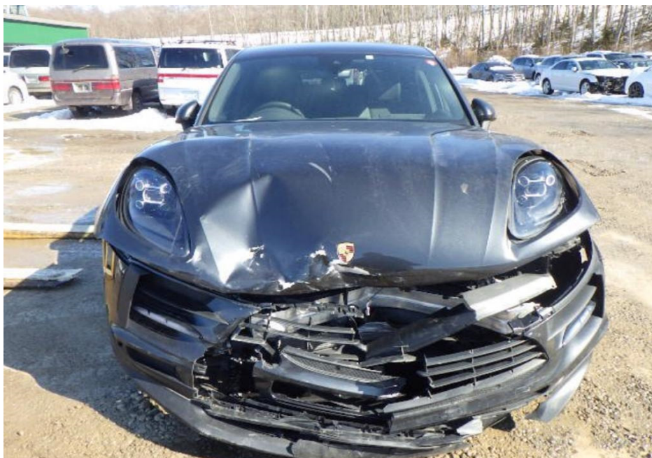
Photo 3 shows the frontal portion of the Motor Car prior to any repairs being carried out (photograph provided to me). The front bonnet, front bumper, front bumper lower grille, front bumper reinforcement and front grille were amongst the body parts that were observed to have been damaged.
