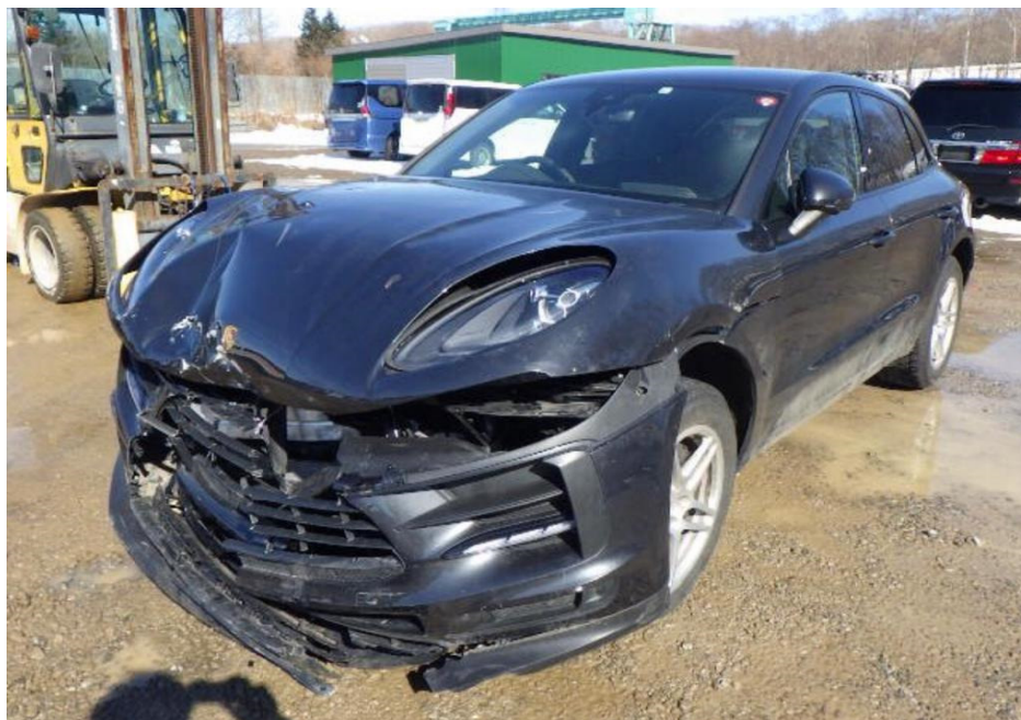
Photo 1 shows the front left body of the Motor Car prior to any repairs being carried out (photograph provided to me). The Motor Car was observed to have sustained damages at its frontal portion. The body parts observed to be damaged had included the front bumper, front bonnet and front left headlamp amongst others.
