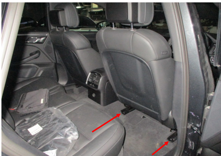
Photo 12 shows the seats of the Motor Car, which were secured via seat rails (arrowed) to the floorboard. All the seats of the Motor Car were fitted with a retractable seat belt reel and pre-tensioner. The seat belts were also able to be fastened into the respective pre-tensions that were fitted on the side of each individual seat.
